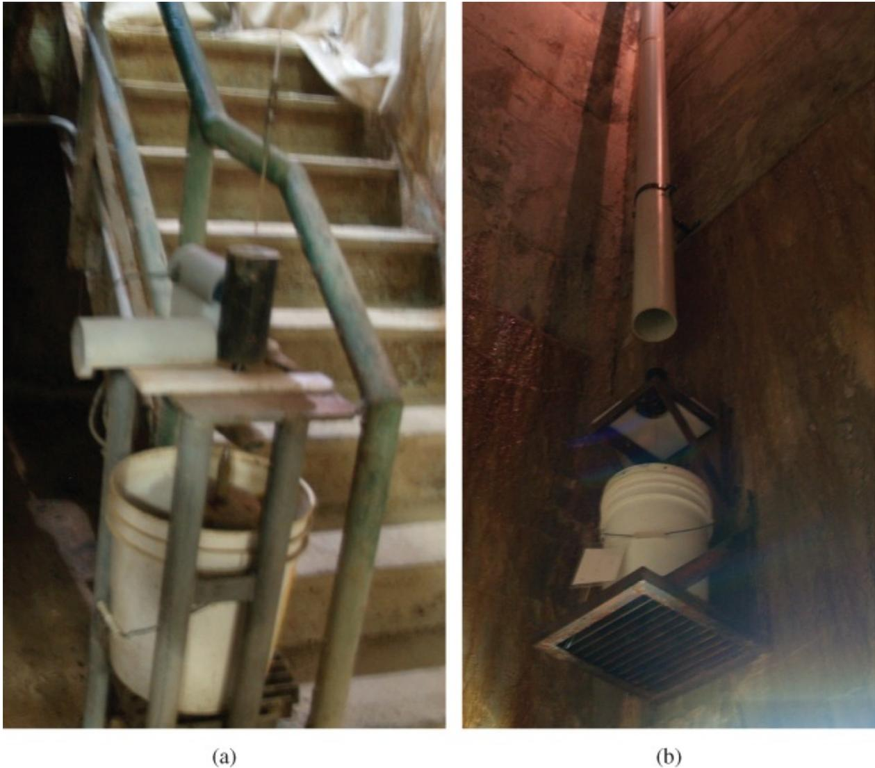
**Figure 11.12** (a) Typical measurement location of stairwell plumbline in a Powerhouse. (b) Typical measurement location of hoist well plumbline in a Powerhouse.
