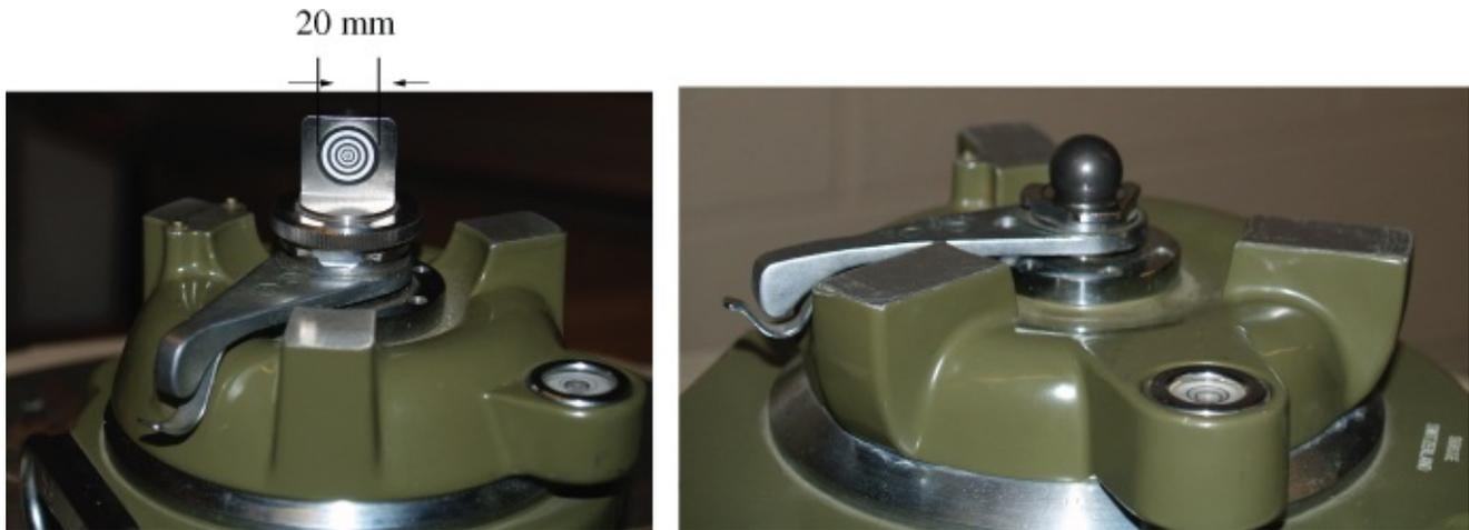
**Figure 14.19** Spherical target and Kern concentric target (for sights of over 4–40 m) set in Kern trivets.
