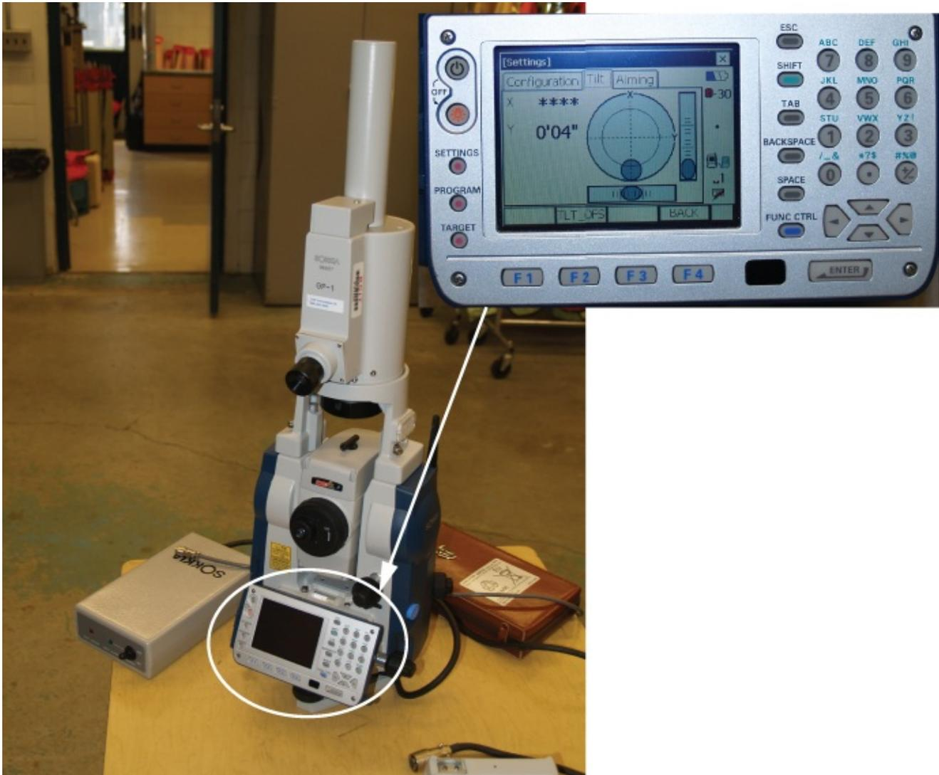
**Figure 12.9** GP-1 gyro unit mounted on Set3X total station.
