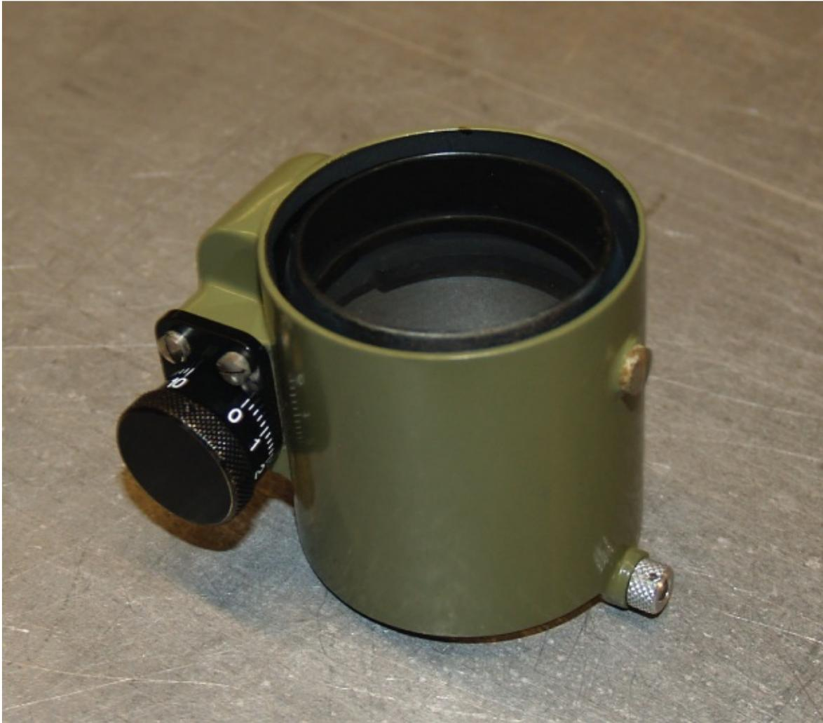
**Figure 14.13** Optical micrometer attachment (graduated to 0.05 mm) for Kern GK23 tilting level.
