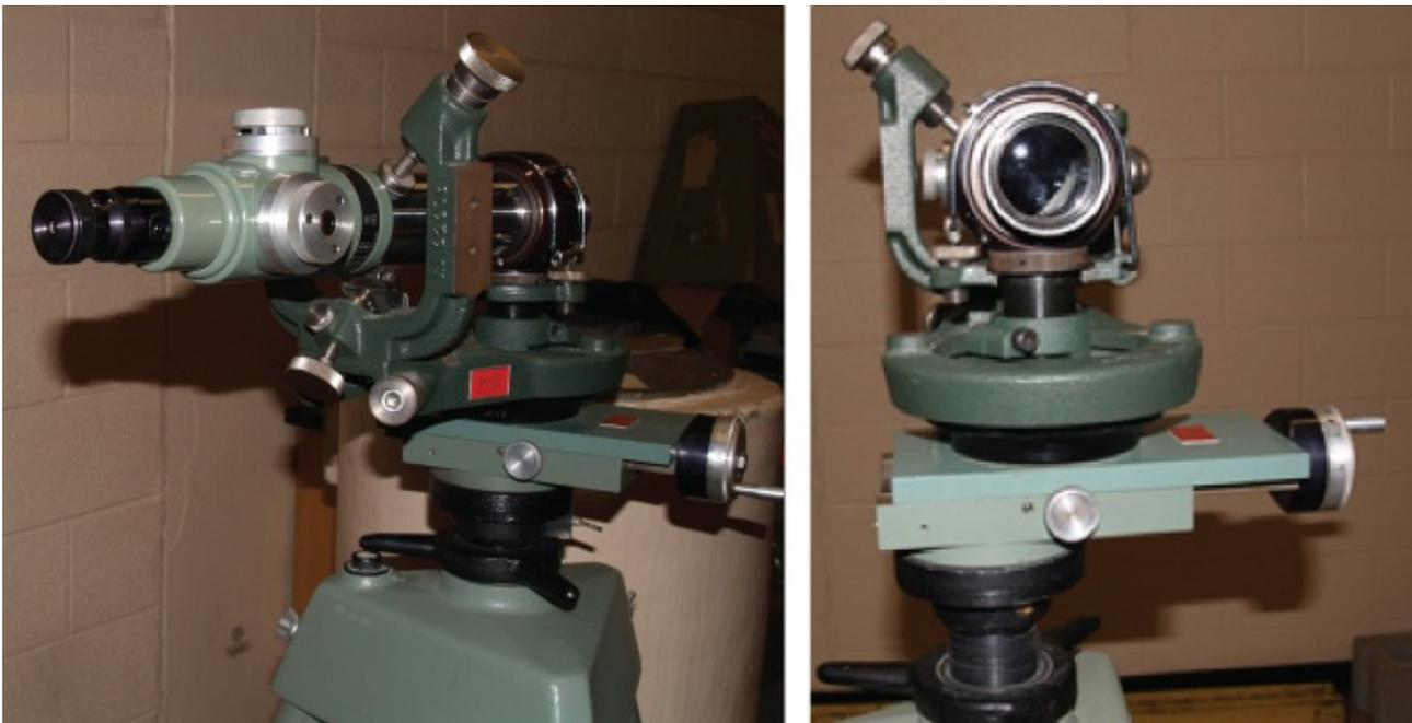
**Figure 14.10** Side and front views of mounted alignment telescope.
