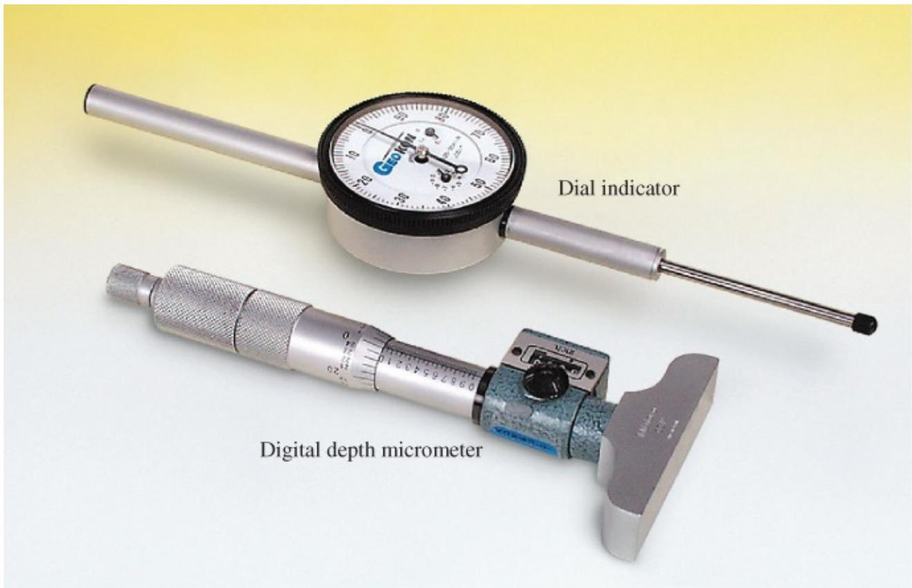
**Figure 11.1** Two mechanical devices for reading rod extensometers.
