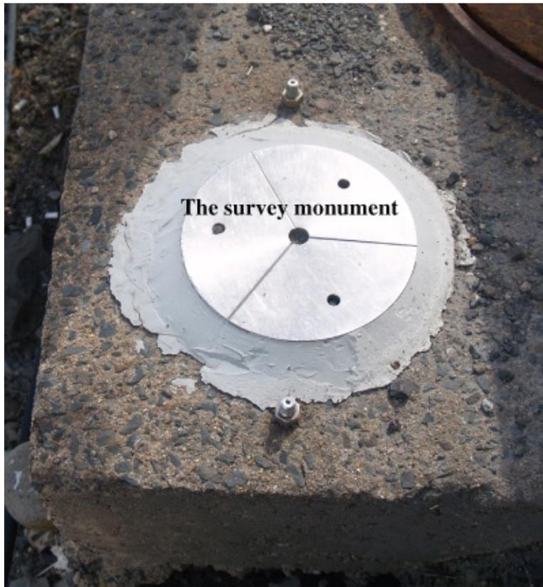
**Figure 9.4** A typical dam crest monument installation.
