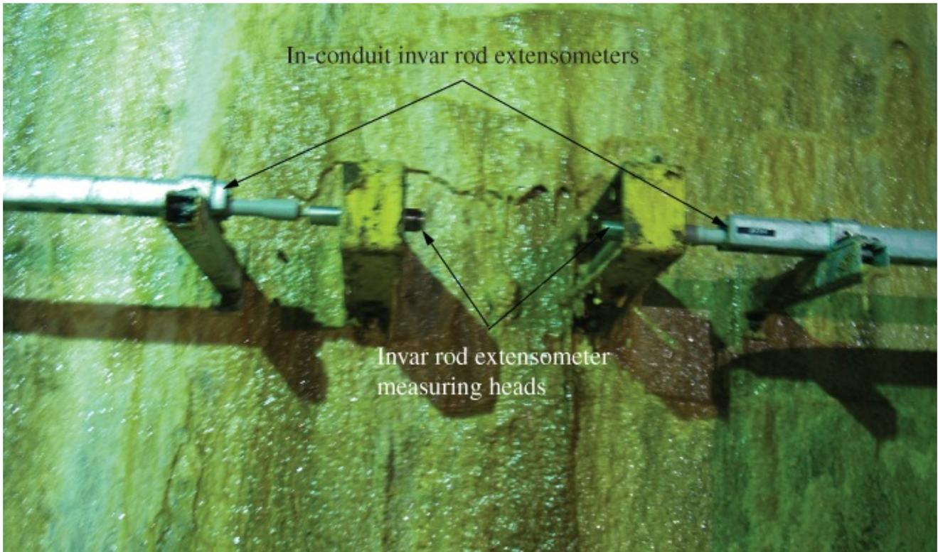
**Figure 11.6** Invar rod extensometer installation with the measuring heads (with micrometer measurements usually taken between the two heads).
