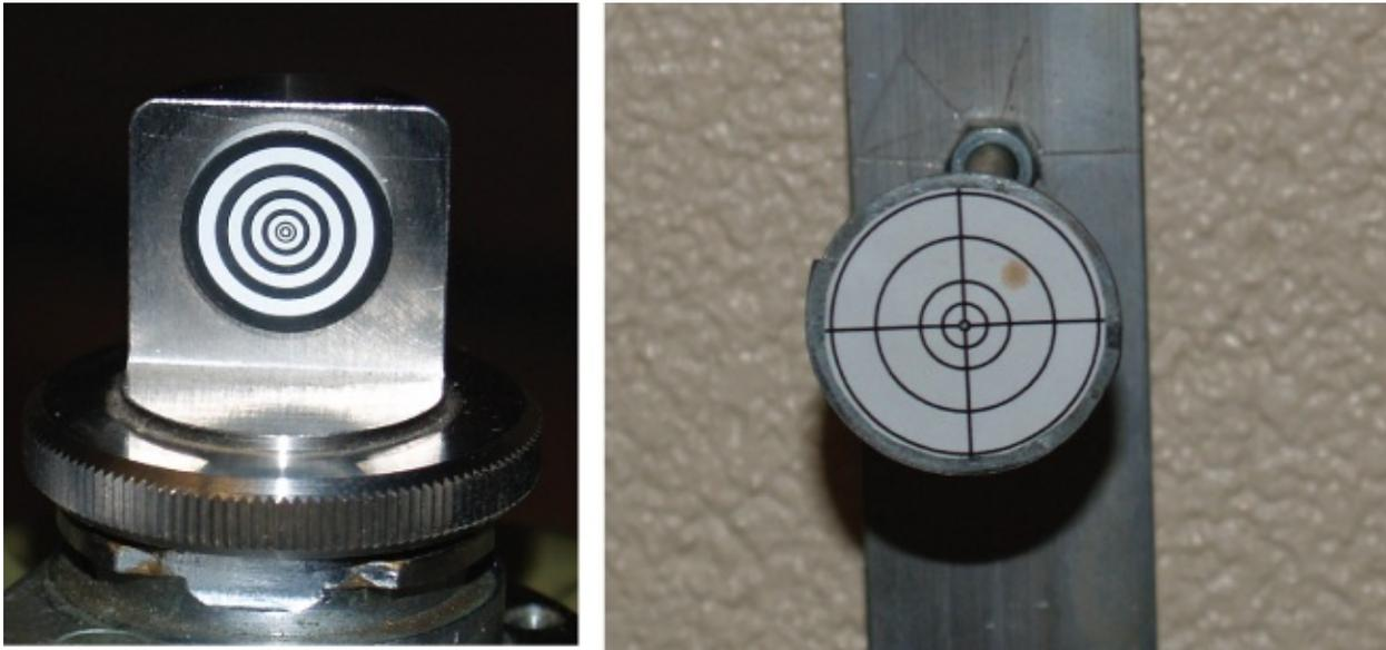
**Figure 14.5** Concentric circle wall target designs.
