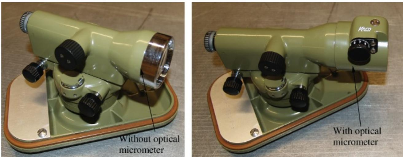
**Figure 14.16** Kern GK23 tilting level without and with optical micrometer.
