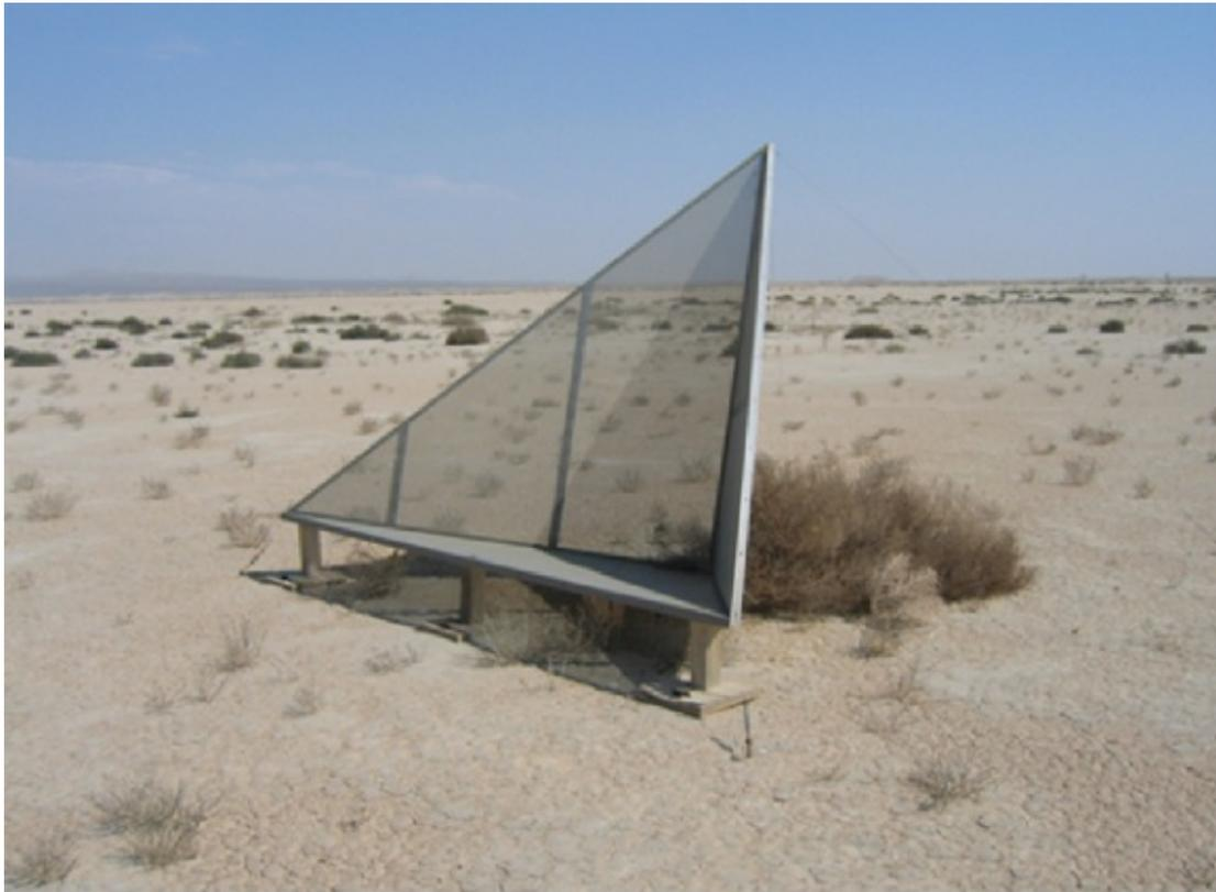
**Figure 10.8** Typical artificial corner reflector.
