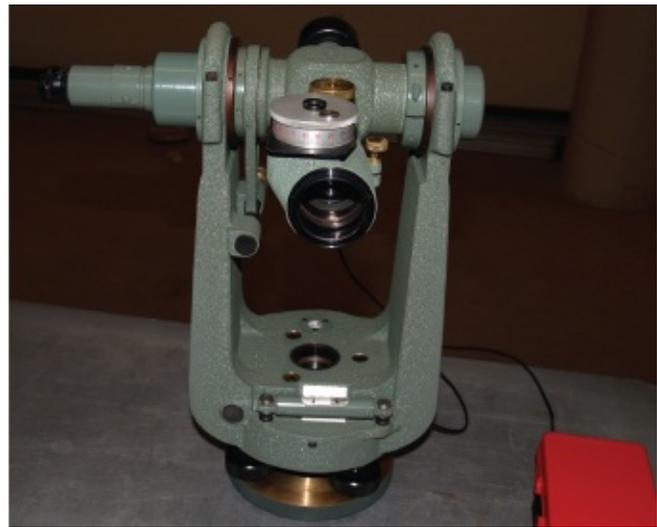
**Figure 14.11** Side and front views of the Jig transit showing an autocollimation unit with a light unit mounted on the viewing end.
