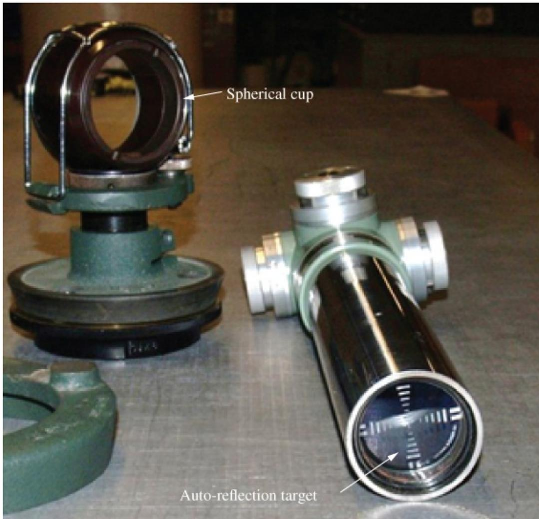
**Figure 14.8** Spherical cup being supported on a large-diameter screw thread in the base of the mount and the alignment telescope showing the auto-reflection target in the objective lens.
