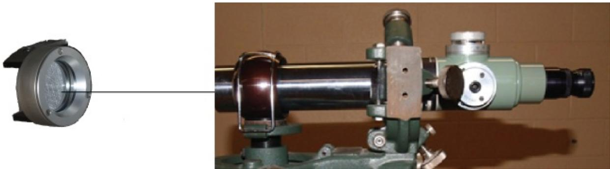
**Figure 14.22** Alignment telescope set for autocollimation/auto-reflection.
