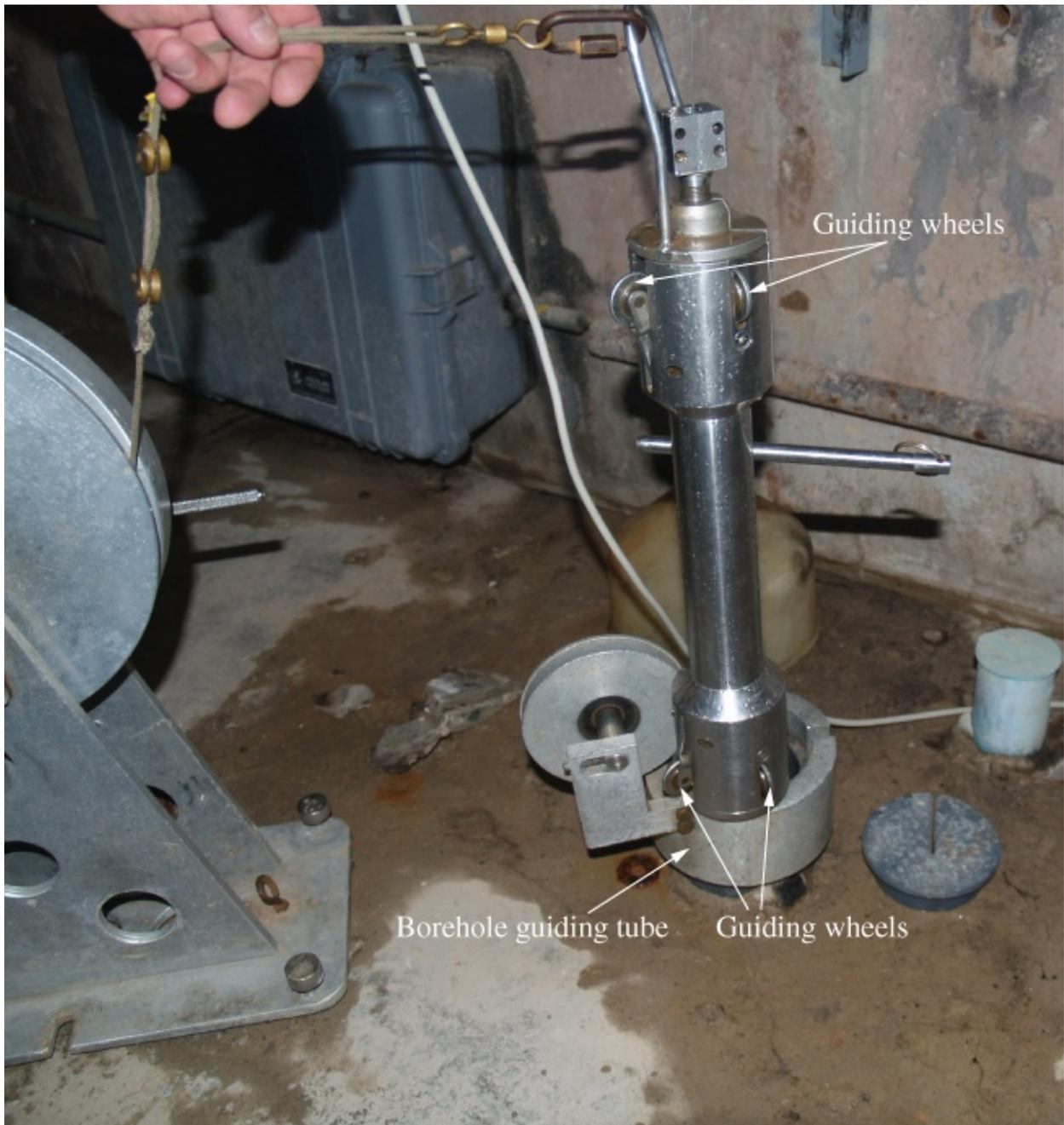
**Figure 11.20** A shuttle probe being lowered into a borehole guiding tube.
