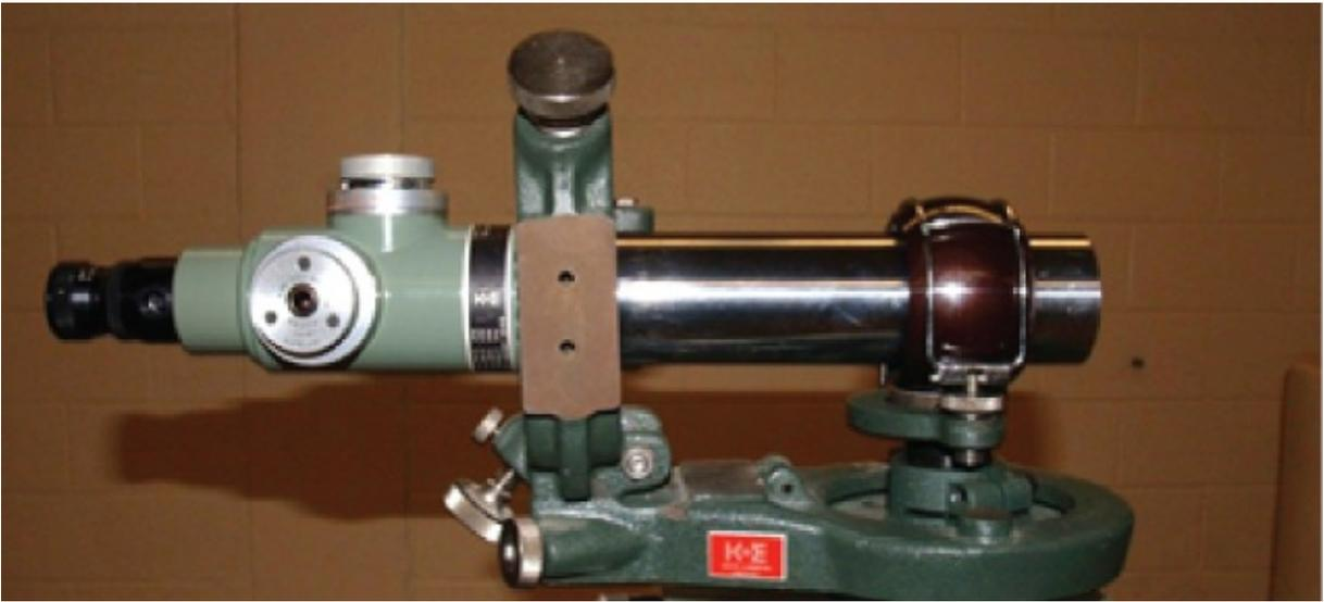
**Figure 14.9** K&E Paragon alignment telescope set in an alignment bracket.
