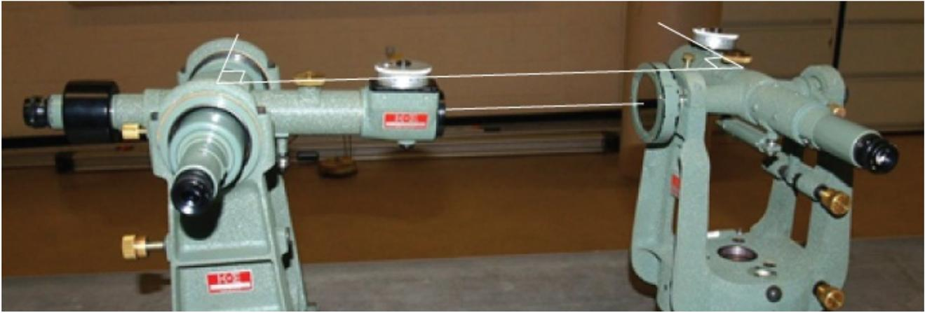
**Figure 14.23** Setting out 90° angle by autocollimation or auto-reflection using side mirror.
