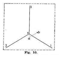
wise; and 2nd, that to put the plate level, the legs must be swung sidewise but not on their pivots. These two points, though small in themselves, are worth remembering as a means of saving time and labor and also of preventing unnecessary wear and strain on the leveling screws owing to faulty construction of the leveling appliances. With many instruments the last point is a very important one.
