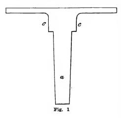
neer has a transit or leveling instrument, in which the upper part is detachable from the leveling screws. This requires a good drawing board, say 18 by 20 inches, to the under side of which is screwed a casting of iron or brass similar to Fig. 1. The conical portion, a, should be made to fit the socket from which the axis of the level or transit is taken; the cylindrical portion, cc should fit in the lower clamps.
