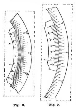
is called a double folded vernier. Thelower numbers on one side of the zero and the upper ones on the other side constitute a vernier. The proper vernier to be read, in any given case. can be determined by either of the rules of the preceding article. The vernier as drawn. reads  $2^{\circ} 30' + 12 = 2^{\circ} 42'$  to the right. Notice that the reading of the vernier is 12' not 17'.
