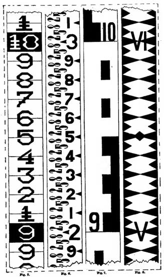
In its essential features, Fig. 7 is the favorite British self-reading level rod. The graduation is to hundredths. Although the one shown is better than the typical English rod, it cannot be considered a good one for the same reason for which the usual target to the New York rod is condemned in a previous paragraph.
