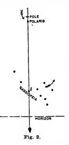
tive position of the stars at the time of observation is shown in Fig. 2. The line determined by observing these stars June 1, 1886, will be within 1" or 2" of a true meridian and will move *east* about 25" per year.
