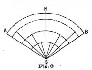
of any level surface, erect an upright staff, shown in horizontal projection, at S, Fig. 3. 'Two or three hours before noon, mark the extremity, A, of its shadow. Describe an arc of a circle with S, the foot of the staff, for a center, and SA, the distance to the extremity of the shadow, for a radius. About as many hours after noon as it had been before noon when the first mark was
