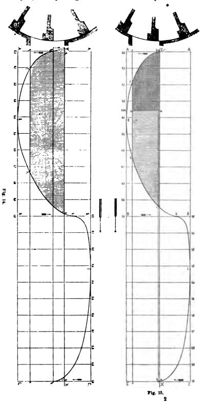
stroke is rendered possible, though it is at once apparent that towards the approach of the cut-off, the steam is much throttled. Continuing its travel the valve progresses to lap rapidly, so much so that the lap is already <sup>15</sup>/<sub>16</sub> in. at the stroke-end. The return-travel begins at first very slowly, but is accelerated towards the stroke-end, so that it may open comparatively rapidly for a fresh steam-supply.
