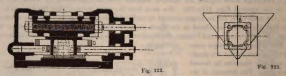
rectangular to the cylinder axis, is thereby imparted to it. The two other sides of this shoulder, are carried in the frame D, which by means of the governor or a lever, can be shifted vertically to the slide-stroke. The two valves are drawn in their central-position. A plate F, is fitted to the expansion-slide, for balancing purposes.
