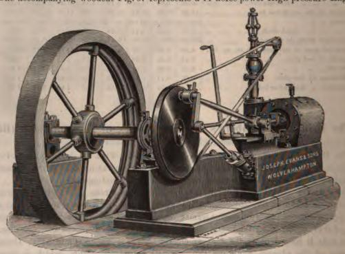
with Pickering's high-speed governor, of which Fig. 68 gives an enlarged view. The form of the bed is characteristic, and the same remark applies to the idea of using the crank-disc as governor
