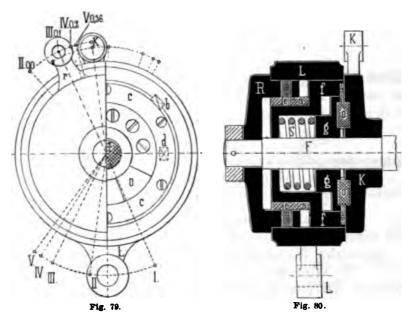
disc K and spindle F are similarly turned, and the inlet valve is opened. This motion however merely continues so long as the pins are sliding in the straight portions of the grooves ee, for as soon as the pins get into the slanting portions of these grooves, the lever r being held firm in a given position from the governor, the box f and plate g are drawn back. The teeth oo beUbland-Tolhausen, Corliss-engines.
