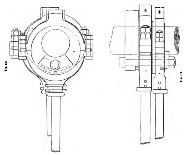
The usual way of fixing the cross-head o the piston-rod, is by keying it on the rod which is slightly tapered at the end; but in this plan, no compensation can be made, for the Uhland-Tolhausen, Corlins-engines.
