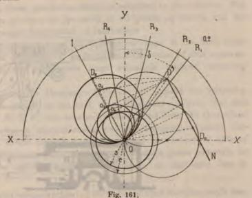
the shifting of the links, the end  $D_0$  moves on the straight line  $D_0$  D, and consequently that the end-points of the relative circles  $o_2$ ,  $o_3$ ,  $o_4$ , also come to lie on a straight line. These points may
