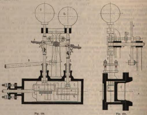
The main-slide G, made very large and after Meyer's principle, is worked as usual by an eccentric. The back of the slide is furnished with two steam-ways, arranged vertically to the
