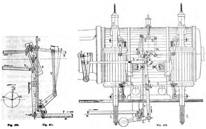
The corresponding external valve-gear is reproduced in the annexed woodcuts Figs 270—272, to which we adapt the description given by "Engineering"\*). It is, like all the other larger winding engines, a double cylinder engine, the two cylinders and frames being entirely separate, and the drums and brake placed on the shaft between the two journals. The general form of
