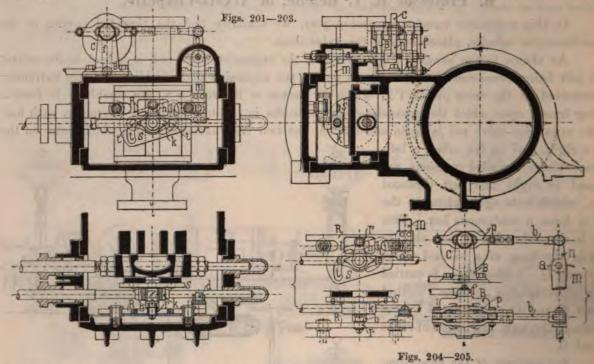
with each oscillation. The one end of the bolt carries a pin d, which fits in the longitudinally slotted hole of a lever m; the axis (a) of the latter is passed out of the valve-box through a suitable stuffing-box and is lightly carried on two pointed studs. The lever n is mounted on the same axis a in the manner shewn.
