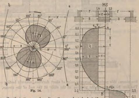
the deviation is so small, that it may be altogether neglected, but if strict accuracy is desired, then the travels of the slide may be corrected in a similar manner to the one described for the piston-travels (vide Fig. 13). Still, such a far reaching method would probably only recommend itself in complicated valve-gears, by using a model.
