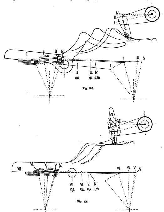
so far screwed through the governor-frame, as to press back the shoulder of the governor-rod. Togovernor-balls are thus brought almost instantaneously and without much trouble, into their high position; this position of the governor, answers to a cut-off at 0.0 stroke, which naturally implement to the cylinder, consequently the engine, is brought to a standstill.
