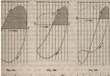
edy a closing action as possible: This is clearly demonstrated e valve-lift diagrams shewn in Figs. 294—298 in which, the shewn above the horizontal line AB indicates the valve-lifts at 3, and 0.8 stroke, whilst the lower curve represents the casual distoff the valve lifting catches. The diagram drawn in Fig. 298 ponds to the exhaust-valve lift, which remains constant for all expongrades.
