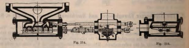
steam off, the lugs p and q no longer come in contact with the worm o. The governor is fitted with two additional spiral springs, whereby the normal engine speed, may be varied.
