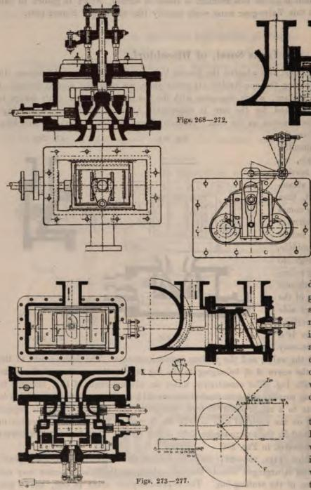
defect of the Farcot valvegear, which as already stated, consists in the limited degree of expansion, is said to be remedied in a number of modifications, embodying the application of a second eccentric, and which thus permits all grades of expansive-working.
