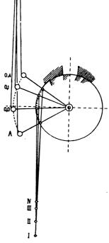
by the upward stroke of this rod S. The same lever L also carries a small rod e to which is attached the piston of an air-cylinder Q, exactly constructed as explained on page 21, and illustrated in fig. 35. As soon as the bolt R (connected as shewn by the link-mechanism with the governor) begins to play on the inclined surface of the steel rod S, the latter becomes disengaged from the Uhland-Tolhausen, Corliss engines.
