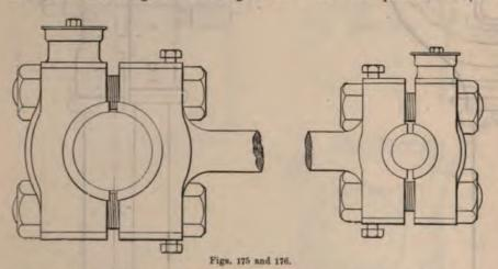
can be ensured in the turning and shaping. The brasses are circular, both inside and out, and can be easily re-made in a common lathe, without any fitting. The brasses are kept in their place, by wrought-iron covers secured by strong bolts; and between the cap and the T end of the rod, a number of very thin steel washers are strung upon the bolts. When it is neces-
