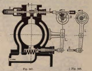
spring-action forces the valve to close. The exhaust-valve H is also driven from the lay-shaft A, by means of the fixed cam K — shewn in Fig. 248 — which articulates a double lever L, the arm  $L_1$  of which is connected with the exhaust valve-spindle.
