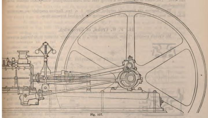
fitted with this gear. An engine of this type is represented in the annexed Fig. 157, as built to the following sizes:
