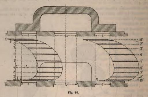
live steam; this period is however only of short duration, scarcely lasting over \(^1\)/<sub>10</sub>th of the stroke. The line 10—0' shews the position of the slide at the end of the stroke, and is similar to the line we first passed under review.
