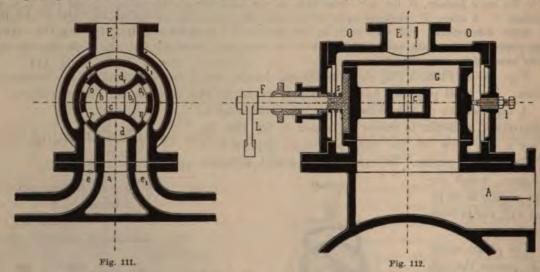
cating with each other — escapes through a into the exhaust-pipe A. The means adopted, for balancing the valve, are the same as we noticed, when describing the Wilson & Schwartzkopf valves.
