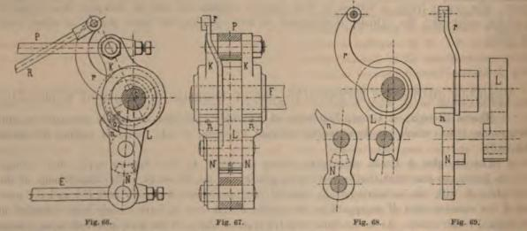
centre of the links NN will be pushed further or nearer to the fixed valve-spindle centre. It is this receding and approaching movement of the links NN, which disengage or set in gear the points or catches nn and the steel nibs oo. When disengagement ensues, the inlet-valve is closed
