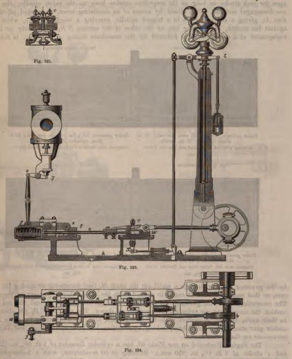
The anchor-gear — Fig. 6 — is worked at the foot of the governor stand by an oscillating or "wrist plate", A, which receives its motion from an eccentric on the engine shaft. On this land-Tolhausen, Corliss-engines.
