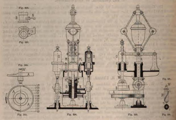
in alternately lifting the valve-spindles  $FF_1$  — corresponding to the opening of the valves of slides — so as to admit steam from 0.0 to 1.0 stroke, if the disengagement mechanism should not previously come into play to close the valves.
