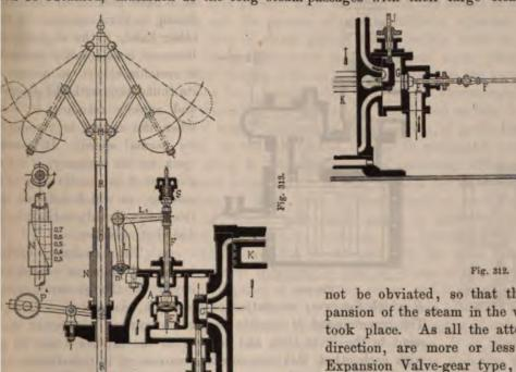
not be obviated, so that the simultaneous expansion of the steam in the valve-chest etc. still took place. As all the attempts made in this direction, are more or less based on Meyer's Expansion Valve-gear type, we begin this last section of our "Corliss-engine" Work with the latter, and illustrate the same by Fig. 312.
