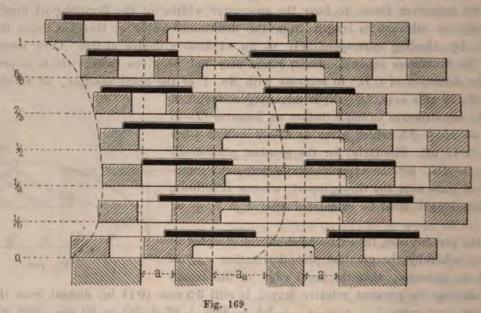
shew themselves in this respect, than later cut-offs. In Fig. 169, we have still further elucidated the slide motions. The valves are shewn over each other, corresponding to piston-positions inscribed as at 0, ½, th, ½, rd, ½, 2/3 rds, ½, ths and full stroke. Expansion begins at ½, stroke.
