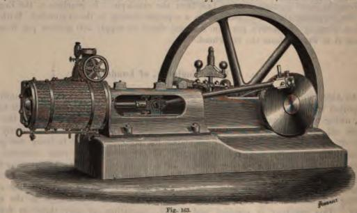
sizes, from 10-35 HP. The condenser in this class is adapted to quick speeds, the valveseatings are of brass, with India-rubber valves. The Air-pump is connected to the tail end of the piston-rod, and a suitable distance piece is introduced between cylinder and condenser to
