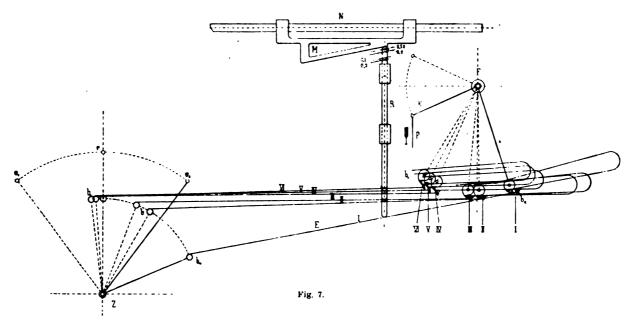
between the initial and end-positions of both the lever L and the rod E from each other is therefore much greater between the earliest cut-off and a cut-off at  $\frac{1}{10}$  of the stroke than the distance between the posi-
