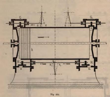
levers CC1, which gear into slots of the valve rods FF1, consequently with the assumed direction of travel, the right-hand valve begins to move while the left slide G, remains closed and stationary, and at a certain expansion-degree the catchbolt n will clear the levernib N. Owing to the steampressure exerted on the endarea of the valve-spindle as well as owing to the dashpot piston weight, the closing of the valve is effected.
