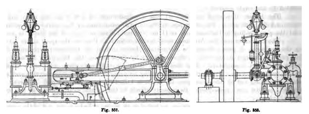
The condenser and air pump are placed below the bed-plate. The pump is single-acting, worked from the crank-pin through the system of levers, whose centre lines are shown in Fig. 357. The vacuum attained is said to be very good.
