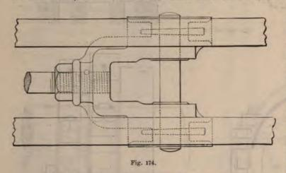
When it is found, that the connecting rod has become shorter, through the wear of the brasses, the guide bars are temporarily taken off, the pin is taken out, and the cross-head unscrewed, as many threads, as are equal to the diminished length of the connecting rod. The pin is then reinserted, and the distance between the piston and the crank shaft becomes, the same, as when the engine was new, and the clearance between the piston and the two cylinder covers, will be perfectly equal.
