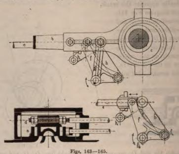
attached to the end of the adjustment-lever  $h_1$   $h_2$  whose fulcrum is a fixed point. We obtain in this manner a range of expansion lying between 0.0 and 0.9 stroke.
