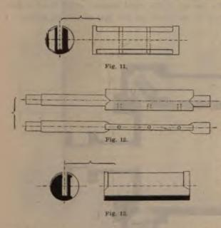
in its extreme open position (vide fig. 10 top right-hand corner). The outer surface of the valve is merely worked up at its ends and seatings, the other portions being kept somewhat recessed for convenience of casting.
