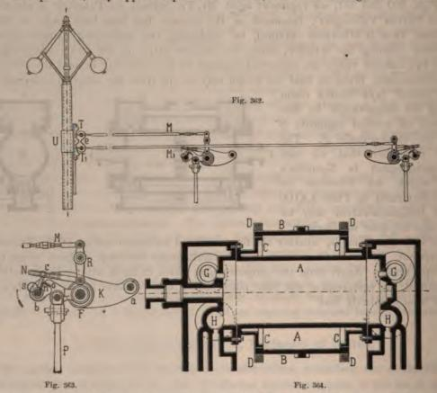
have already observed, that regard has been paid to this question by several Engineers. A rule, the unequal piston-motions were compensated for, by giving different forms to the gover knocker-offs, so that the two admission valves on each cylinder-side, shut-off steam, when piston was exactly at equal distance, from one stroke end as it was from the other.
