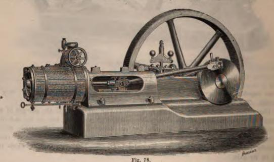
observe that the present design is a modification of an older design with box-bed pattern and inside crank. The cylinder is cast separate with an inner lining of very hard metal, which simultaneously forms the steam-jacket. The slide- and piston-rod are of steel, and the slipper block is made adjustable. The difference between this engine and the one previously illustrated in Fig. 163 (Vol. II) lies in the governor, and in the addition of an adjustable eccentric for obtaining variable expansion.
