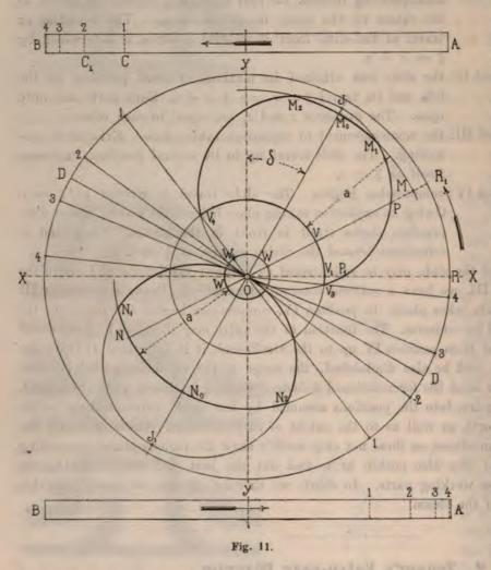
from its neutral position, when the crank is thus placed. The upper circle denotes the path of the slide to the right, whilst in the lower circle, we have represented, the travel of the slide in opposite direction—return stroke; — as both are symmetrical to each other, it suffices in most cases, to draw merely one of these circles.
