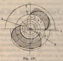
tends over 4 per cent of the stroke, while compression is limited to 71/2 per cent. Consequently, the steam-exhaust during the piston-stroke calculates itself to 921/20/0.
