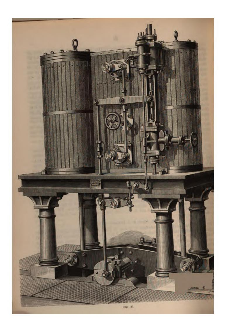
The action of the steam is consequently as follows: The steam from the boiler, enters the high-pressure cylinder forcing its piston down; the cut-off for this cylinder, subsequently takes place at about half-stroke, and the steam is allowed to expand during the remainder of the stroke. After this, it passes into the outer cylinder, where the expansive working is continued; ultimately the steam escapes through the lower, engine-chamber into the condenser or into the atmosphere.
