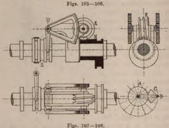
each other. The segment being the driver, the latter will make equal revolutions to the crank-shaft. If we now conceive the counter-shaft to be rotated by some external means, (even when the main shaft revolves,) then an accelerated or retarded motion may be thereby given to the loose wheel, and
