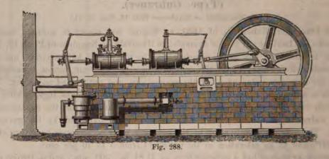
which works on a spindle driven by wheel gear at the same number of revolutions as the crank shaft. By prolonging this spindle it may also be used for driving the governor. The cam is raised or lowered by the action of the governor, and thus cuts off the admission sooner or later as the load necessitates.
