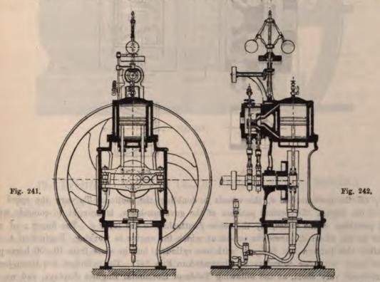
the annexed illustrations Figs. 241—247, shewing this arrangement to vertical and horizontal designs. Two piston rods are used, as may be seen in Figs. 241—242. Constructed in this manner,
