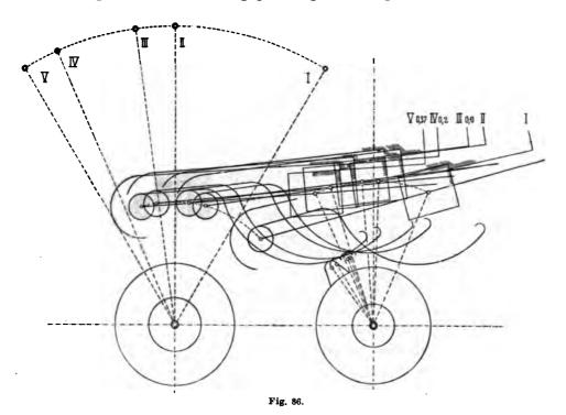
As this drawing explains, the automatic cut-off, lies within narrow limits in this arrangement, worked as it is by one eccentric. Our outline was drawn under a presumed lead-angle of 15°.
