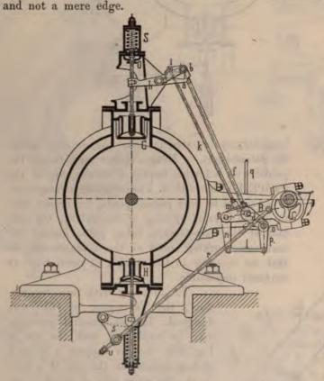
The great advantages possessed by this valve-gear, as displayed by its adaptability to high piston-speeds, and by its feeble reaction on the governor, are increased by its suitability to all Engine-types, whether for Winding or Marine purposes.
