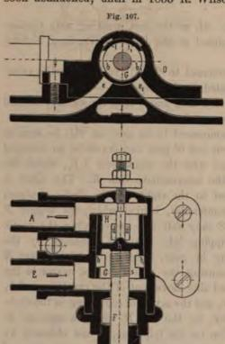
valve. The latter was largely used for Steam-hammers, but at the present time, it is very seldom fitted to Steamengines, because Corliss-valves have been largely used instead.
