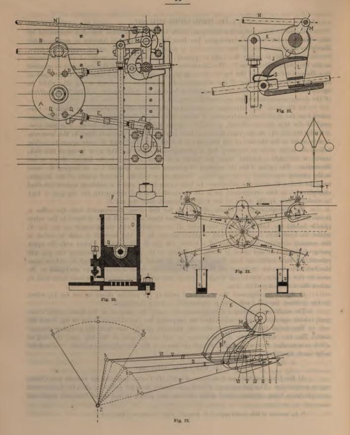
especially in the application of springs instead of weights for the closing of the valves. This fifth arrangement was patented by Corliss already in 1859, though on account of the time at which it became known in Europe it is sometimes called the Corliss valve-gear of 1867. Additional importance is attends this arrangement owing to the first application of a bayonet-formed support commonly known as the Corliss engine frame.
