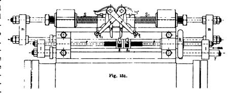
The annexed woodcuts Fig. 150 and Fig. 151, represent a double slide-valve designed by H. Ochwadt of Louisenthal, near Saarbrücken. It is specially adapted to High-speed Engines such as Marine or Locomotive-engines, and its chief characteristic consists in its working up to any degree of expansion or cut-off, without requiring any expansion-eccentric.
