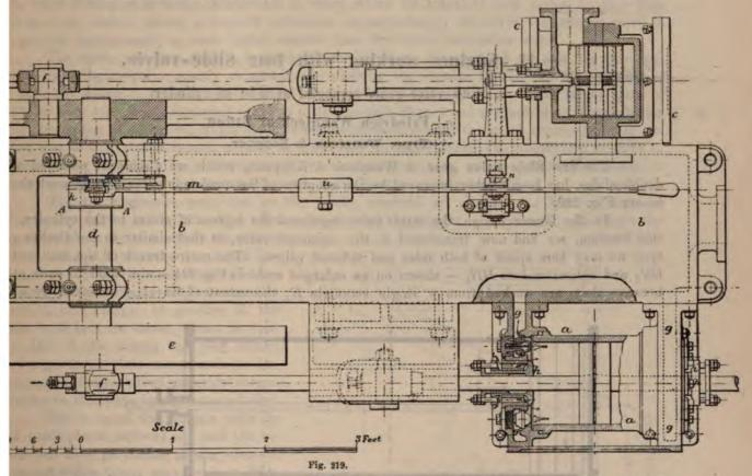
ve, according as the air-pressure, in the receiver, rises above or falls below, the desired working essure. It is claimed that this arrangement acts almost without friction, and is consequently re sensitive, being also less complicated than the first-named method.
