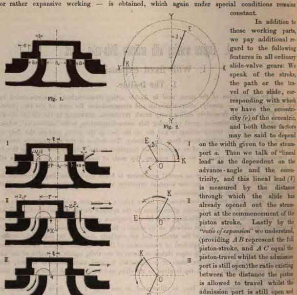
$\frac{AC}{AB} = E = \text{ratio of expansion}$ As the crank may rotate in either direction - i. e. in the same of in opposite directions to the erdinary watch fingers - the ad-
