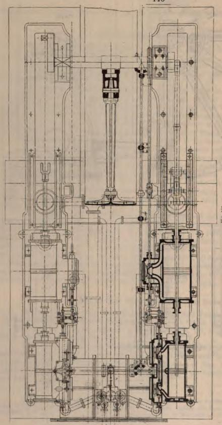
The Engines are of the tandem type, constructed to develop a power of 650 horses indicated, having each a high pressure cylinder 20 in. diam. and a low pressure cylinder of 34 in. diam. The stroke of the Engines is 5 feet, running at 42 revolutions per minute. The high pressure cylinders, are each fitted with slide valves at each end, with expansion valves worked from the governor, as more fully described hereafter. The low pressure cylinders are fitted with the ordinary slide-
