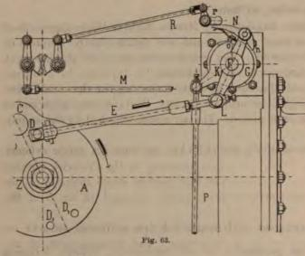
This rotary movement of the valve-spindle opens the inlet-valve and allows steam to enter the cylinder behind the piston.
