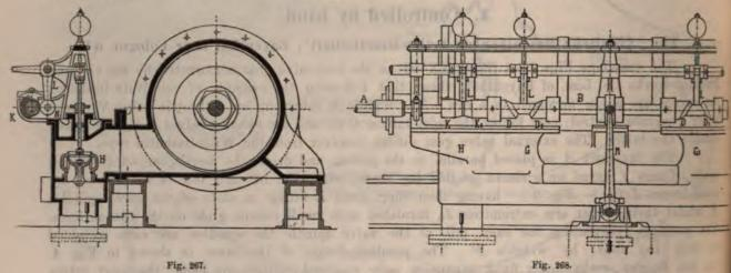
The advantage possessed by this valve-gear, consists in the engine tenter having only one lever to attend to for reversing and expansion purposes, both of which functions he is enabled to do without either drawing or throttling of the steam.
