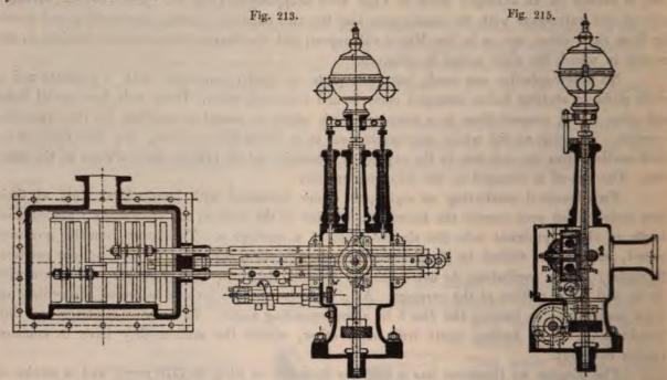
Underneath the expansion valve rod s, we have, a worm o mounted on a steel-pin t fixed to the governor-stand; this worm can be easily motioned off the governor by the rack w, and the toothed wheel v. Now when the lugs p and q on the expansion-rod  $s_1$ , strike again the worm, a stoppage ensues — i. e. the expansion rod  $s_1$  — assumes a different position; this however commands an altered position of the rod e through the lever  $hh_1$ . If the governor has shat
