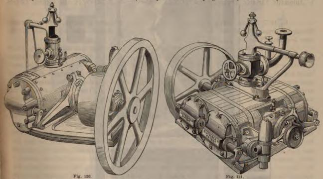
pies a ground-space of only 32 by 14 inches, the height over all being 13 inches, and it weighs no more than about 31/4 cwt.; the diameter of cylinder is 9 inches and the length of stroke 6 inches. This engine, although actually designed to drive a stone-breaker, is of the type supplied for steam launches, yachts, and gunboats, and even for propelling torpedoes themselves under the water.
