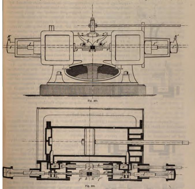
expansion is taking place in the right end, inasmuch as the expansion valve port, is closed by the plate  $c_1$ . The valves a  $a_1$  have assumed their extreme left travel, the trigger g is about getting into gear, and the expansion-valve c and main slide a are on the point of moving uniformly to the right. As soon as the crank is on its left dead centre, the position of the valves will be, as shewn by Figs. 212 and 213. The unequal lineal lead of the two working edges is apparamental.
