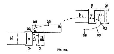
dicated therein. When  $NN_1$  are in position  $x_1$   $y_1$ , disengagement — corresponding to cut-off — ensues at  $\sqrt[3]{10^{\text{ths}}}$  stroke.
