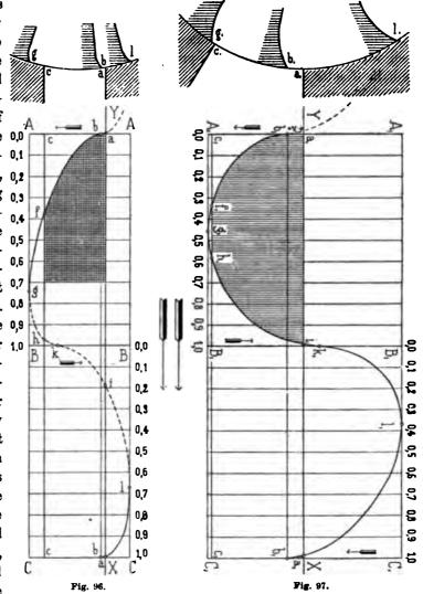
must be taken to effect automatic disengagement at the latest at g, if not before. For this reason, the line referring to the travel of the valve-edges is shewn dotted in our diagram from g to l, since, such a travel may never take place.
