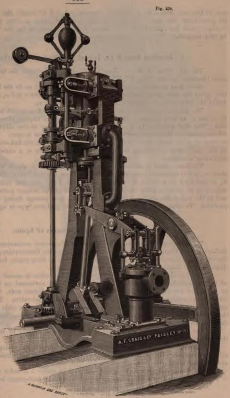
was 55 lbs., and with a 20 in. cylinder diameter and a 3' 6" stroke, the engine was ranking at 60 revolutions per min. It may be here observed, that a long range of heating pipes through which the exhaust steam is passed, somewhat accounts for the back-pressure indicated by this diagram.
