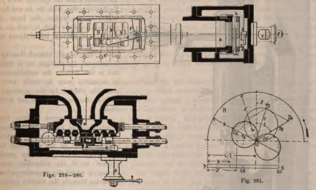
lugs. The middle valve is here dispensed with, and the grid plates of the drag-valve move again on the main-slide a; the remainder of the mechanism is somewhat complicated. This mechanism must be so arranged, as to be able to impart two motions: namely the to and fro motion of the
