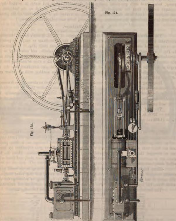
d keyed on to the shaft. The crank-pin is of steel. The connecting-rod is of best hammered iron, Uhland-Tolhausen, Steam-Engines.
