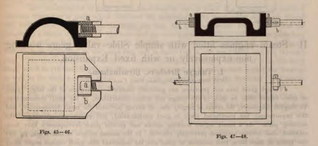
of the slide. The nut allows a certain amount of play to the valve, and for this reason its edges are rounded off. In these various slide and spindle connections, it is customary, - to ensure a sure
