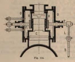
In 1877, the Journal of the Society of German Engineers, discussed a rocking-valve, designed by Eugen Schleh of Cologne, the ingenious construction of which, offers various advantages. Its chief merit, as will be seen on referring to fig. 113 and 114, lies in the cylindrical form of the
