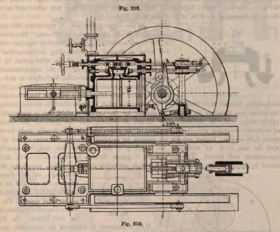
on the axis of the groove c, inasmuch as this wheel following the motion of the eccentric, is moved forward by a tooth each stroke, through a pawl fitted to the engine-bed. Hence, each oscillation of the slide depends on the number of teeth in the ratchet wheel.
