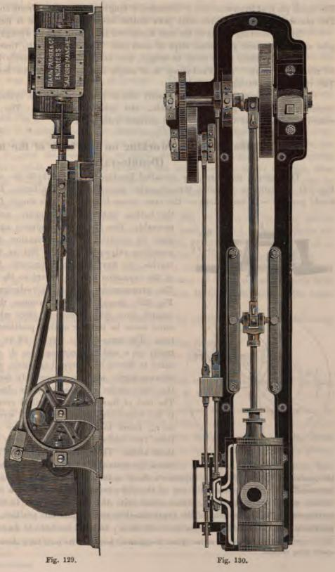
The crank pin is of Bessemer steel, 4" diameter, 6" long in bearing; it is shrunk and keyed into the crank. The crosshead is wrought iron with jaws slotted out of the solid and is finished bright all over.
