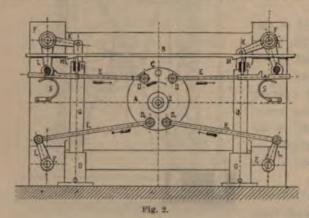
It is fitted to a horizontal cylinder, and its arrangement not merely betrays analogy to the first-named Corliss valve-gear, but it forms without doubt the connecting link to the constructive arrangement of the first Corliss engine subsequently introduced in Europe.
