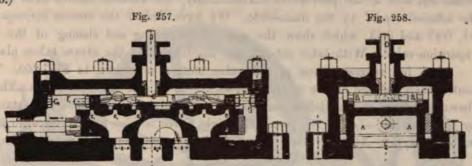
poses, each plate is furnished with a stud F — resp.  $F_1$  — which, with each stroke-end strikes against a fixed bolt G — resp. G — screwed in the valve-chest. The last named in no wise controls the rate of cut-off; it is only necessary to choose the distances between the stude and bolts, so that the through-port is quite opened out when the main-slide is at its stroke-end.
