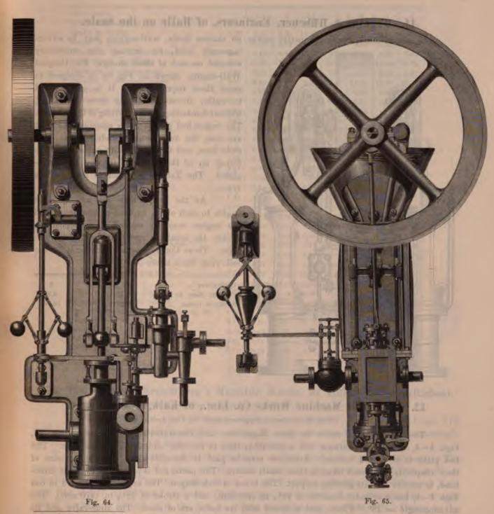
valves may be derived from the inlet eccentric, whereby the altered position of the valves do not demand extra gear. Again, by giving the cams suitable forms, the working of the exhaust valves is brought more under command.
