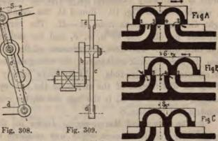
application of one eccentric. In this case an E-slide is used, which reverses the steam-distribution, as soon as its oscillating centre x is shifted. The valve is drawn in its central position in Fig. A, when
