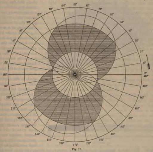
and commences to shut off the exhaust port at  $h_1$ , completely closing the same at  $i_1$ . With the return of the piston, the exhaust-valve is at  $k_1$ , and having attained its maximum ascent at  $l_1$ , the exhaust-port begins to open after  $\frac{9}{10}$  of the piston-stroke.
