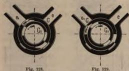
this double-valve in fig. 128 when the admission is beginning, whilst fig. 129 illustrates the position of the valves when the admission is about ceasing with a cut-off at  $\frac{2}{5}$  stroke. The inlet-ports are marked with  $ee_1$  G is the admission and  $G_1$  is the expansion-valve.
