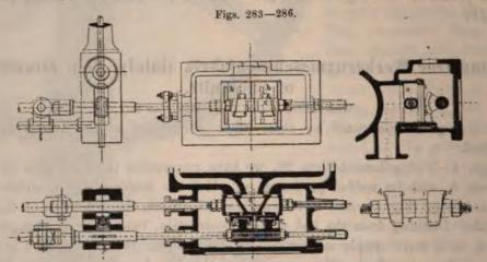
pansion-plates are rather worked off the expansion-eccentric, than dragged. On the top of the main-slide a, (whose through ports divide into two openings on its back), we find the expansion-plates b, which are guided in a ledge shewn in our drawing; these expansion-plates do not slide in the valve-box, but on a plate fixed over the main-slide.
