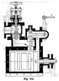
at a fixed portion of the stroke during uniform speeds. On the other hand, if the engine speed becomes considerably increased, it remains closed on account of its connection with the governor, and merely resumes to work when the engine is running at its normal speed. It remains open, on the contrary, if the engine-speed is continually diminishing, in which extreme case, the steam is only cut-off, by the distributing-valve.
