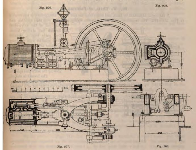
consists in the expansion-valve rods not passing separately out of the valve-box, inasmuch as by making the one hollow, the other rod is inserted inside it. The expansion-plates may thus be grasped centrally, and the whole arrangement displays greater symmetry, than Dack's design. A second stuffing-box has of course to be introduced on the extremity of the one valve-rod, so as to pack the internal rod steam-tight.
