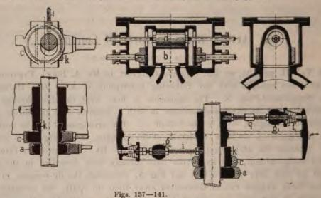
Moreover to balance the governor still more efficiently, the expansion valve is introduced in the form of a piston-valve, which runs in a cylindrical casing of the main-slide. As it is made sufficiently long, it merely requires grinding in, to fit steam-tight.
