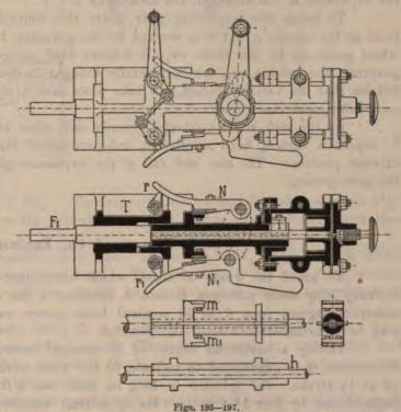
Variable-expansion Valve-gear in sizes from 10 HP. upwards, calculating these for a steam-pressure of 6 atm. and a normal cut-off at 1/8 stroke.
