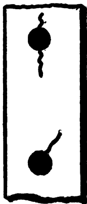
FIG. 26.—CRACKS AROUND STAYBOLTS.
