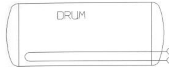
Figure 4.11 Exchanger inside boiler drum.
