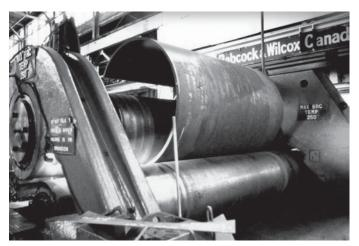
Fig. 6 Cold rolling plate for steam generator cylindrical shell.
