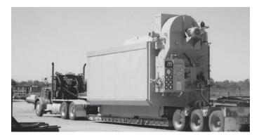
Fig. 1 Small shop-assembled package boiler.
