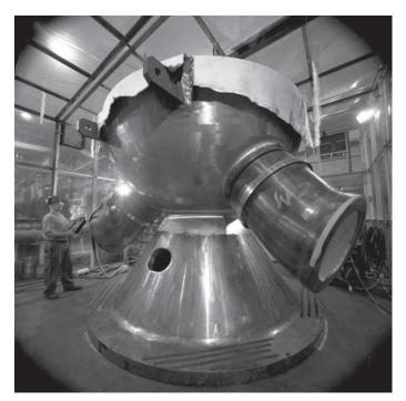
Fig. 8 Once-through steam generator primary head.
