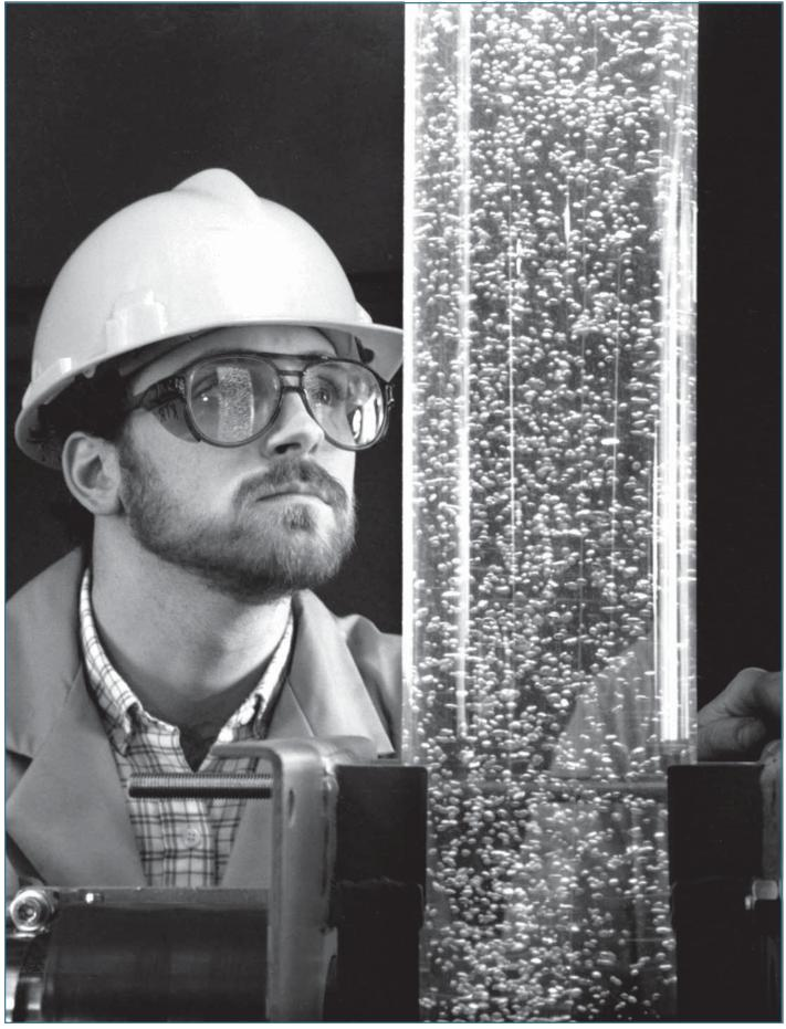
Two-phase flow void fraction measurements.
