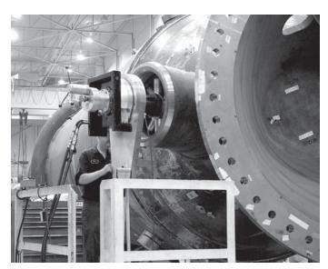
Fig. 22 Final nozzle end machining.
