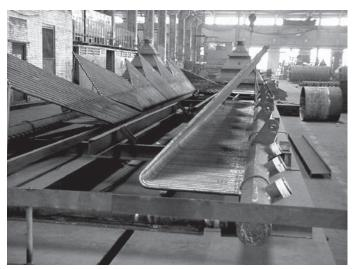
Fig. 14 Hopper panel fabrication for a spiral wound universal pressure boiler.
