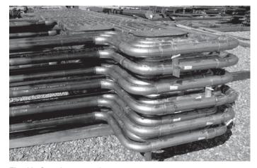
Fig. 18 Superheater sections.
