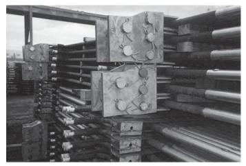
Fig. 25 The use of pins and collectors simplified construction and improved reliability by eliminating original welded supports.
