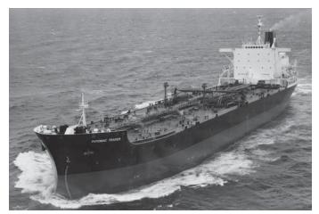
Fig. 6 M.V. Potomac Trader, LaJolla Class vessel with diesel propulsion plus waste heat and auxiliary steam boilers (*courtesy Penn-Attransco Corp.*).
