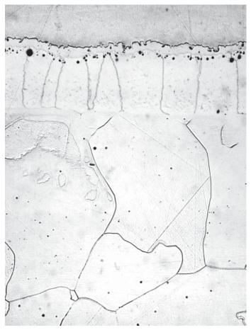
Fig. 14 Chromized 2-1/4Cr-1Mo at 400 X magnification.
