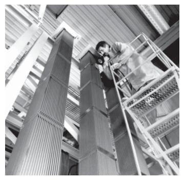
Fig. 16 Final visual inspection of fuel assemblies.
