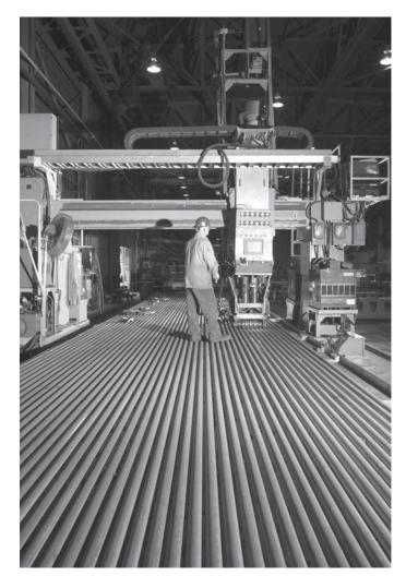
Fig. 15 Wall panel membrane operation.
