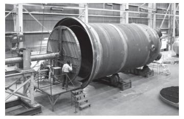
Fig. 16 Installation of lattice grid tube bundle support.
