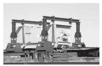
Fig. 10 Hydraulic gantry system.
