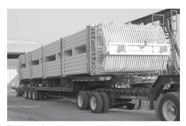
Fig. 19 Longflow economizer prepared for shipment.
