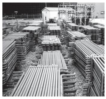
Fig. 13 Typical superheater elements for a replacement project.
