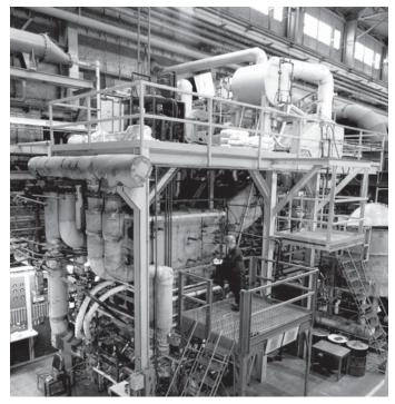
Fig. 30 B&W's small boiler simulator.
