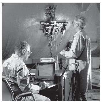
Fig. 17 Ultrasonic inspection of seam weld.
