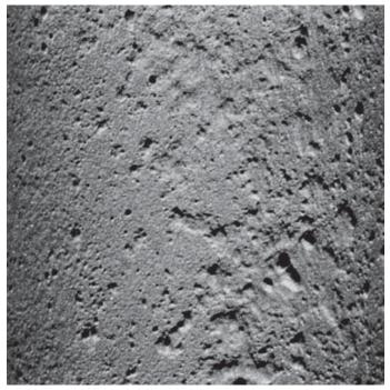
Fig. 15 Oxygen pitting of economizer feedwater inlet.
