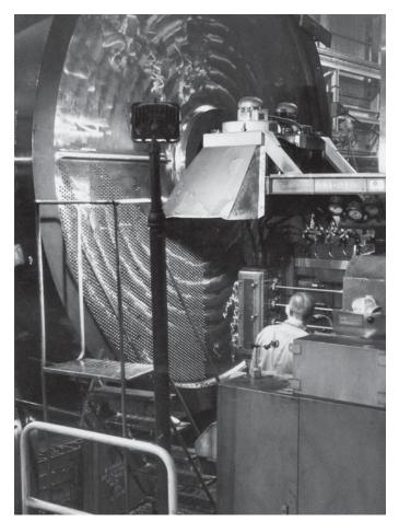
Fig. 7 Gundrilling a tubesheet.
