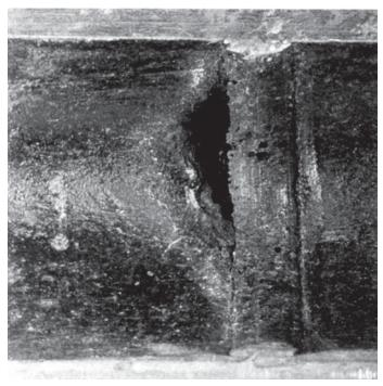
Fig. 19 Caustic gouging initiated along weld backing ring.
