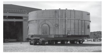
Fig. 9 Hydraulic platform trailer.
