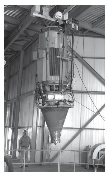
Fig. 10 Rotary atomizer assembly.
