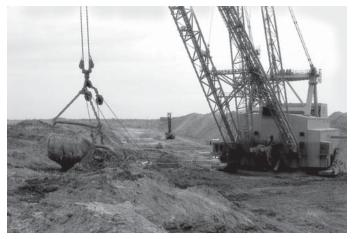
Fig. 2 Large coal dragline in operation (*courtesy of National Coal Association*).
