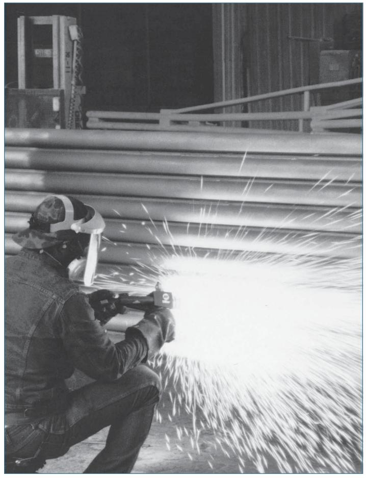
Application of protective coating to boiler tubes.
