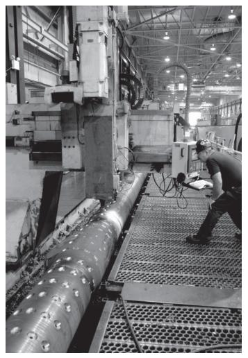
Fig. 11 Header drilling on vertical boring mill.
