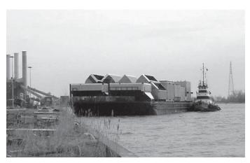
Fig. 8 A barge carrying SCR components is positioned for off-loading.
