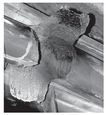
Fig. 14 Rupture of 6 in. (152 mm) feedwater pipe in an area thinned by internal corrosion.
