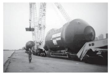
Fig. 23 Steam generator awaiting offloading to heavy lift ship.
