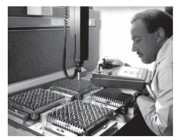
Fig. 15 Spacer grid coordinate measuring machine.
