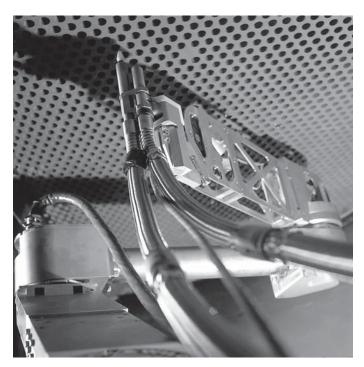
Fig. 3 Robotic eddy current inspection shown in a recirculating steam generator mockup.
