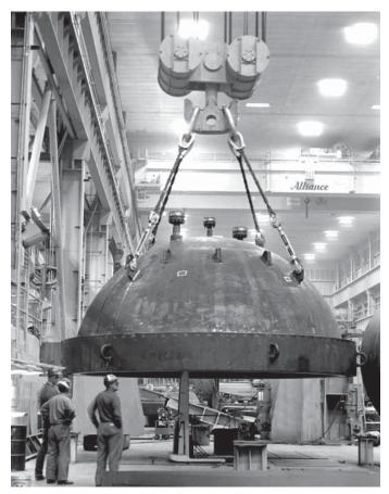
Fig. 1 Head of nuclear reactor vessel.
