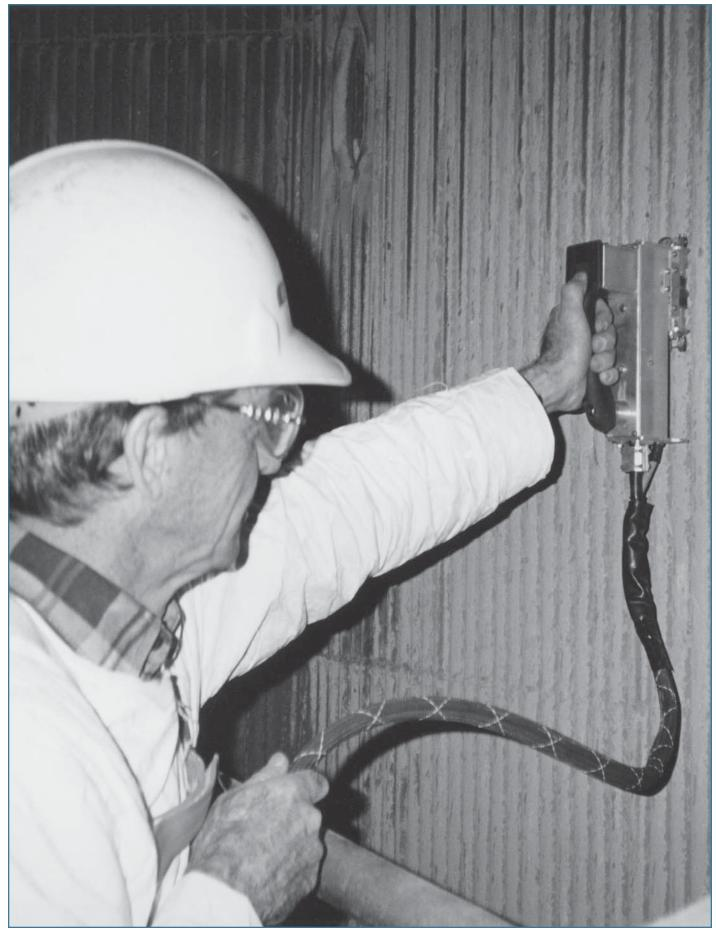
Electromagnetic acoustic transducer (EMAT) technology is one method used to determine remaining life of boiler tubes.
