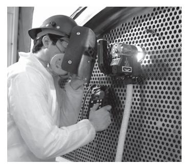
Fig. 19 Tube-to-tubesheet welding.
