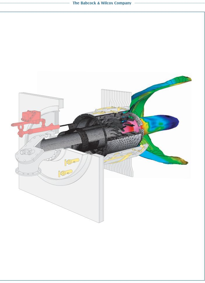
Advanced computational numerical modeling of a pulverized coal burner.
