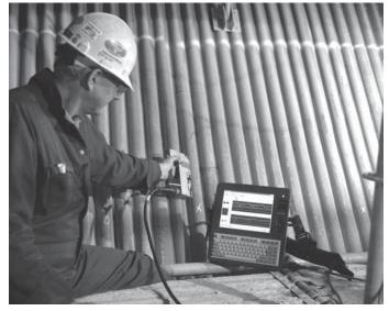
Fig. 6 B&W's Fast-Scanning Thickness Gage (FST-GAGE<sup>®</sup>) EMAT based system can provide continuous measurement of tube wall thickness.
