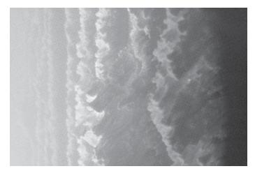
Fig. 4 Heavily fouled surface.
