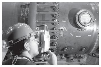
Fig. 21 Set up of nozzle machining tools using coordinated measuring machine.
