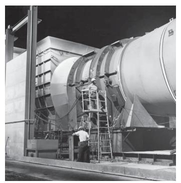
Fig. 18 Full-scale testing of variable-pitch axial flow fan.
