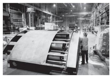
Fig. 20 Fabrication of steam separator subassembly.
