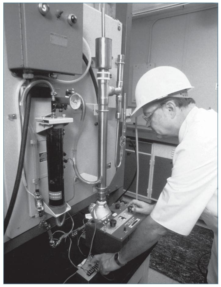
Degassed conductivity analyzer for water quality analysis.
