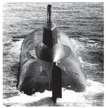
Fig. 34 Soviet Typhoon-class ballistic missile submarine.
