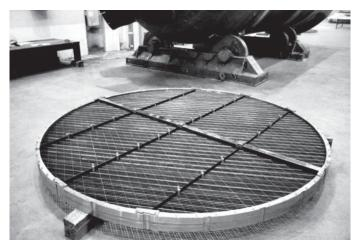
Fig. 12 B&W lattice grid tube support assembly.
