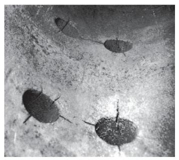
Fig. 10 Large ligament cracks on header ID.
