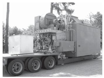
Fig. 15 FM O-type boiler.
