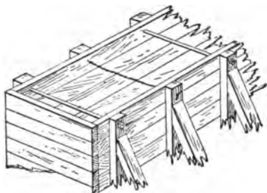
FIG. 242.—Bracing for concrete forms.
