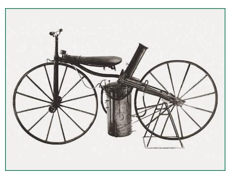
This first motorized bicycle was steam-powered. Built by S. H. Roper in 1867, the steam engine was positioned underneath a raised seat. A precursor to the motorcycles driven today, the steam-powered bicycle could reach speeds of up to 19 miles per hour.
