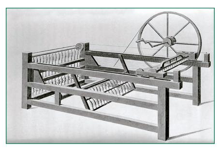
The Spinning Jenny was invented by James Hargreaves in 1764. While his invention was revolutionary in itself — spinning cotton eight times faster than prior spinning wheels — waterwheels were eventually introduced to power many machines simultaneously. These new advancements in weaving led to the birth of the textile mill, which played a key role in the Industrial Revolution.
