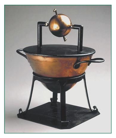
Hero, a Greek mathematician of the first century, invented this early steam engine. Called an aeolipile, it was a hollow ball into which steam from the sealed cauldron of boiling water rose. The short pipes extending from the ball were bent at a right angle and emitted jets of the highly pressurized steam, causing the ball to rotate.
