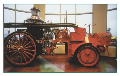
Early steam-pump fire engines were pulled by horses. When the alarm sounded, the firemen threw burning coals in the engine's firebox to heat the boiler. By the time the truck arrived at the fire, the steam pump was ready to spray water 180 feet from the end of the hose and up to 29 feet in the air.
