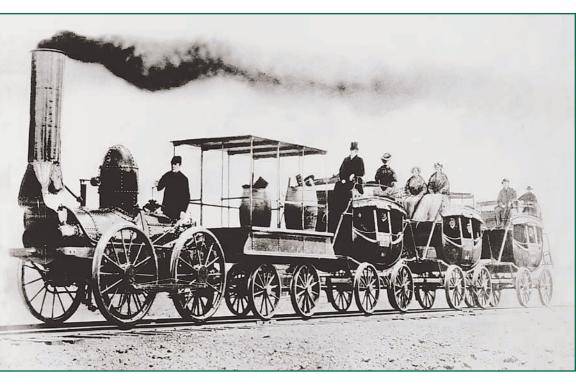
The first passenger trains were stagecoaches equipped with railroad wheels pulled by a steam locomotive. The coaches' backless wooden seats and low roofs were so uncomfortable that they prompted George M. Pullman to develop his Pullman Sleeper cars, which made it possible for travelers to ride in comfort.
