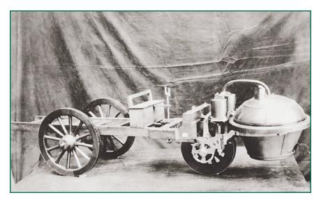
Nicolas Cugnot's Steam Road Carriage was propelled by steam generated in the combination stove and kettle at the vehicle's front. Travel by the steam carriage was considerably slow — not only did it travel at two to three miles per hour, but the driver also had to stop and fill the kettle with water every 15 minutes.
