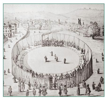
Deemed the "Father of the Locomotive" for a train engine he built in 1804, steam engineer Richard Trevithick built another locomotive that he called *Catch-me-who-can* in 1808. Trevithick pioneered the idea of using steampowered machines on rails. He charged the London public a small fee to ride around a circular track in a carriage pulled by the engine.
