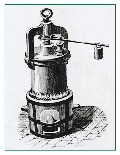
This pressure cooker was invented by Denis Papin, a French physicist, in the 1680s. The sealed pot on a furnace base cooked foods quickly with pressurized steam. Papin was captivated by the power of steam and developed many machines to harness its power.
