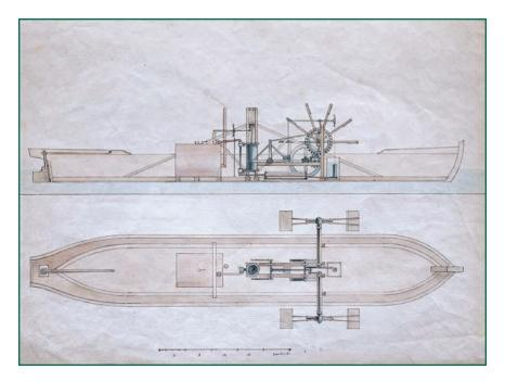
This steamboat diagram was prepared by Robert Fulton, an American who built the steam-driven *Clermont* in 1807. The *Clermont* had two large paddle wheels positioned on each side of the boat. These two wheels were connected by arms to a pumping piston, which was attached to the steam engine. Power from the steam engine would rotate the wheels, forcing the boat into motion.
