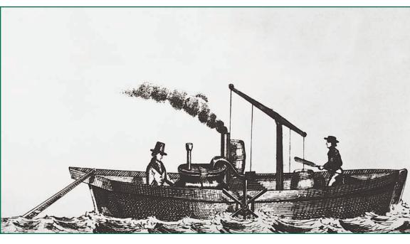
In 1787, John Fitch's first steamboat was outfitted with six paddles on each side of its hull. The paddles were powered by a single cylinder steam engine, moving the boat along at a speed of three miles per hour. The addition of steam power to watercraft made it possible to move goods upstream, expediting overseas transport.
