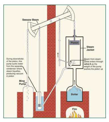
This illustration of Watt's basic steam engine includes a steam jacket, which he added to Newcomen's model to condense the steam more quickly, and an air pump, which sucks air out of the condenser, creating a vacuum that forces steam from the hot cylinder into the condenser. The hot air immediately condenses and moves the piston.
