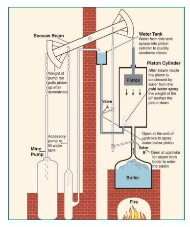
This illustration shows how the parts in Newcomen's steam engine work together to draw water from mines. Newcomen's steam engine was the first machine developed to utilize steam power to complete tasks.
