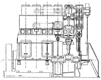
FIG. 15.—PART SECTIONAL ELEVATION OF THREE-CRANK "CLAYTON" ENGINE. 600 I.H.P., 300 REVS.
