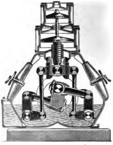
FIG. 123.--SECTIONAL VIEW OF MERTZ'S SINGLE-ACTING ENGINE.
