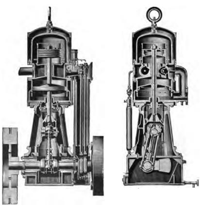
FIG. 46.—LONGITUDINAL VERTICAL SECTION. FIG. 47.—TRANSVERSE VERTICAL SECTION. THE "UNIVERSAL" ENGINE.
