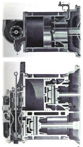
FIG. 83.-DETAIL OF CYLINDERS, PISTONS, STEAM CHEST AND VALVES.
