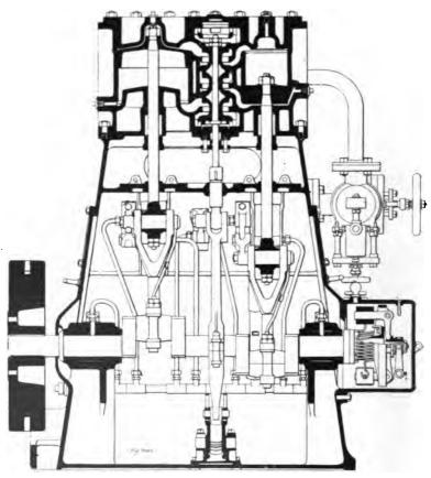
FIG. 20.-SECTIONAL ELEVATION OF "ERITH" COMPOUND ENGINE.
