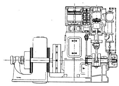
FIG. 14.—PART SECTIONAL ELEVATION OF COMPOUND "CLAYTON" ENGINE. 120 I.H.P., 380 REVS.
