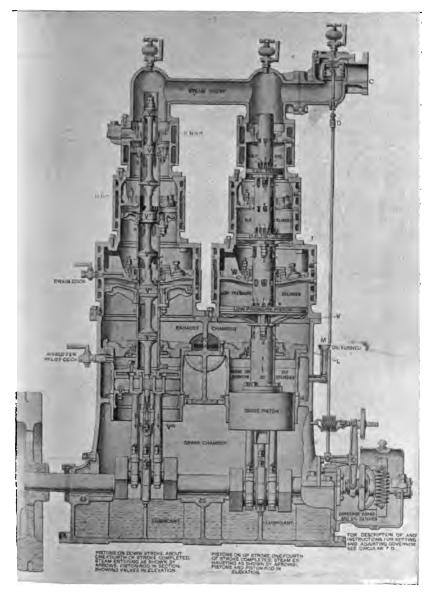
FIG. 4.--SECTIONAL VIEW OF THE "WILLANS" STANDARD PATTERN ENGINE.
