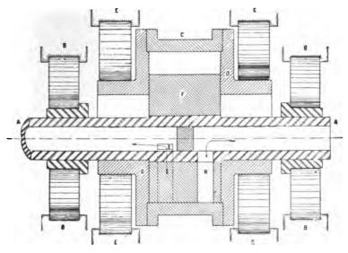
FIG. 133 .- FRONT SECTIONAL VIEW OF THE "HULT" ROTARY ENGINE.
