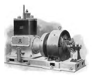
FIG. 66 .- " SENTINEL " CLASS "C" SIMPLE FNGINE, COUPLED DIRECT TO DYNAMO.
