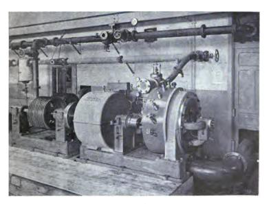
FIG. 113.-300 B.H.P. "DE LAVAL" STEAM TURBINE MOTOR.
