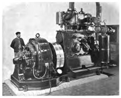
FIG. 147.- 100 R.H.P. FNCLOSED DOUBLE-ACTING COMPOUND HIGH SPEED ENGINE, LY MESSRS. RUSTON, PROCTOR & CO., LTD., LINCOLN.
