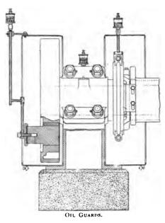
through the inner excentric R, which fits loosely on the hub of the governor wheel A, and is connected with the weight arms F, through the links K, in such a manner that the inner excentric is moved round the hub of the governor, forward or backward, as the weights change their position. This forward or backward is movement communicated through the inner excentric strap Q to the main excentric strap B, causing this to slide on the hub plate C, in a straight
