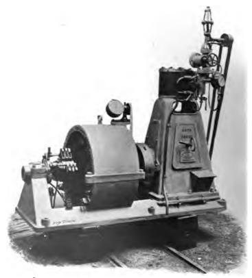
FIG. 18.—SINGLE CYLINDER "ERITH" ENGINE, COUPLED TO FOUR-POLE DYNAMO. 580 REVS. PER MINUTE.
