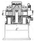
FIGS. 95 AND 96 .- SECTIONAL VIEWS OF THE HARRISBURG "IDEAL" SIMPLE ENGINE.
