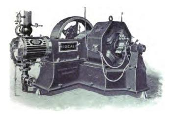
FIG. 97.-VIEW OF A HARRISBURG "IDEAL" ENGINE RUNNING ON THREE STEEL POINTS, SHOWING BALANCE
