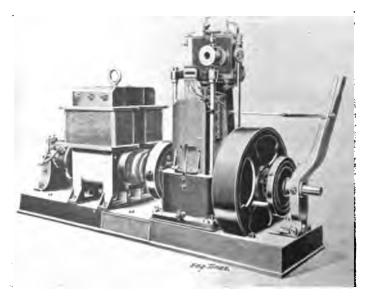
FIG. 56.—" ROBINSON AND AUDEN " SINGLE CYLINDER ENGINE, COUPLED DIRECT TO DYNAMO.
