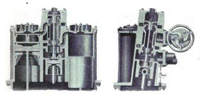
FIG. 81.-DETAIL, SHOWING CYLINDERS, PISTONS, STEAM CHEST AND VALVE.
