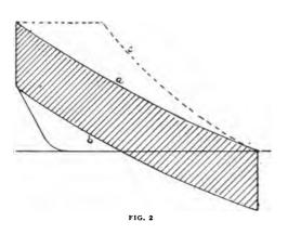
temperature of thecylinder walls, and provides reevaporation during expansion. Hence the line a can be made more nearly parallel to b by careful designing than c can.
