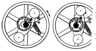
FIG. 84.—AT LONGEST CUT-OFF. FIG. 85.—AT SHORTEST CUT-OF POSITION OF GOVERNOR PARTS AT LONGEST AND SHORTEST CUT-OFF.
