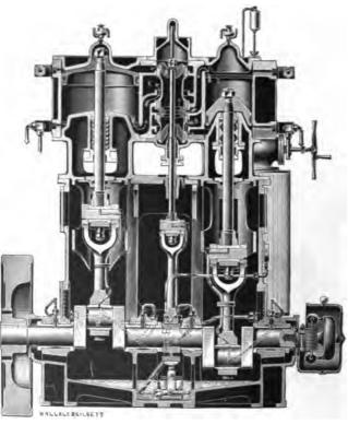
FIG. 6 .- " BELLISS " ENGINE. SECTIONAL ELEVATION.
