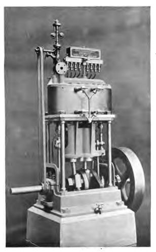
FIG. 49.—HIGH-SPEED ELECTRIC LIGHT ENGINE, BY MESSRS. COULTHARD & CO. Shown with steel sheet covers removed.
