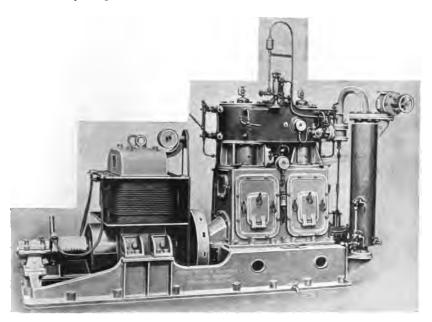
FIG. 31.—ERNEST SCOTT AND MOUNTAIN'S CENTRAL VALVE ENGINE, COUPLED TO A "TYNE" DYNAMO.
