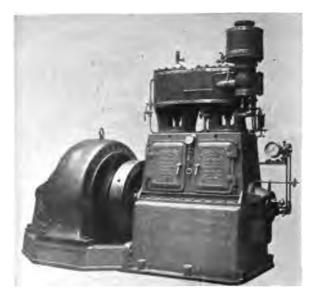
FIG. 149.-DOUBLE-ACTING, FORCED LUBRICATION COMPOUND ENGINE, BY THE ANDERSTON FOUNDRY CO., LIMITED, GLASGOW.
