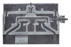
FIG. IOI.--"RUSSELL" ENGINE-PART SECTIONAL PLAN THROUGH CYLINDER AND STEAM CHEST.
