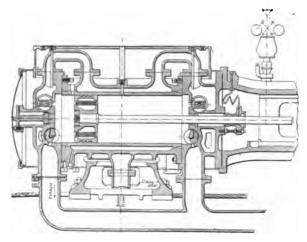
FIG. 127.-SECTION OF "FARCOT" ENGINE CYLINDER.
