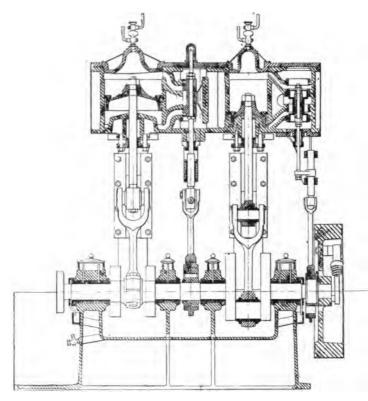
FIG. 125 .-- SECTIONAL VIEW OF THUNE'S DOUBLE-ACTING COMPOUND ENGINE.
