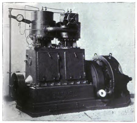
FIG. 39.-THE "SCOTT" COMPOUND ENGINE, ATTACHED TO DYNAMO.
