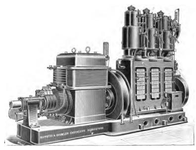
FIG. 69.—THE "CHANDLER" COMPOUND ENGINE.
