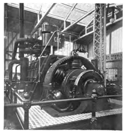
FIG. 139.-369 I.H.P. "TEACHE" ENGINE. BY WESNES. DAVEY, PANMAN & CO., COLCHESTER, DRIVING DYNAMO BY THE GENERAL ELECTRIC CO.
