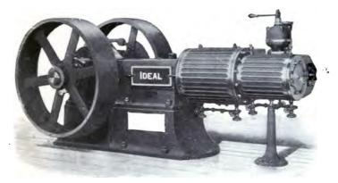
FIG. 91.-TANDEM COMPOUND "IDEAL" ENGINE, COUPLED TO DYNAMO.
