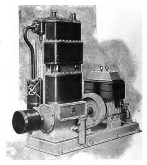
FIG. 67 .--- " SENTINEL " TANDEM COMPOUND ENGINE, COUPLED DIRECT TO DYNAMO.
