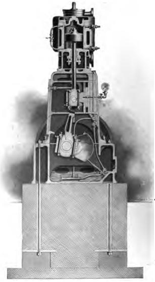
FIG II.-SECTIONAL END VIEW OF "B.I." QUICK SPEED ENGINE.
