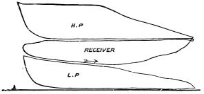
FIG. 71.—" CHANDLER " ENGINE, DIAGRAM.
