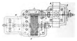
FIGS. 114 AND 115.-SECTIONAL VIEWS OF A 20 P.H.P. "DE LAVAL" MOTOR TURBINE.
