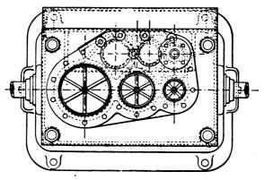
FIG. 55.—SECTIONAL VIEW OF COULTHARD'S HIGH SPEED TRIPLE EXPANSION ENGINE.
