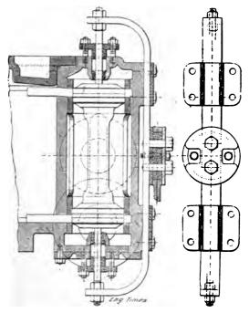
FIG. 57 .-- " ROBINSON AND AUDEN " ENGINE VALVE DRIVE.
