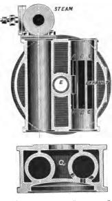
FIG. 48.—VALVE CHEST OF "UNIVERSAL" ENGINE.
