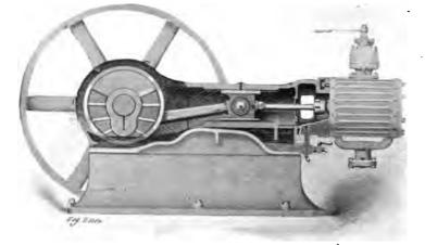
FIG. 90.-" IDEAL" SELF-OILING SYSTEM. A. L. IDE & SONS, SPRINGFIELD, ILL.
