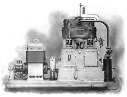
FIG. 60.-THE "RESTLER" ENGINE, COUPLED TO DYNAMO.
