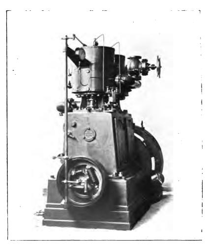
FIG. 40.-END VIEW OF "SCOTT" ENGINE, SHOWING GOVERNOR.
