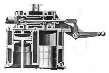
FIG. 89.—DETAIL SHOWING STEAM CHEST, CYLINDERS, VALVE AND PISTONS OF. WESTINGHOUSE "JUNIOR."
