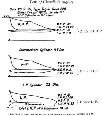
Water consumption on four hours' test, 14 lb. per one H.P. hour. M.E.P.L.P. piston (22 in. diameter) = 42 lb. per sq. inch.
