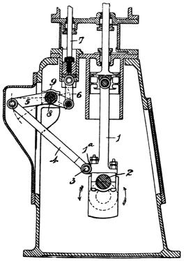
FIG. 70 .- VIEW SHOWING VALVE GEAR OF THE "CHANDLER" ENGINE.
