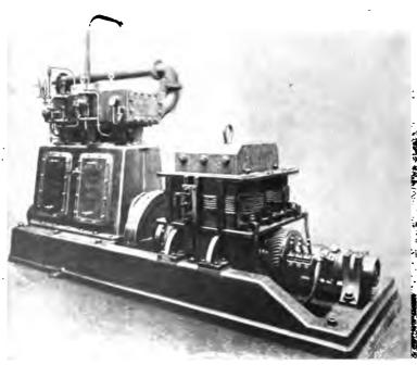
FIG. 25.—"ROBEY" COMPOUND ENGINE, DESIGNED WITH INDEPENDENT VALVES TO EACH CYLINDER, SHOWN COUPLED TO DYNAMO.
