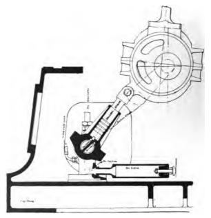
FIG. 16.—"CLAYTON" ARRANGEMENT OF VALVELESS OSCILLATING OIL PUMP.
