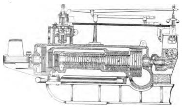
FIG. 109.-SECTIONAL VIEW OF PARSONS' STEAM TURBINE.
