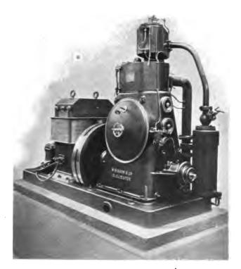
FIG. 153.—THE "SISSON" COMPOUND ENGINE, SHOWN DIRECTLY CONNECTED TO A "CLARKE-CHAPMAN" DYNAMO.
