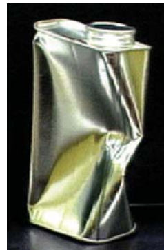
Figure 9b Result of condensation. This can was filled with steam and then closed. The steam condensed, and the resulting vacuum caused the damage shown.
