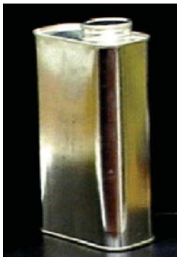
Figure 9b Result of condensation. This can was filled with steam and then closed. The steam condensed, and the resulting vacuum caused the damage shown.
