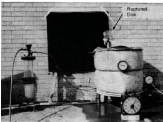
Figure 8c The remains of the ruptured disc at the top of the vessel leave no doubt that there was an explosion inside the vessel.
