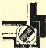
Fig. 807.—Section of Corliss valve by the Sangerhauser Engine Works.
