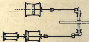
Fig. 34.—Triple Expansion Engine, semi-tandem; two cranks at 90 degrees.
