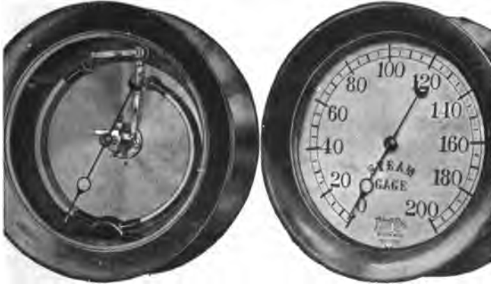
FIG. 16.—Interior and exterior view of steam gage, showing principle of operation.
