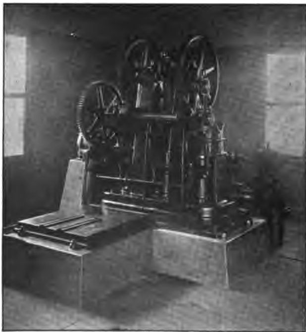
FIG. 125.—One of the pumps which handle the oil from the main storage tank to the auxiliary tank. This pump was originally arranged for belt drive but was found unsatisfactory. The gearing is now direct.
