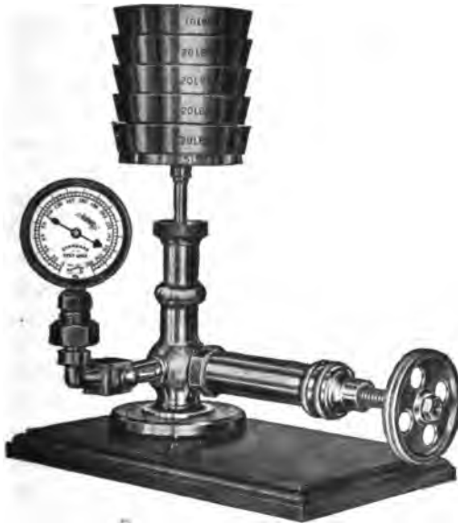
FIG. 13.—The steam gage tester illustrates the application of a fundamental law, wherein a pressure is balanced against the force due to gravity.
