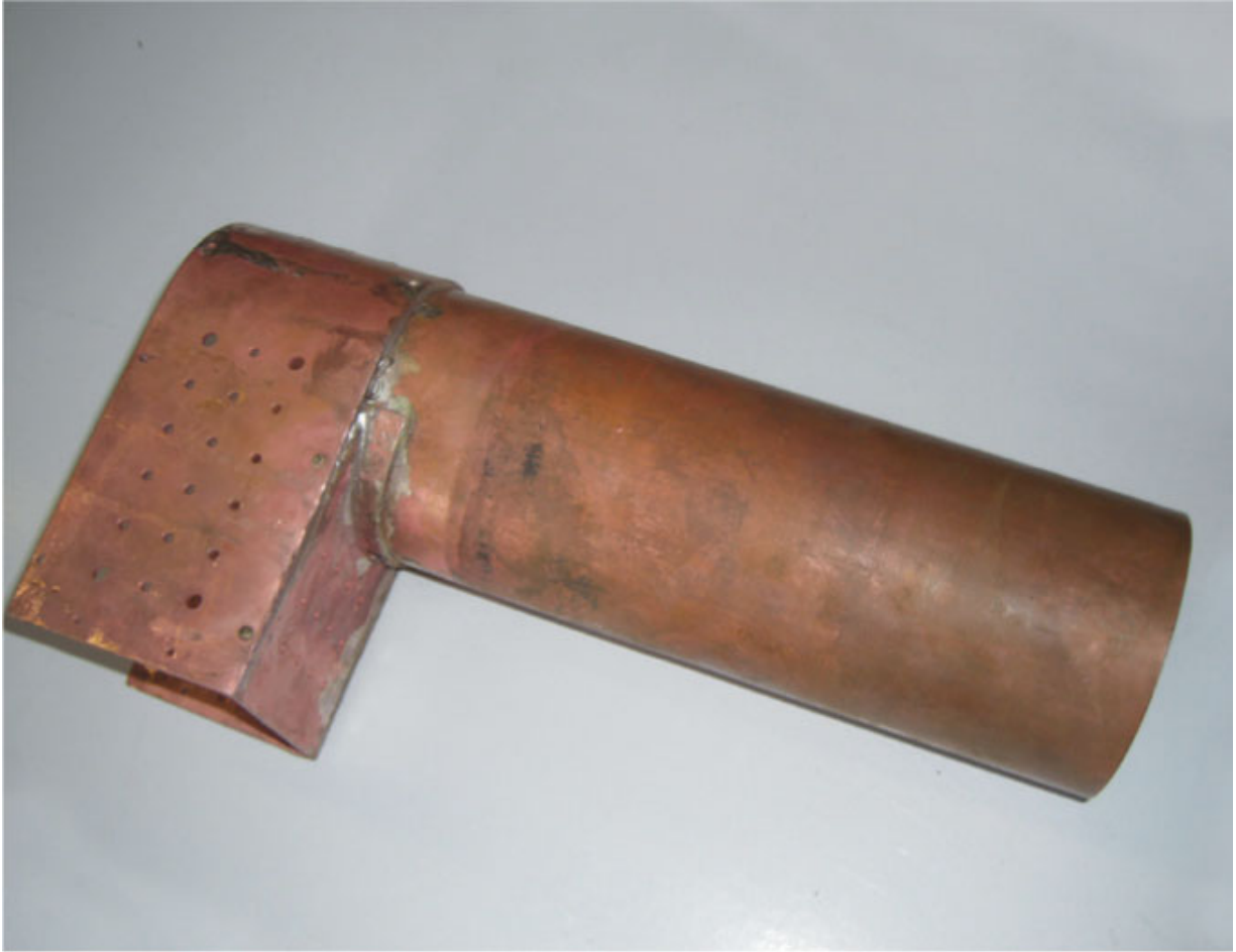
Barrel, throat plate and wrapper silver soldered together.
