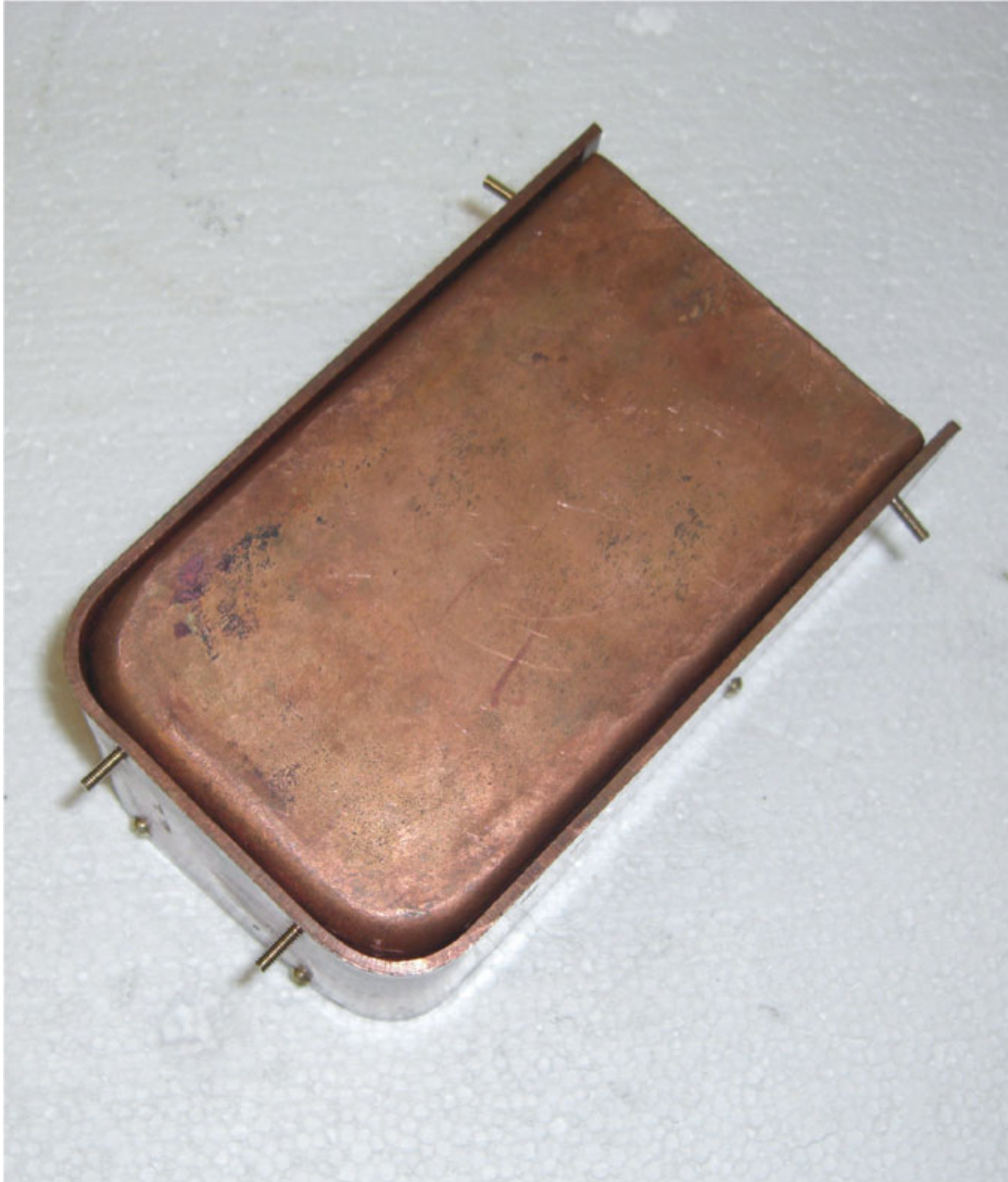
Inner firebox trial assembly. Note that the screws are inserted from the inside.
