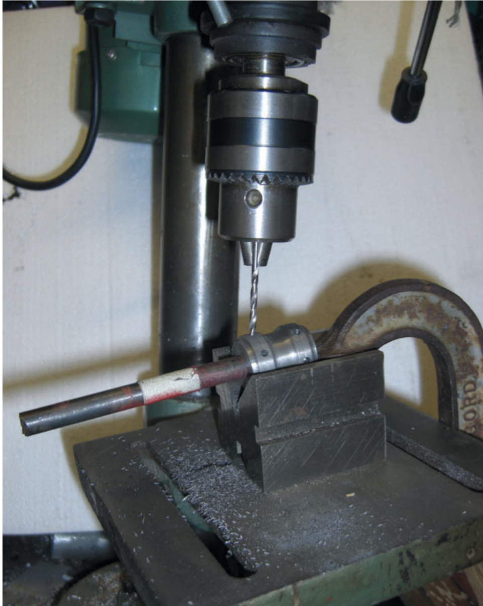
Drilling the spoke holes at an angle.
