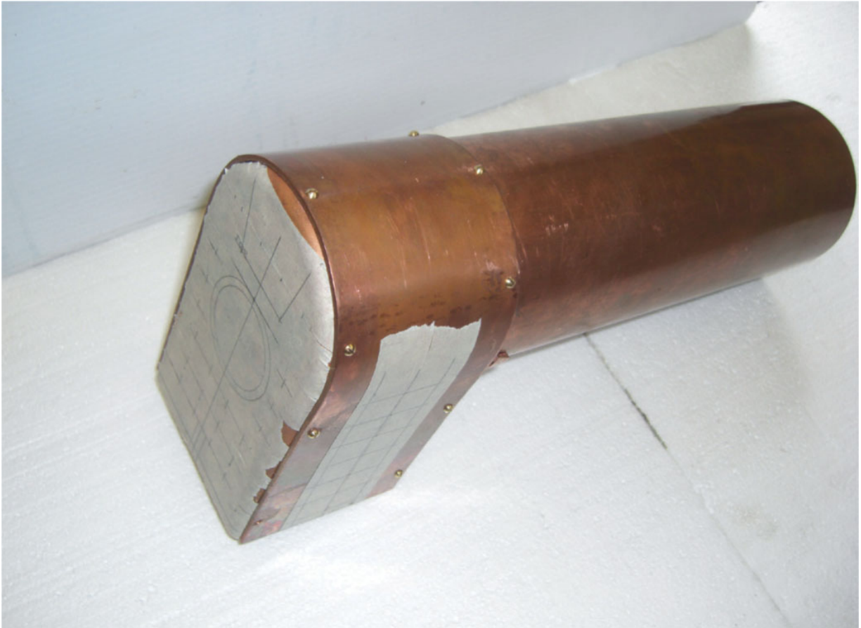
Door-plate and firebox side with stay positions marked out.
