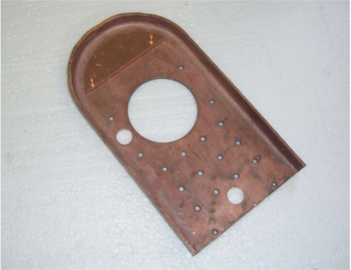
Door-plate with reinforcing plate riveted on. Note that the water gauge bush should be higher.
