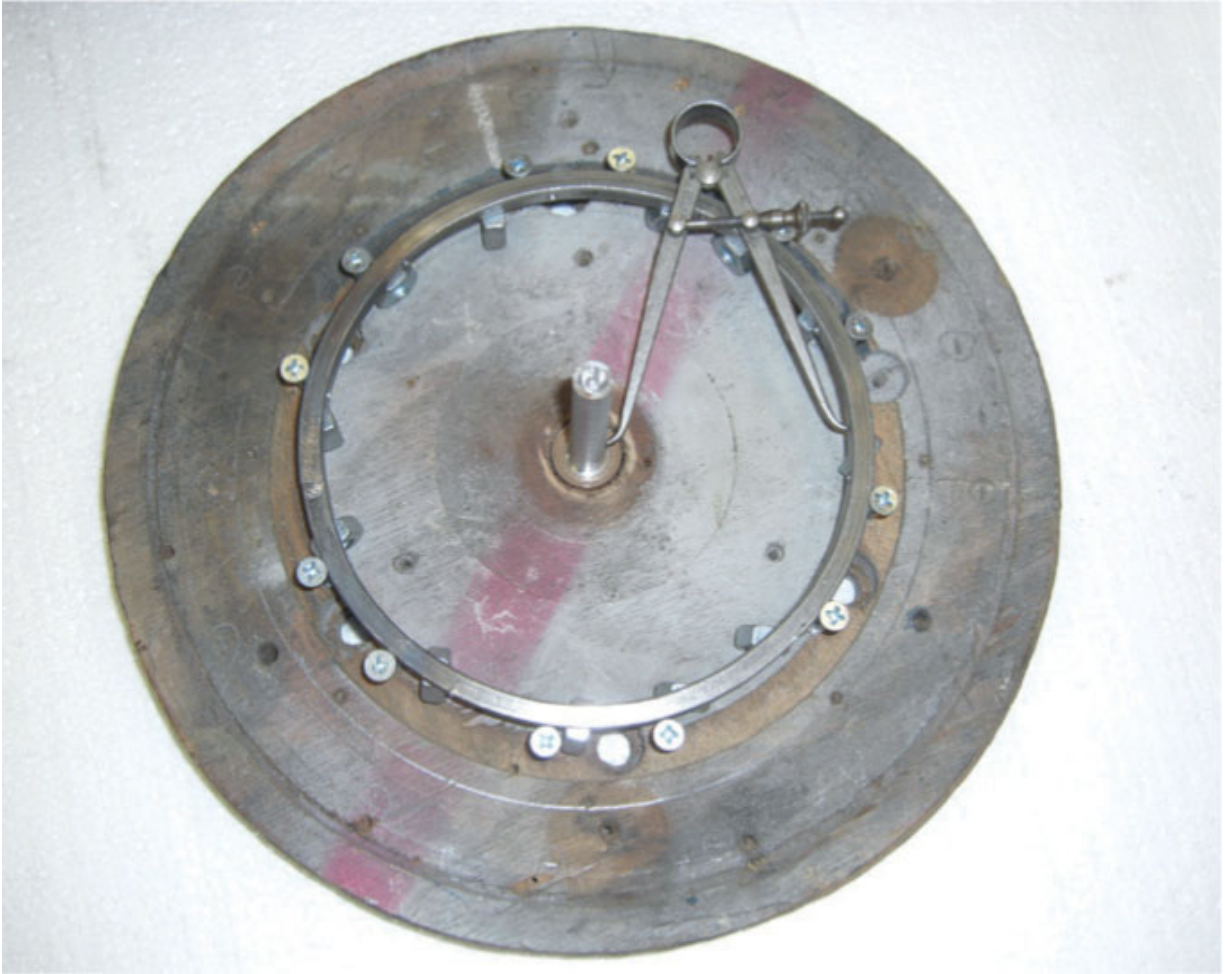
Checking rim is concentric to dummy axle.
