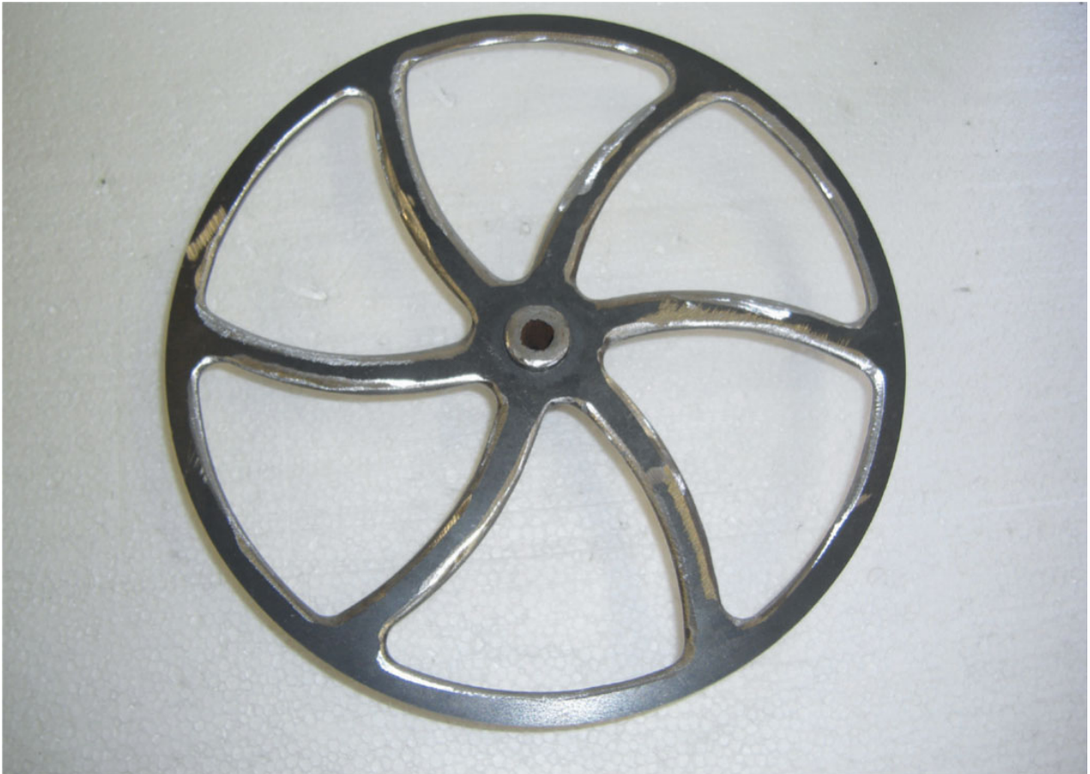
Spokes carefully dressed with an angle grinder
