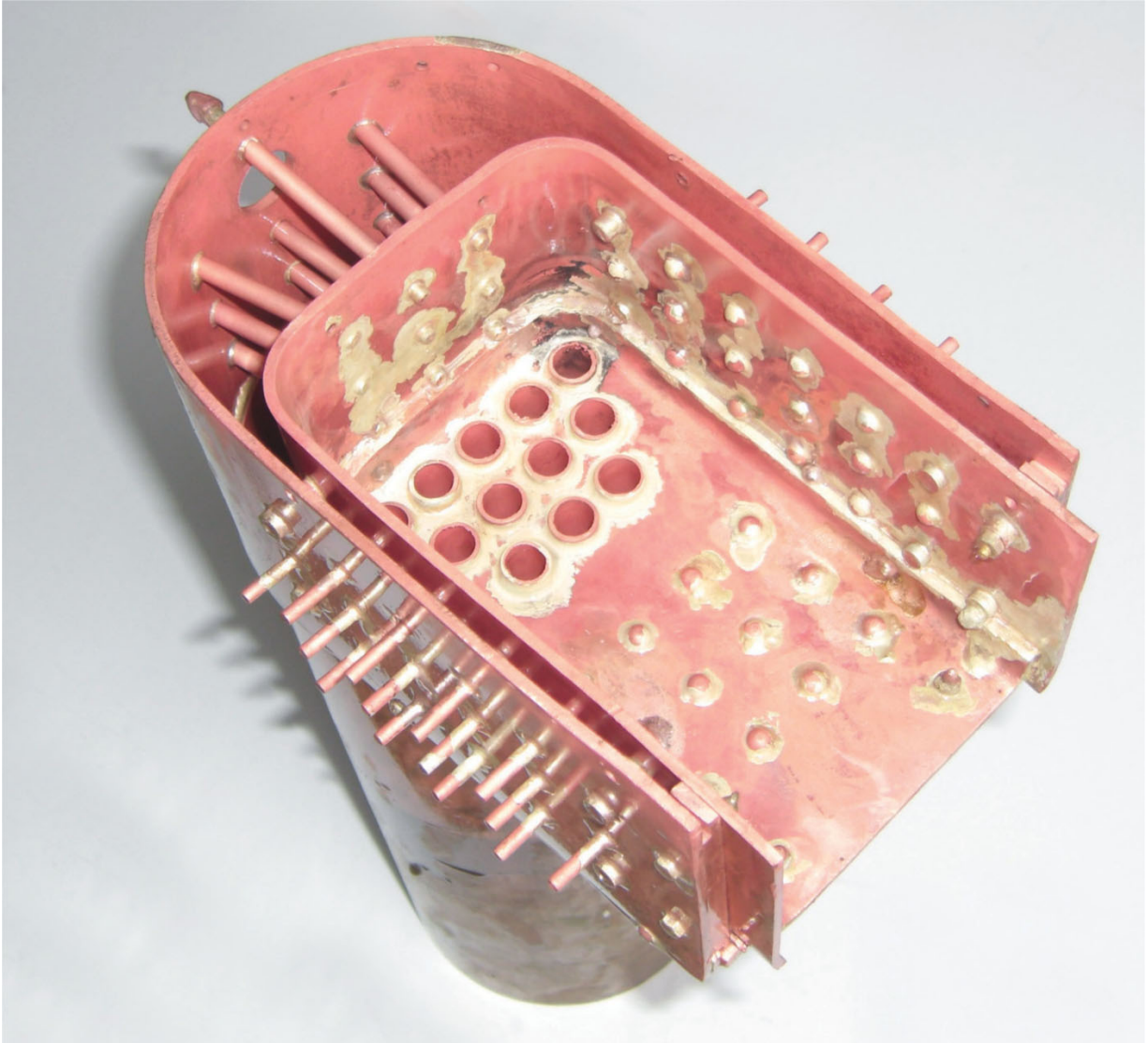
Stays and tubes after pickling.
