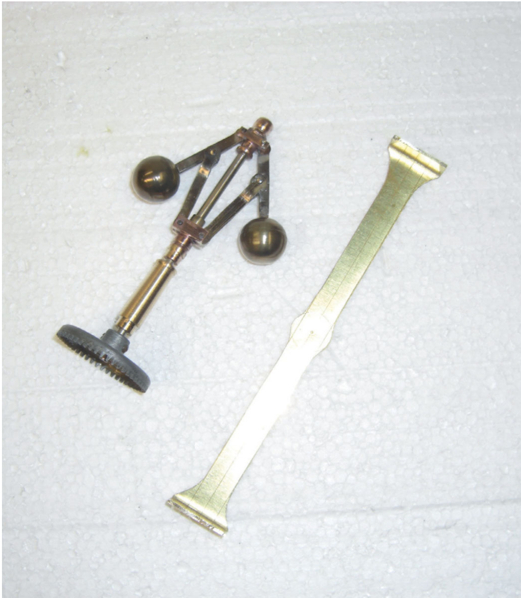
Governor, down, with bracket material.
