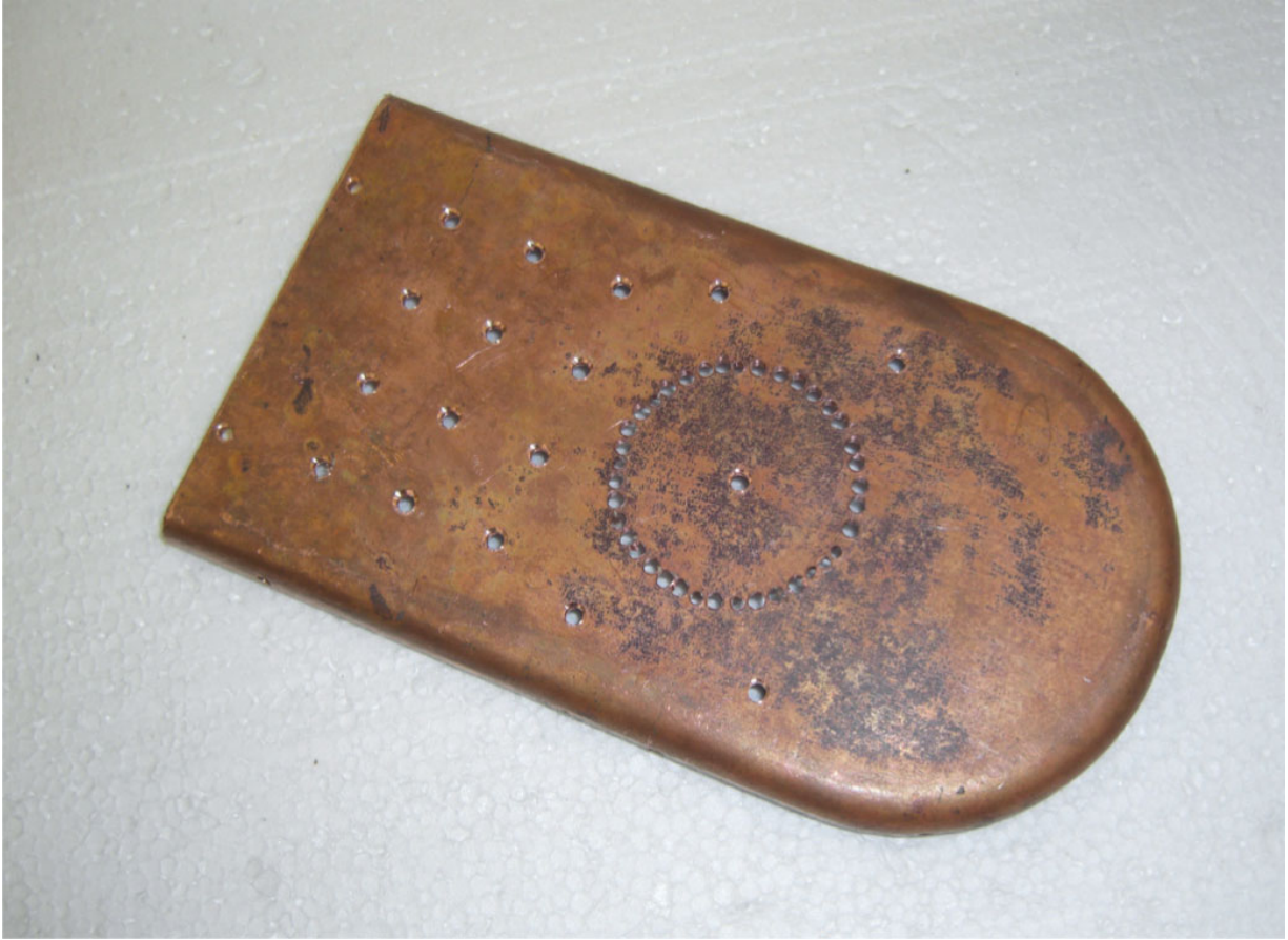
Door-plate with fire-hole chain drilled.
