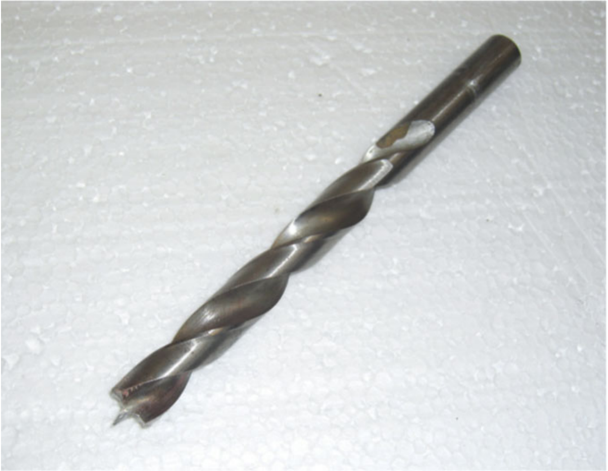
Twist drill ground to drill thin sheet.
