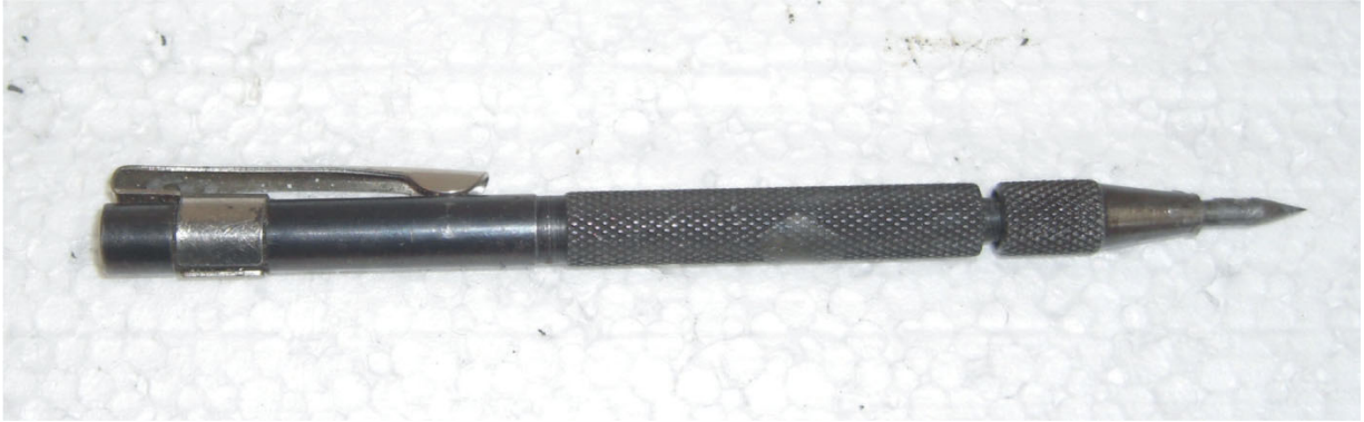
Scriber with replaceable tip.
