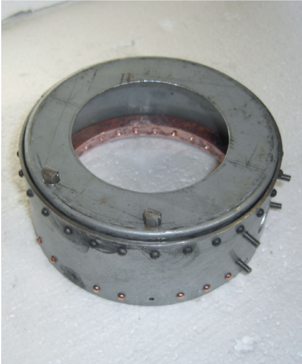
Front plate riveted to smokebox.
