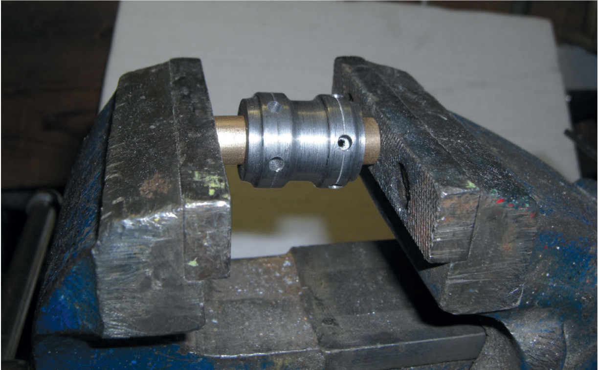
Pressing Oilite bushes into steel hub.
