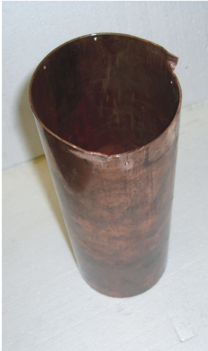
End of barrel tube cut back and shaped on trial assembly.
