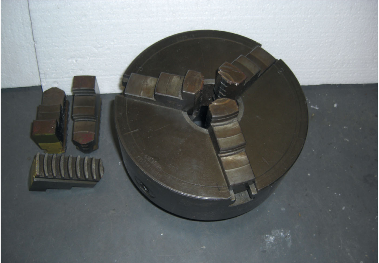
Three-jaw chuck with inside jaws fitted. The outside jaws are supplied loose.
