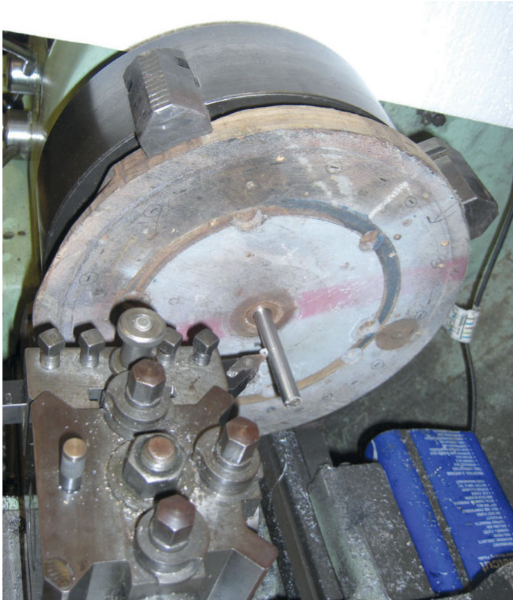
Truing dummy axle on assembly jig.
