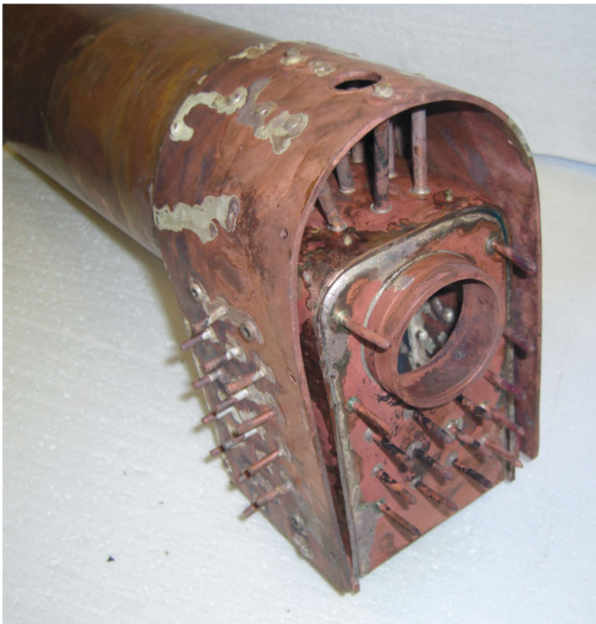
Firebox door-plate silver soldered in place.
