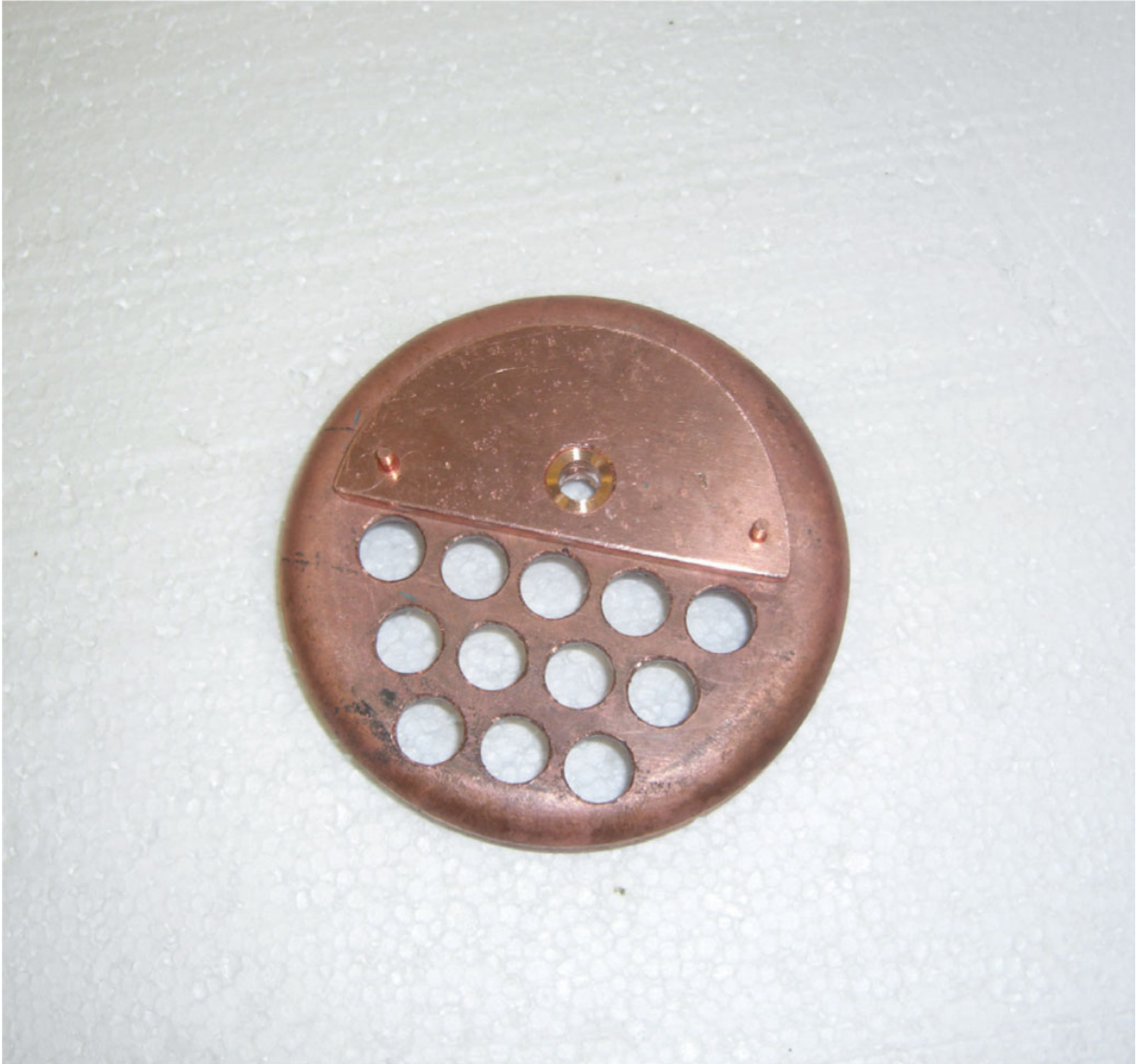
Reinforcing plate riveted on before silver soldering.
