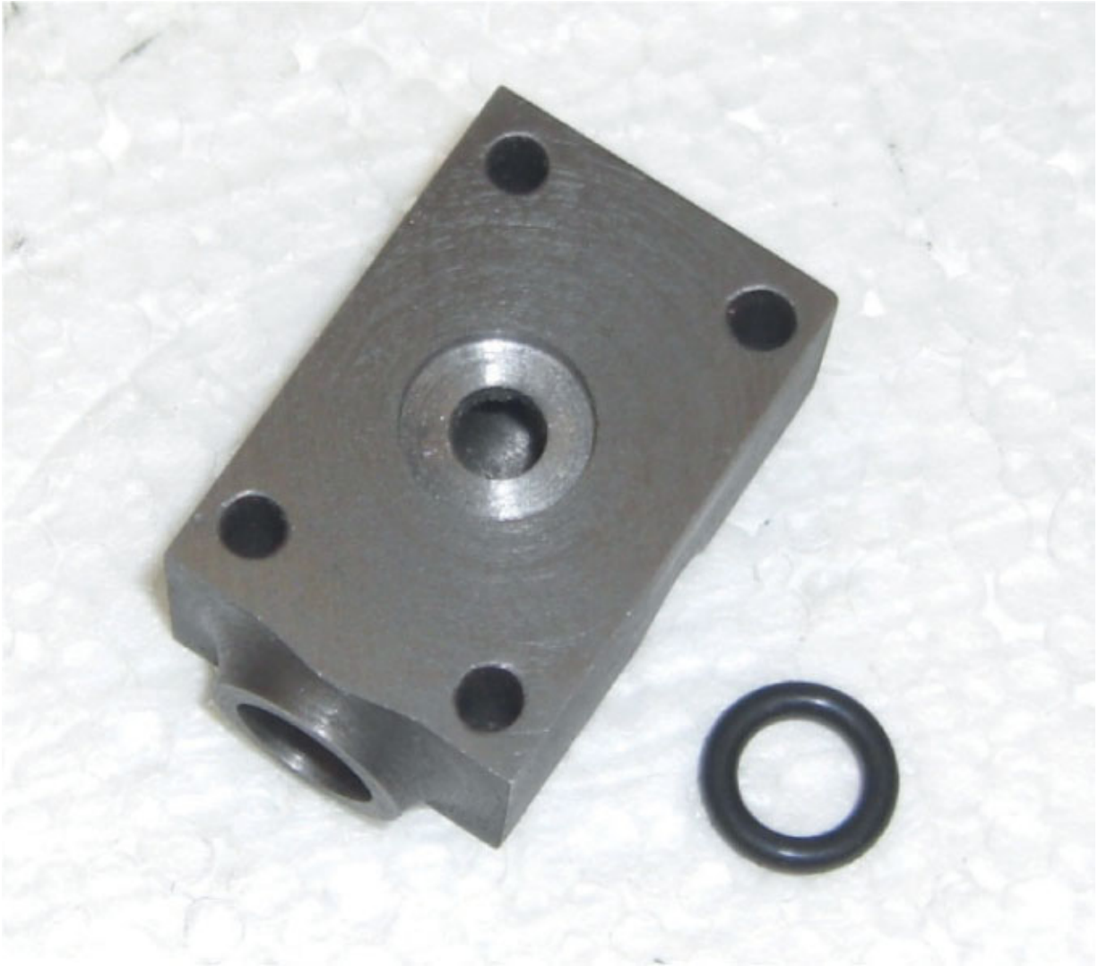
Regulator chest with 'O' ring recess around the steam passage.
