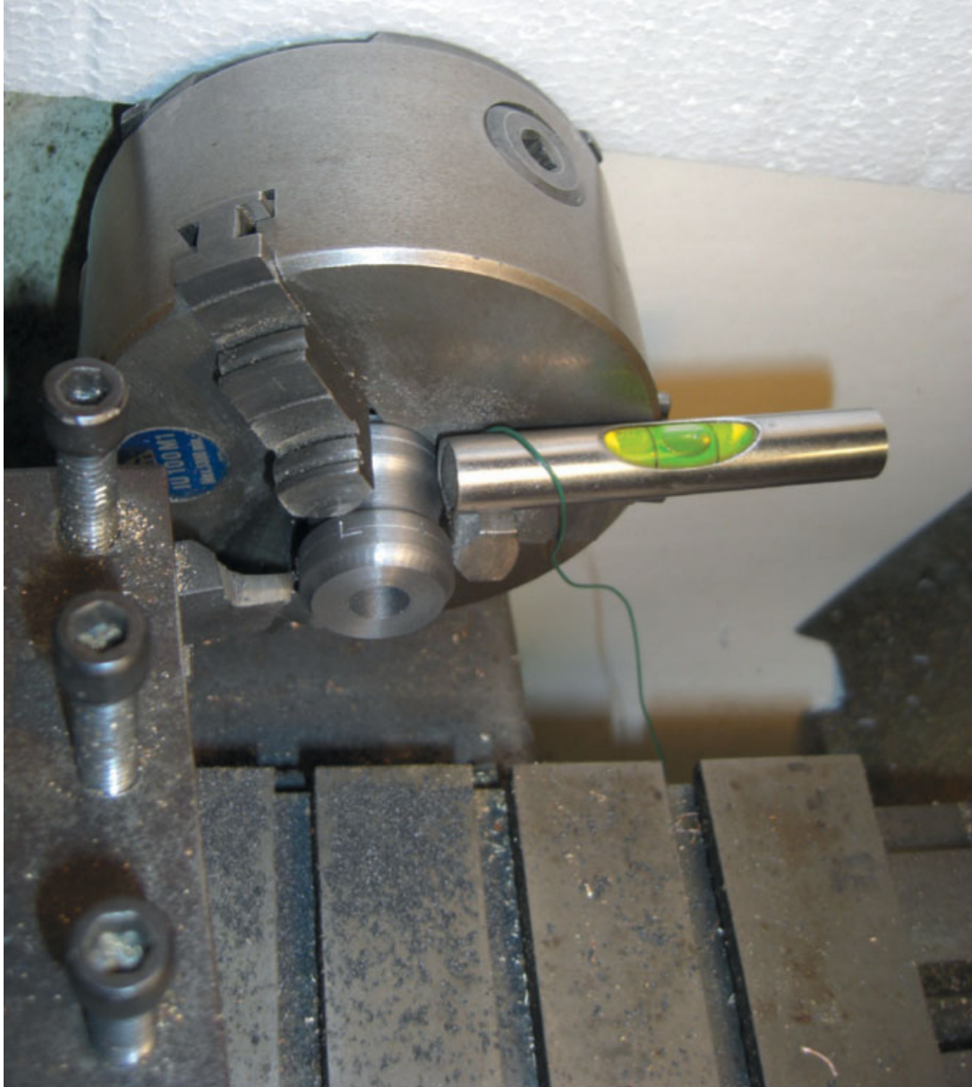
Dividing by six, using a spirit level on the chuck jaws.
