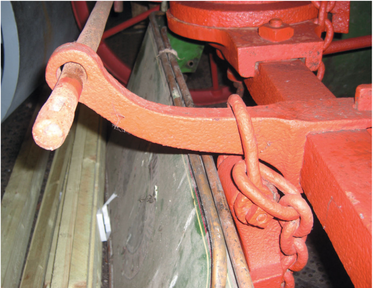
Towing eye for horse shafts, clamped to front axle of preserved engine.
