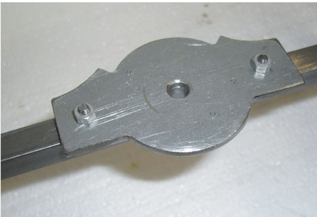
Fore axle with central plate to limit lock.
