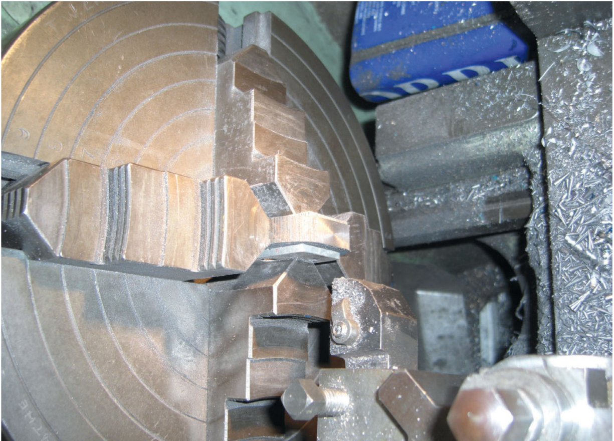
Facing the end of the valve chamber.
