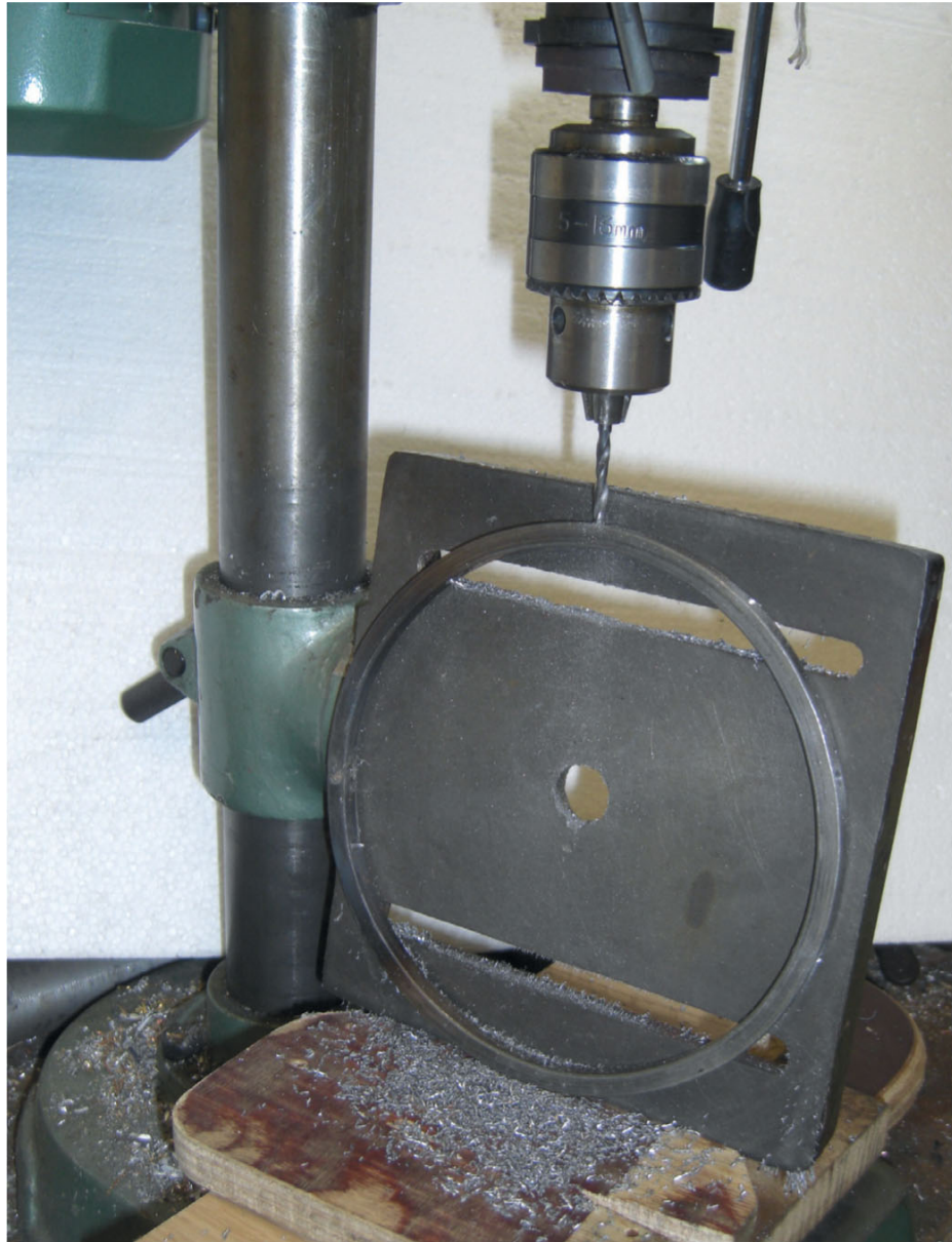
Drilling the spoke holes in the rim.
