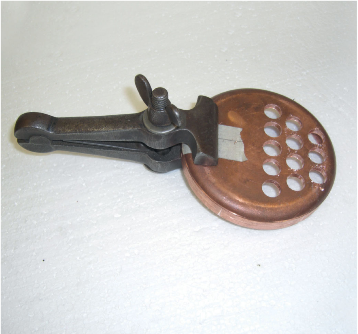
Safe work holding to drill the tube holes in the front tube plate.
