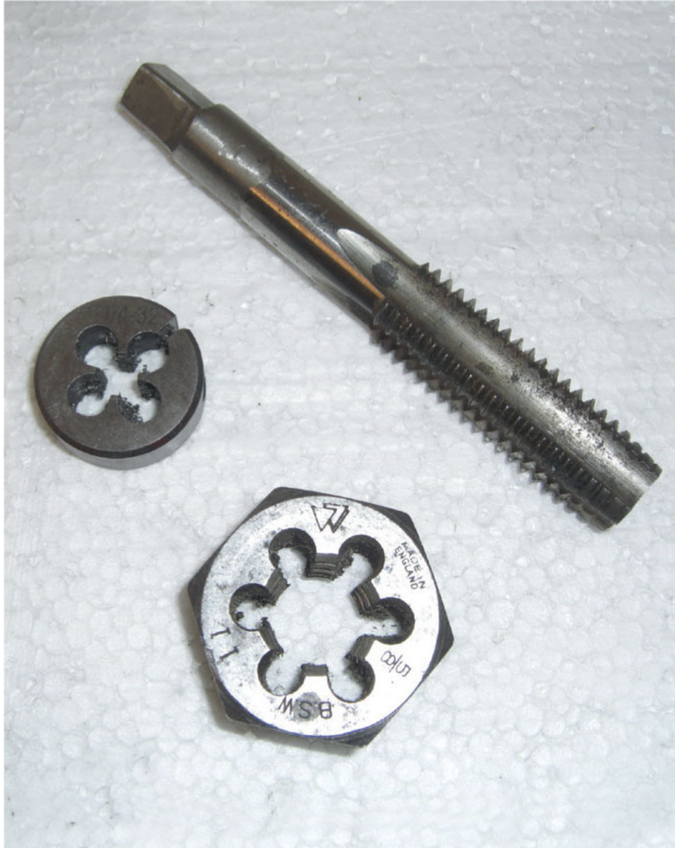
Second tap, split button die and die nut for final sizing.
