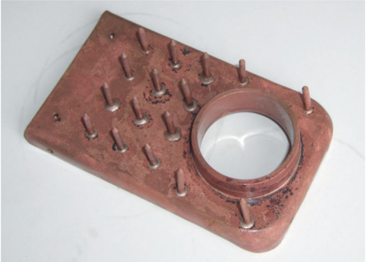
Firebox door-plate with fire-hole and stays silver soldered in place.
