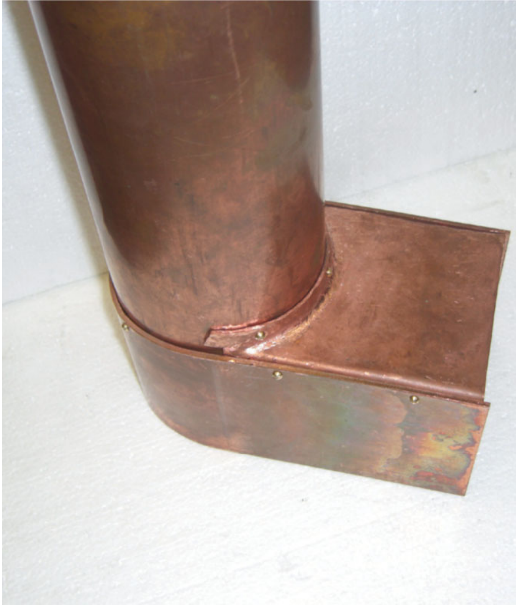
Barrel, throat plate and outer wrapper ready for silver soldering.
