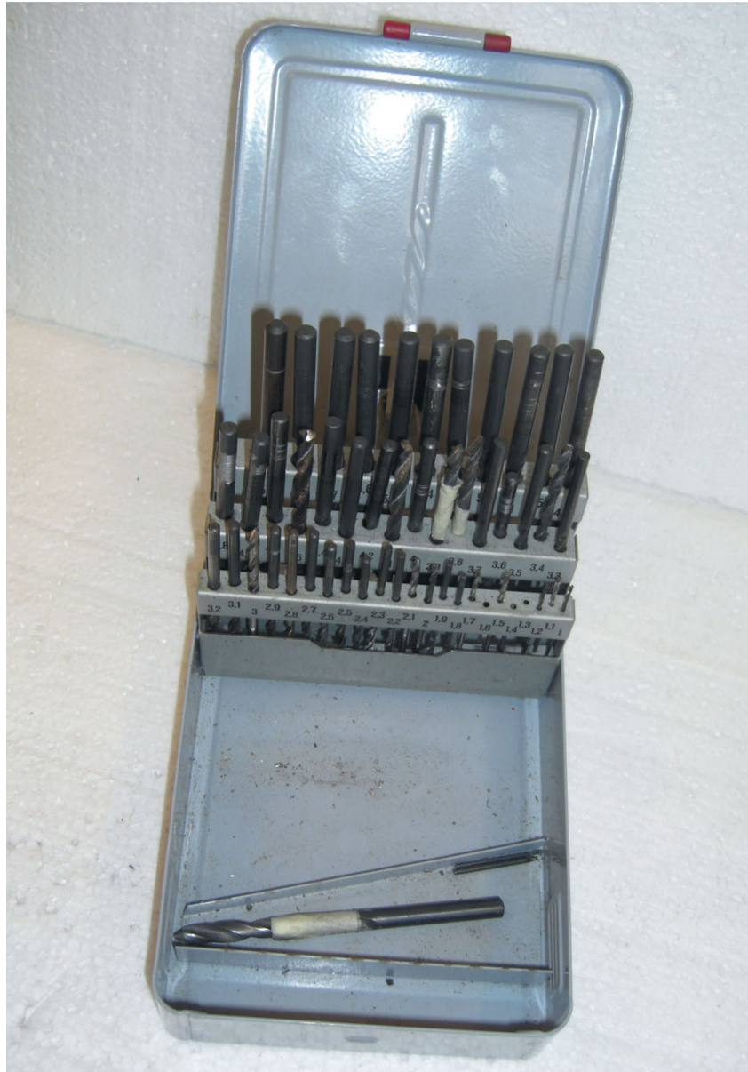
Drill set covering 1 to 5.9mm.
