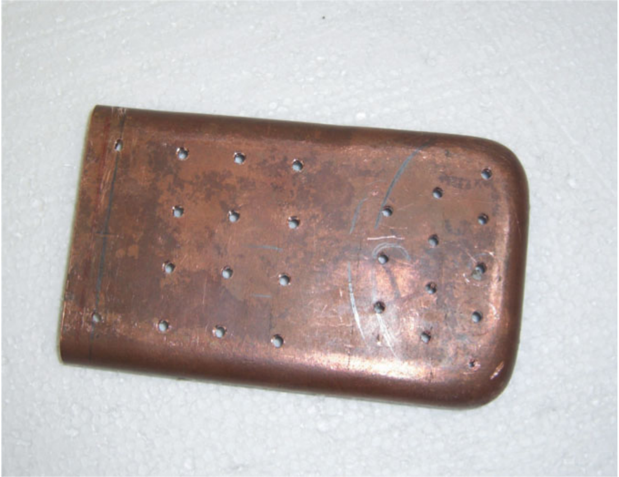
Firebox tube plate. Stay holes and tube pilot holes drilled.
