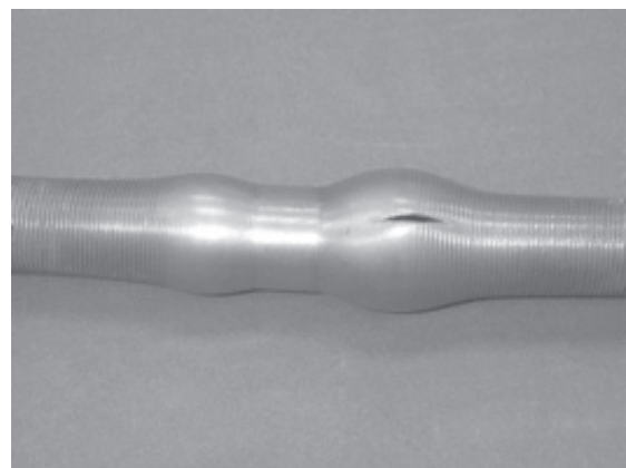
Figure 5-30. Chiller tube after freezing
