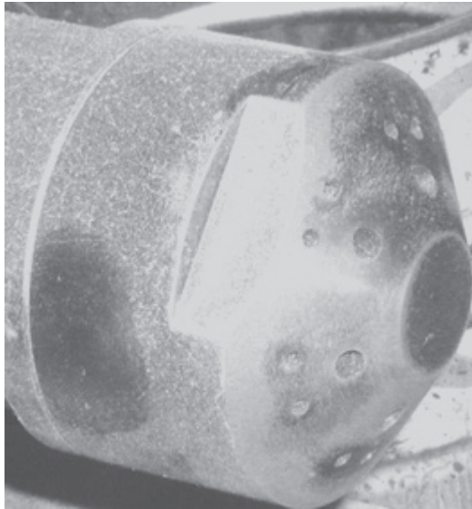
Figure 10-53. Irregular drilling in oil tip
