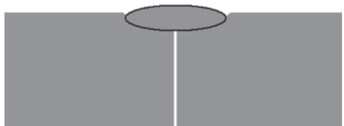
Figure 6-23. Incomplete weld section
