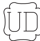
FIG. UG-129.2 OFFICIAL SYMBOL FOR STAMP TO DENOTE THE AMERICAN SOCIETY OF MECHANICAL ENGINEERS' STANDARD FOR NONRECLOSING PRESSURE RELIEF DEVICES
