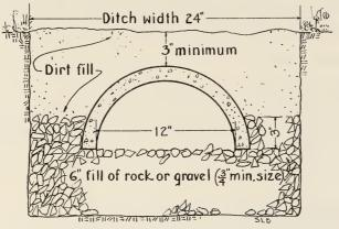
Fig. 16.—Cross section of half-section pipe drain line.
