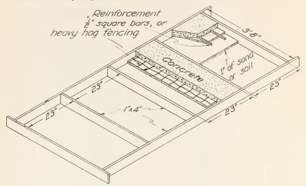
Fig. 13.—The form for cover slabs.
