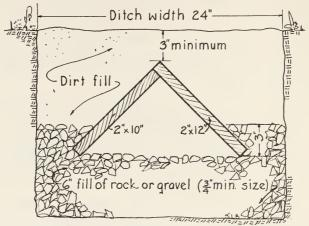
Fig. 14.-Cross section of V-trough drain line
