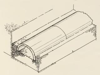
Fig. 17 .--- View of half-section concrete pipe in trench.
