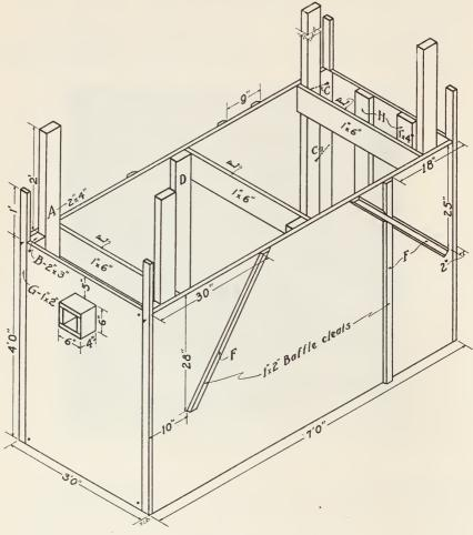
Fig. 5.—View of form for septic tank.
