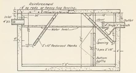
Fig. 2.—Longitudinal view of septic tank. The size shown is recommended for not more than 7 persons.
