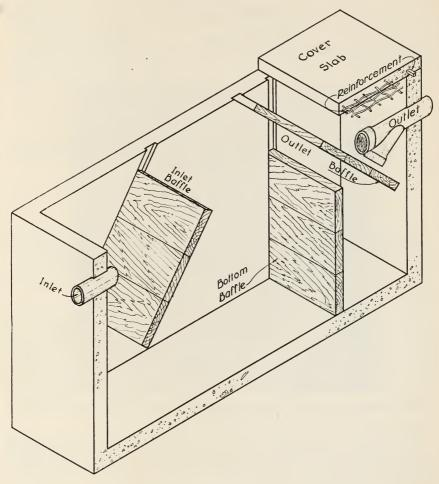
Fig. 3.—Half-section view of septic tank.
