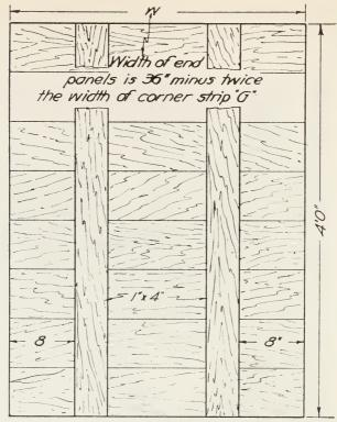
Fig. 10.—End panel. Four 6d nails, one at each corner, hold the end panels to the  $2 \times 3$  inch studding *B*, figure 5.
