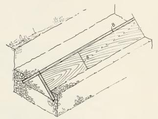
Fig. 15.—View of V-trough in trench. Joints should be staggered as at A and B.
