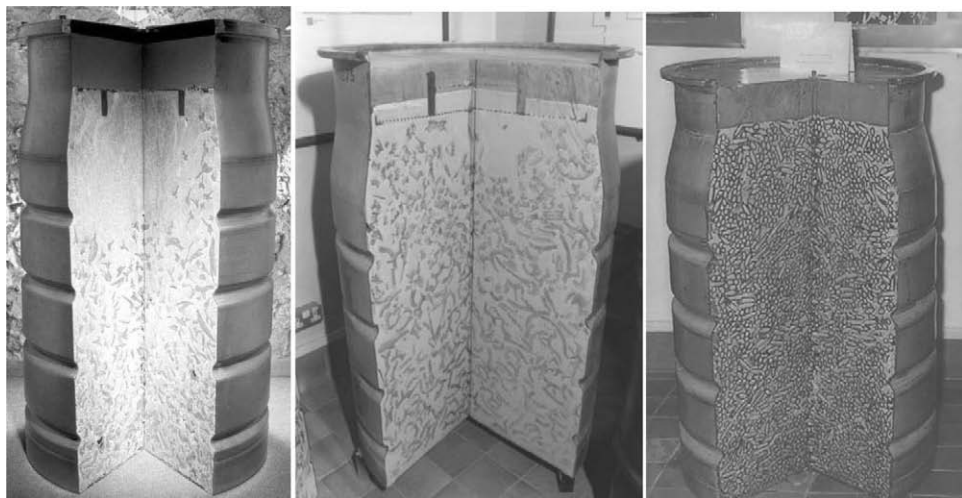
Figure 15.9: Cement-encapsulated solid, liquid and slurry ILW in 500-L drums. Courtesy of BNFL.
