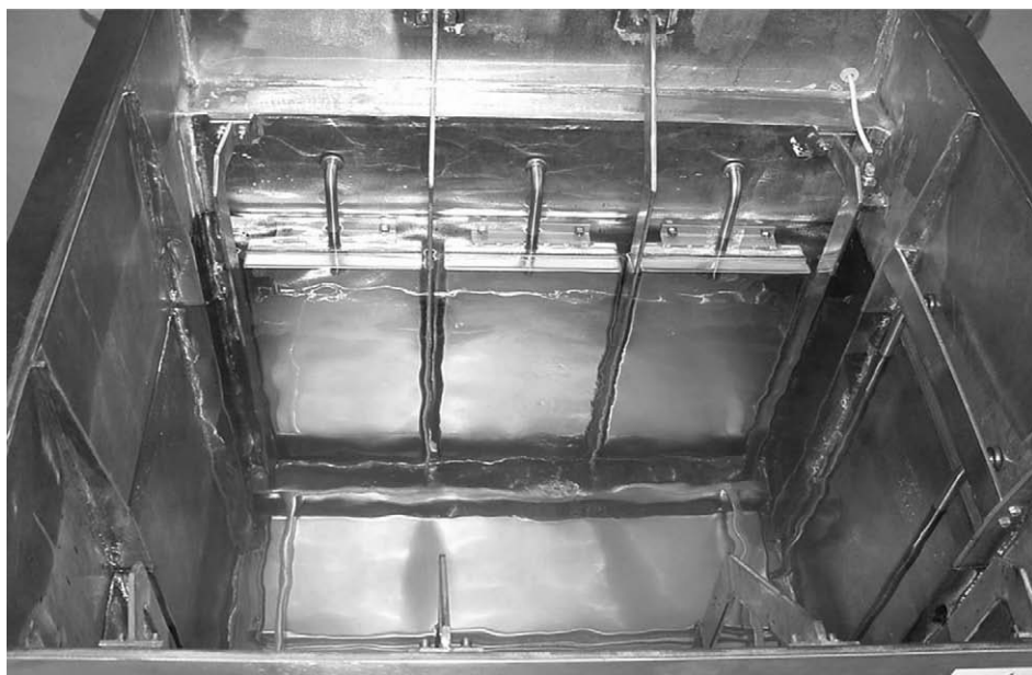
Figure 13.2: Chemical ultrasonic bath. Courtesy M. Prazska, All Deco, Slovakia.
