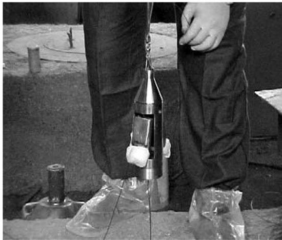
Figure 12.6: Smear test kit for repository loading channels. Authors' photo.
