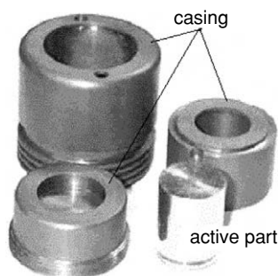
Figure 10.2: ^{60}\text{Co} commercial sealed radioactive sources used in industry and medicine.
