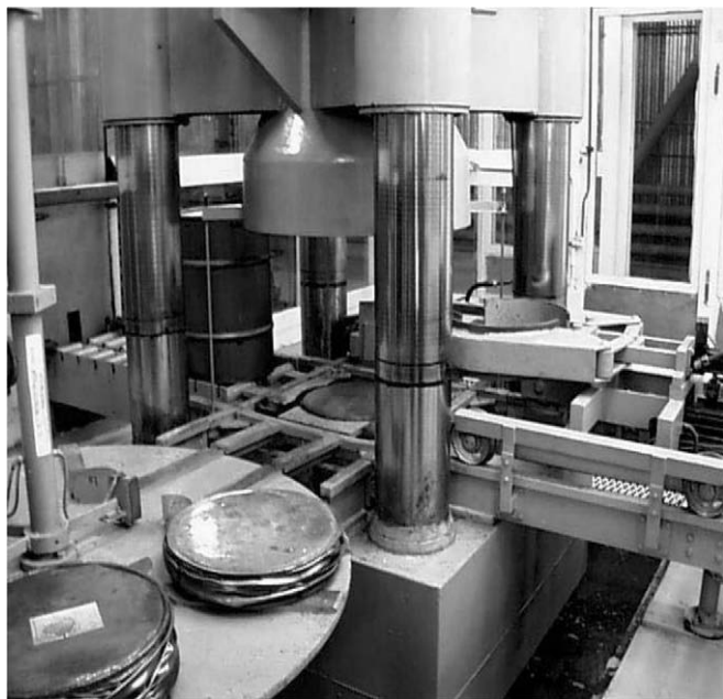
Figure 14.10: Super-compacting of radioactive waste drums. Courtesy of F.A. Lifanov, SIA RADON, Russia.
