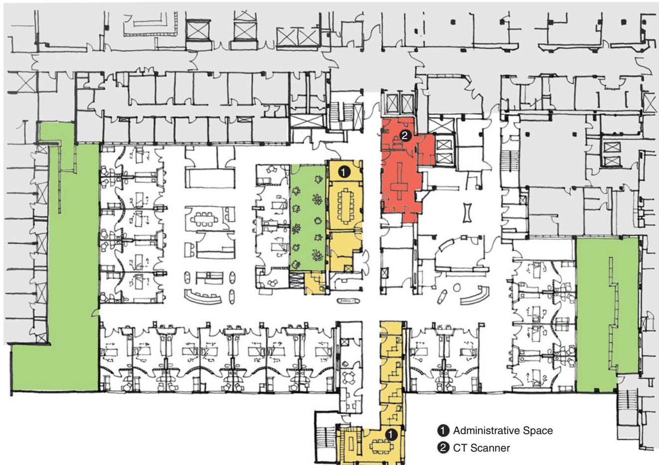
Fig. 3.16 Emory University Hospital Neurosciences ICU, Atlanta, Georgia, 2008 winner. Administrative and support spaces within the unit (Courtesy of WHR Architects)
