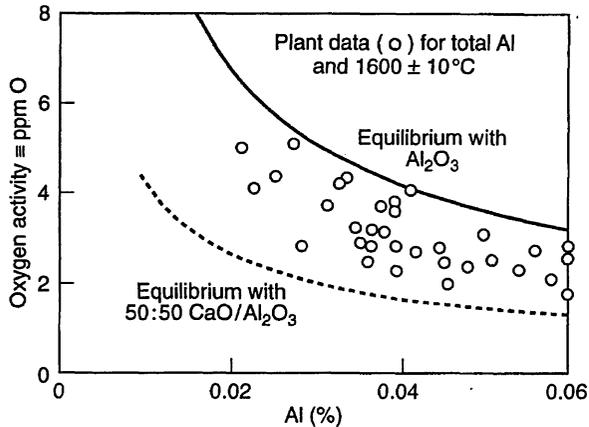
Fig. 9.20 Plant data for deoxidation with Al and calcium aluminate ladle slag during furnace tapping compared with equilibrium values for  $\text{Al}_2\text{O}_3$  and molten calcium aluminate (50:50  $\text{CaO}/\text{Al}_2\text{O}_3$ ) inclusions.
