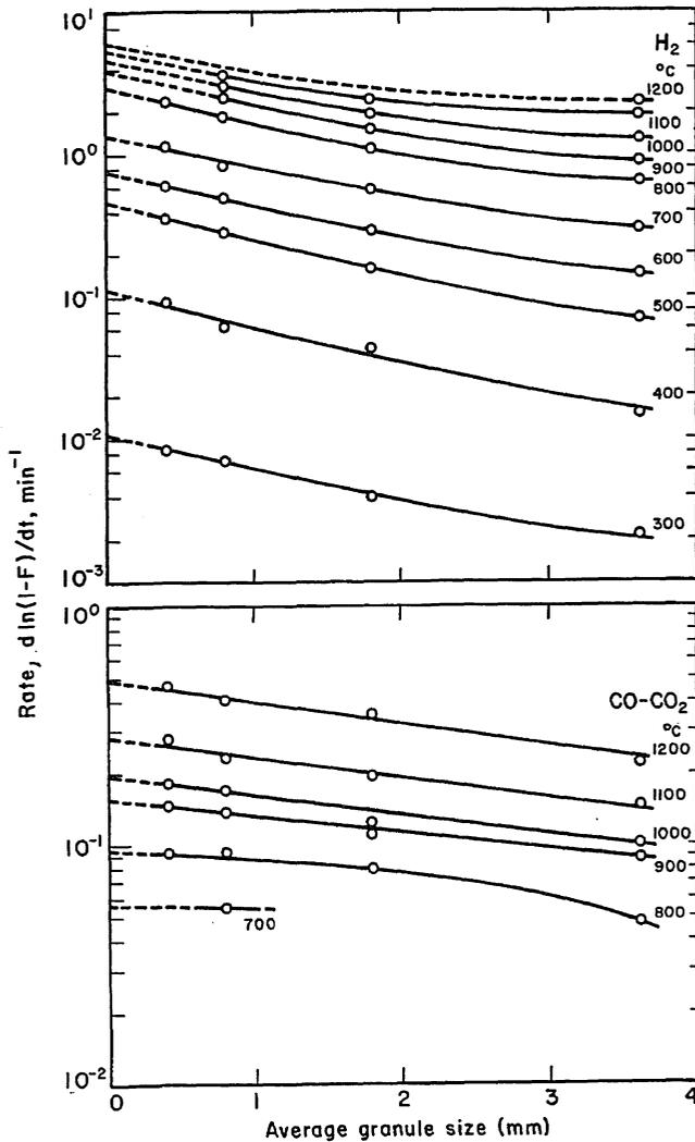
Fig. 2.19 Effect of granule size on the rate of internal reduction of haematite ore in H<sub>2</sub> and 90% CO + 10% CO<sub>2</sub> mixture. From Ref. 42.
