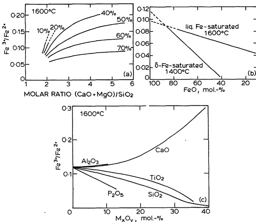
Fig. 5.29 Effect of slag composition on the ratio  $Fe^{3+}/Fe^{2+}$  in melts saturated with metallic iron at 1600°C: (a) CaO-MgO-SiO<sub>2</sub>-FeO melts at indicated molar concentrations of total iron oxide FeO; (b) MgO-SiO<sub>2</sub>-FeO melts; (c) pseudobinary FeO-M<sub>x</sub>O<sub>y</sub> melts. From Ref. 25.
