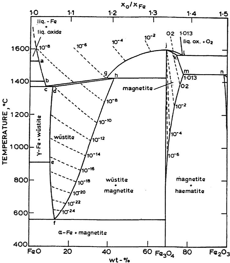
Fig. 4.17 Iron–oxygen phase equilibrium diagram between FeO and Fe<sub>2</sub>O<sub>3</sub> compositions, based mainly on the data of Darken and Gurry<sup>16</sup>; broken lines in single phase regions are oxygen isobars in bar.
