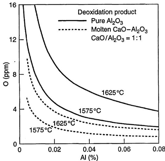
Fig. 6.19 Deoxidation with aluminium in equilibrium with  $\text{Al}_2\text{O}_3$  or molten calcium aluminate with  $\text{CaO}/\text{Al}_2\text{O}_3 = 1:1$ .
