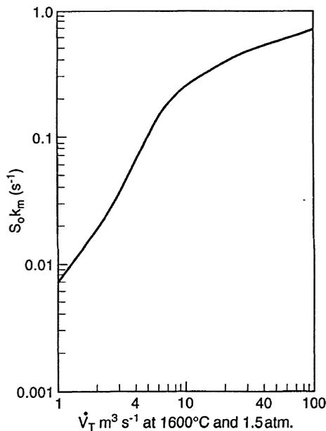
Fig. 2.32 Calculated rate constant for mass-transfer controlled reaction of gas bubbles in 220 ± 20 tonne steel bath in the BOF or Q-BOP vessel.
