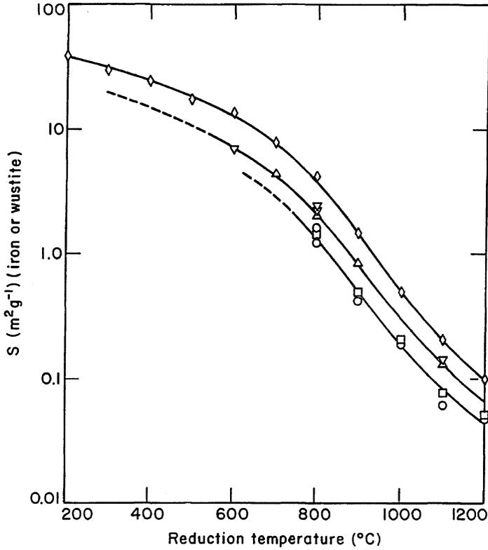
Fig. 2.22 Connected internal pore surface area of iron and wustite formed by reduction of haematite ores A and B; (a) ore A reduced to iron in  $H_2$  ( $\diamond$ ); (b) ore B reduced to iron in  $H_2$  ( $\nabla$ ) and reduced to wustite in an  $H_2$ - $H_2O$  mixture ( $\Delta$ ); (c) ore B reduced to iron in a  $CO$ - $CO_2$  mixture ( $\square$ ) and reduced to wustite in another  $CO$ - $CO_2$  mixture ( $\circ$ ). From Ref. 42.
