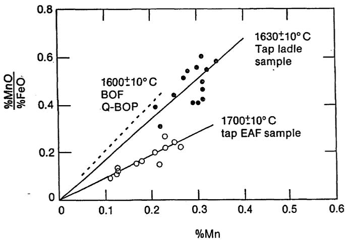
Fig. 9.17 Manganese content of steel in EAF at tap and in tap ladle is related to %MnO/%FeO ratio in furnace and ladle slags. From Ref. 10.
