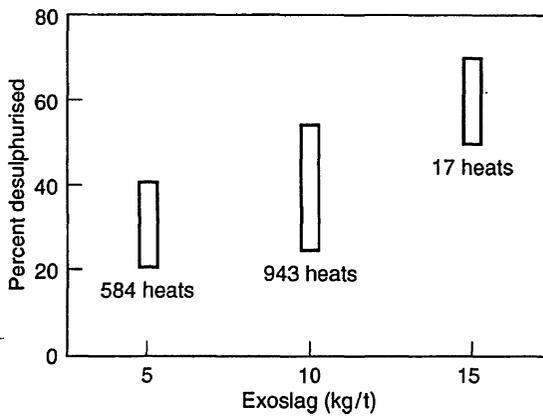
Fig. 9.25 Percent sulphur removed during furnace tapping increasing with an increase in amount of EXOSLAG in tap ladle. From Ref. 15.
