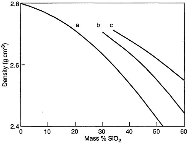
Fig. 5.38 Densities of CaO–MgO–Al<sub>2</sub>O<sub>3</sub>–SiO<sub>2</sub> melt at 1550°C, using data in Refs. 40–42. a: 0% MgO, CaO/Al<sub>2</sub>O<sub>3</sub> = 1; b: 0% MgO, 5% Al<sub>2</sub>O<sub>3</sub>; c: 5% MgO, 5% Al<sub>2</sub>O<sub>3</sub>.
