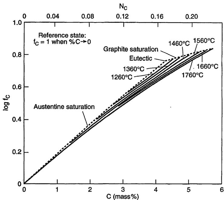
Fig. 4.4 Activity coefficient ( $f_C$ ) of carbon in liquid iron.
