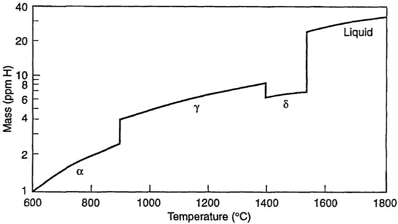
Fig. 4.5 Solubility of hydrogen in pure iron (or low-alloy steels) at 1 atm pressure of  $H_2$ .
