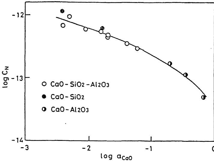
Fig. 5.27 The relation between the nitride capacity and the activity of lime for CaO-SiO<sub>2</sub>-Al<sub>2</sub>O<sub>3</sub> slag at 1550°C. From Ref. 24.
