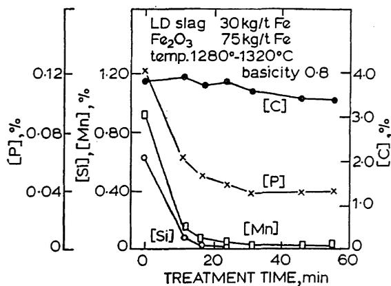
Fig. 7.8 Changes in hot metal composition during dephosphorisation treatment from data reported by Nashiwa *et al.*<sup>5</sup>
