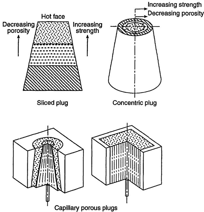
Fig. 9.8 Typical examples of porous plugs. From Ref. 4.
