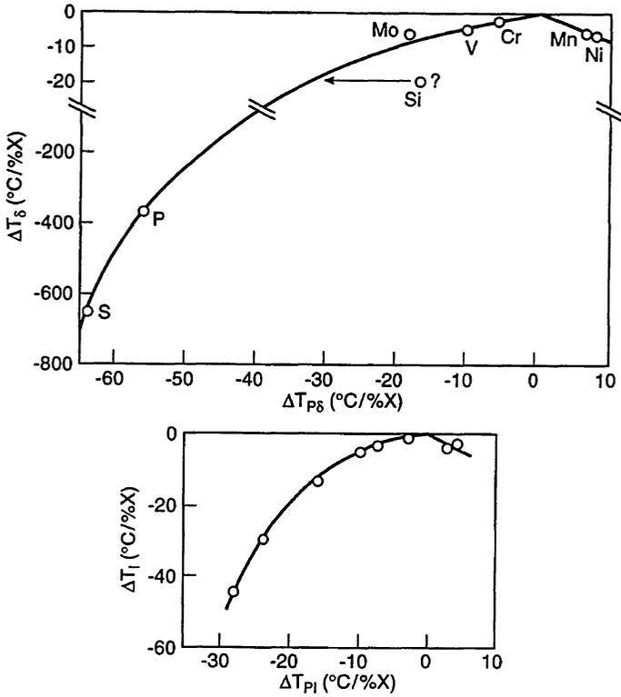
Fig. 4.13 Linear decrease in solidus,  $\Delta T_{\delta}$ , and liquidus,  $\Delta T_l$ , temperatures at low solute contents in binary systems Fe-X, related to changes in peritectic temperatures with respect to the binary Fe-C system.
