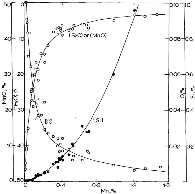
Fig. 6.15 Concentrations of Mn, Si and O in liquid iron equilibrated with SiO<sub>2</sub>-saturated iron-manganese silicate melts at 1600° ± 10°C. From Ref. 21.
