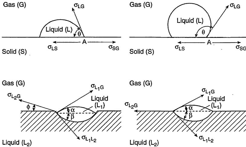
Fig. 1.19 Contact angles at solid-liquid and liquid-liquid interfaces.
