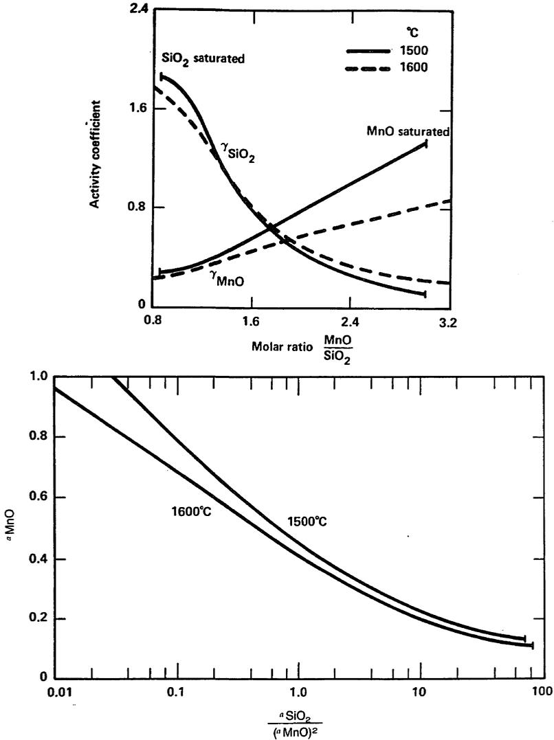
Fig. 6.16 Activities in MnO–SiO<sub>2</sub> melts with respect to solid oxides, derived from the experimental data in Refs. 22 and 23.
