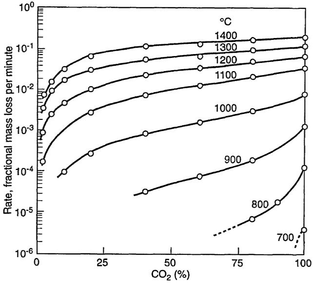
Fig. 2.13 Effect of temperature and gas composition on the rate of oxidation of granular metallurgical coke ( $\sim 0.5$  mm dia.) in CO<sub>2</sub>-CO mixtures at 0.96 atm total pressure. From Ref. 28.
