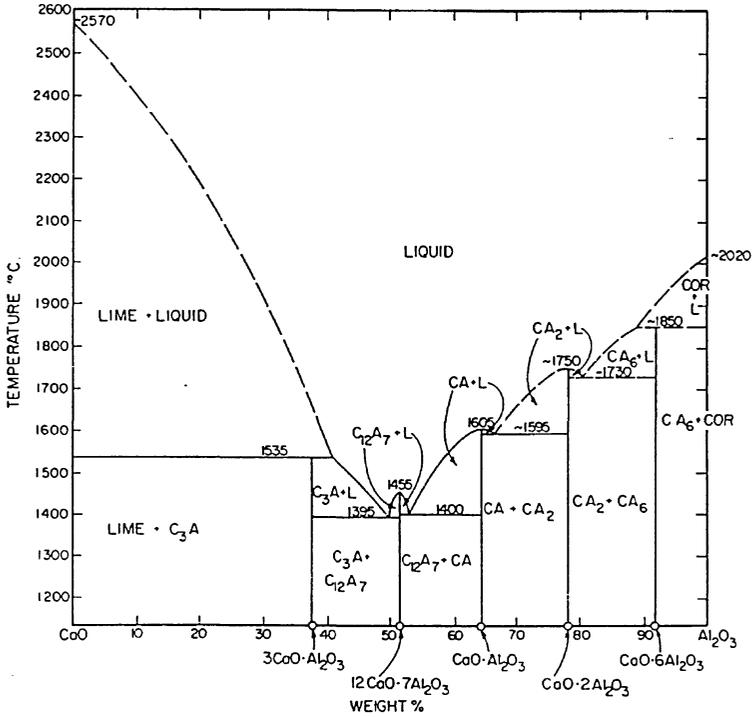
Fig. 5.9 Phase diagram for CaO–Al<sub>2</sub>O<sub>3</sub> system.
