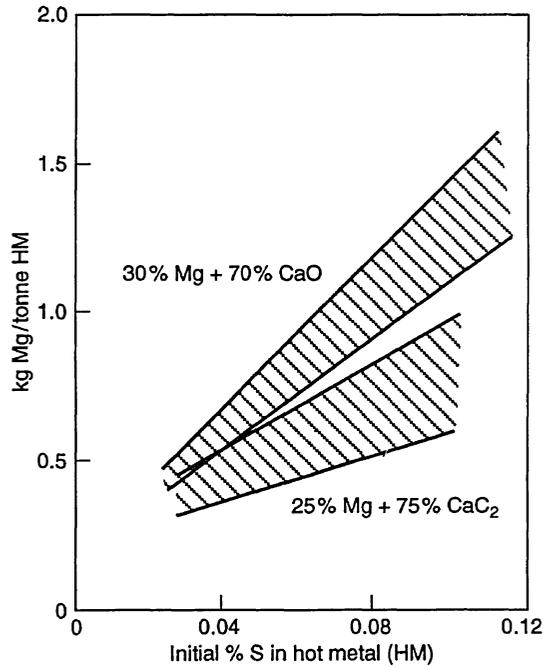
Fig. 7.10 Plant data within shaded area showing magnesium usage in hot metal desulphurisation with Mg+CaO and Mg+CaC<sub>2</sub> injection in the transfer ladle at the rate of 30 to 40 kg min<sup>-1</sup>.
