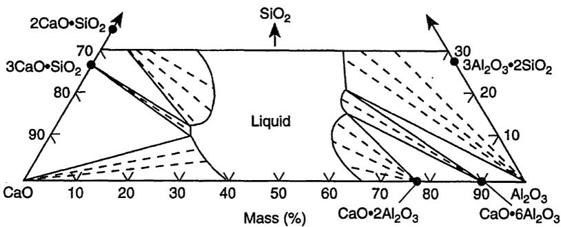
Fig. 5.17 Phase equilibria in the system CaO-Al<sub>2</sub>O<sub>3</sub>-SiO<sub>2</sub> at 1600°C.
