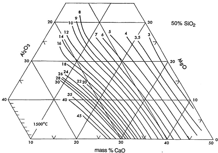
Fig. 5.41 Isokoms ( $0.1N \text{ s m}^{-2}$ ) for CaO–MgO–Al<sub>2</sub>O<sub>3</sub>–SiO<sub>2</sub> system at 1500°C for melts containing 35% and 50% SiO<sub>2</sub>. From Ref. 43.
