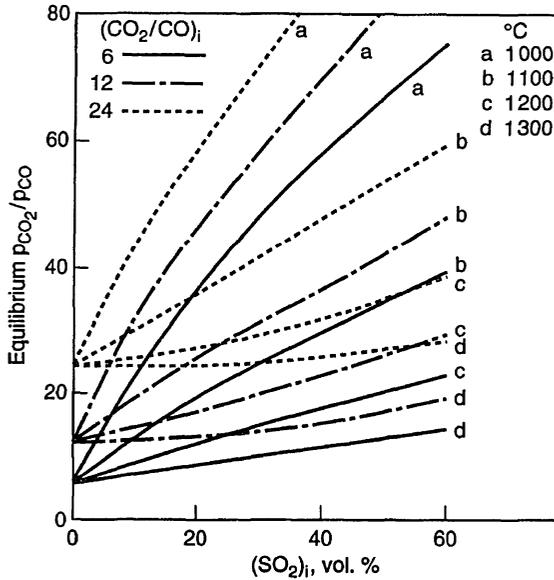
Fig. 3.3 Equilibrium ratios  $p_{CO_2}/p_{CO}$  at indicated temperatures as a function of pct  $(SO_2)_i$  for indicated ratios  $(CO_2/CO)_i$  in ingoing gas mixtures CO-CO<sub>2</sub>-SO<sub>2</sub> at atmospheric pressure.
