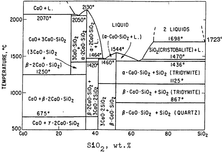
Fig. 5.6 Phase diagram for CaO-SiO<sub>2</sub> system.
