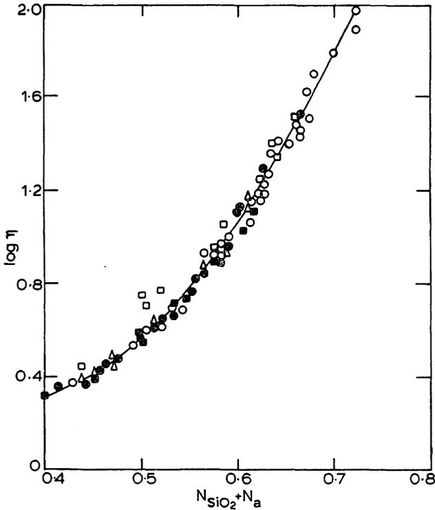
Fig. 5.42 Viscosities of CaO–MgO–Al<sub>2</sub>O<sub>3</sub>–SiO<sub>2</sub> melts at 1500°C as a function of SiO<sub>2</sub> and Al<sub>2</sub>O<sub>3</sub> contents. Points ○ ● ■ from Ref. 43; Points Δ from Ref. 45; points □ from Refs. 43 and 46.
