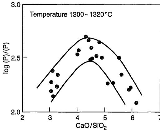
Fig. 7.7 Relation between  $\text{CaO}/\text{SiO}_2$  and phosphorus partition ratio.
