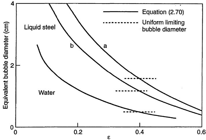
Fig. 2.31 Calculated bubble diameter for bubble fragmentation mechanism equation (2.70), compared with uniform limiting diameter at high ε values for water and liquid steel: (a) for O < 4 ppm and 40 ppm S (b) for 600 ppm O and 120 ppm S.
