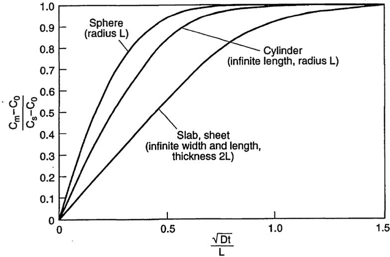
Fig. 2.5 Mean concentration or fractional saturation of slab, cylinder, or sphere of uniform initial concentration  $C_0$  and constant surface concentration  $C_s$ ,  $C_m$  is the mean concentration at time  $t$ .
