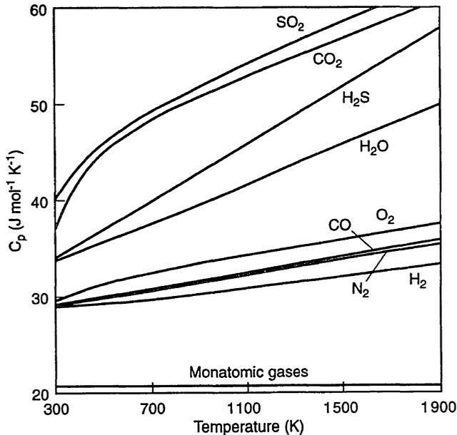
Fig. 3.1 Molar heat capacities of simple gases.
