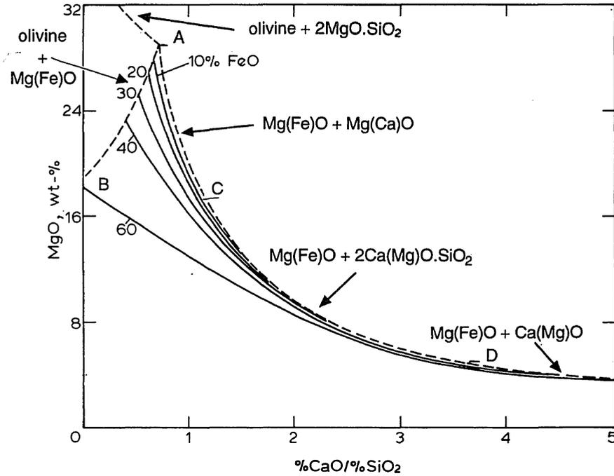
Fig. 5.15 Solubility of MgO, as magnesio-wustite, in the system CaO–MgO–SiO<sub>2</sub>–FeO at 1600°C as a function of slag basicity and FeO concentration, derived from the data in Fig. 5.14.
