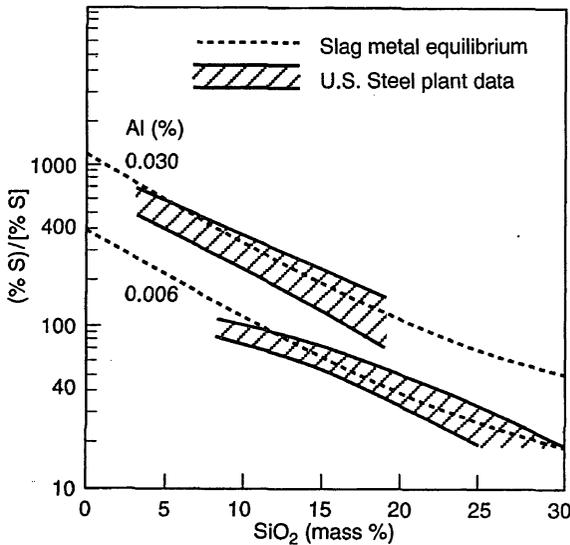
Fig. 9.23 Slag/metal sulphur distribution ratios after desulphurisation with lime-saturated  $\text{CaO-MgO-Al}_2\text{O}_3\text{-SiO}_2$  slags at  $1600 \pm 15^\circ\text{C}$  with steels containing residual  $0.006 \pm 0.002\%$  Al or  $0.03 \pm 0.01\%$  Al are compared with the equilibrium values.
