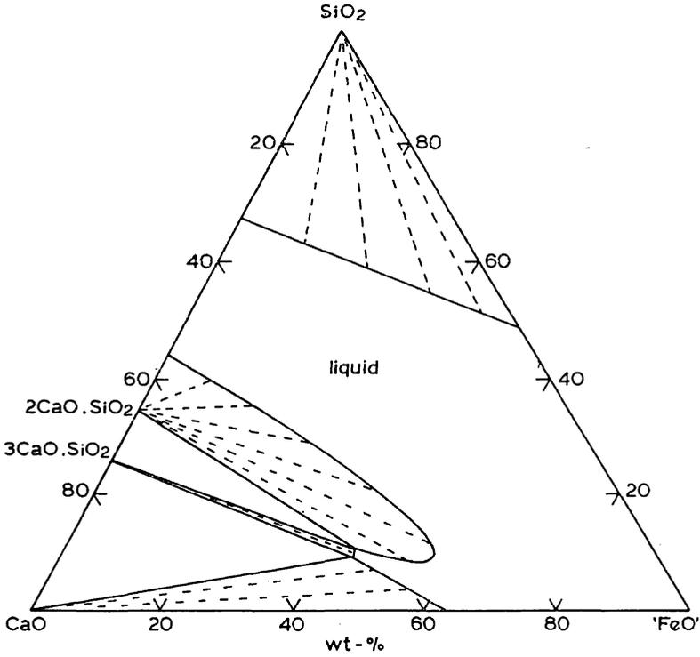
Fig. 5.11 Phase equilibria in the system CaO-SiO<sub>2</sub>-FeO in equilibrium with liquid iron at 1600°C.
