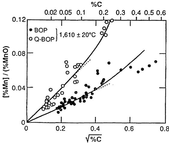
Fig. 8.20 Metal/slag manganese distribution ratios in BOP and Q-BOP are related to carbon content of steel at first turndown.
