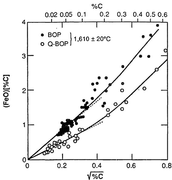
Fig. 8.19 Variation of product (FeO)[%C] with carbon content of steel at first turndown.
