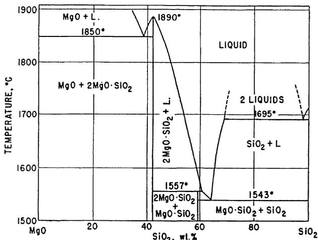
Fig. 5.8 Phase diagram for MgO-SiO<sub>2</sub> system.
