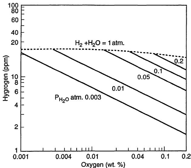
Fig. 4.7 Concentrations of hydrogen and oxygen in liquid iron at 1600°C in equilibrium with indicated compositions of H<sub>2</sub>-H<sub>2</sub>O mixtures.
