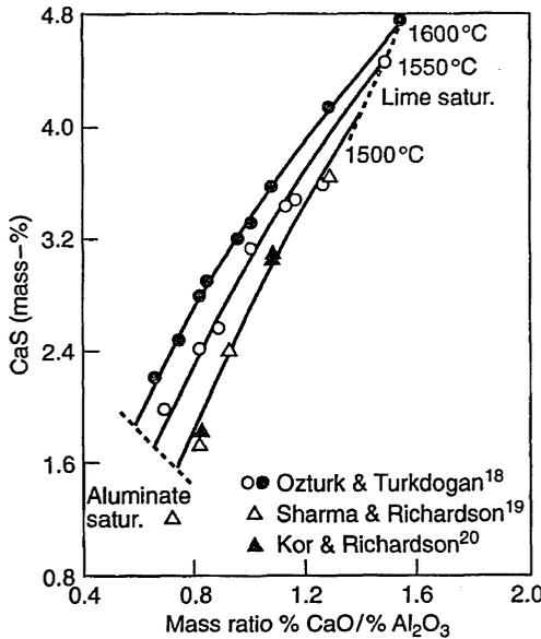
Fig. 6.13 Solubility of CaS in calcium aluminate melts at indicated temperatures as a function of mass ratio  $\% \text{CaO} / \% \text{Al}_2\text{O}_3$ .
