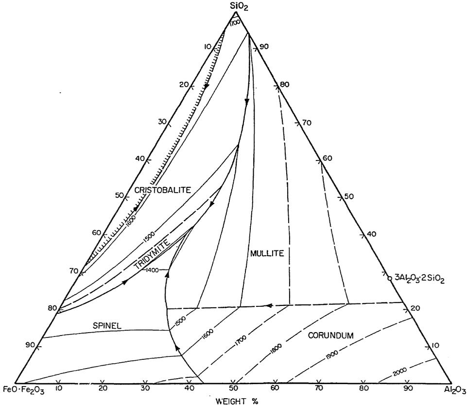
Fig. 1.15 Phase relations at liquidus temperatures in the system  $\text{Fe}_3\text{O}_4\text{-SiO}_2\text{-Al}_2\text{O}_3$  in air, based mainly on the data of Muan.<sup>13</sup>
