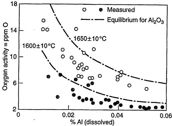
Fig. 9.21 Oxygen sensor measurements after Al deoxidation and hard argon stirring in 30 t AOD, reported by Riley and Nusselt.<sup>11</sup>
