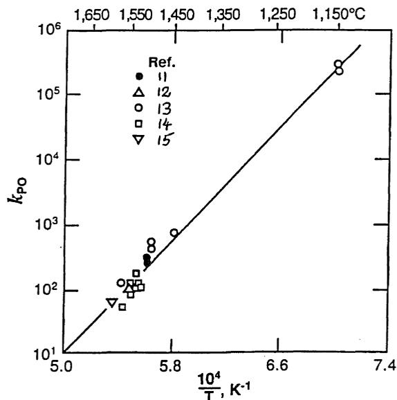
Fig. 6.8 Phosphate capacities of iron phosphate melts.
