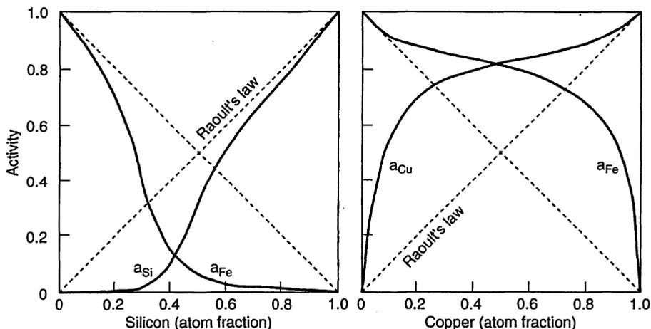
Fig. 1.6 Activities in liquid Fe-Si and Fe-Cu alloys at 1600°C showing strong negative and positive departures from Raoult's law.
