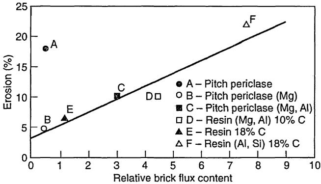
Fig. 9.1 Erosion by a 3-percent-SiO<sub>2</sub> slag vs. relative flux content. From Ref. 1.
