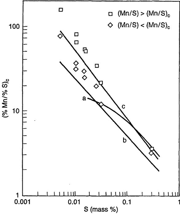
Fig. 10.10 The critical ratio  $(\%Mn/\%S)_c$  as a function of sulphur content of steel. Calculated lines: a Ref. 8, b Ref. 12, c Ref. 13; Experimental points:  $\square$ ,  $\diamond$  Ref. 14.
