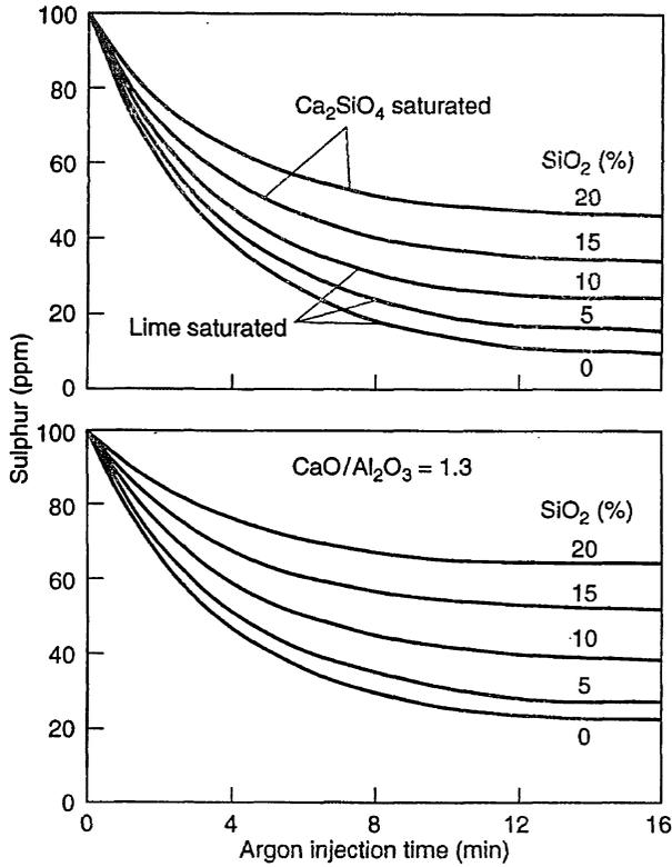
Fig. 9.28 Calculated rate curves for desulphurisation at 1600°C of a 200 t steel containing 0.03% Al with 2 t ladle slag and argon stirring at 1.5 Nm<sup>3</sup>min<sup>-1</sup> ( $\approx \epsilon$  100 Wt<sup>-1</sup>).
