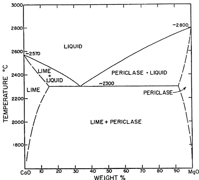
Fig. 5.5 Phase diagram for CaO–MgO system.
