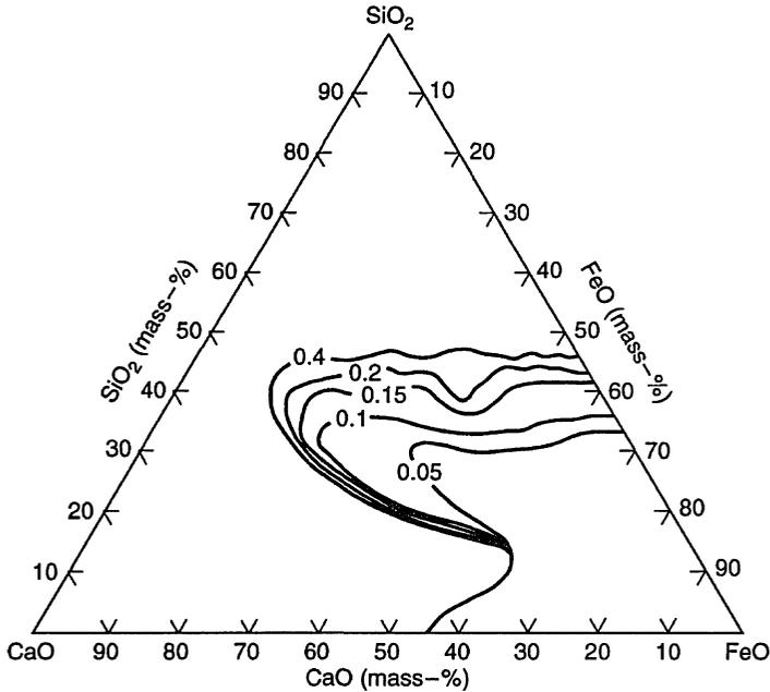
Fig. 5.43 Viscosity ( $\text{N s m}^{-2}$ ) of CaO–FeO–SiO<sub>2</sub> melts at 1400°C. From Ref. 27.
