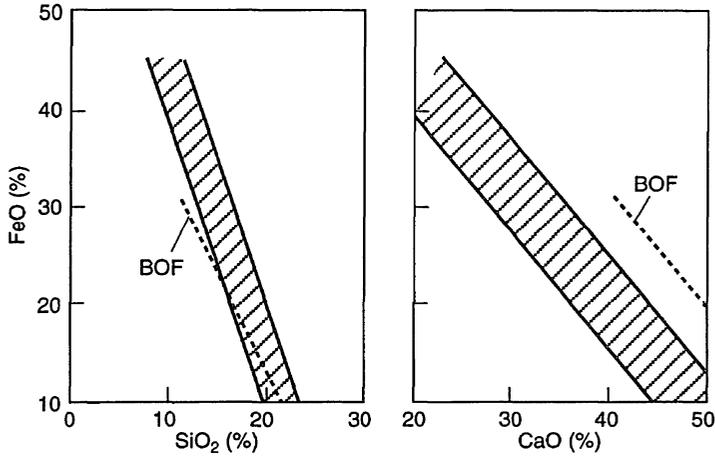
Fig. 8.25 FeO, SiO<sub>2</sub> and CaO contents of EAF slags at tap, are compared with the BOF slags.
