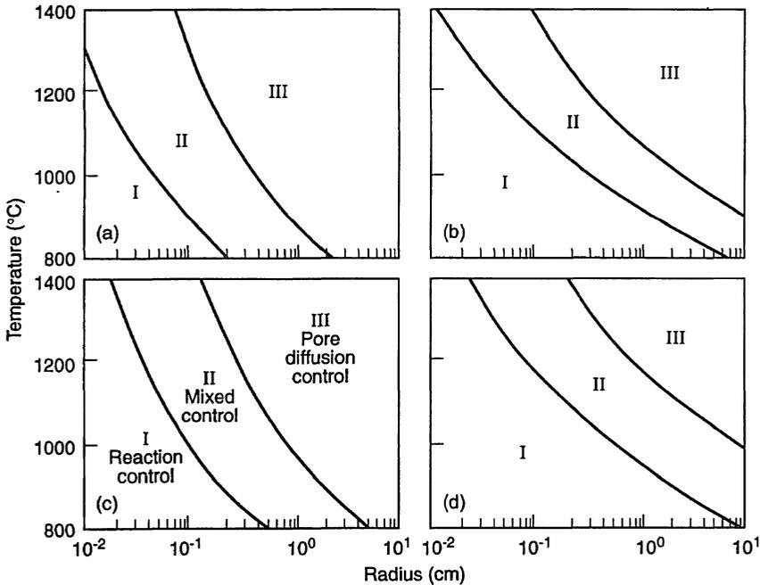
Fig. 2.15 Critical radius and temperature for the limiting rate controlling processes at 1 atm pressure. (a) Coke, 100 per cent CO<sub>2</sub>; (b) Coke, 1:1 CO:CO<sub>2</sub>; (c) Graphite, 100 per cent CO<sub>2</sub>; (d) Graphite, 1:1 CO:CO<sub>2</sub>. From Ref. 36.
