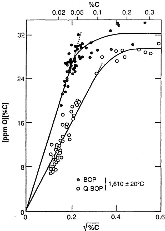
Fig. 8.17 Variation of product  $[\text{ppm O}][\%C]$  with carbon content of steel at first turndown.
