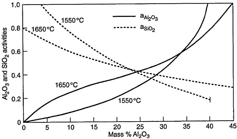
Fig. 5.21  $Al_2O_3$  and  $SiO_2$  activities in  $MnO-Al_2O_3-SiO_2$  system for mass ratio of  $MnO/SiO_2 = 1$ , derived from data compiled by Fujisawa & Sakao.<sup>14</sup>
