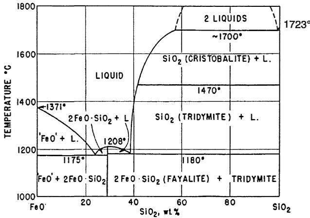
Fig. 5.7 Phase diagram for FeO-SiO<sub>2</sub> system.
