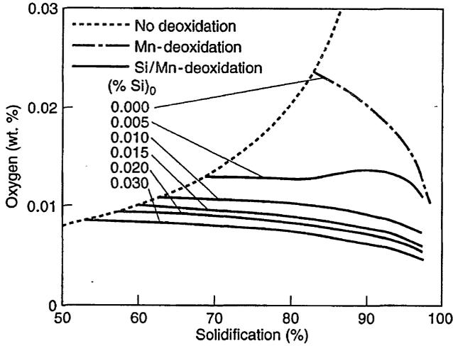
Fig. 10.2 Oxygen content of enriched liquid controlled by Si–Mn deoxidation during solidification. From Ref. 6.
