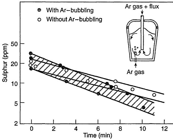
Fig. 9.29 Desulphurisation of liquid steel to very low levels with injection of (80% CaO + 20% CaF<sub>2</sub>). From Ref. 16.
