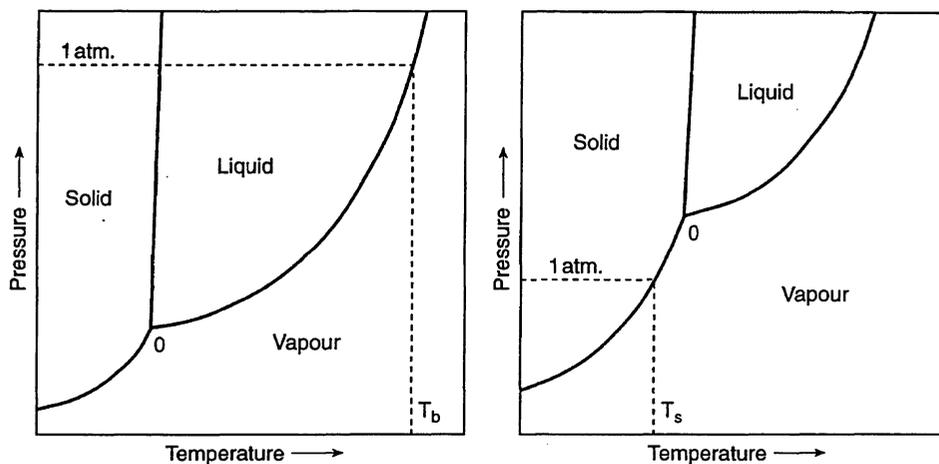
Fig. 1.8 Phase relations for single component systems.
