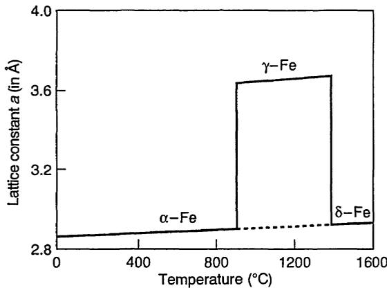
Fig. 4.8 Variation of lattice constant of pure iron with temperature.
