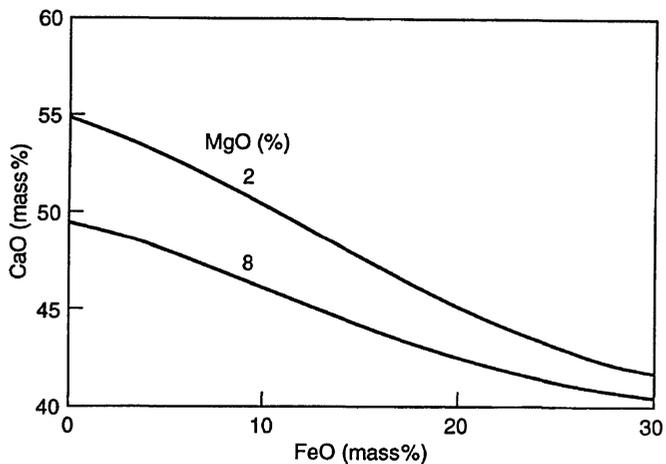
Fig. 5.13 Solubility of CaO in (CaO-MgO-SiO<sub>2</sub>-FeO) slags saturated with 2CaO-SiO<sub>2</sub> at 1600°C.
