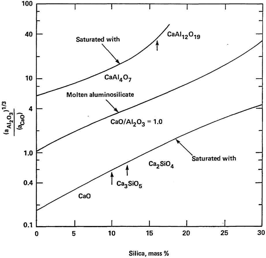
Fig. 5.20 Effect of slag composition on the activity ratio  $(a_{Al_2O_3})^{1/3}/a_{CaO}$  for the system  $CaO-Al_2O_3-SiO_2$  at  $1600^\circ C$ .
