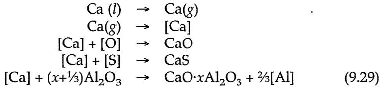
Depending on the steel composition, the manner of calcium injection and other process variables, there will be variations in the conversion of alumina inclusions to aluminates inclusions; the smaller inclusions will be converted to molten calcium aluminate more readily than the larger inclusions.
