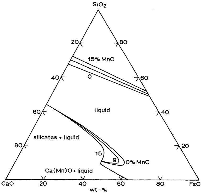
Fig. 5.16 Shift in the solubility isotherms at 1600°C with the addition of 9 and 15% MnO to the system CaO-SiO<sub>2</sub>-FeO; the total CaO, SiO<sub>2</sub> and FeO contents are related to 100%.
