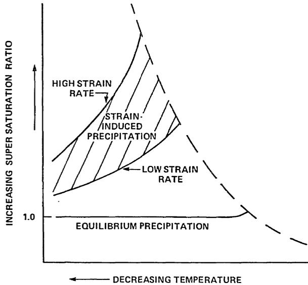
Fig. 10.16 Nitride and carbonitride precipitation from supersaturated solution in austenite.
