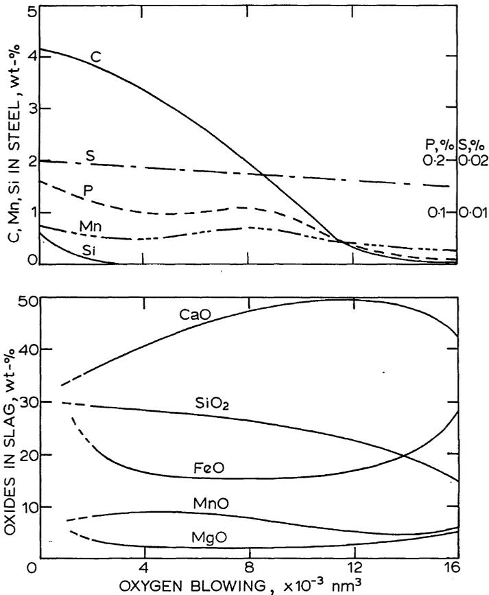
Fig. 8.4 Changes in metal and slag compositions during steelmaking in the BOF for about a 300 t melt, using data of van Hoorn *et al.*<sup>2</sup>.
