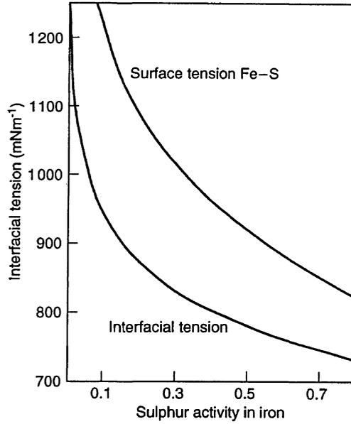
Fig. 5.33 Effect of sulphur in iron on the interfacial tension between liquid iron and CaO-Al<sub>2</sub>O<sub>3</sub>-SiO<sub>2</sub> melts, determined by Gaye *et al.*<sup>30</sup> is compared to the surface tension of Fe-S melts at 1600°C.
