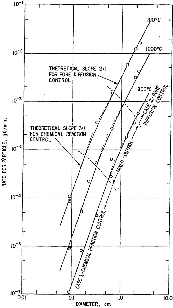
Fig. 2.10 · Rate of oxidation of electrode graphite as a function of particle diameter for 0.96 atm CO<sub>2</sub>. From Ref. 27.
