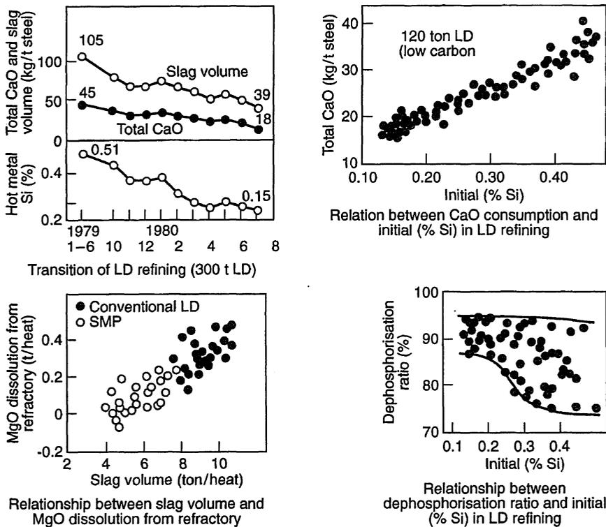
Fig. 7.11 Selected diagrams from a paper by Itoh *et al.*<sup>8</sup> on the development of slag minimum refining process (SMP) by Nippon Steel Corporation.
