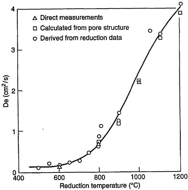
Fig. 2.24  $\text{H}_2\text{-H}_2\text{O}$  effective diffusivity derived from data for rate of reduction of haematite to iron is compared with that obtained by direct measurements and calculated from pore structure. From Ref. 43.
