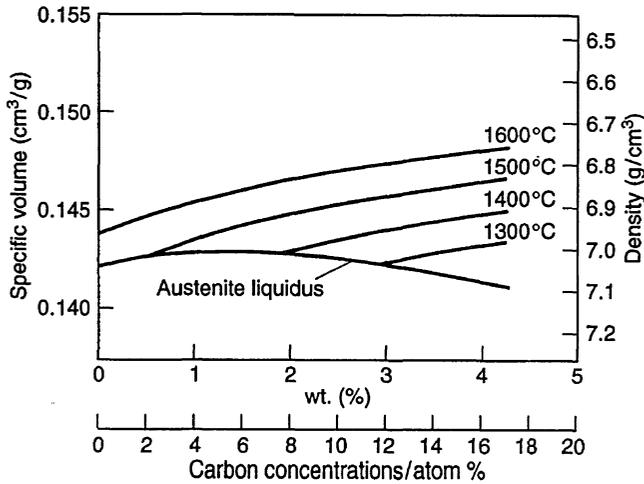
Fig. 4.36 Density of iron-carbon alloys. From Ref. 48.
