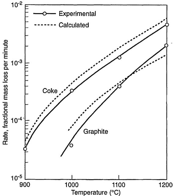
Fig. 2.14 Effect of temperature on rate of oxidation of coke and graphite (1.9 and 2.2 cm dia. spheres, respectively) in 50:50  $\text{CO}_2$ - $\text{CO}$  at 1 atm. From Ref. 36.
