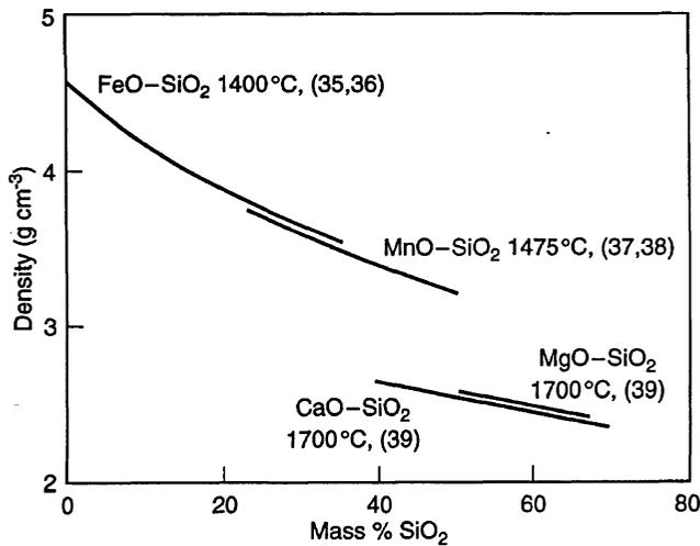
Fig. 5.37 Densities of binary silicate melt. From Refs. 35-39.
