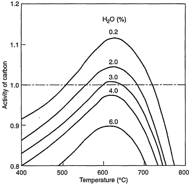
Fig. 3.4 Calculated activity of carbon for complete gas equilibrium at 4 atm and indicated temperatures for reformed natural gas containing 73% H<sub>2</sub>, 18% CO, 8% CO<sub>2</sub> and 1% CH<sub>4</sub> to which an indicated amount of H<sub>2</sub>O is added.
