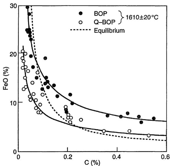
Fig. 8.18 Iron oxide-carbon relations in BOP and Q-BOP are compared with the average equilibrium relation (----).
