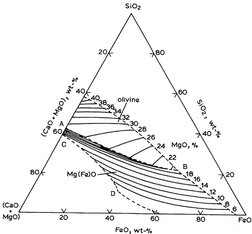
Fig. 5.14 Iso-MgO concentrations (wt.%) for CaO-MgO-SiO<sub>2</sub>-FeO slags saturated with olivine and magnesio-wustite in equilibrium with liquid iron at 1600°C.
