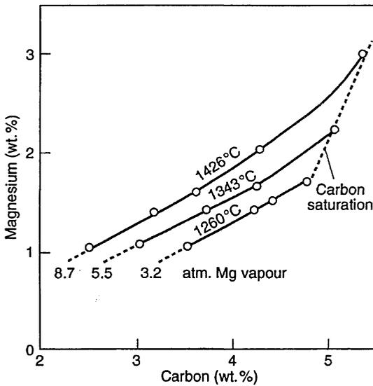
Fig. 4.27 Solubility of magnesium in liquid iron-carbon alloys at indicated temperatures and pressures of magnesium vapour. From Ref. 30.
