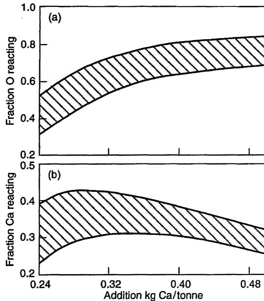
Fig. 9.22 Fractions of oxygen and calcium reacting in deoxidation of semi-killed steel ( $\sim 75$  ppm O) with Cal-Sil (30% Ca) cored-wire injection are related to the amount of Ca added, derived from plant data reported by Thomas *et al.*<sup>12</sup>
