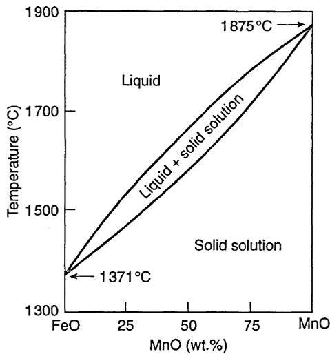
Fig. 5.4 Phase diagram for  $\text{FeO}$ – $\text{MnO}$  system.
