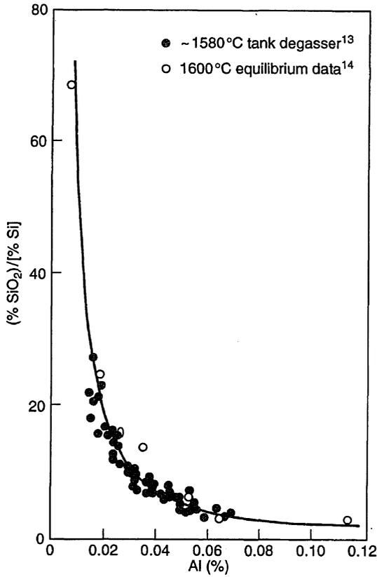
Fig. 9.24 Tank degasser data are compared with the experimental equilibrium data for aluminium reduction of silica from lime-saturated calcium aluminate melts containing SiO<sub>2</sub> < 5%.
