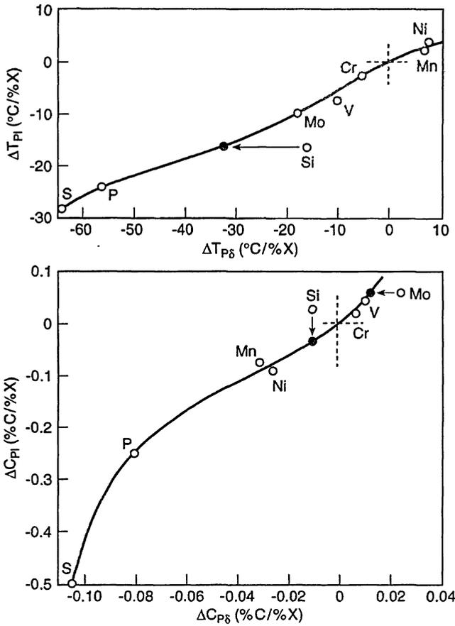
Fig. 4.15 Interrelations between peritectic temperature and composition changes.
