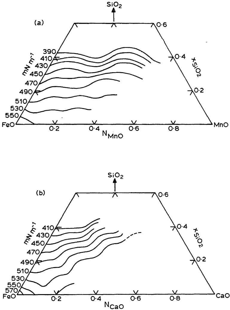
Fig. 5.32 Isosurface tension curves in FeO–MnO–SiO<sub>2</sub> and FeO–CaO–SiO<sub>2</sub> melts saturated with iron at 1400°C.
