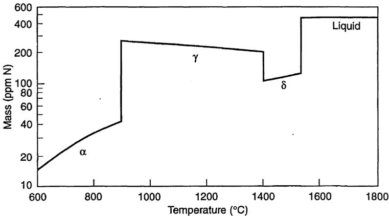
Fig. 4.6 Solubility of nitrogen in pure iron (or low-alloy steels) at 1 atm pressure of N<sub>2</sub>.
