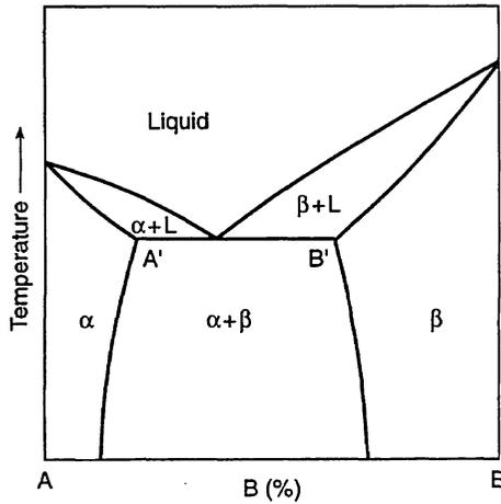
Fig. 1.10 Binary eutectic systems with partial solid solubilities.
