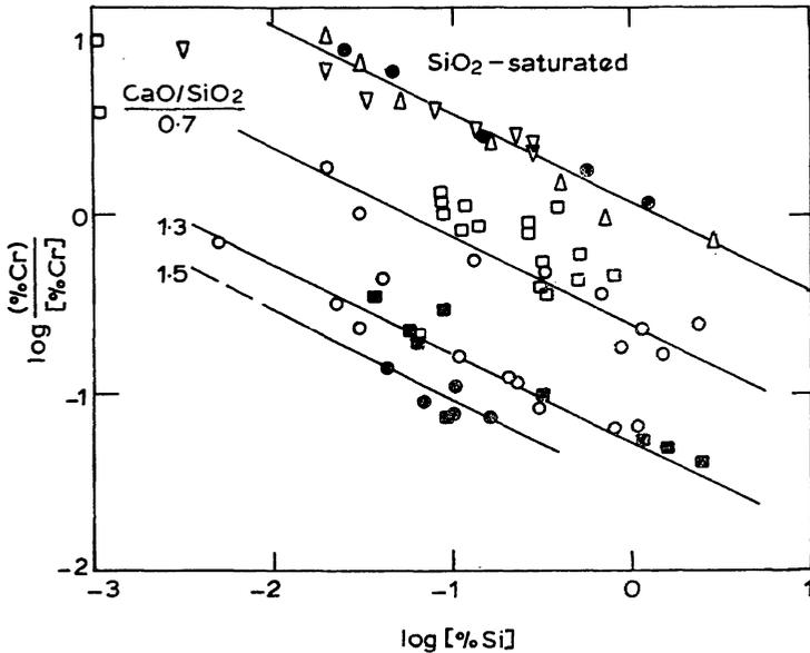
Fig. 6.5 Equilibrium slag/metal chromium distribution varying with the concentration of silicon in iron coexisting with chromium oxide containing CaO–Al<sub>2</sub>O<sub>3</sub>–SiO<sub>2</sub> slags at temperatures of 1600° to 1690°C. See Ref. 5 for references to experimental data.
