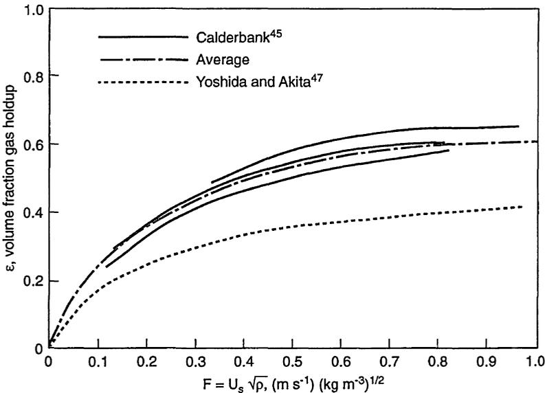
Fig. 2.29 Experimental data of Calderbank<sup>45</sup> on gas holdup in sieve plate columns for the air-water system are compared with those of Yoshida and Akita<sup>47</sup>.
