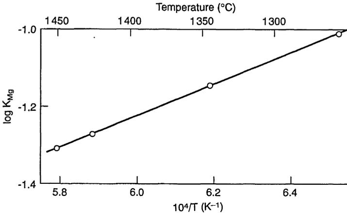
Fig. 4.29 Temperature dependence of the equilibrium constant for the solubility of Mg in liquid iron (undercooled), %Mg atm<sup>-1</sup>.
