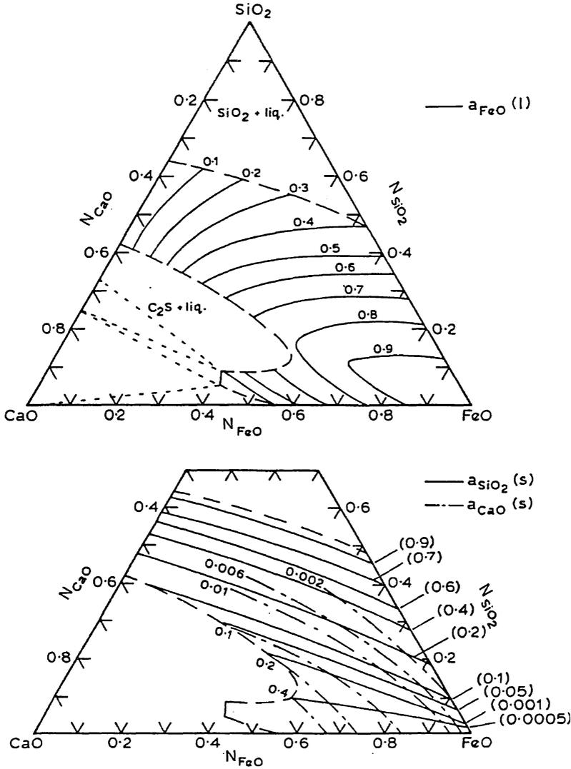
Fig. 5.18 Activities of FeO(l) (experimental), CaO(s) and SiO<sub>2</sub>(s) (by Gibbs-Duhem integration) in CaO-FeO-SiO<sub>2</sub> melts in equilibrium with liquid iron at 1550°C. From Refs. 11, 12.
