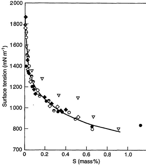
Fig. 4.34 Surface tension of Fe-S alloys at 1550–1600°C.
