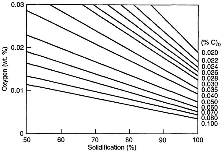
Fig. 10.3 Equilibrium oxygen content of steel, for carbon–oxygen reaction at 1 atm. CO at various stages of solidification for several initial carbon concentrations. From Ref. 6.
