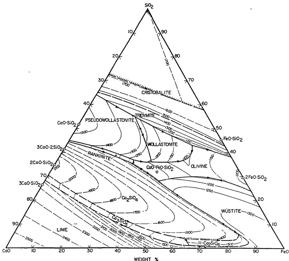
Fig. 5.10 Liquidus isotherms of CaO-SiO<sub>2</sub>-FeO system.
