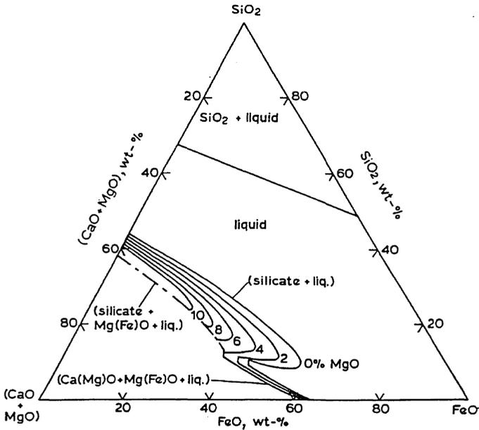
Fig. 5.12 Effect of MgO (wt.%) on the solubility isotherms at 1600°C in the system (CaO + MgO)-SiO<sub>2</sub>-FeO in equilibrium with liquid iron.
