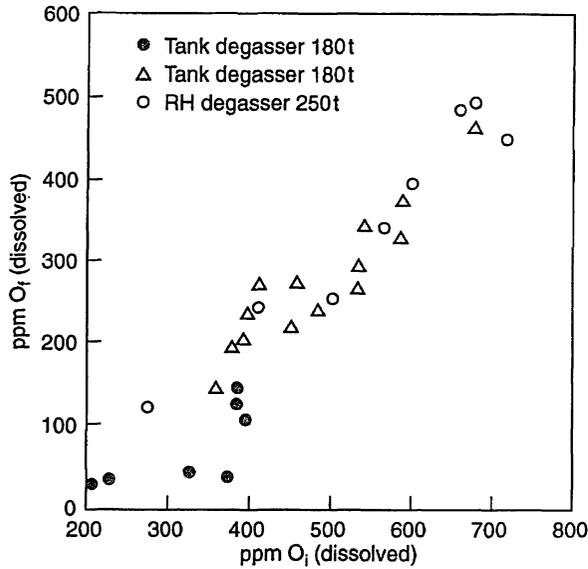
Fig. 9.34 Oxygen contents of steel before and after vacuum decarburisation. Points ● Δ ○. Ref. 13 17 18.
