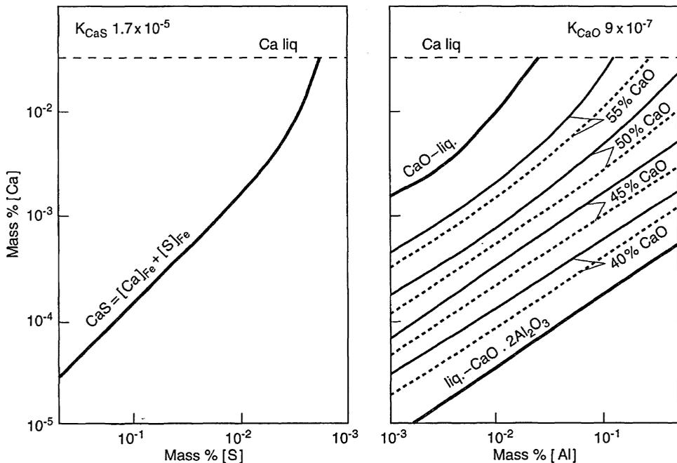
Fig. 9.42 Computed equilibrium diagram for Fe–Al–Ca–O–S system at 1600°C; (---) curves for aluminates containing 5% SiO<sub>2</sub>. From Ref. 34.
