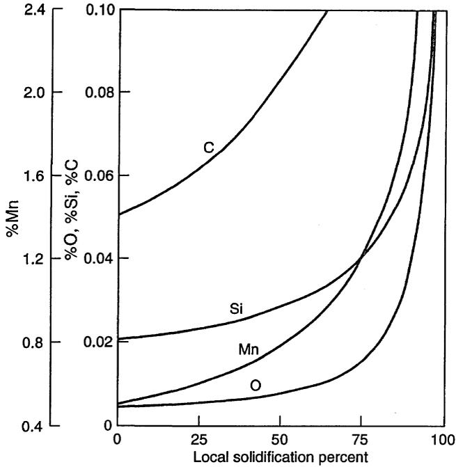
Fig. 10.1 Interdentritic solute enrichment, if no reaction occurs between them during solidification of the steel.
