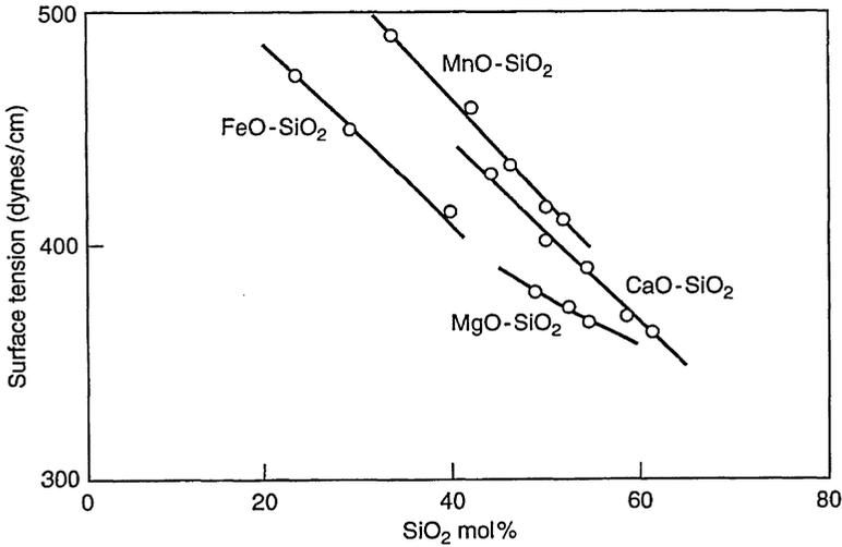
Fig. 5.30 . Surface tensions of binary silicate melts:  $FeO-SiO_2$  at 1420°C, other silicates at 1570°C. From Ref. 26.
