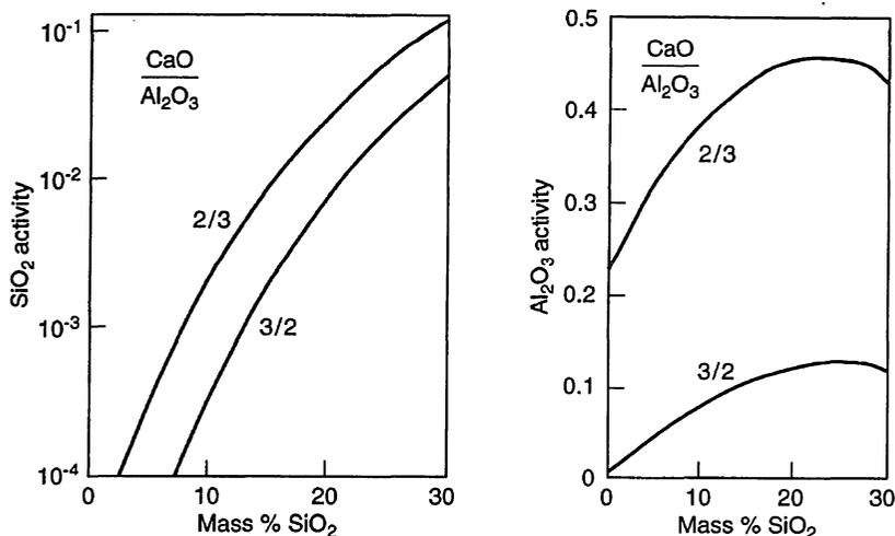
Fig. 5.19 Silica and alumina activities, with respect to solid oxides, in CaO–Al<sub>2</sub>O<sub>3</sub>–SiO<sub>2</sub> melts at 1600°C, derived from experimental data of Rein and Chipman.<sup>13</sup>
