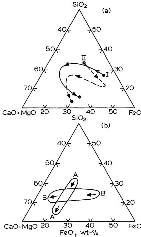
Fig. 8.5 Changes in composition of slag during oxygen blowing for various BOF practices: (a) I, van Hoorn *et al.*<sup>2</sup> and II, Bardenheurer *et al.*<sup>3</sup> (b) AA, Nilles *et al.*<sup>4</sup> and BB, Baker<sup>5</sup>.
