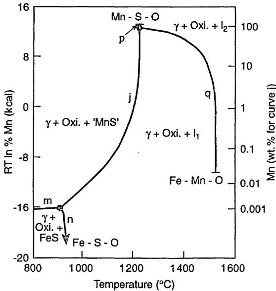
Fig. 4.25 Univariant equilibria in Fe-Mn-S-O system in the presence of  $\gamma$ -Fe and Mn(Fe)O phases. From Ref. 25.
