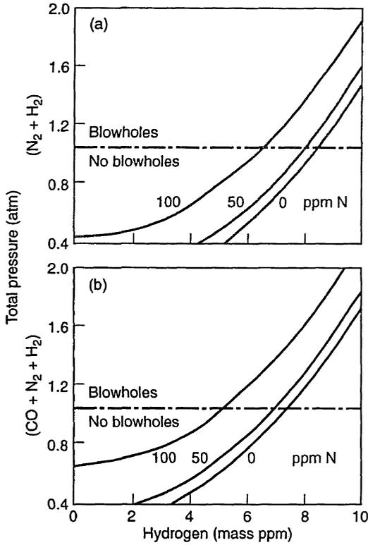
Fig. 10.7 Total gas pressure at 90% local solidification. (a) Al-killed steel containing  $< 0.1\%$  C (b) Semi-killed steel containing: (i) 1.5% Mn, 0.2% Si, 0.08% C, 10 ppm O (ii) 0.5% Mn, 0.03% Si, 0.02% C, 40 ppm O.
