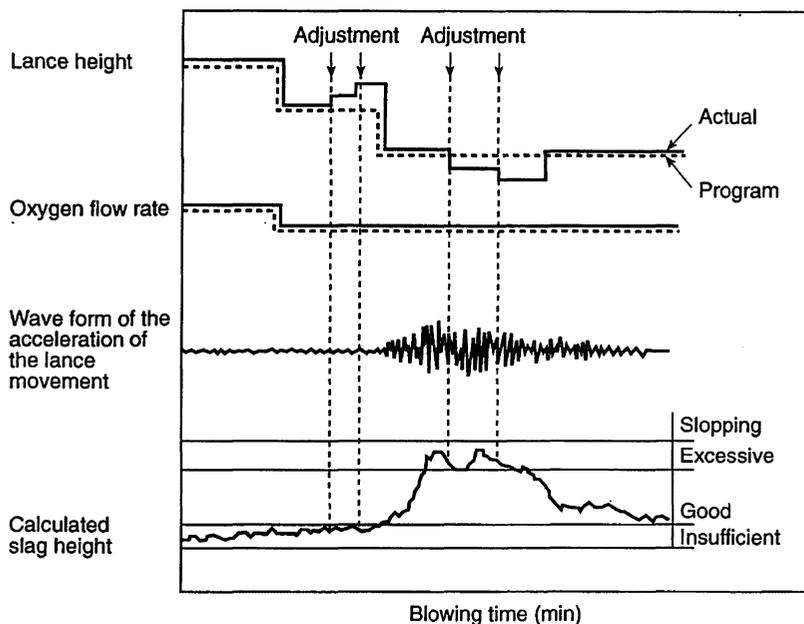
Fig. 8.15 Example of automatic blowing control. From Ref. 1.
