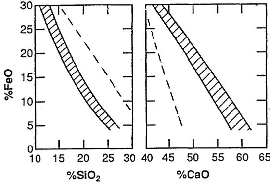
Fig. 8.6 The total iron oxide (as FeO) content of steelmaking slags is related to the SiO<sub>2</sub> and CaO contents. The dotted line is for CaO-6%MgO-FeO-SiO<sub>2</sub> system saturated with dicalcium (magnesium) silicate.
