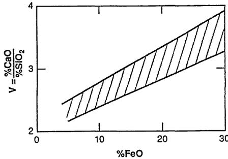
Fig. 8.7 Variation of slag basicity with total iron oxide content of steelmaking slags containing P<sub>2</sub>O<sub>5</sub> < 3%.
