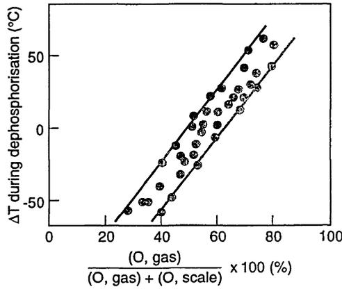
Fig. 7.6 Relation between the gaseous oxygen ratio and  $\Delta T$  during dephosphorisation.
