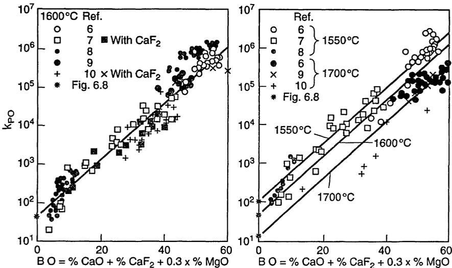
Fig. 6.7 Equilibrium data showing the decisive effects of CaO, CaF<sub>2</sub> and MgO on phosphate capacities of simple and complex slags.
