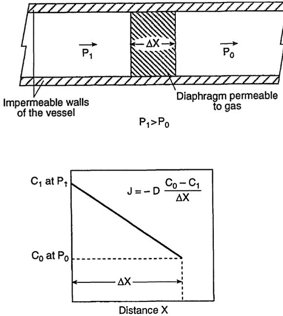
Fig. 2.4 Illustration of steady state diffusion.
