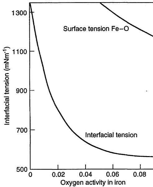
Fig. 5.34 Effect of oxygen in iron on the interfacial tension between liquid iron and CaO-Al<sub>2</sub>O<sub>3</sub>-SiO<sub>2</sub> melts, determined by Gaye *et al.*<sup>30</sup> is compared to the surface tension of Fe-O melt at 1600°C.
