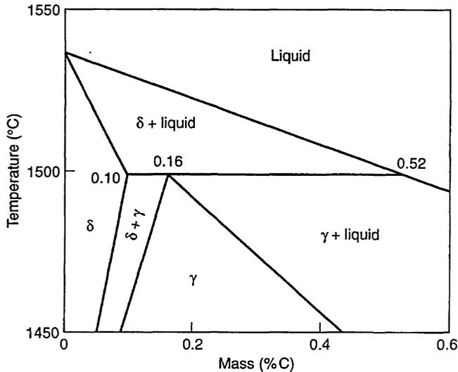
Fig. 4.11 Peritectic region of binary iron–carbon system.
