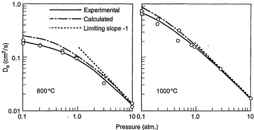
Fig. 3.5 Pressure dependence of effective diffusivity He-CO<sub>2</sub> at 20°C in iron reduced from haematite ore in hydrogen at indicated temperature.
