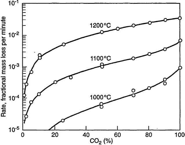
Fig. 2.12 Effects of temperature and gas composition on the rate of oxidation of electrode graphite granules ( $\sim 0.5$  mm dia.) in CO<sub>2</sub>-CO mixtures at 0.96 atm total pressure. From Ref. 28.
