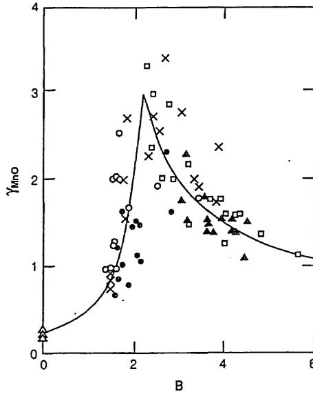
Fig. 5.24 Effect of slag basicity on the activity coefficient of manganese oxide in simple and complex slags at 1600°C.
