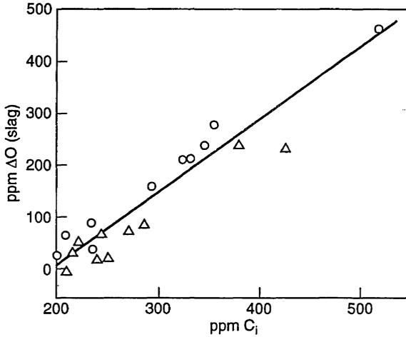
Fig. 9.35 Oxygen pickup from ladle slag during decarburisation in (Δ) tank degasser and (O) R H degasser.
