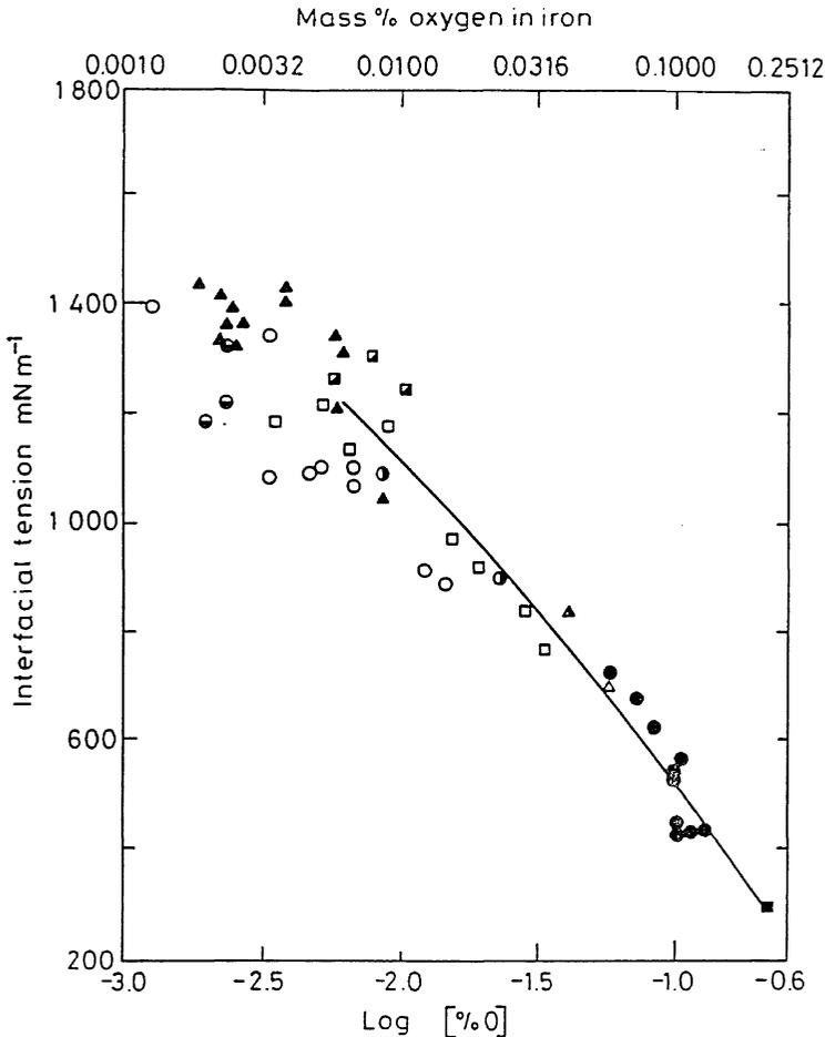
Fig. 5.35 General relation between the oxygen content of iron and the interfacial tension between the metal and various slag systems at 1580°C. From Ref. 31.
