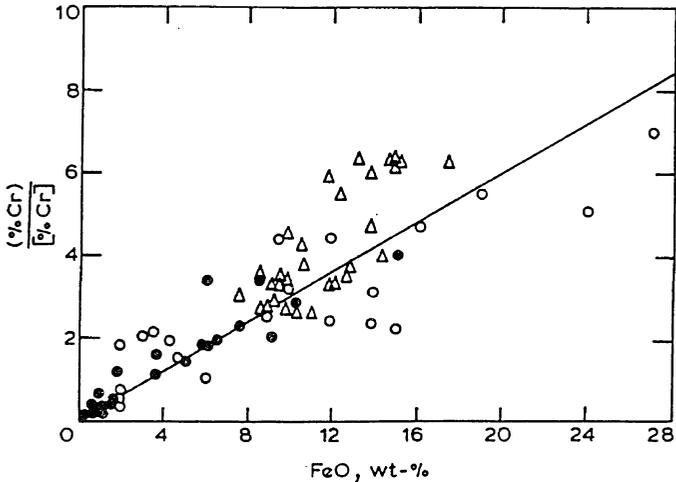
Fig. 6.3 Variation of chromium distribution ratio with the iron oxide content of slag, in the (Δ) open hearth<sup>1</sup> and (○) electric arc furnace<sup>3</sup> at tap is compared with the results of laboratory experiments<sup>2</sup> (●).
