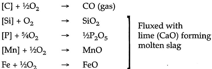
At the end of oxygen blowing the slag basicity (as  $V = \% \text{CaO} / \% \text{SiO}_2$ ) is in the range 2.5 to 4.0, with iron oxide contents of 10 to 35% FeO depending on the aimed carbon, sulphur and phosphorus contents of the steel at tap. From trial and error calculations the following formulation has emerged for the quantities of burnt lime and burnt dolomite to be charged, depending on the total silicon content of the furnace charge.
