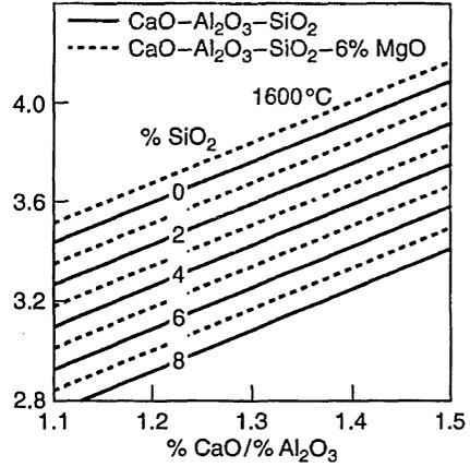
Fig. 6.11 Effects of temperature and composition of calcium aluminate melts on the equilibrium constant  $K_{SA} = \frac{(\%S)}{[\%S]} [\%Al]^{-2/3}$ .
