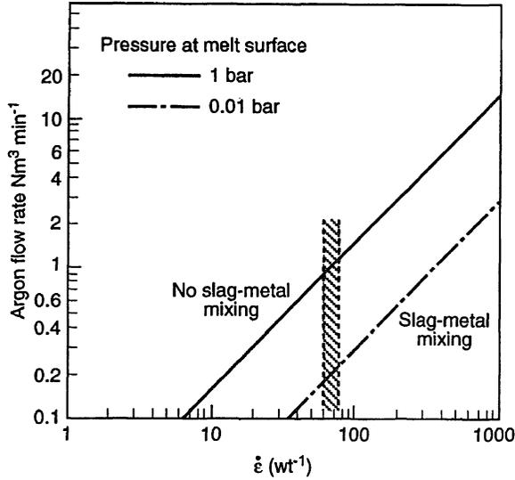
Fig. 9.27 Density of power of stirring by gas injection at 3m below the surface of a 200 t melt.
