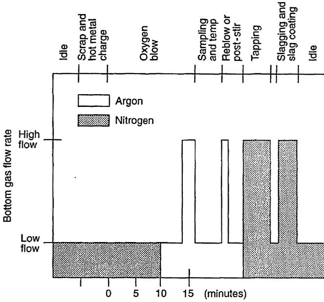
Fig. 8.10 Bottom-stirring practice for low-carbon heats (< 0.10%C).
