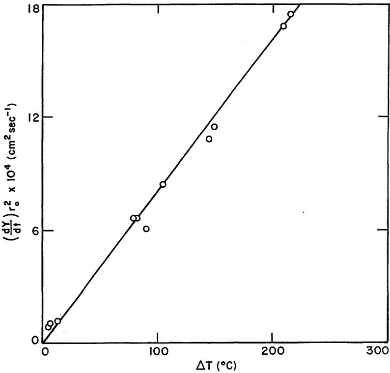
Fig. 2.9 Variation of the rate of calcination,  $(dY/dt)r_c^2$ , with the temperature difference across the calcinated layer. From Ref. 20.
