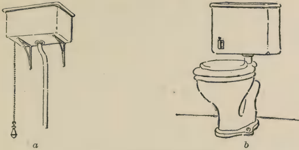
FIG. 57. FLUSHING TANKS. a , Ordinary Style; b , Low Down Style.
