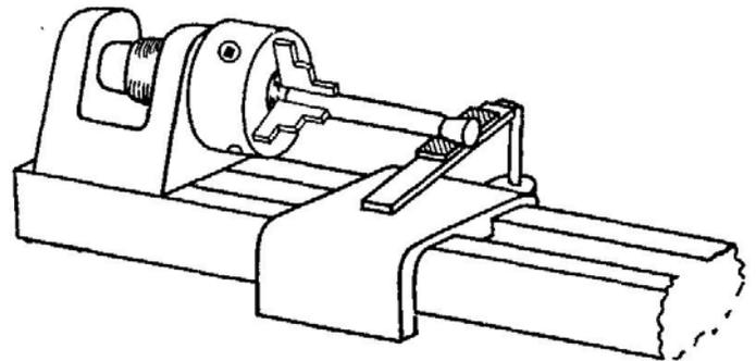
FIG. 11.5. Socket forming with a paddle fitted to a lathe.
