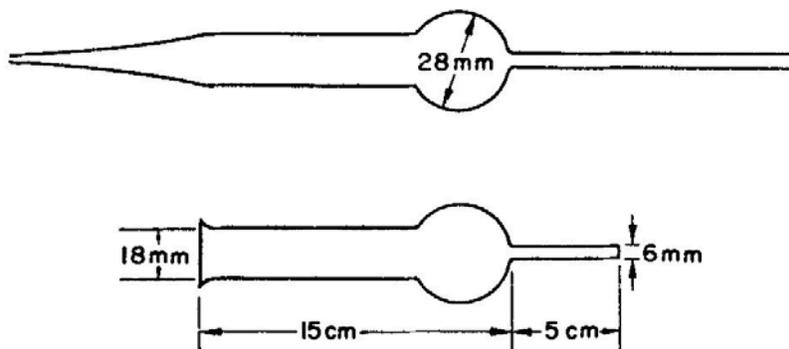
FIG. 8.7. A calcium chloride tube, showing the stages and suitable dimensions for its preparation.
