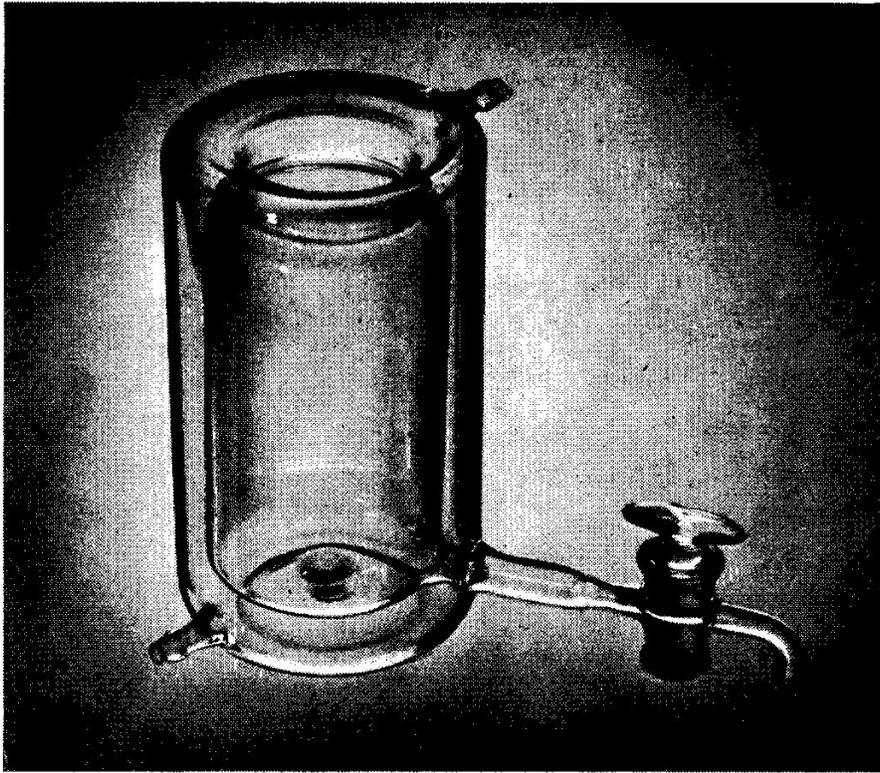
PLATE 9.1. A jacketed beaker. Made in the lathe.
