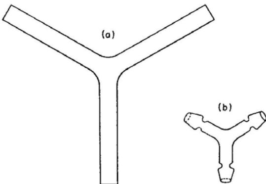
FIG 6.30. Y-pieces: (a) Shows the proportions and shape for practice work. A strong and compact form is shown in (b).
