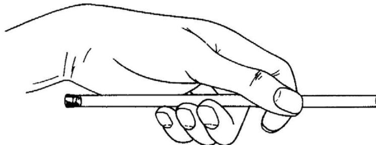
FIG. 6.10. Tubing ready for rotation in the left hand. Note the positions of the fingers and thumb.
