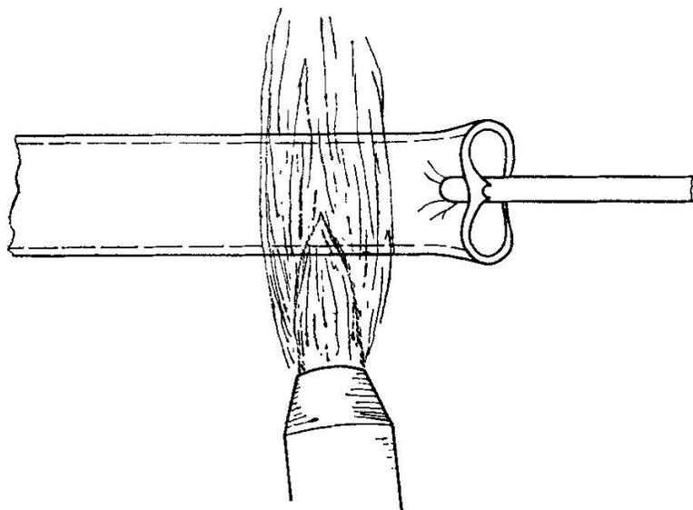
FIG. 6.18. The attachment of the rod handle to the plastic tube end.
