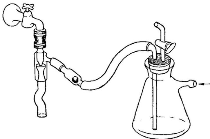
FIG. 10.3. A water-jet pump fitted with safety devices.
