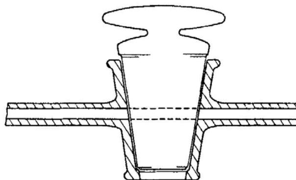
FIG. 11.12. The effect of wear on an imperfect stopcock. The shoulders on the key and barrel prevent the ground surfaces from making good contact with one another, and cause the stopcock to leak.
