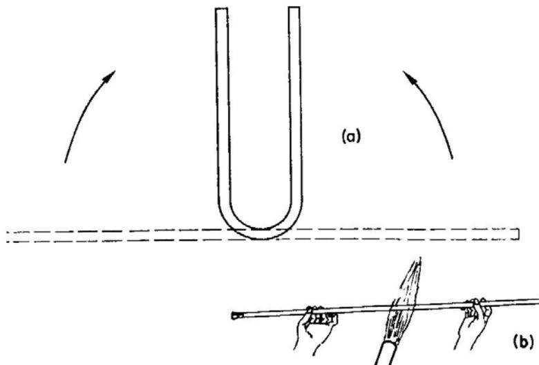
FIG. 6.21. Bending rod and tubing. (a) The heated rod is bent upwards in a vertical plane. (b) Hand position for heating rod and tubing as a preliminary to bending.
