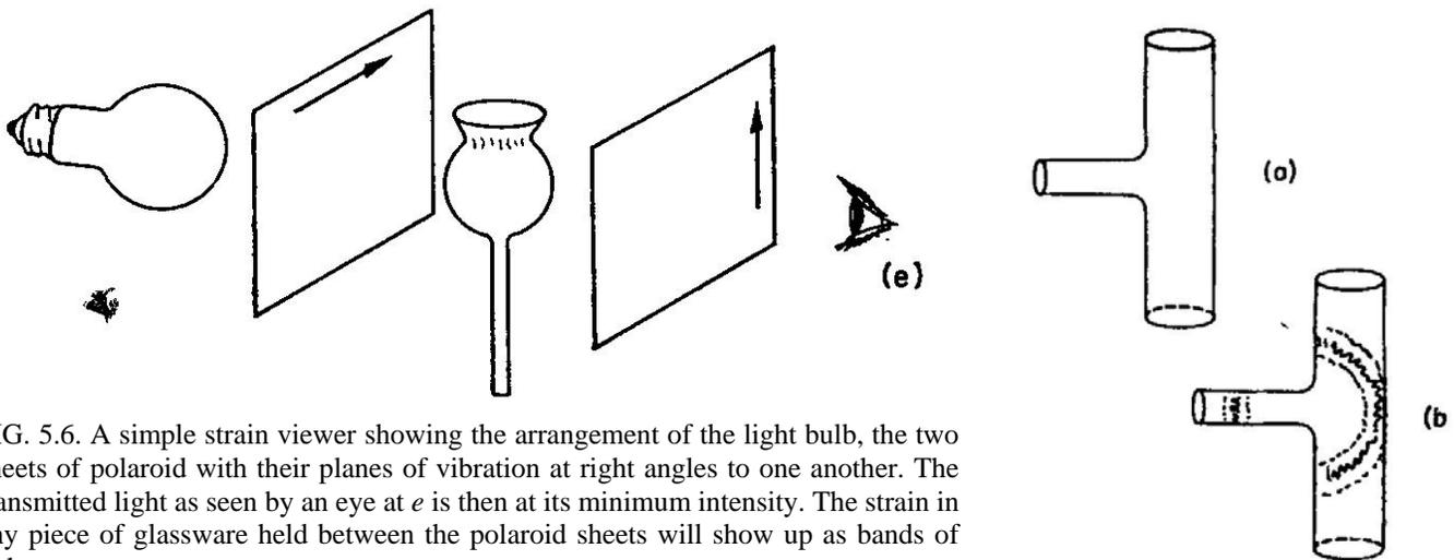
FIG. 5.6. A simple strain viewer showing the arrangement of the light bulb, the two sheets of polaroid with their planes of vibration at right angles to one another. The transmitted light as seen by an eye at *e* is then at its minimum intensity. The strain in any piece of glassware held between the polaroid sheets will show up as bands of light.
