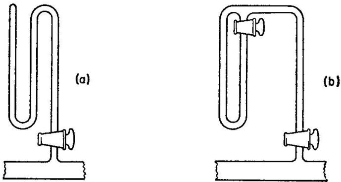
FIG. 10.11. (Up) Two closed limb manometers.
