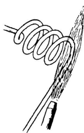
FIG. 8.14. Making a free-hand spiral coil. The glass must be moved and turned in the flame so that the tube is heated all round its circumference.
