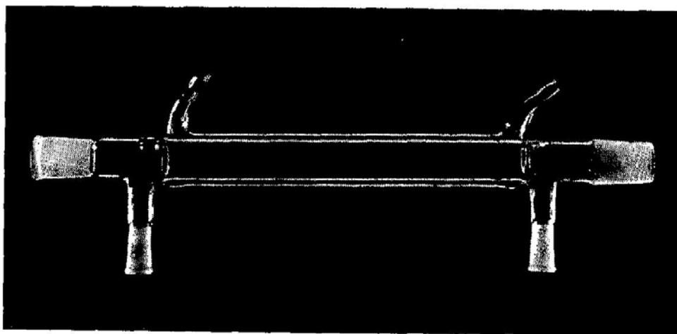
PLATE 11.1. An example of experimental glassware fitted with interchangeable ground-glass joints.
