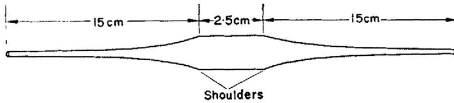
FIG. 6.19. Double points, showing the shoulders. Both points should be concentric with the tube.
