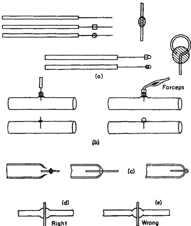
FIG. 7.1. (a) Beading a platinum wire into lead glass. The wire may be straight or bent into a circle. (b) Sealing the beaded wire into a hole in the side of a glass tube. (c) Sealing a beaded wire into the end of a glass tube. (d) An enlarged view of the glass wall showing no great variation in wall-thickness in the vicinity of the platinum wire. (e) An enlarged view showing variations in wall thickness likely to cause cracks.
