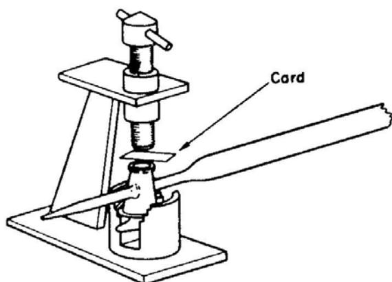
FIG. 8.1. A tool used to remove stopcock keys.
