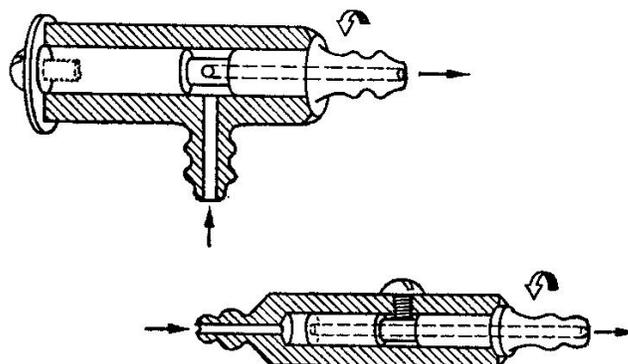
FIG 4.12. Blowing swivels. These swivels are necessary when glass must be blown in the lathe. They are also used to blow into glass worked at the bench burner if there is no convenient end for mouth blowing.
