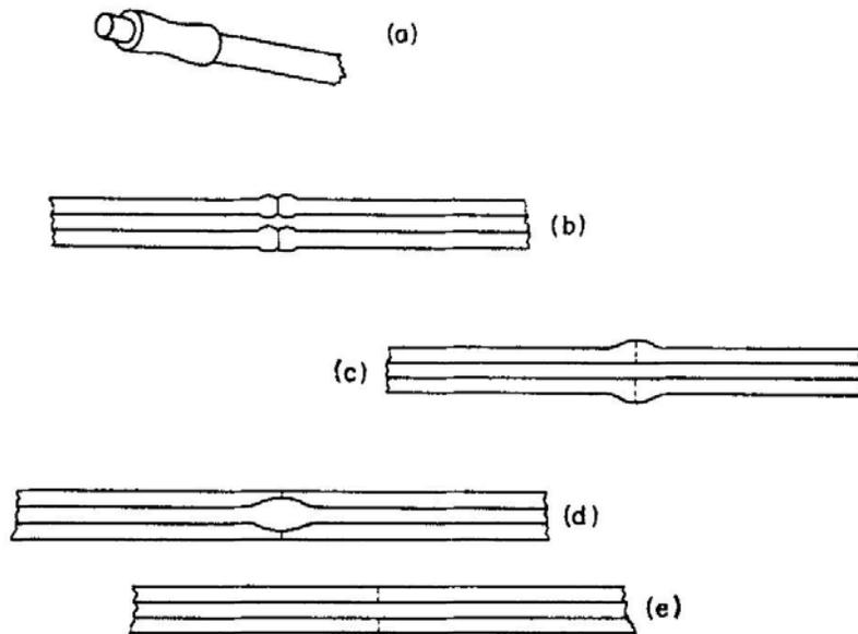
FIG. 6.27. Joining capillary tube of 2 mm bore or more. Note the stoppered rubber tube plug (a). (b) Shows the capillary tubes immediately after they have been brought together and just before they have been very slightly pulled apart. At (c) the glass is ready to blow and pull into a uniform tube (e). (d) Shows the result of excessive blowing.
