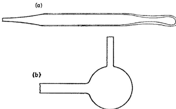
FIG. 6.39. Blowing a bulb on the end of a tube. First prepare a test-tube end on a suitable piece of tubing and mark the required length on the tube. (a) Shows the glass heated and gathered, ready to blow up. (b) The blown bulb with a side tube attached. Such a shape is difficult to preserve if the bulb is thin-walled.
