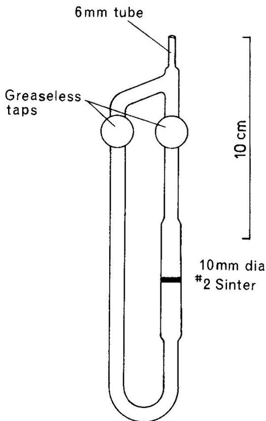
FIG. A.6. Another H<sub>2</sub>O separator, this type is detachable.
