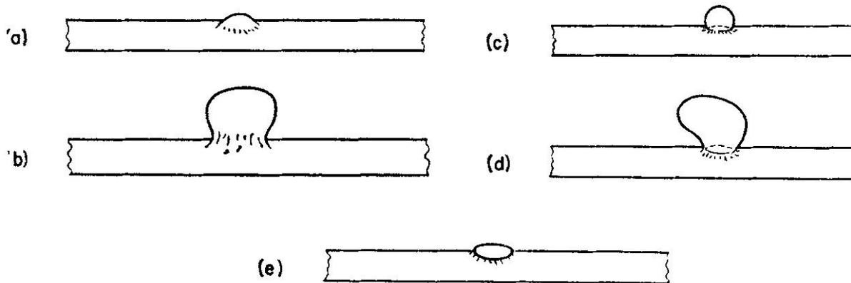
FIG. 6.29a. Making a T-join. The diagrams should be studied when reading the text. Special attention should be given to blowing the hole in the cross-piece; if too much glass is heated and a large blister blown up (b), the T-join will be unnecessarily difficult to make.
