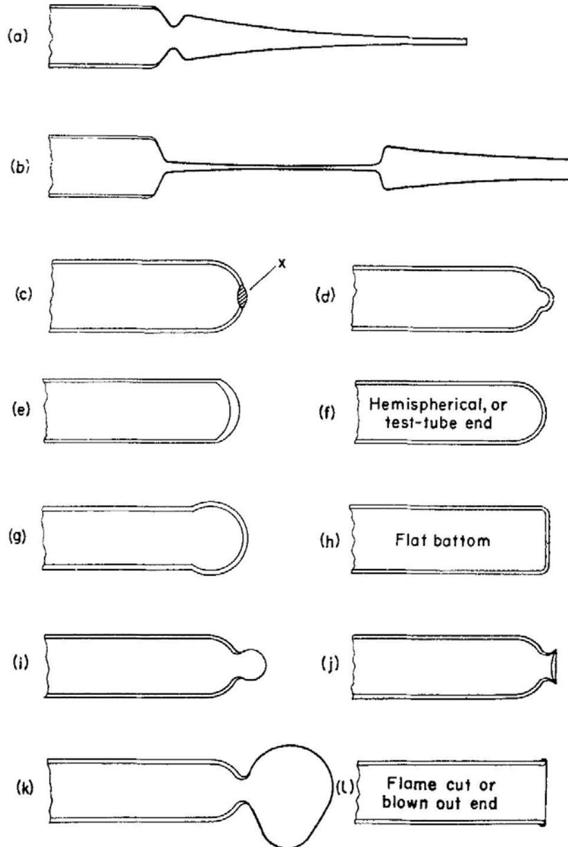
FIG. 6.20. The steps required to make test-tube ends, flat-bottomed ends and blown-out ends.
