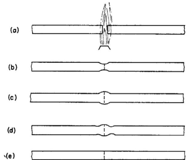
FIG. 6.25. Some other faults in short-radius bends.
