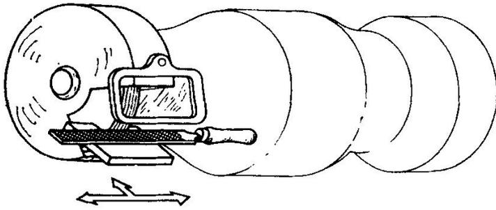
FIG. 4.1. Renewing the edges on a glass-cutting file. A small thickness of metal is ground off the narrow faces with an engineer's grindstone.
