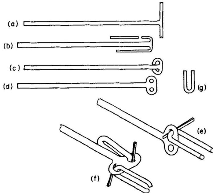
FIG. 8.6. Link stirrers. (a) A T-joint made with rod. (b) The ends bent round and melted off. (c) The ends bent further, ready to join to the rod shaft. (d) Shows the completed shaft end. (e) The first link, wedged in place with a matchstick. (f) Shows the first link completed and wedged so that it will be clear of the flame. The second link is wedged in place and its ends bent round ready to be joined. (g) A link of bent rod, ready to be wedged in the shaft end.
