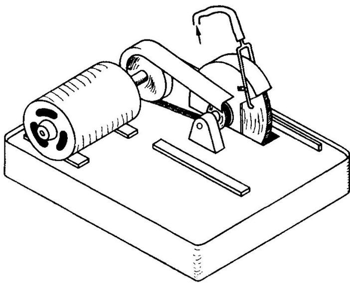
FIG. 4.7. Glass-cutting machine fitted with thin rubber-bonded carborundum disc. Water cooled. The previously marked tube is pressed gently against the cutting edge and rotated until the cut penetrates the glass wall all round.
