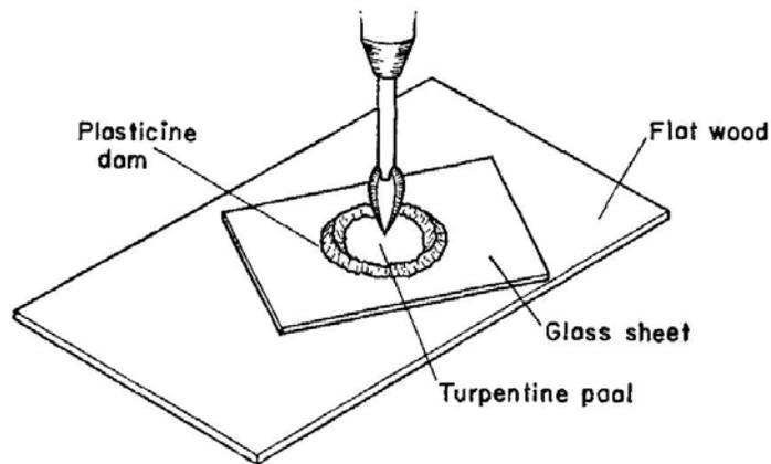
FIG. 6.6. Cutting a hole in a sheet glass.
