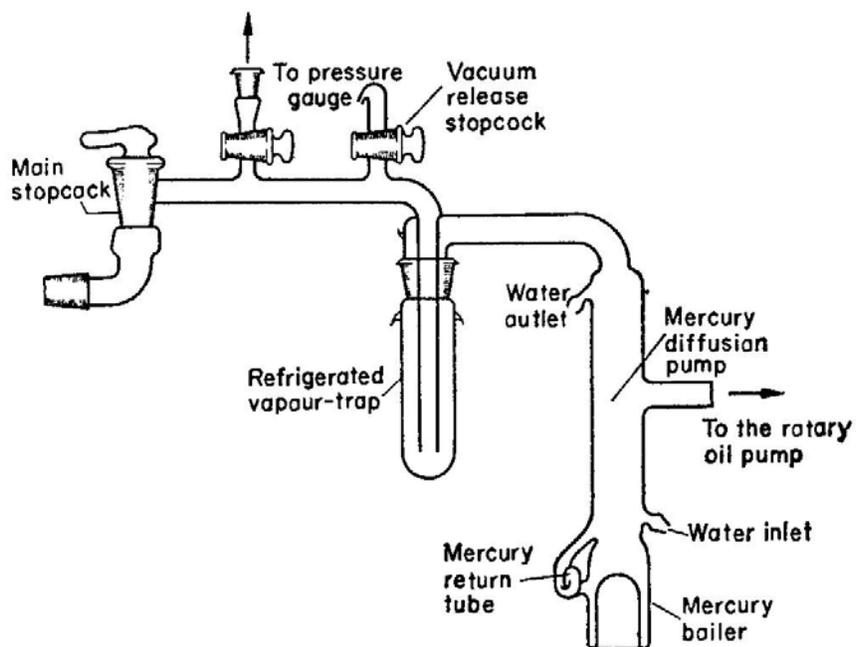
FIG. 10.6. A simple high vacuum system. The diffusion pump is connected to the rotary oil pump through the oil reservoir. The apparatus to be evacuated is attached to the standard joint below the main stopcock.
