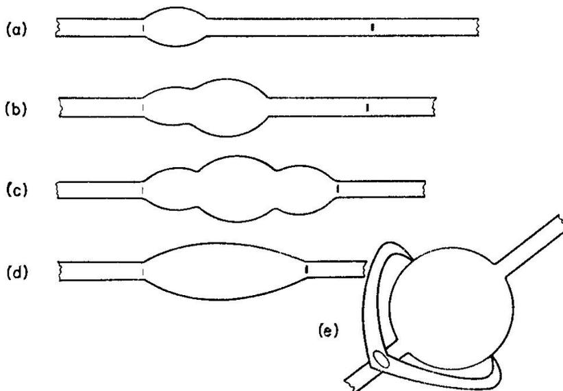
FIG. 6.38. Large bulbs. The glass is gathered up by blowing a succession of small bulbs as shown in (a), (b) and (c). The wall-thickness of these small bulbs should not be less than that of the tube. (d) All the glass between the marks is then gathered in to a smooth mass of nearly uniform wall-thickness and free from constrictions. (e) The bulb is blown up and measured with calipers. Some care is necessary to avoid making the bulb too large.
