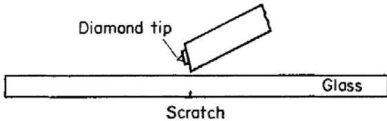
FIG. 6.4. Starting a crack in plate glass. It is essential to make a good deep mark with a sharp tool. The glass is inverted and tapped with the metal edge of the tool directly opposite the mark.
