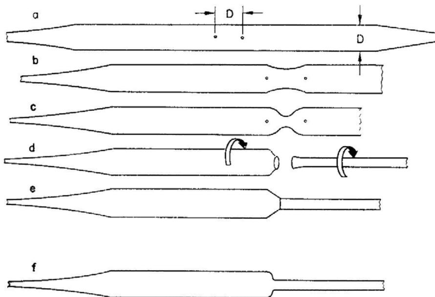
FIG. 6.32. Another method of joining tubes of different diameter: (a) shows the larger tube marked ready to be constricted; (b) the first step in making the constriction; (c) the finished constriction; (d) the tube ends ready to join together; (e) the shape of the joint before blowing up; (f) the completed join.
