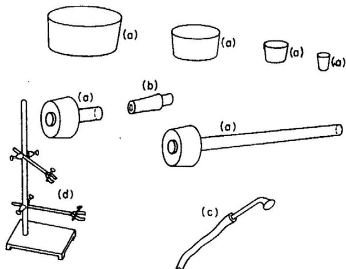
FIG 4.15. Bench-top accessories: (a) cork stoppers with and without blowing tubes and handles; (b) rubber tube plug, or policeman; (c) rubber blow-tube with plain mouthpiece; (d) laboratory stand with two clamps.
