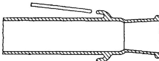
FIG. 11.13. Hooks on ground glass joints permit a pair of joints to be held together with springs or elastic bands. Reentrant angles at the base of the hooks are undesirable and the result of insufficient melting of the glass.
