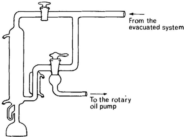
FIG. 10.7. Stopcock arrangement for by-passing a diffusion pump. Such an arrangement allows the rotary oil pump to recover the low pressure required before the diffusion pump can operate and eliminates the need to discontinue the supply of heat to the pump boiler. The diffusion pump can be made to function again by opening the stopcock and turning stopcock handle through 180°.
