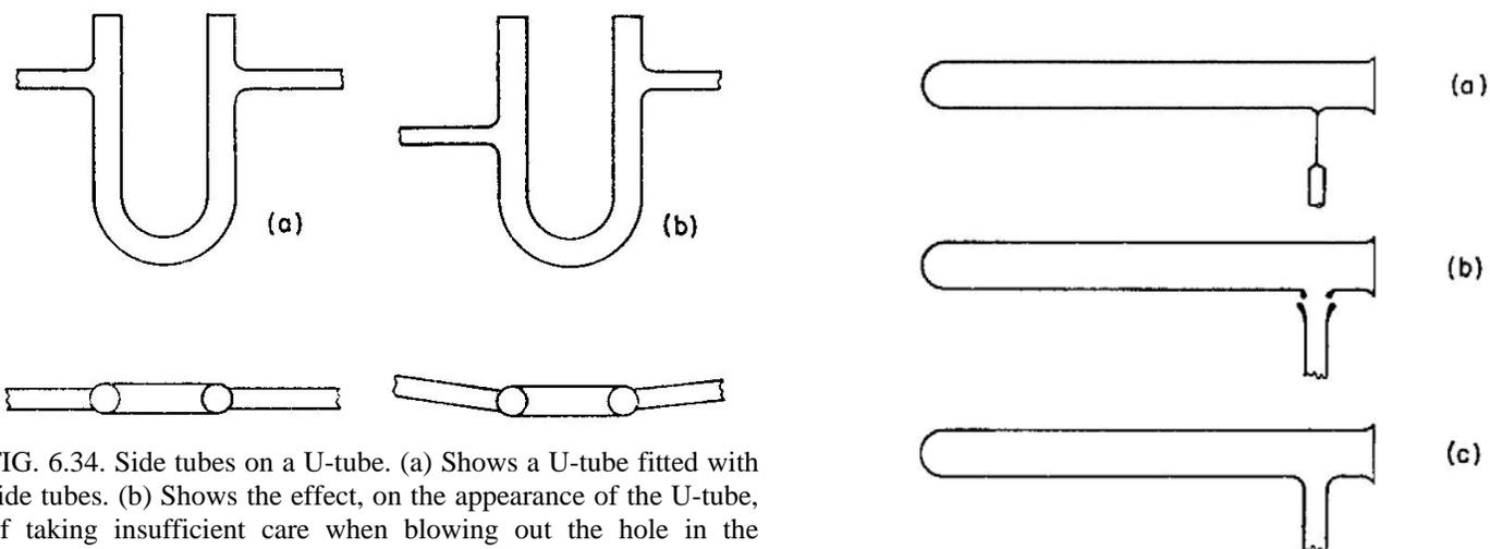
FIG. 6.34. Side tubes on a U-tube. (a) Shows a U-tube fitted with side tubes. (b) Shows the effect, on the appearance of the U-tube, of taking insufficient care when blowing out the hole in the second limb; the side tubes are not in line.
