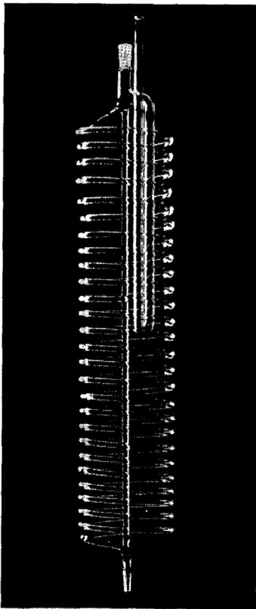
PLATE 8.1. A 610 cm (20 ft) spiral coil for gas chromatography. This coil was made, in five sections, on an asbestos-covered glass tube. The sections were joined together with a hand lamp.
