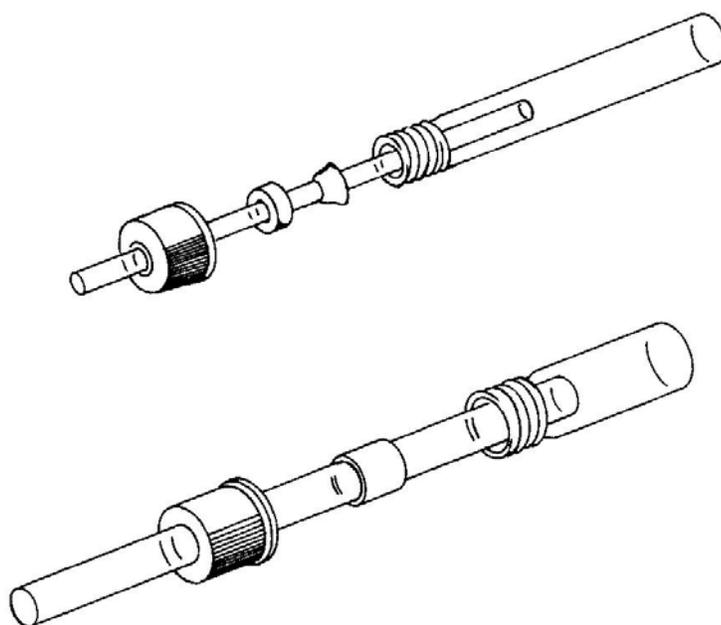
FIG. A.4. Two types of screw-thread connectors.
