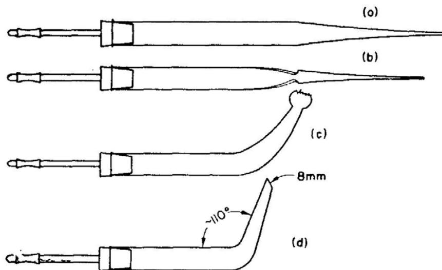
FIG. 8.12. The essential stages in making a condenser adaptor. (a) The prepared tube fitted with an asbestos stopper and plugged tube handle. (b) Shows the glass constricted and gathered. (c) The first stage of bending, pulling and blowing. (d) Finished adaptor. The small end is cut off with a rubber-bonded cutting wheel.
