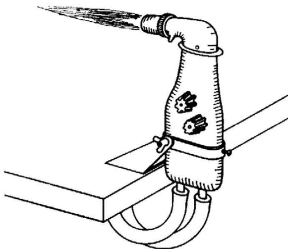
FIG. 4.18. A Flamemaster handlamp with bench clamp.
