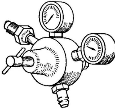
FIG. 4.19. A pressure regulator with two gauges.
