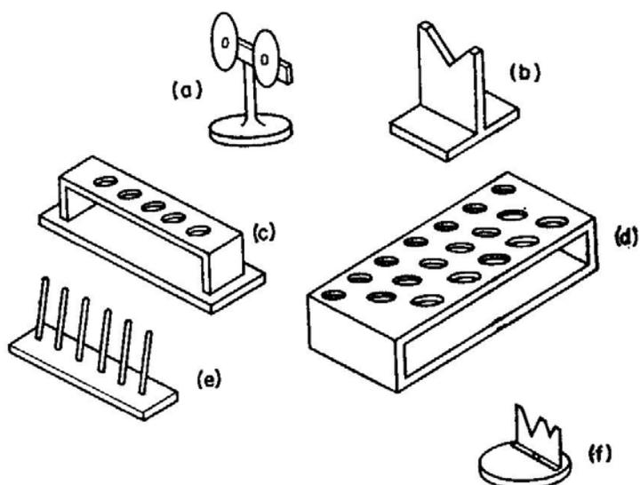
FIG. 4.14. Bench-top accessories: (a) and (b) are used to support long lengths of tubing; (c), (d) and (e) are typical cooling racks made from wood; (f) is a useful cutting aid. Small diameter tubes or capillary tubes, or rods are marked with the knife and placed in a notch so that the mark is directly above the edges; a sharp blow with the back of the knife will cause the glass to break off cleanly at the mark.
