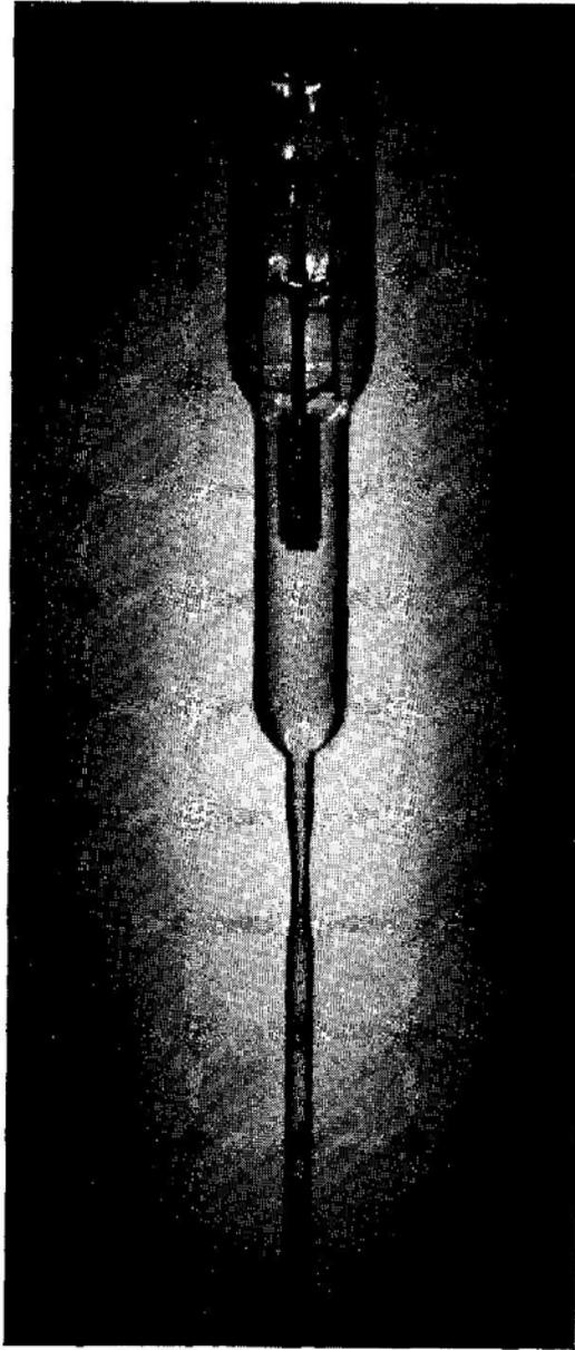
PLATE 7.1. An experimental gas discharge tube electrode. Tungsten wires sealed through Pyrex glass.
