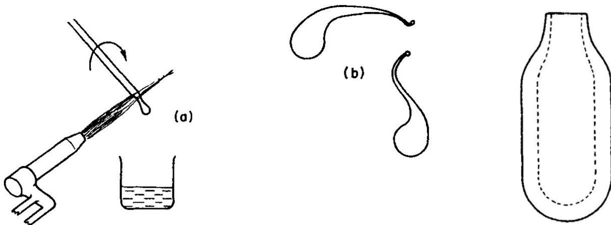
FIG. 5.4. Prince Rupert's drops. (a) Shows the heated glass about to drop into a beaker of water. Typical shapes for these drops are shown in (b).
