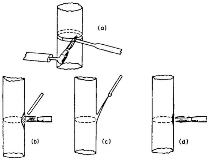
FIG. 8.19. I-handlamp joint using rod fill. (a) The rod being fed into the space between the previously heated tube ends. (b) and (c) Removing a thick spot from join. (d) Remelting the spot to recover the shape.
