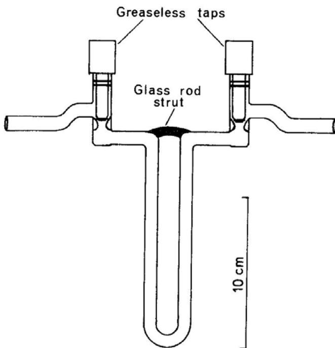
FIG. A.8. A U-tube for collecting condensable gases. Note that the lower limbs of the taps are connected to the U-tube so that potential leaks into the condensed gases are minimized.
