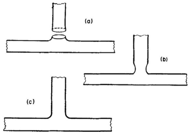
FIG. 8.20. T-join made with the handlamp. (a) Shows the side-arm and the cross-piece ready to be joined. (b) The joint pulled up immediately after it is first made. (c) The finished join; the glass has been freed from irregularities in wall-thickness and diameter.
