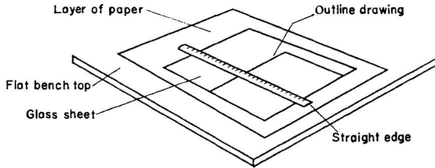
FIG. 6.1. Cutting glass sheet to an outline drawing.
