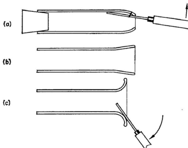
FIG. 6.12. (Right) Flaring and flanging tube ends. (a) The tool is moved away from the tube centre-line to flare the plastic glass. (b) Finished flared end. (c) A flanged end, made by taking the methods of (a) a step farther.
