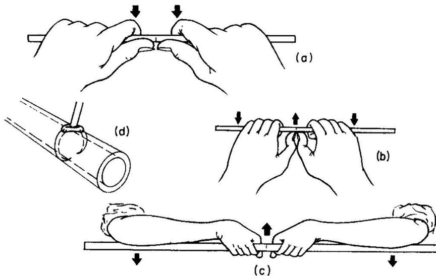
FIG. 6.9. Hand positions for breaking tubing and rod. (a) A method of breaking small diameters glass tubing. (b) A method of breaking rod. (c) Hand and forearm action for breaking large tubes. (d) Applying hot glass to knife mark.
