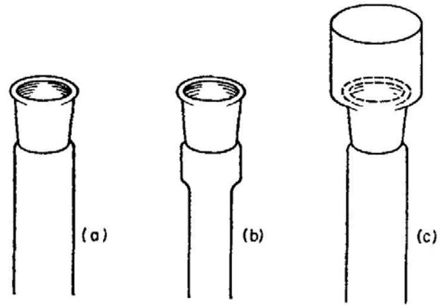
FIG. 11.3. Types of sockets. (a) Plain tube socket. (b) Socket with attached tube of similar diameter to that of the corresponding cone. (c) Cup socket.
