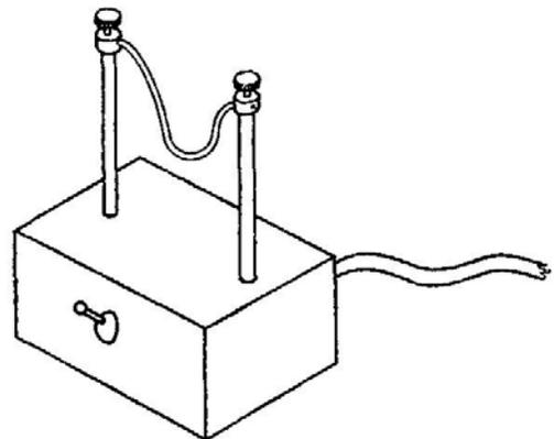
FIG. 4.6. Electrically heated wire. The hot wire is used to cut straight ends in the same way as the iron wire hooks. The wire easily adjusts itself to fit any tube diameter.
