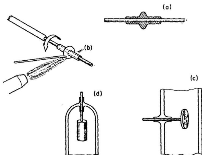
FIG. 7.4. Seals made with tungsten wire and borosilicate glass. (a) A prepared wire with sleeves and button. (b) Building up the button with thin rod. (c) and (d) show two electrodes with this type of seal.
