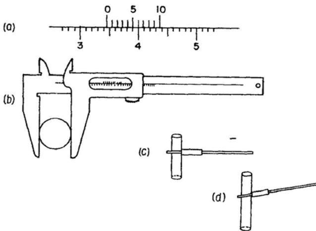
FIG. 2.1. (Left) (a) Vernier scale set at a reading 3.45 cm. (b) A typical Vernier caliper gauge. (c) Shows the correct angle for accurate measurement of tube diameters. (d) An incorrect angle, which will result in errors of measurement.
