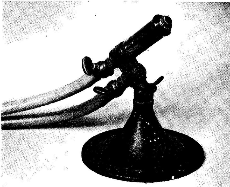
PLATE 4.1. An orifice-mixing bench burner with interchangeable air jets.
