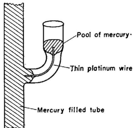
FIG. 7.2. A thin platinum wire sealed into a borosilicate tube to make contact with mercury at both ends of the wire.
