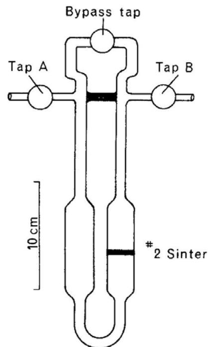
FIG. A.5. An H<sub>2</sub>O separator with a No. 2, 10 mm diameter sintered disc. The U-tube and the sintered disc must be immersed in LN before the gas mixture is admitted to the separator.
