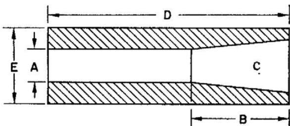
FIG. 11.8. A cone-grinding tool. *A*, the diameter of the small end of the ground zone  $-0.25\text{mm}$ . *B*, the length of the ground zone  $+2\text{mm}$ . *C*, standard taper of 1 in 10 in the diameter. *D*, about 15 cm to allow for remachining. *E*, any convenient diameter which allows an adequate thickness of metal.
