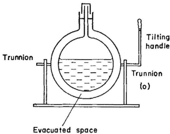
FIG. 10.9. A LN dispenser (a) mounted on a stand and capable of being tilted to fill small capacity Dewar flasks. This type of dispenser has a capacity of about 50 l., and is made of metal. A Dewar flask (b). This is a double-walled glass vessel, the inner space is evacuated and its glass surfaces are coated with silver. Capacity range up to 1.5 l.
