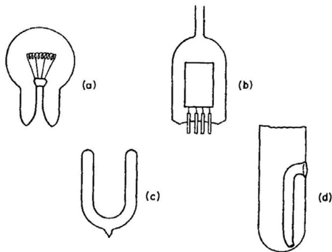
FIG. 6.43. Ring seals in (a) an electric lamp, (b) a radio valve, (c) a Dewar flask, and (d) part of a steam distillation apparatus.
