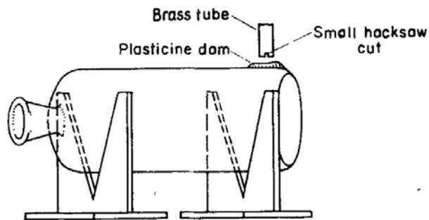
FIG. 6.7. Cutting a hole in a bottle. The small cut in the brass tube helps to retain carborundum grit.
