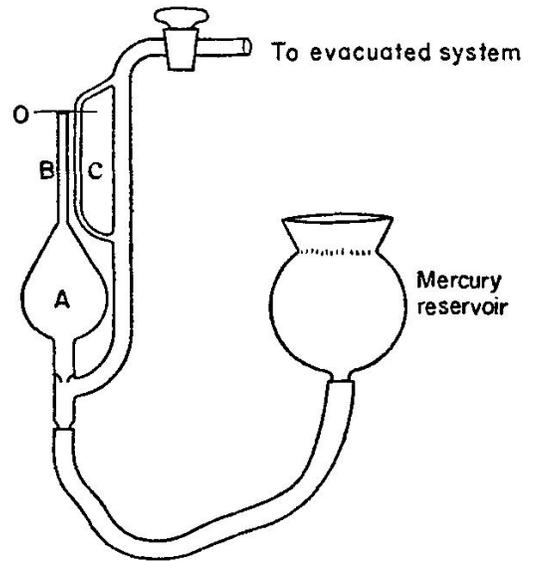
FIG. 10.12. (Right) A McLeod gauge. The gauge head and reservoir are made of glass. The range of pressure that can be measured depends on the volume of bulb A, and the bore and length of the capillary tube B. Capillary tubes B and C are made from tubing of identical bore to eliminate the need for capillary corrections.
