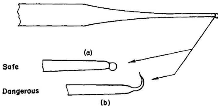
FIG. 6.16. Safe and dangerous points. The end of the point should be melted into a round blob as shown in (a). Ends left as shown in (b) can be very sharp.
