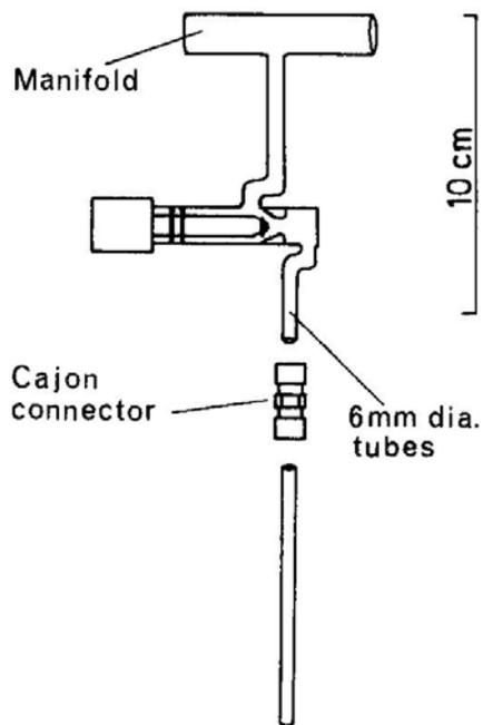
FIG. A.2. One application of Cajon "O"-ring metal connectors.
