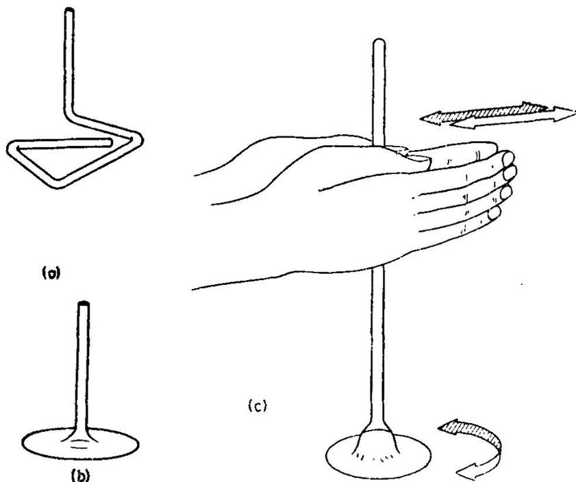
FIG. 8.11. (a) Triangular foot made from glass rod. (b) Wine glass Foot made by spinning. (c) Spinning the foot.
