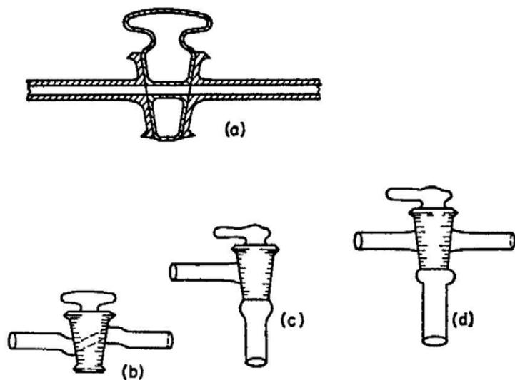
FIG. 11.11. Four common types of stopcock. (a) A straight stopcock with a hollow key. (b) An oblique bore stopcock with a hollow key. (c) An L-type stopcock. The key is a simple hollow cone with a hole drilled through it in line with the side arm. (d) A T-type stopcock. The key is similar to that of (c) but the barrel has two side arms. This stopcock provides alternative paths for gas flow.
