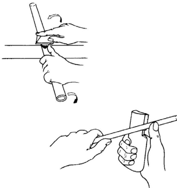
FIG. 6.8. Alternative methods of making a knife mark on glass tubing and rod.
