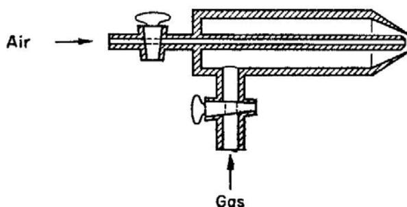
FIG. 4.16. An orifice-mixing bench burner shown in section.
