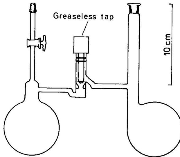
FIG. A.9. A pair of mixing vessels for air, grease, and water-sensitive reagents with a Teflon keyed tap.
