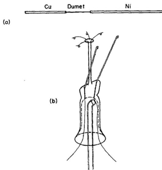
FIG. 7.3. (a) Shows a prepared Dumet wire. One end is welded to a length of copper wire, the other end is welded to a nickel wire. The copper sheath of the Dumet is borated. (b) Dumet wires sealed into an electric lamp foot.
