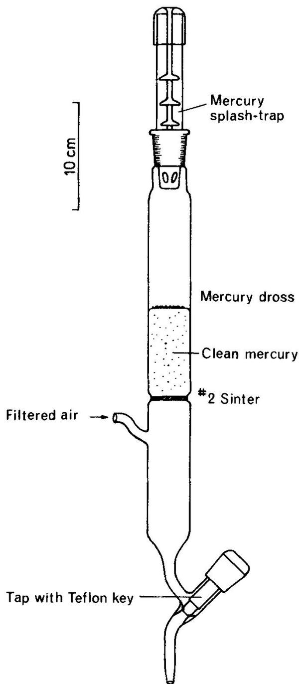
FIG. A.12. A device for cleaning mercury (Hg). This unit consists essentially of a No. 2, 30 mm diameter sintered disc filter tube with a Rotaflow tap on one end and a ground glass socket on the other. A Hg splash trap is incorporated in the stopper,
