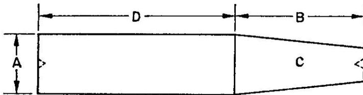
FIG. 11.7. A socket-grinding tool. A, the diameter of the large end of the ground surface  $\pm 0.25$  mm. B, the length of the round zone + 10 mm. C, standard taper of 1 in 10 in the diameter. D, any convenient length to allow for remachining, say 15 cm.
