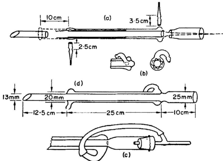
FIG. 8.21. A Liebig condenser. (a) Shows the component parts and the corrugated paper sleeve supporting the inner tube in the jacket. (b) Details of the shape of the water outlet tube are shown in both elevations. The corrugated paper sleeve, in two parts, is shown in section. (c) A blowing arrangement used to make the second internal seal. (d) The finished Liebig condenser.
