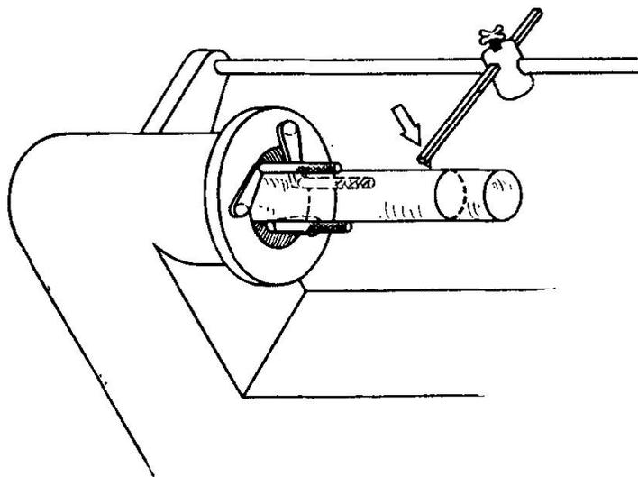
FIG. 4.8. A diamond-tipped tool, used to cut glass tubing held in the lathe chuck. The lathe chuck is turned by hand; some care is desirable to avoid pressing too hard on the tool bar and to avoid extending the scratch beyond one complete turn.
