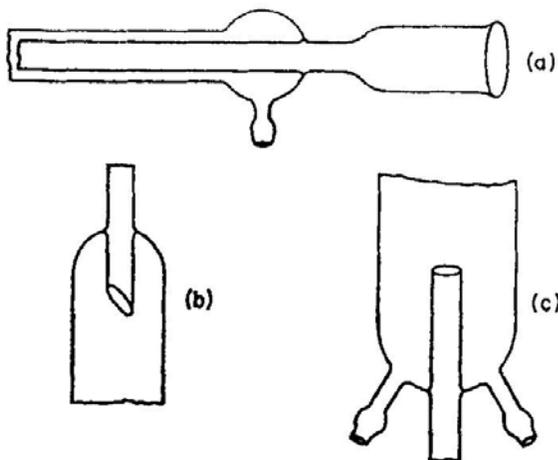
FIG. 6.42. Internal seals. (a) Internal seal in a Liebig condenser. (b) A drop counter, and (c) a constant level device.
