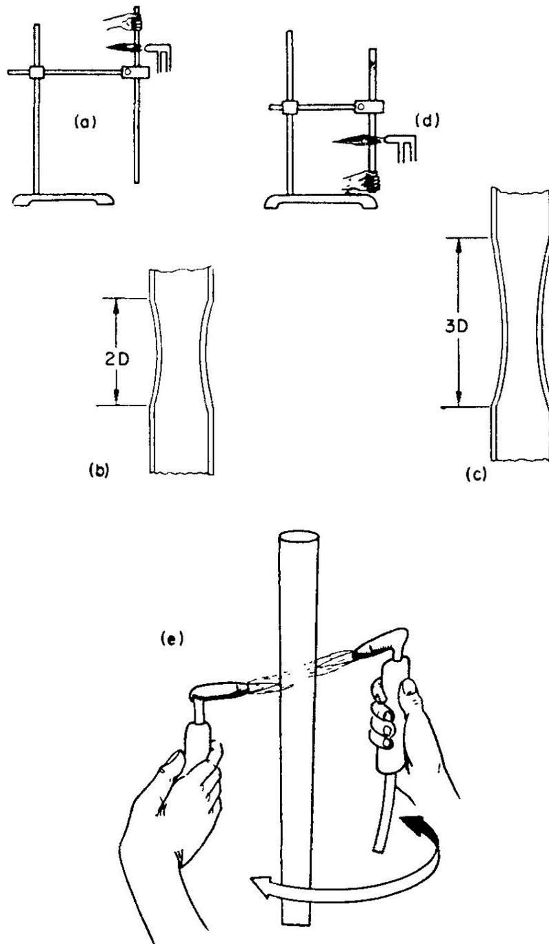
FIG. 8.16. Constrictions made with the handlamp. (a) The tube set up in a retort stand. (b) The glass heated, constricted and ready to pull up. (c) The finished constriction. (d) An alternative arrangement of (a). (e) Shows the movement of the handlamp necessary to heat the glass uniformly all round.
