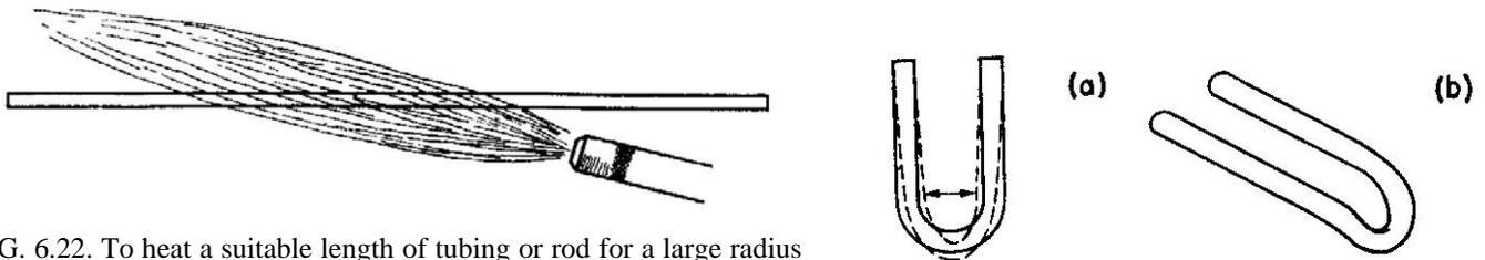
FIG. 6.22. To heat a suitable length of tubing or rod for a large radius bend, the glass is held and rotated in the flame as shown.
