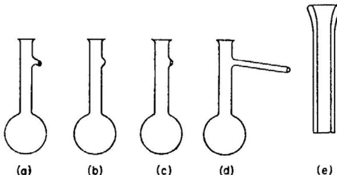
FIG. 8.4. Replacing the side-arm on a distilling flask. (a) Shows the flask and the remnant of the side-arm. (b) The side-arm melted and pulled off with tweezers. (c) A hole blown in the flask neck. (d) The new side-arm joined on. (e) Shows the shape and wall-thickness of the side-arm prepared for joining to the flask.
