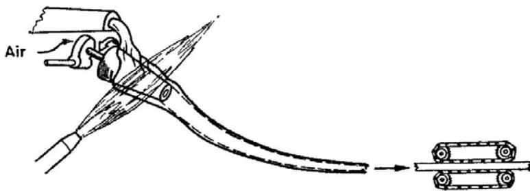
FIG. 1.2. Tube drawing by machine. The Danner Process. The molten glass from the continuous furnace flows on to the hollow rotating mandrel and is drawn off as a tube.
