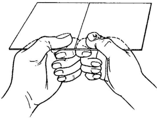
FIG. 6.2. Hand position for a breaking a glass sheet at a mark. The thumbs exert a downward pressure, the fingers press upwards.
