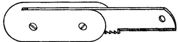
FIG. 4.4. Glass-cutting knife made from a high-speed hack-saw blade.
