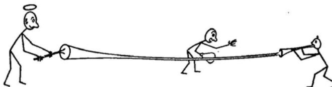
FIG. 1.1. Tube drawing by hand showing two members of the team walking backwards, drawing and blowing the hot glass into a tube, under the direction of a third member who is measuring the tube diameter.
