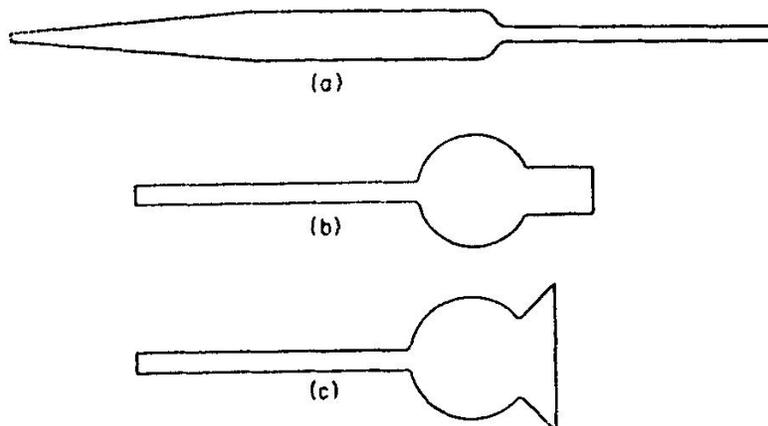
FIG. 8.8. A thistle funnel. (a) Join the stem to a constriction on the larger tube. The point on the larger tube must be straight and of reasonable length. (b) The bulb is blown; note that ample glass must be left to make the flared top. (c) The completed funnel. The flare should be reasonably proportioned and have an angle of about  $90^\circ$ .
