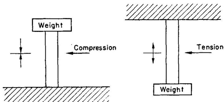
FIG. 5.1. The stresses introduced into a loaded rod.
