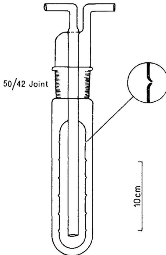
FIG. A.7. A refrigerated impact H<sub>2</sub>O separator. The holes in the inner tube should be about 1.5-2 mm in diameter and distributed evenly over the cylindrical area.
