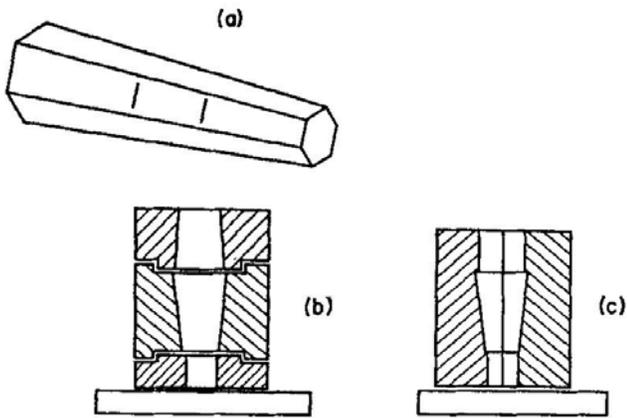
FIG. 11.4. (a) Socket-forming tool showing pencil marks indicating large and small end diameters and overall length of the socket taper. (b) A horizontally split mould. The sections are separated to remove the blown conical joint blank. (c) A vertically split mould. The two sections are separated when the joint blank is ready to be removed.
