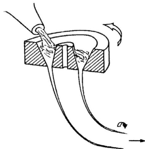
FIG. 1.3. (Right) Tube drawing by machine. The Vello Process. The molten glass flows into the rotating "sink", here shown in section, and emerges as a tube. The tube is drawn away by rollers or tracks similar to those in Fig. 1.2.
