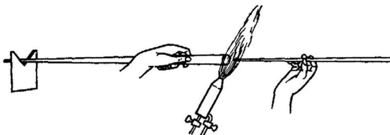
FIG. 6.17. Pulling a point on a tube end. Showing the tube rest, hand positions, burner flame and rod handle.
