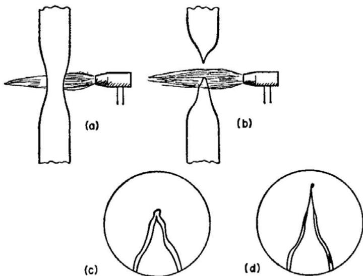
FIG. 8.17. Sealing off a constricted tube. (a) Preliminary heating with soft flame. (b) Sealing off with small, hot flame. (c) A satisfactory seal with no thin glass. (d) The result of pulling the glass up too far. Note the thin fragile glass.
