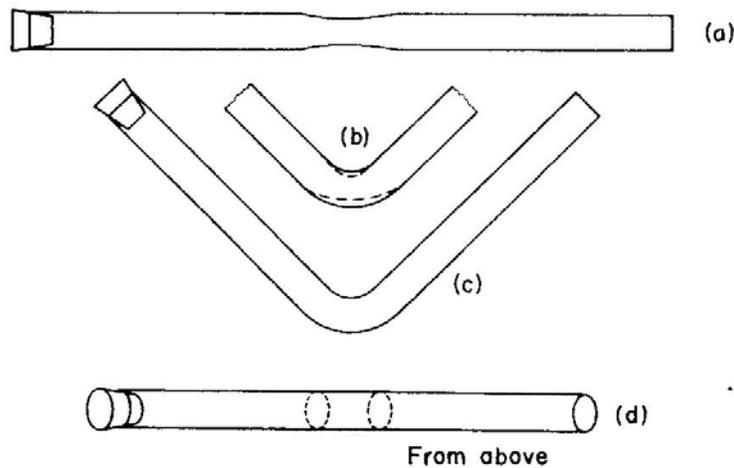
FIG. 6.24. Short radius bend. (a) The glass heated and constricted slightly and ready to bend; (b) the dotted lines show the tube after bending and before blowing up; (c) and (d) show the finished bend in plan and elevation. Note that both limbs and the bend lie in the same plane.
