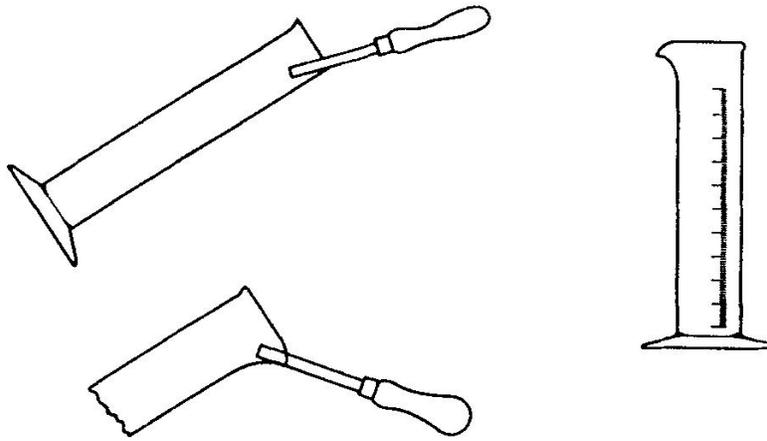
FIG. 8.3. Forming a new spout on a measuring cylinder.
