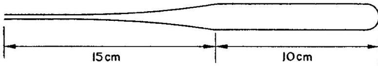
FIG. 11.6. A blank for a 14/23 cone.
