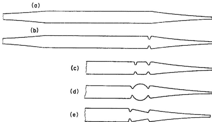
FIG. 6.41. Ruffled side tubes. These tubes are prepared in pairs from double points shown in (a). (b) The first constriction and (c) the second constriction must be neat and of reasonable wall-thickness. (d) Shows the bulb blown up. (e) Shows the bulb drawn into shape after heating on one side. The procedure is repeated at the other end of the double point.
