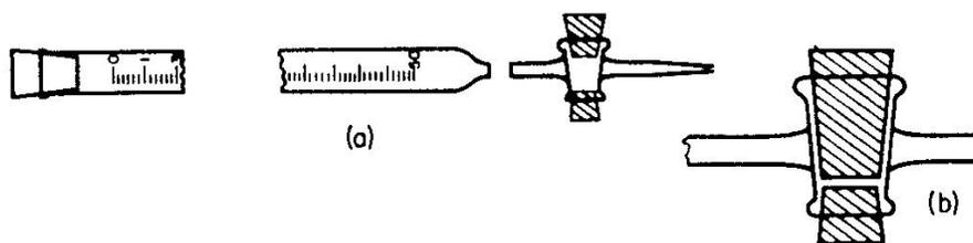
FIG. 8.2. Replacing burette stopcocks. (a) The burette and stopcock ready to be joined. Note the orientation of the stopcock bari'el and the scale. (b) Shows the side tube bore blocked by a stopper which is too long.
