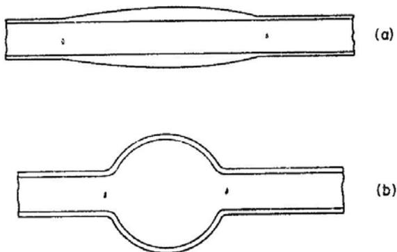
FIG. 6.37. Bulb blowing. (a) The length of glass required for the bulb is marked on the selected tube. All the glass between these marks is heated and gathered, as shown, before the bulb is blown. (b) Shows the bulb blown to the required size, and the final position of the marks.
