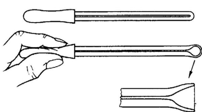
FIG 3.2. Blowing out a capillary tube end with the aid of a small rubber bulb or a stoppered rubber tube.
