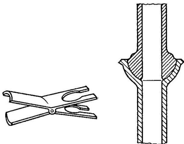
FIG. 11.9. Ball and socket joint with clip.
