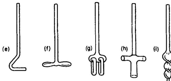
FIG. 8.5. Glass rod stirrers. (a) Plain rod stirrer. (b) Paddle stirrer. (c) Button stirrer. (d) Button stirrer pushed too far down and liable to crack. (e) Bent rod stirrer. (f) Propeller stirrer. (g) Link stirrer. (h) Centrifugal stirrer. (i) Spiral stirrer.
