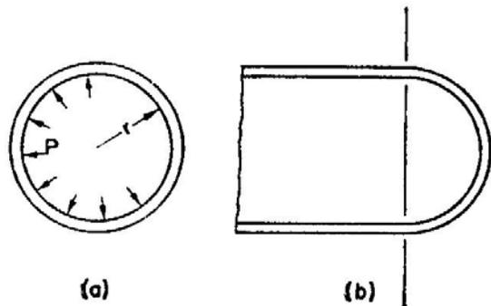
FIG 3.1. The excess internal pressure required to blow out a test-tube end (b), is the same as that required to blow out a spherical liquid bubble (a).
