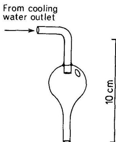
FIG. A.1. A cooling-water flow indicator. The drainage tube should be slightly larger in internal diameter than the inlet tube. The vent hole in the bulb ensures that the water pressure is independent of the length of the drainage tube.
