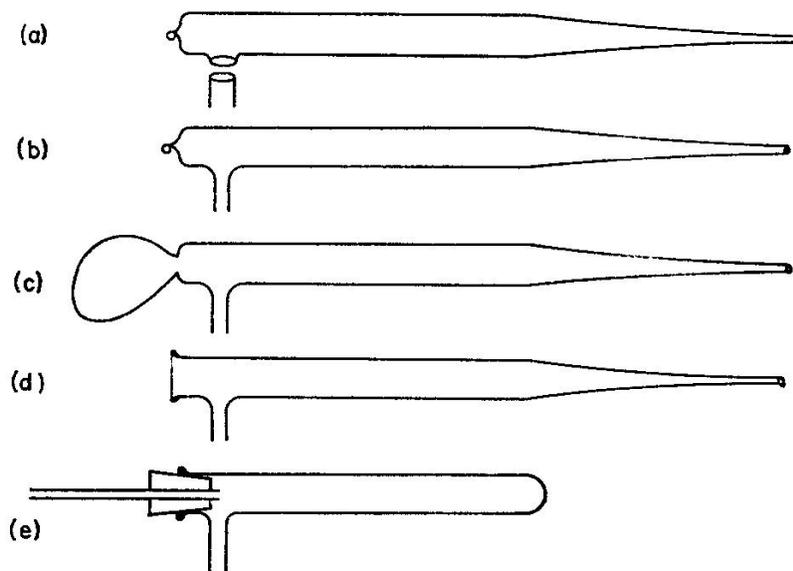
FIG. 6.35. Side tube near the end of a test-tube. (a) Double points are made from suitable tubing, one point is sealed off and the side tube attached as shown in (b). (c) The sealed off end is blown out and rimmed as in (d). (e) When the newly made rim has cooled, the open end of the test tube is fitted with a bored cork carrying a handle; the other end is sealed off and blown up to a neat hemisphere.
