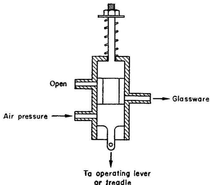
FIG. 3.3. A two-way valve for controlling air pressure. The air in the glass being heated can expand to atmosphere when the piston is in the position shown. Air pressure is admitted to the molten glass when the lever is depressed.
