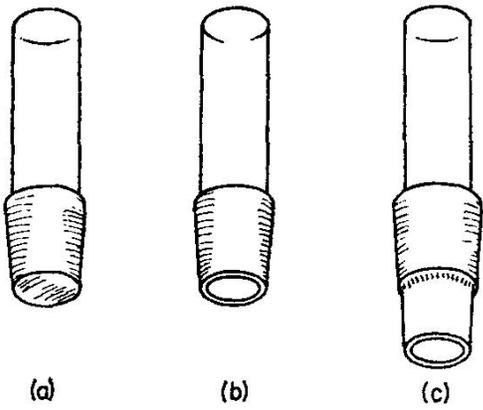
FIG. 11.2. Types of cones. (a) Closed-end cone, used for stoppers. (b) Open-end cone for general purposes. (c) Tube extension on cone, used for thermometer pockets, gas admission leads and other similar purposes.
