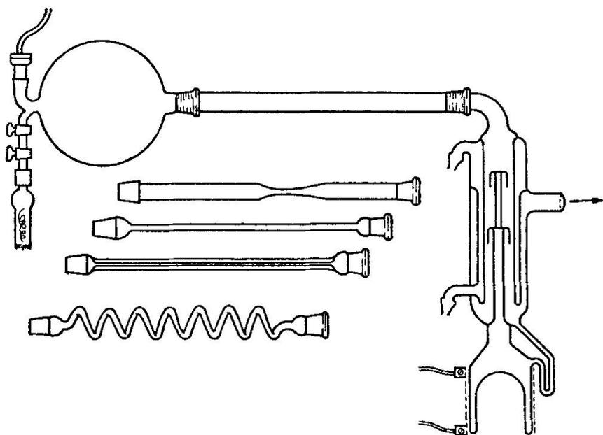
FIG. 10.2. Glassware used in an experiment designed to show the effect of tube diameter on pumping speed.
