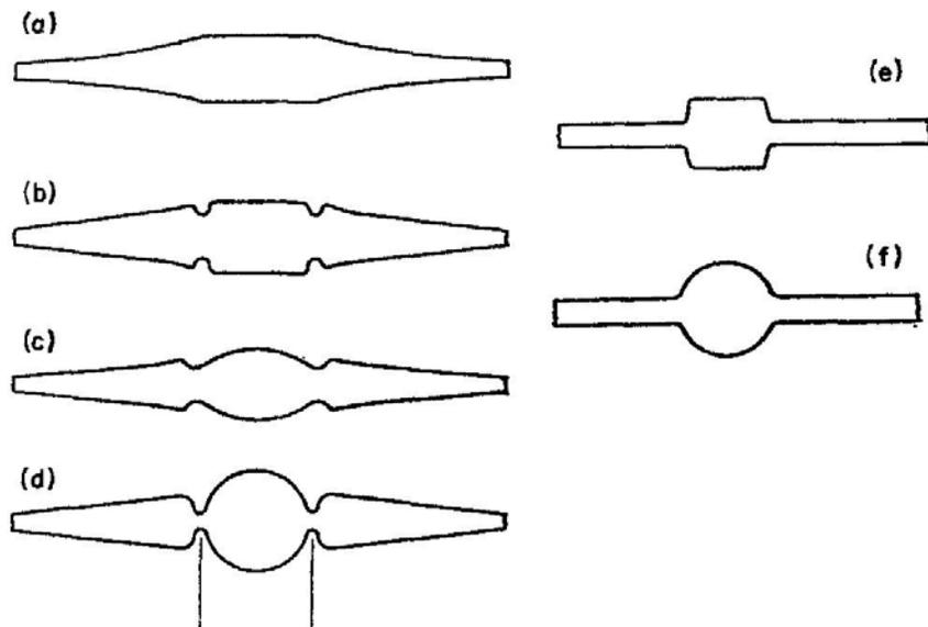
FIG. 6.40. Blowing a bulb from a large diameter tube. (a) Shows double points drawn from tubing of four-fifths the diameter of the required bulb. (b) The constrictions made at the shoulders. (c) The heated and gathered glass ready for blowing up to the desired size, as shown in (d). (e) Shows tubes joined to the constrictions before blowing the bulb. (f) The finished bulb with tubes attached.
