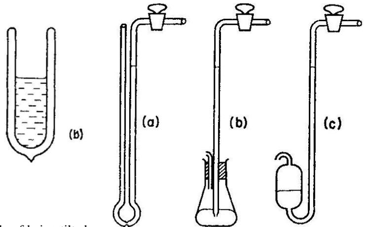
FIG. 10.10. Three types of open limb U-tube manometer.
