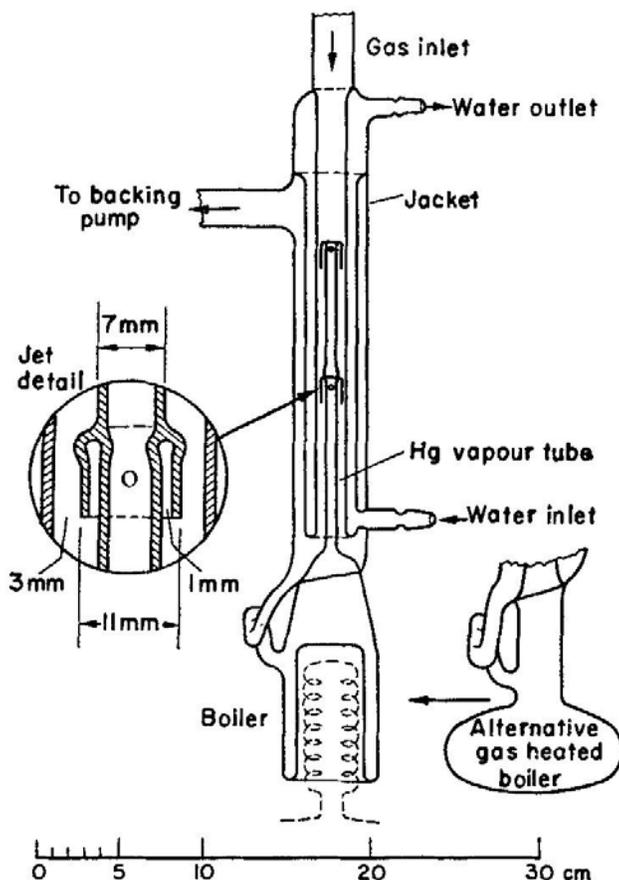
FIG. 9.3. A mercury diffusion pump and an alternative boiler for gas heating.
