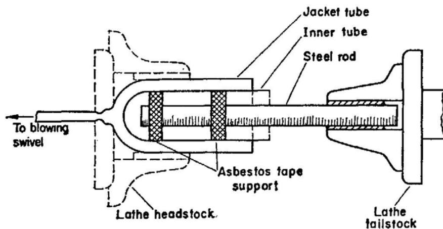
Borosilicate glass is recommended as it is able to withstand the wide range of temperatures involved in using liquid nitrogen. The author makes such flasks from English Pyrex brand glass tubing, and employs a glassworking lathe.
