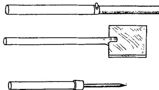
FIG. 4.10. Hand tools for lathe work. Made from carbon and fitted with brass tube handles.
