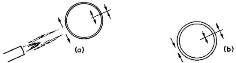
FIG. 5.3. Shows the effect of applying local heat to a thin slice of glass tube. At a radial section opposite the heated spot, compressive stresses are set up in the outer layer of glass, and tensile stresses are set up in the inner layer, as shown in (a). These stresses disappear when the heated spot begins to soften. When the glass is allowed to cool the heated spot contracts and sets up compressive stresses in the inner layer and tensile stresses in the outer layer as shown in (b).
