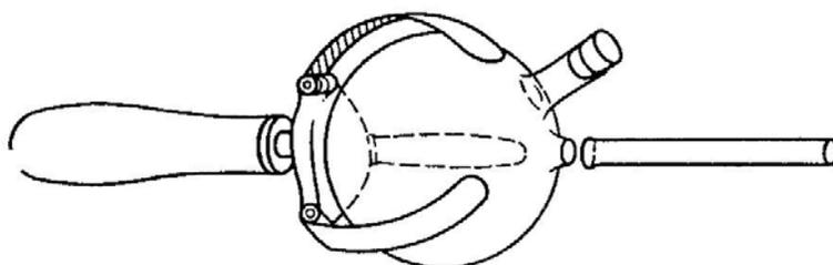
FIG 4.13. An adjustable bulb holder.
