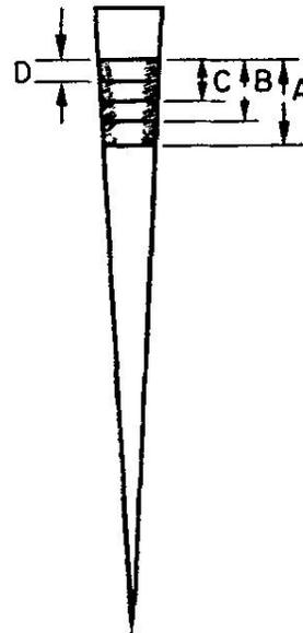
FIG. 11.1. Shows a standard taper conical surface with the height equal to ten times the diameter of the base. The ground surfaces of all standard taper conical joints are part of an exactly similar cone; the proportions of these surfaces depend on the purpose for which they are to be used and may be A, B, C, or D.
