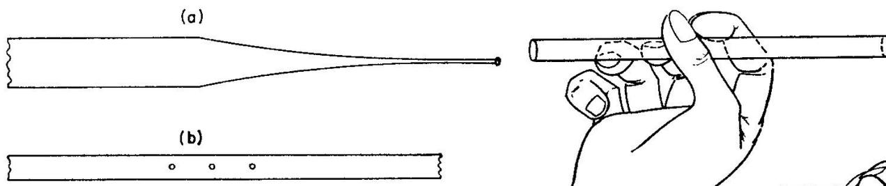
FIG. 6.13. (a) A point on a glass tube. (b) Shows guide marks which help to keep the tube free from twists.
