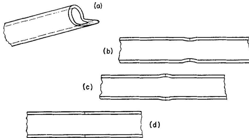
FIG. 6.28. Joining normal tubing: (a) shows the type of sharp edge that may cut the lips; (b) the tube ends pulled very slightly apart after first bringing them together; (c) the joint is shown melted thoroughly, slightly gathered and ready to be blown and pulled into shape as shown in (d).
