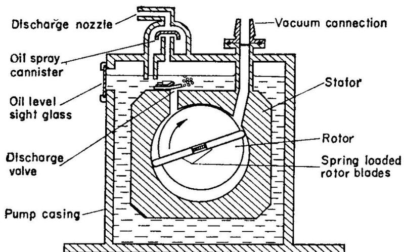
FIG. 10.4. Section through a rotary oil pump.
