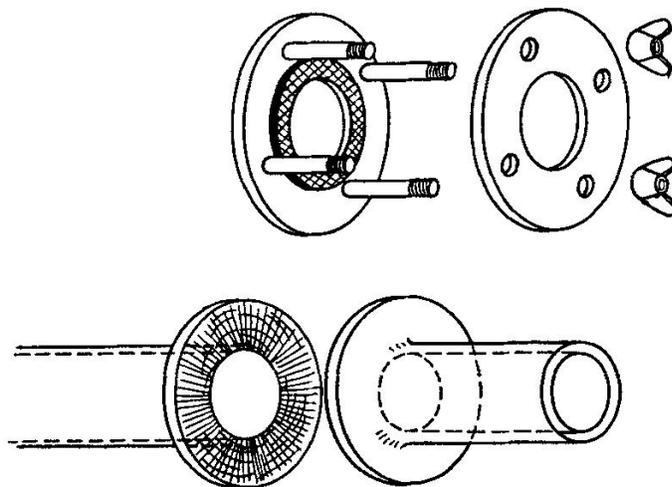
FIG. 11.10. Flat flange joint and clamp.
