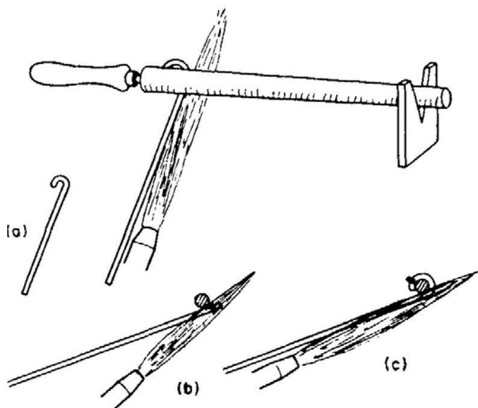
FIG. 8.13. (Left) Spiral coils, "(a) Shows the small U-bend ready to hook into the metal loop on the forming tool. (b) The elevation of the tube at the beginning. (c) The elevation of the tube when winding is under way.
