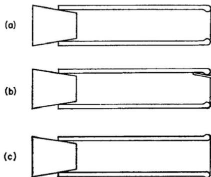
FIG. 6.11. Making a rim on a tube. (a) The heated glass thickened and constricted. (b) The tube end being opened out with a reamer. (c) The finished reinforced end ready for flame-annealing.
