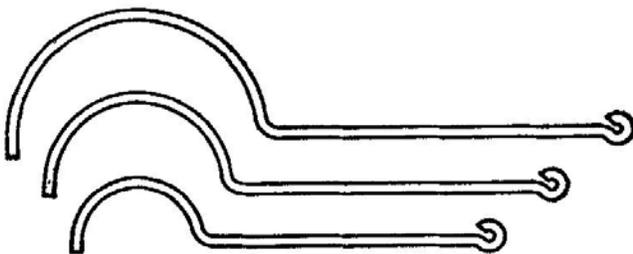
FIG. 4.5. Iron wire hooks. The glass tube is scratched with a knife or file, the wire hook is heated to cherry red. The tube is held horizontally and rotated with the scratch in contact with the hot wire. A crack will immediately appear and travel round the tube, leaving a clean straight cut end.
