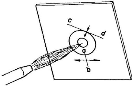
FIG. 5.2. Local heat applied to a thin sheet of glass (inner circle) will set up stresses in the surrounding glass (outer circle). These stresses will be compressive at a tangent to the outer circle and tensile in the radial direction.
