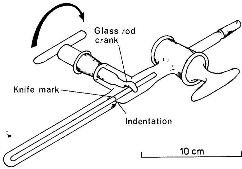
FIG. A.11. A break-seal attachment, used to open sealed N.M.R. tubes to allow for recovery of a sample.
