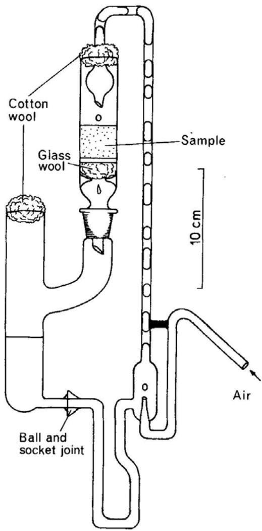
FIG. A.10. An improved perfusion unit, This unit operates with compressed air. The components are easily assembled and are interchangeable with those of similar units.
