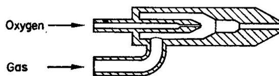
FIG 17. A premix burner shown in section.
