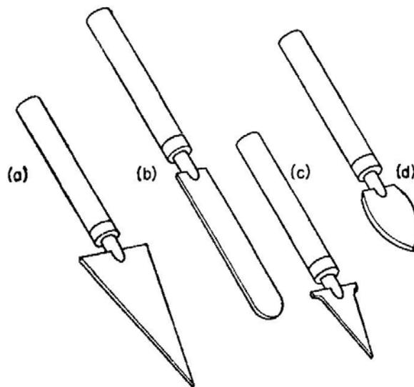
FIG. 4.9. Hand tools with brass blades. Used for bench work: (a) is used to make moderately large flanges; (b) is used to make rims on tube ends; (c) is used to rim and flange small diameter tubes; (d) is a general purpose flanging and rimming tool.
