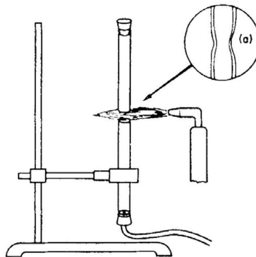
FIG. 8.18. Handlamp joint showing the retort stand and blow tube. The stopped tube is held in the left hand; the handlamp is held in the right hand and moved round to heat all the joint. (a) shows the joint pulled slightly apart immediately after the ends are touched together.
