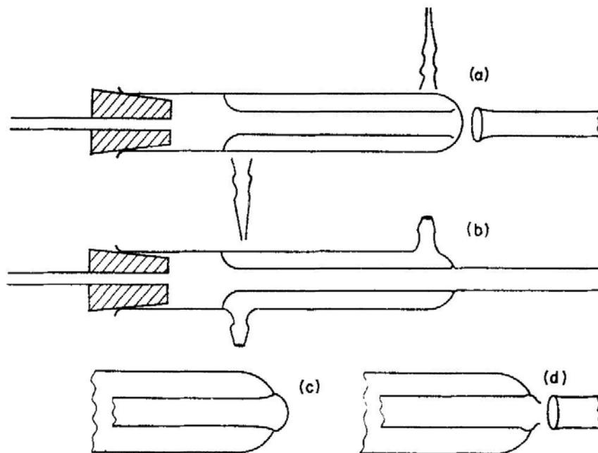
FIG. 6.47. A simple condenser. (a) Shows the proportions of the five parts. The large test tube is 18 mm long and 20 mm in diameter. (b) The completed condenser. The order of steps taken in the assembly of the parts is described in the text. (c) and (d) Details of the formation of the first internal seal.
