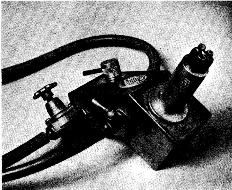
PLATE 4.2. A premix bench burner with turret head and provision for attaching a hand lamp. Made by L.V.D.Scorah, 44 Northfield Road, Birmingham 30, England.
