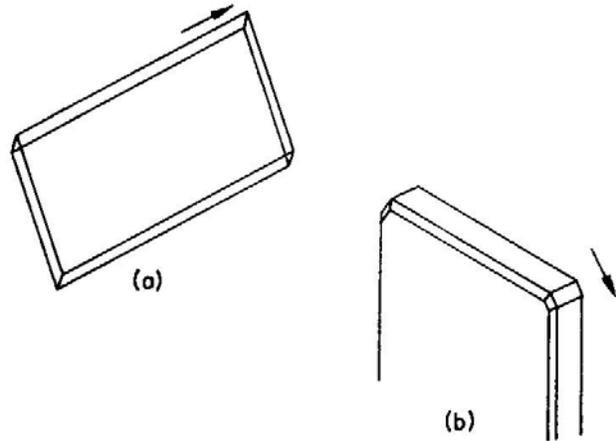
FIG. 6.3. Removing sharp edges with a hand-stone. (a) Shows the edges of a newly cut piece of glass sheet. (b) Shows the edges ground off. The arrows indicate the direction of movement of the stone.
