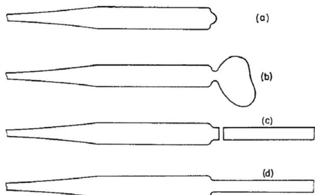
FIG. 6.31. A method of joining tubes of different diameter: (a) shows the test-tube end with the small bulb blown up. This bulb is blown out in (b). The completed joint is shown in (d).
