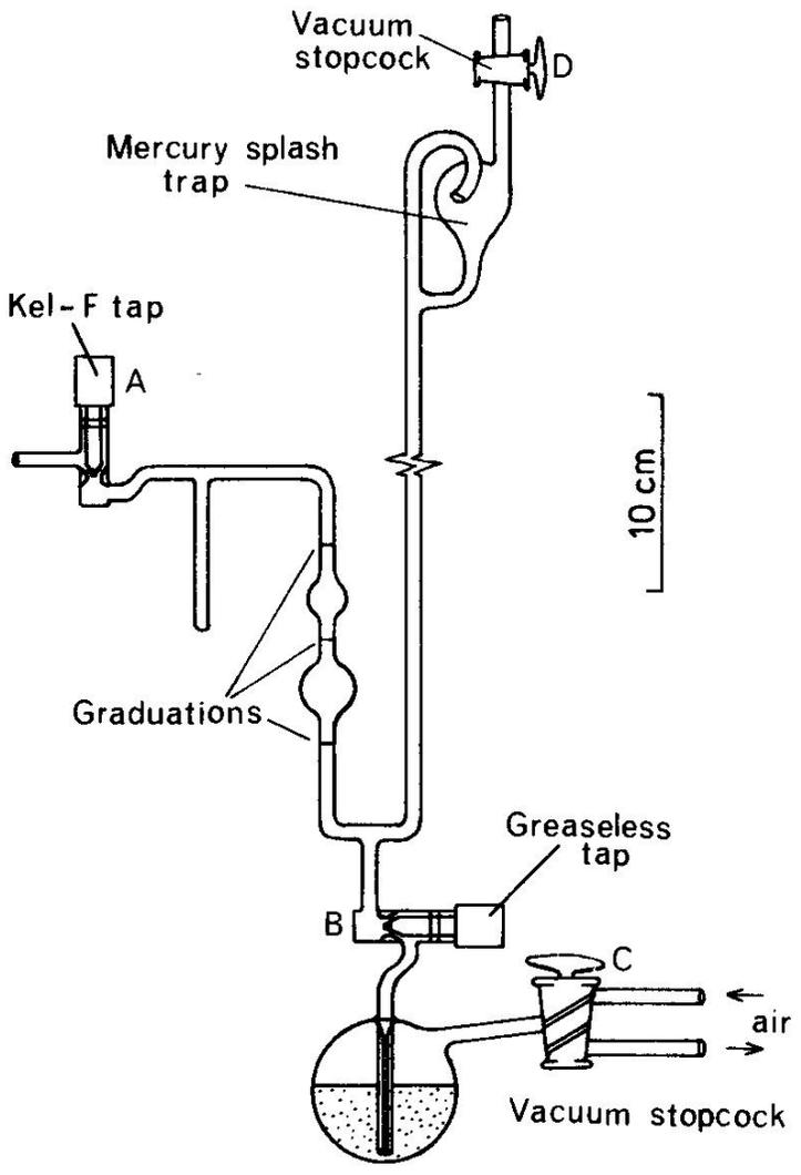
FIG. A.13. An improved constant volume manometer. The inclusion of a Kel-F type greaseless tap permits the measurement of grease sensitive gases. The Rotaflow tap between the U-tube and the reservoir prevents contamination of the Hg.
