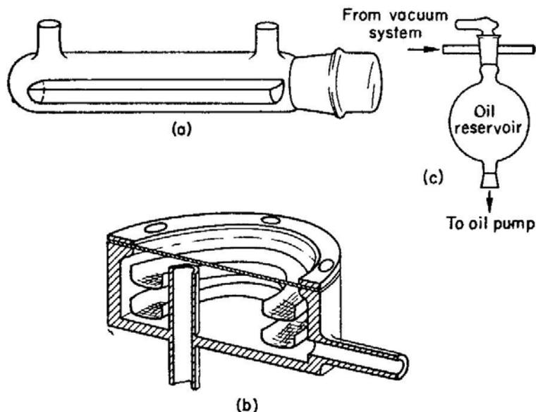
FIG. 10.5. (a) A glass moisture trap containing a boat for phosphorus pentoxide. (b) A metal moisture trap in section, showing the trays for phosphorus pentoxide. (c) Oil reservoir, fitted to the vacuum connection on a rotary oil pump. The two-way stopcock is opened to the atmosphere when the pump is stopped.
