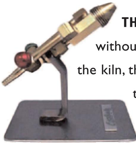
**THE TORCH:** Nothing in glassmaking proceeds without heat and once the molten glass is removed from the kiln, the torch is the way additional heat is applied. The torch has an outer flame that allows you to work a large section of glass and an inner flame that's very sharp and allows for details. Working at glassblowing with a torch is also known as lampworking.
