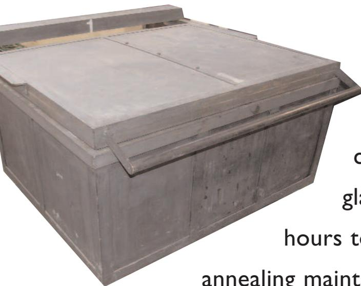
**ANNEALING OVEN:** This is a chamber to gradually cool glass down to room temperature. Because it gradually cools the hot glass down, it prevents the glass from cracking. It takes about 24 hours to properly cool a piece down. Proper annealing maintains the longevity of your piece as well.
