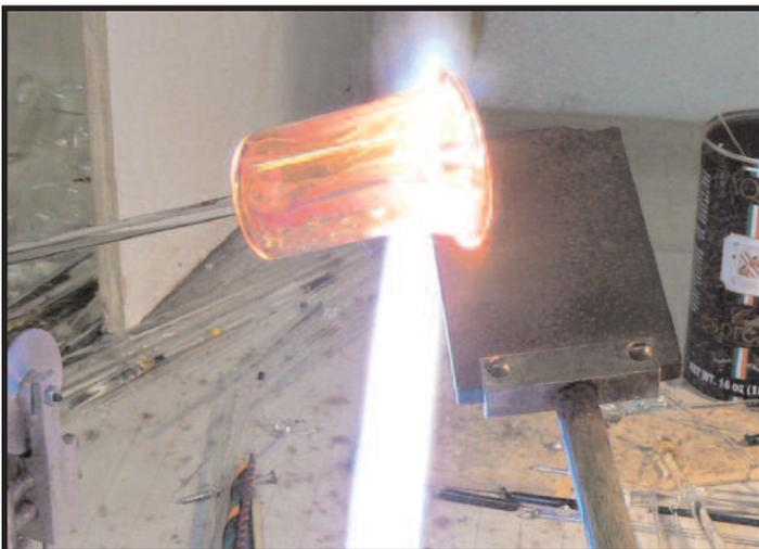
Now it's time to heat the open end of your cup, after which you will immediately marver it down to a size that can accept the size of a blowtube which is needed at this point.
