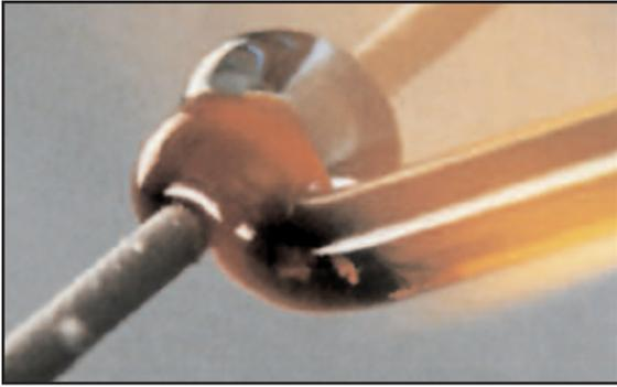
marver in much the same way you would roll out a cylinder of dough. A graphite paddle can be used to even the ends up. If you want to make a bead with a groove or pattern, you can roll it
