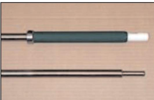
**THE PUNTY:** A punty is basically a solid or hollow rod, often stainless steel or graphite, used to transfer a piece from the blowpipe onto the punty. This allows
