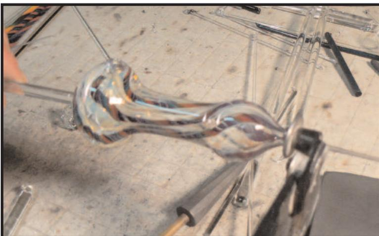
When the basic pipe is formed, you can remove the blowtube and attach the punty again to work on the finishing touches of your pipe, including cutting off the end with disc cutter.
