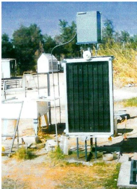
**Figure 3.34** Photograph of the vertical solar still erected at Algeria (Boukar and Harmin, 2007).
