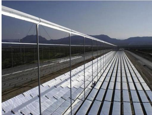
**Figure 6.3** Linear receiver of linear Fresnel type mirrors.
