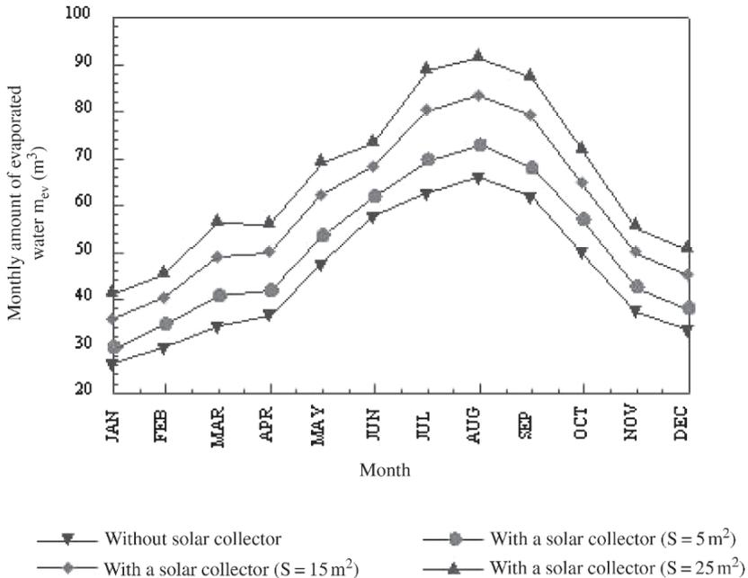
Figure 2. Variation of the monthly evaporated water for different solar collector surfaces.
