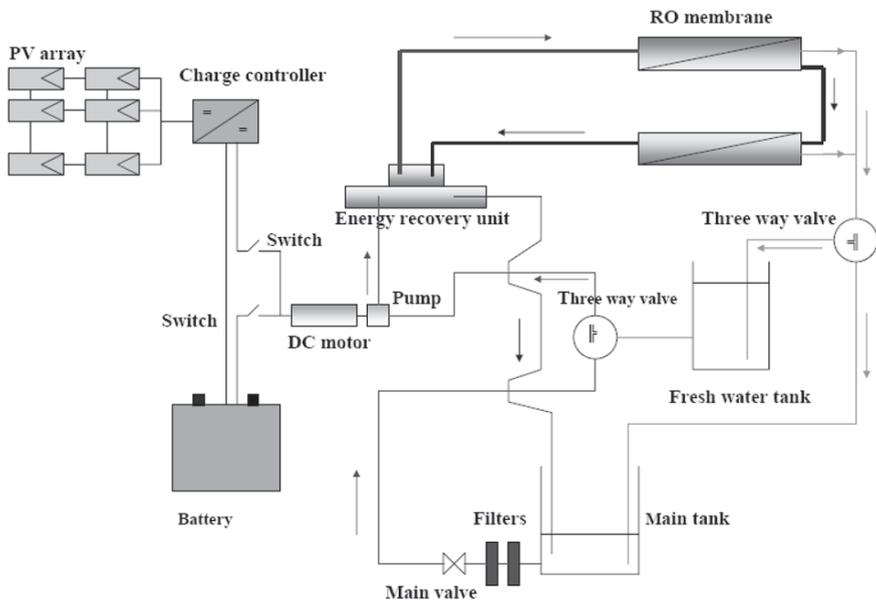
Figure 1. Schematic diagram of a PV-battery driven RO system equipped with energy recovery of the Clark pump type.
