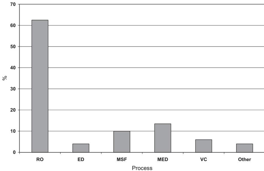
Figure 2. Desalination processes used in conjunction with renewable energy<sup>5</sup>.
