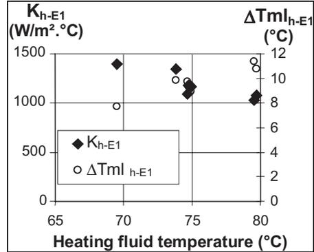
Figure 5. Heat transfer coefficient between heating cell and evaporator 1 and mean temperature difference as functions of heating fluid inlet temperature for  $Q_h = 7 \text{ m}^3/\text{h}$ .
