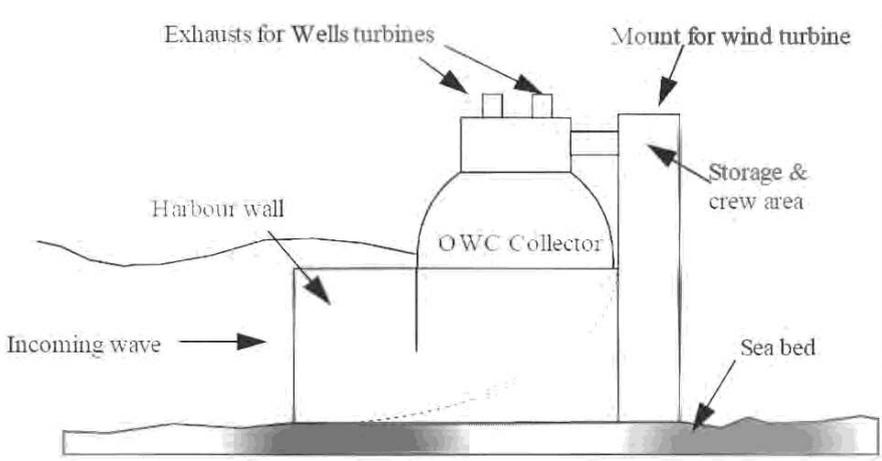
Figure 13. Osprey device. Source: Wavegen
