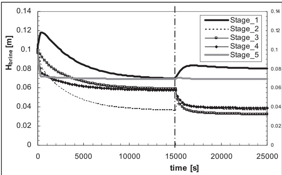
Figure 11. Trends in brine levels in the stages after the introduction of a leakage in the third stage.
