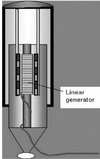
Figure 14. Archimedes wave swing device. Source: Teamwork Technology.
