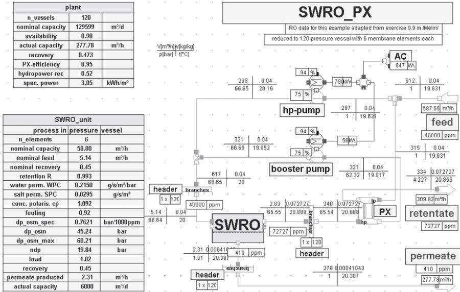
Figure 4. IPSEpro scheme for basic SWRO system (no pre- and post-treatment considered).
