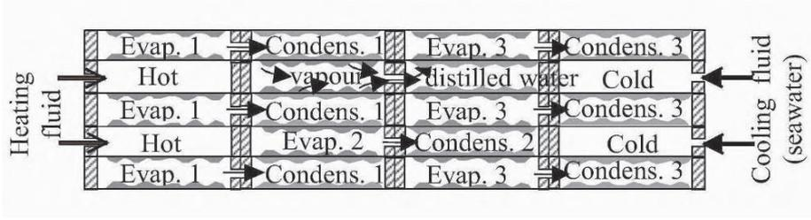
Figure 2. Top view of the association of elementary cells: 3 in series x 5 in parallel.
