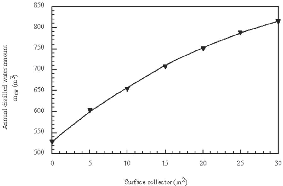
Figure 3. Variation of the annual evaporated water amount versus the solar surface collector ( $m_{air}=0,3$  kg/s).
