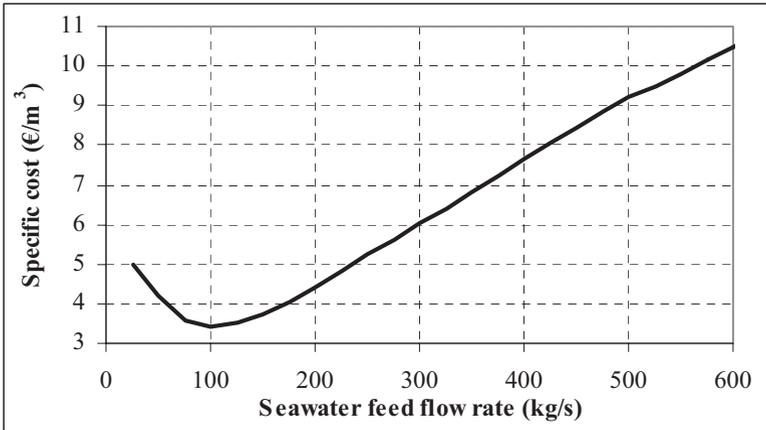
Figure 7. Cost as a function of the seawater flow rate sent to the MSF-M section.
