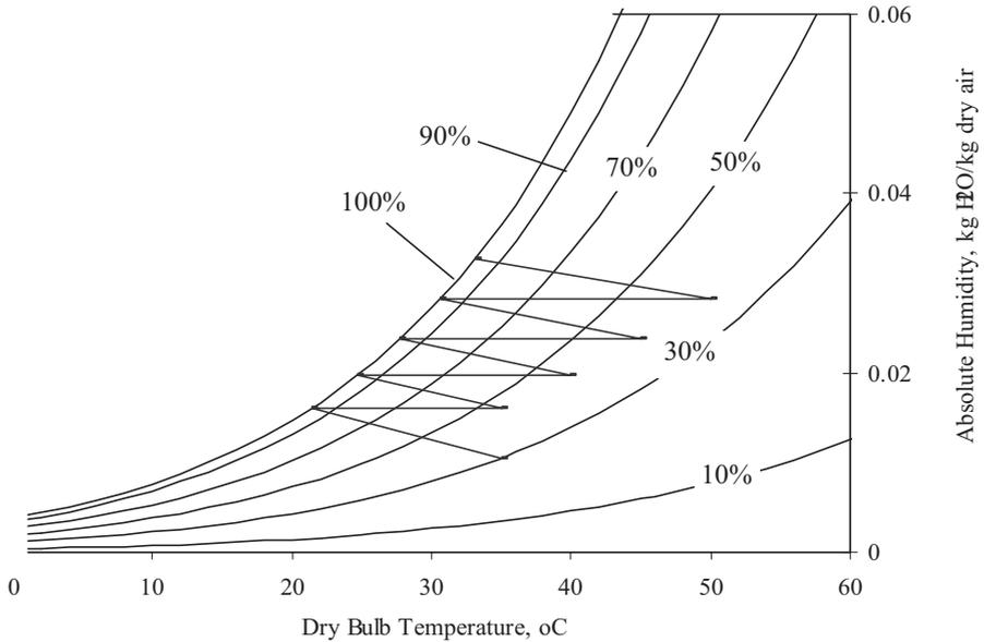
Figure 9. Humidity chart for multiple air heating humidification dehumidification process.
