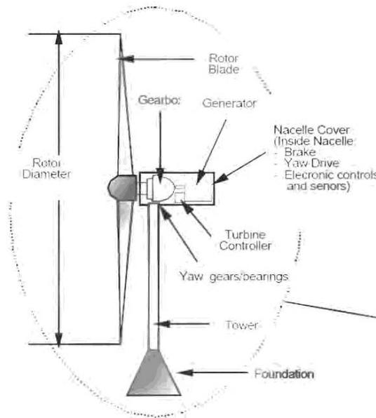
Figure 5. Horizontal axis wind turbine.
