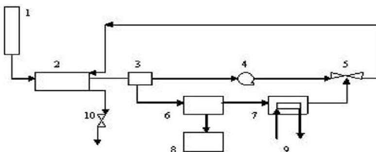
Figure 4. 1 - Vessel with NaCl water solution, 2- RO membrane, 3 - flow dividing valve, 4 pump, 5 - ejector, 6 - flashbox, 7- condenser, 8 - accumulator tank, 9 - cooling water, 10 - flow controller of feed water.
