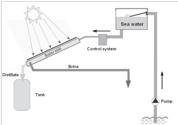
Figure 2. Principle of desalination by solar still.
