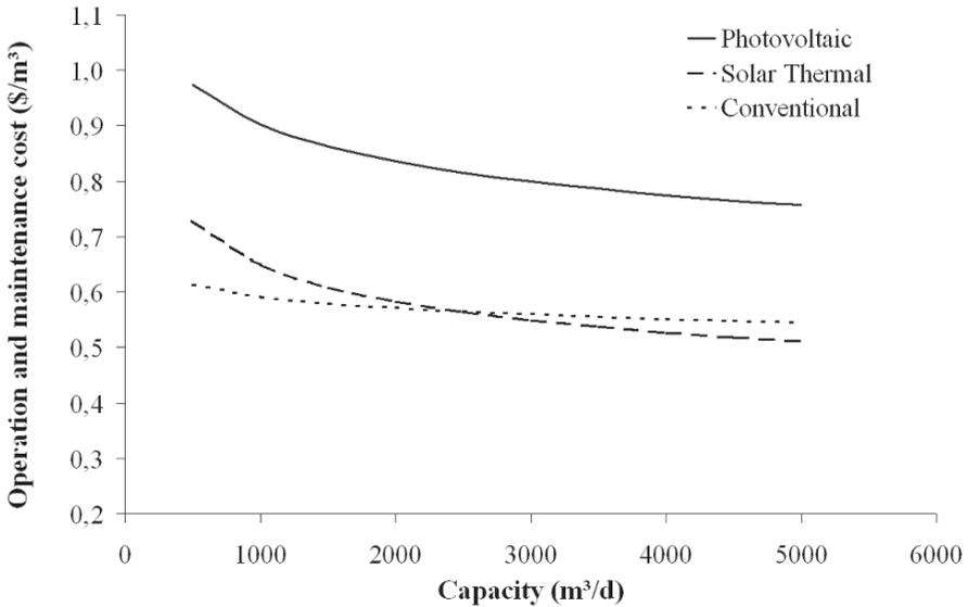
Figure 3. Operation and maintenance specific cost as a function of plant capacity by means of two solar systems (PV/RO and ST/MEE) and a conventional one.
