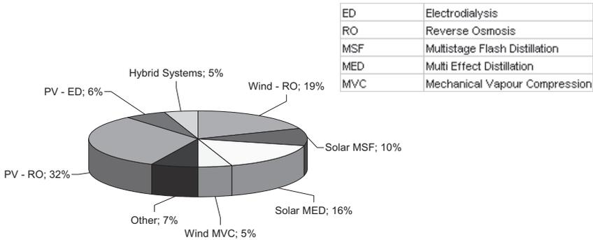
Figure 1. Technology combinations used in the installations identified.
