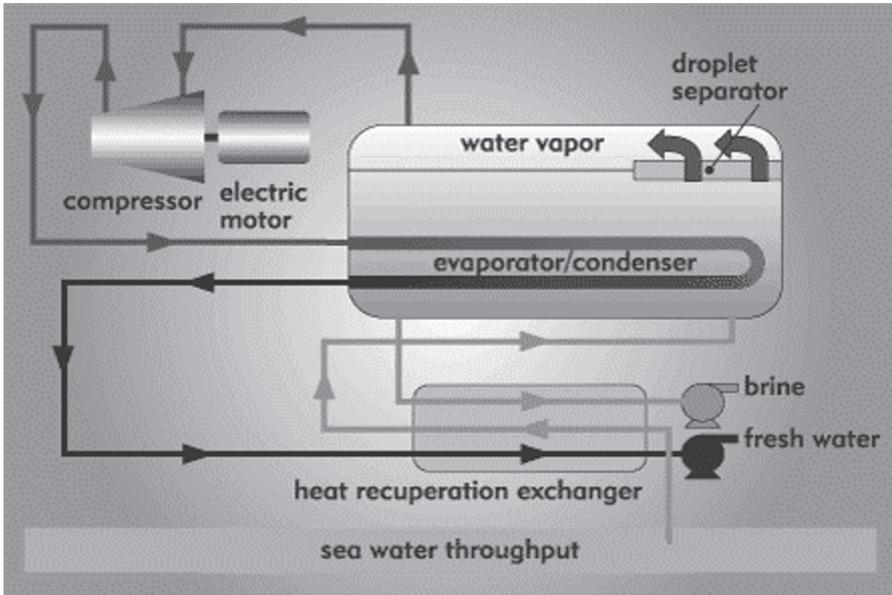
Figure 3. Mechanical vapour compression. Source: French Atomic Energy Commission.
