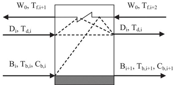
Figure 2. Scheme of the single flash in a MSF plant.
