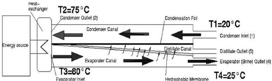
Figure 2. Schematic set-up of a membrane distillation module with internal heat recovery function.
