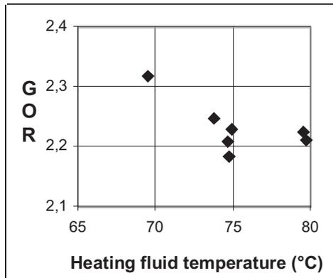
Figure 7. Gain Output Ratio as a function of heating fluid temperature for  $Q_h=7 \text{ m}^3/\text{h}$ .
