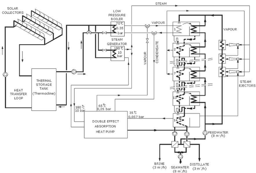
Figure 2. Improved solar MED system (STD Project - Phase II).
