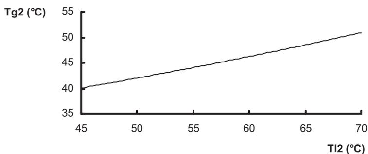
Figure 8. Impact of water temperature at the evaporation tower inlet on the air temperature (top of the evaporation tower).
