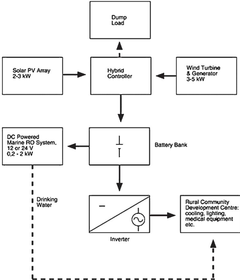
Figure 1. Combined Community Centre Electrification and Water Desalination with Renewable Energy.
