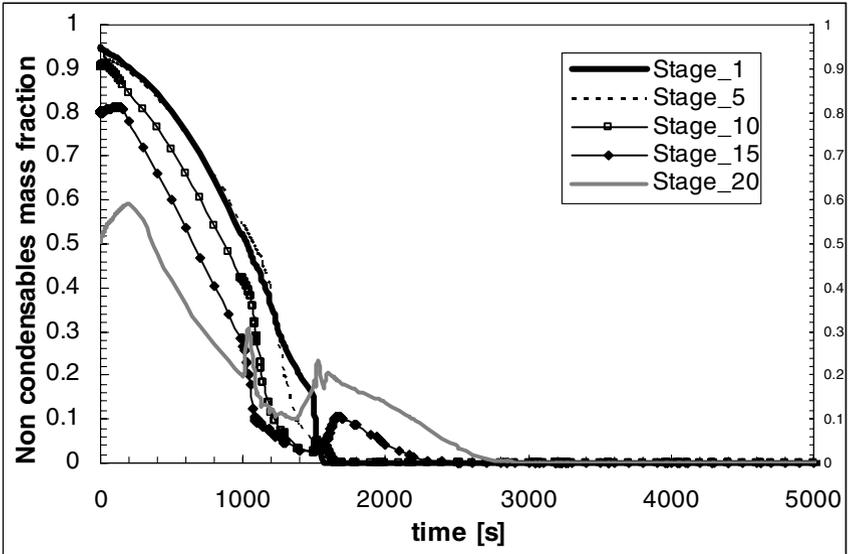
Figure 8. Variation in the mass fraction of non-condensables during start-up operations (first 5000s).
