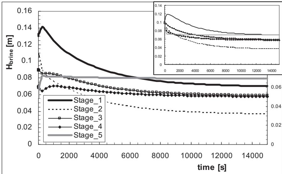
Figure 9. Comparison of trends in brine levels between the standard case (small inset in the upper part of the figure) and the case with different initial brine levels in the stages.
