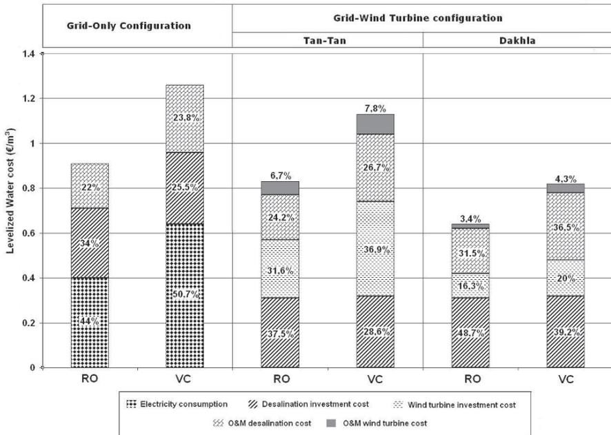
Figure 8. The Levelized Water Cost breakdown.
