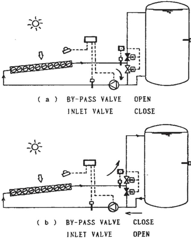
Figure 7. Bypass valve operation for the solar collector field.
