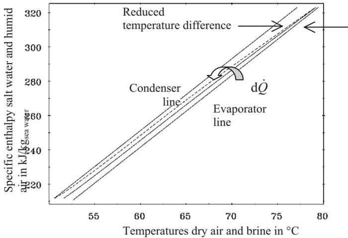
Figure 3. Adapting the volume flows of dry air and fluid in the correct way, the temperature difference is mainly determined by heat and mass flow resistances. “Specific” herein is related to mass flow of salt water.
