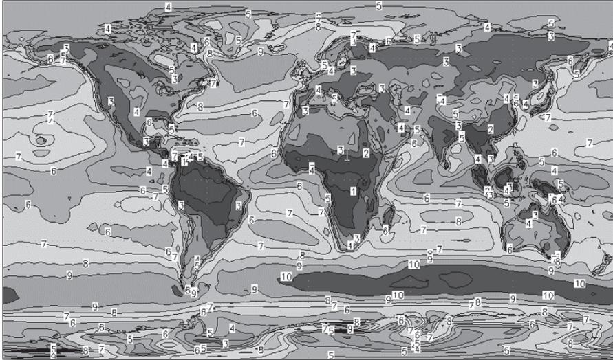
Figure 4. Wind Atlas of the World (wind speed in  $\text{ms}^{-1}$ ). Source: Risoe National Laboratory.
