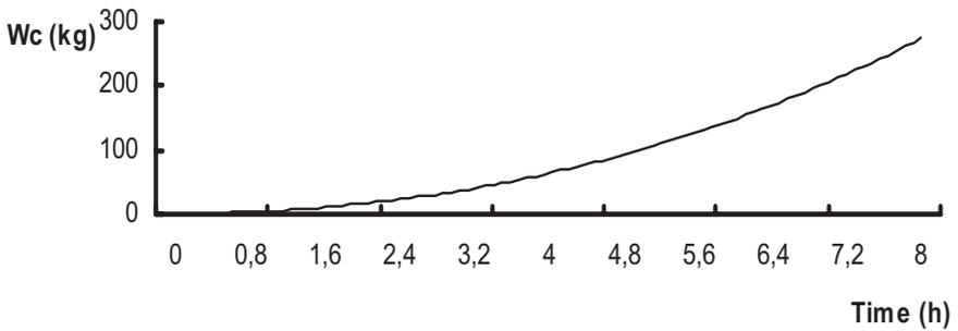
Figure 11. Variation of the distilled water produced for a pilot unit.
