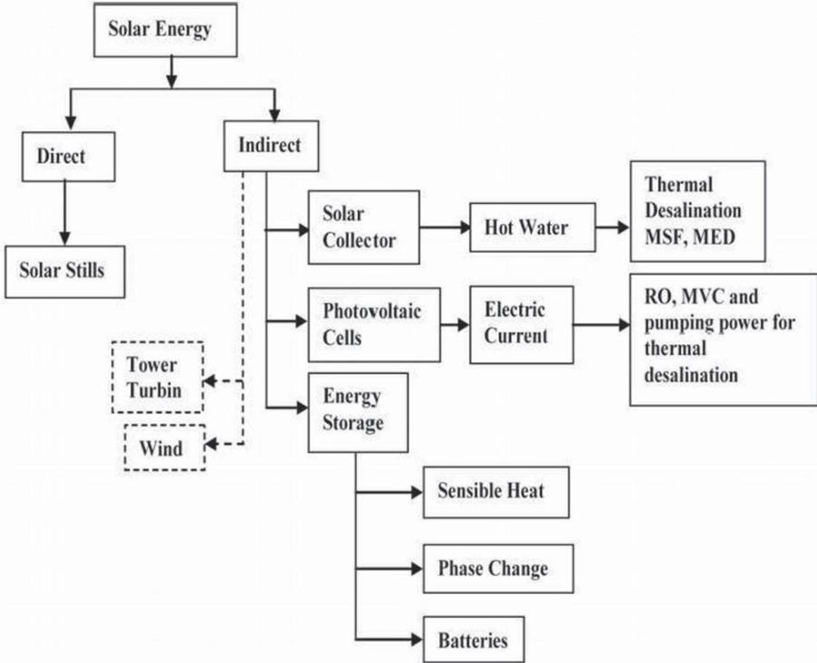
Figure 1. Classification of direct and indirect solar desalination.
