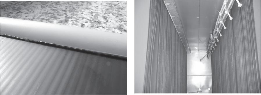
Figure 5. Newly developed plastic welding method ensures high performing condenser plates made from polypropylene material.
