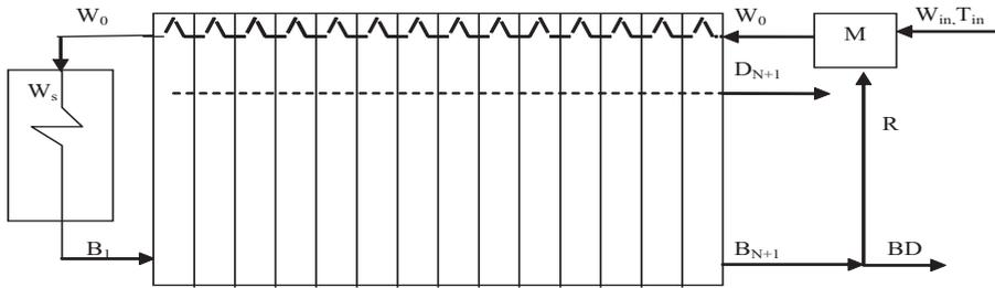
Figure 3. Scheme of a MSF-M plant.
