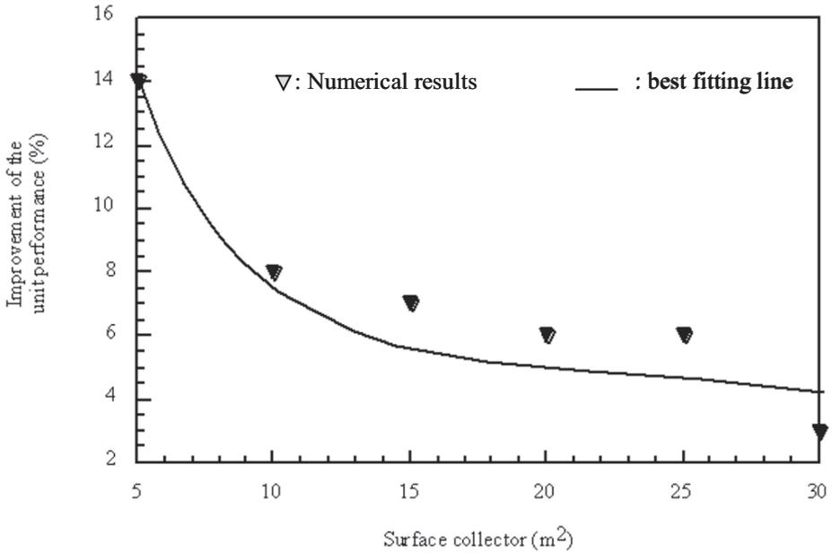
Figure 4. Variation of unit performances versus the solar collector surfaces ( $m_{air} = 0,3$  kg/s).
