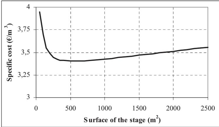
Figure 5. Specific cost as a function of the surface of the stage.
