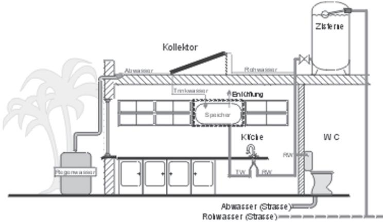
Figure 6. Complete package of licensed partner in Puerto Rico including raw water tank, solar cell, Rosendahl collector.
