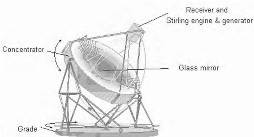
Figure 4. Scheme of a Dish/Stirling system<sup>6</sup>.
