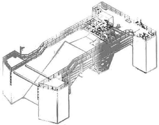
Figure 16. Floating Wave Power Vessel device. Source: Sea Power International.
