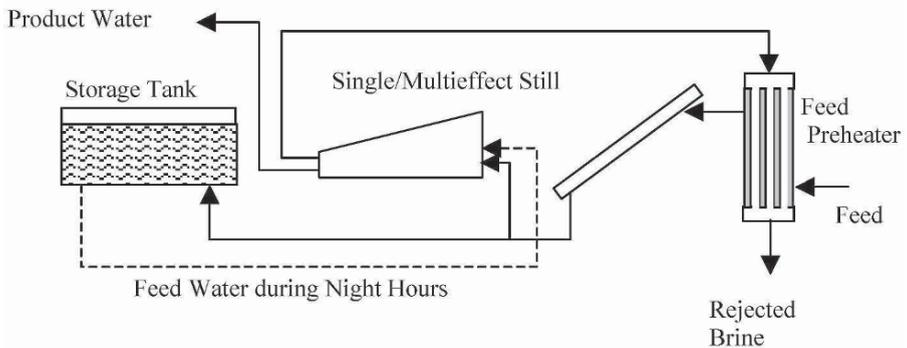
Figure 3. Schematic of a solar still configuration together with feed preheating, collector, and hot water storage.
