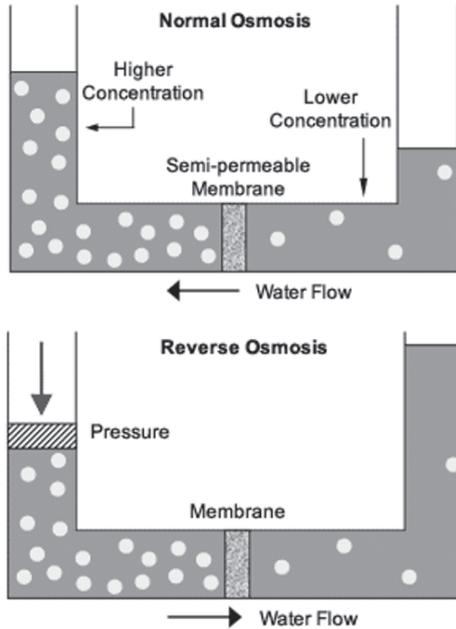
Figure 1. Normal and reverse osmosis. Source: Vision Engineer.
