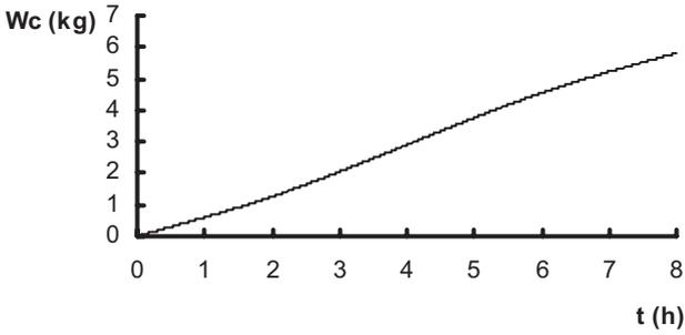
Figure 9. Variation of the condensation rate: Operating mode 1 (nominal mode).
