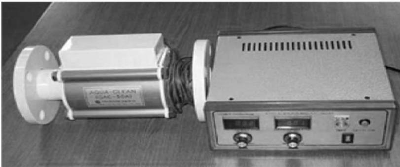
*Figure 3.* Water disinfecting device used for water pre-treatment.
