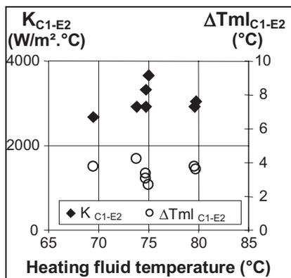
Figure 6. Heat transfer coefficient between condenser 1 and evaporator 2 as a function of effect 2 brine temperature for  $Q_h=7 \text{ m}^3/\text{h}$ .
