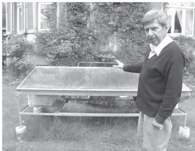
*Figure 4.* This picture shows the inventor with a F8-250 Compact Unit that carries all the parts needed to purify water virtually anywhere (decentralised).
