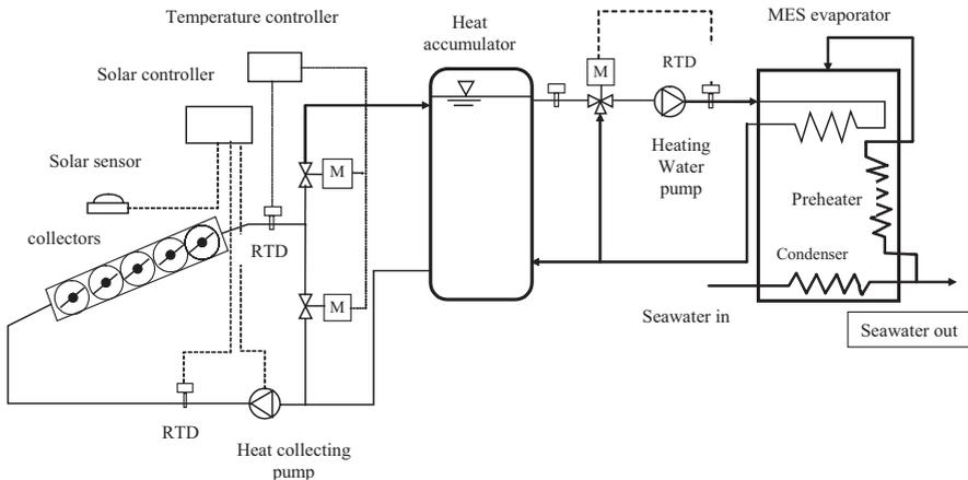
Figure 1. Schematic of the solar desalination system.
