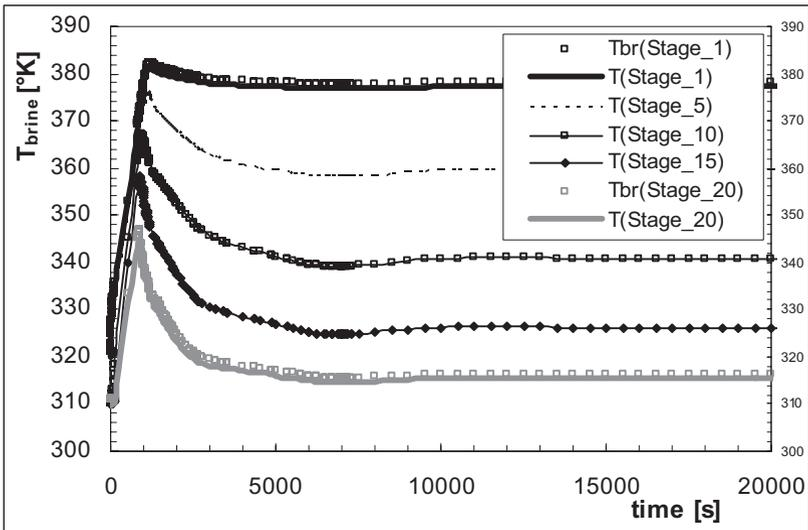
Figure 6. Temperature trends during start-up operations.
