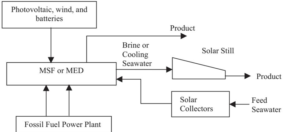
Figure 4. Hybrid of solar stills, collectors, and conventional desalination.
