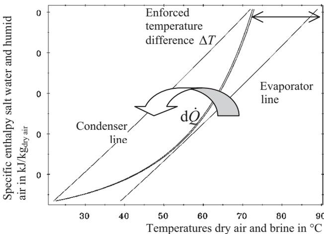
Figure 2. Heat and mass transfer in a system without adapted volume flows.
