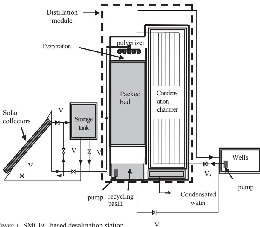
Figure 1. SMCEC-based desalination station.
