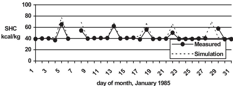
Figure 6. Daily average evaporator specific heat consumption (SHC) for January.
