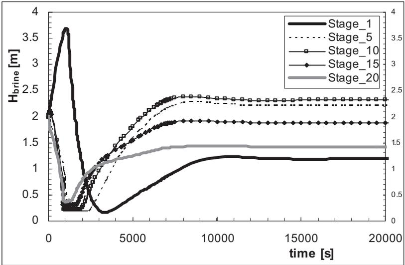
Figure 7. Brine level trends during start-up operations.
