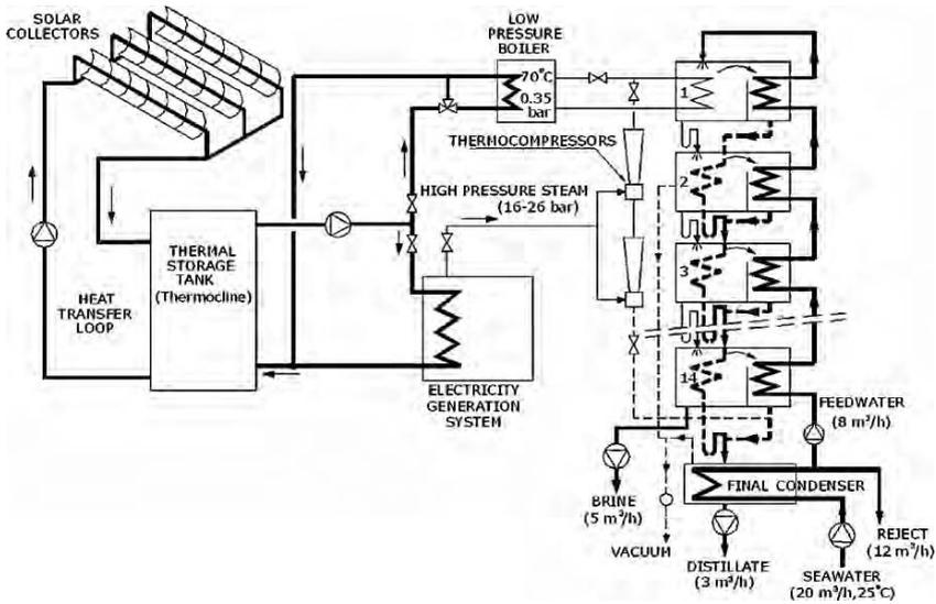
Figure 1. Schematic diagram of the solar MED system installed at PSA at Phase I of STD Project.
