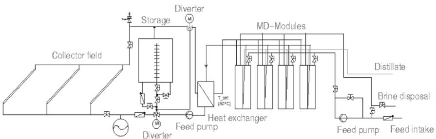
Figure 7. System set up of a two-loops system set up in Aqaba, Jordan.
