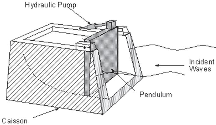
Figure 12. Pendulor device Source: EC ATLAS Project.
