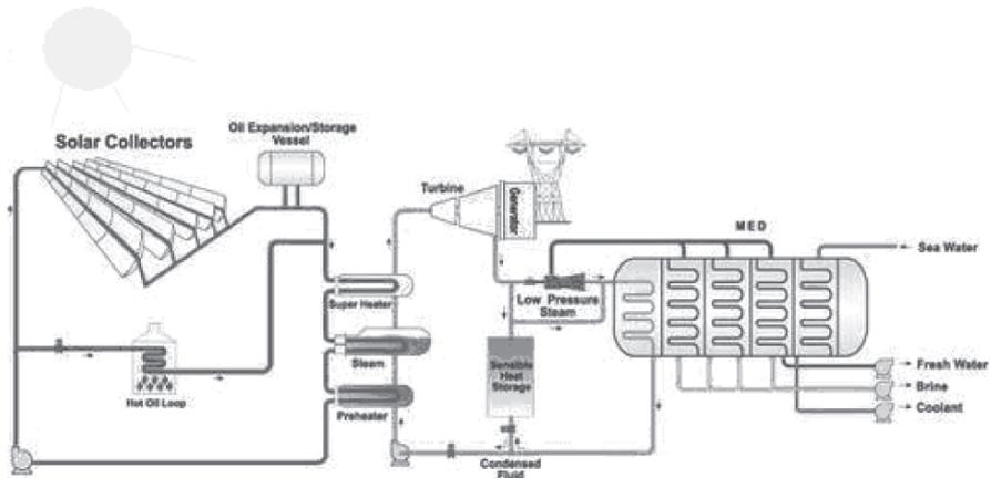
Figure 3. Scheme of a solar field coupled to a MED system.
