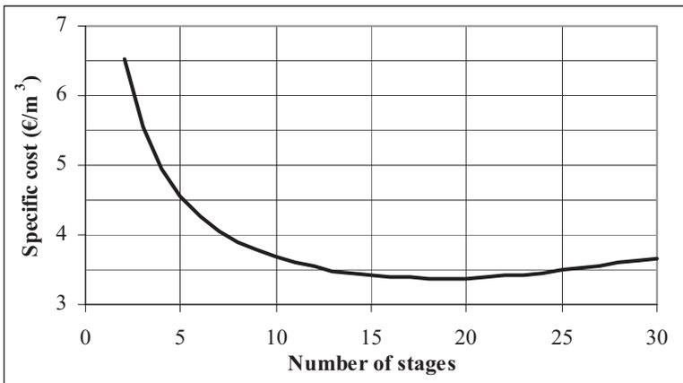
Figure 8. Cost of the desalted water as a function of the number of stages in MSF-M section.
