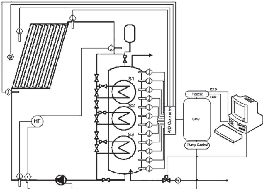
Figure 5. Sketch of the solar thermal system and heat accumulator tank with stratified layers supplied electrically by the PV system at the SWU “Neofit Rilsky” in Blagoevgrad, Bulgaria.
