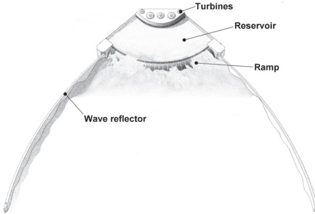
Figure 17. Wave dragon device. Source: Wave Dragon ApS.
