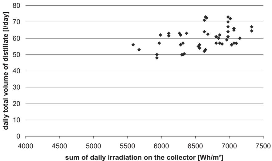
Figure 6. Daily volume of distillate produced by the compact system installed in Alexandria, Egypt (Data from August to October 2005).
