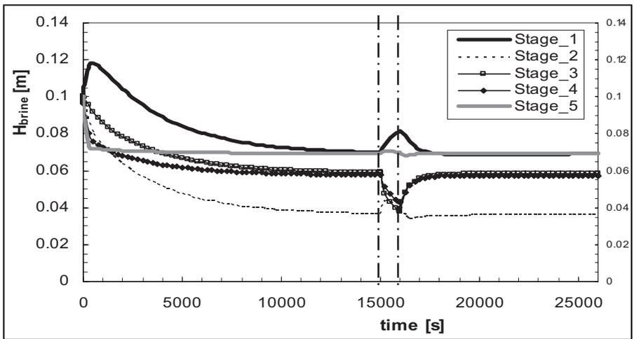
Figure 13. Trends in brine levels in the stages after the introduction of a leakage in the third stage for 1000s.
