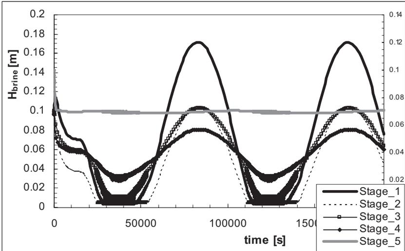
Figure 15. Trends of brine levels in the stages with an oscillating inlet brine temperature.
