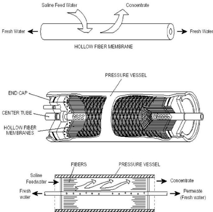
Figure 3. Pressure Vessel with Hollow Fibre Membrane Assembly<sup>2</sup> and Icon of Unit for RO Pressure Vessel in Model Development Kit.
