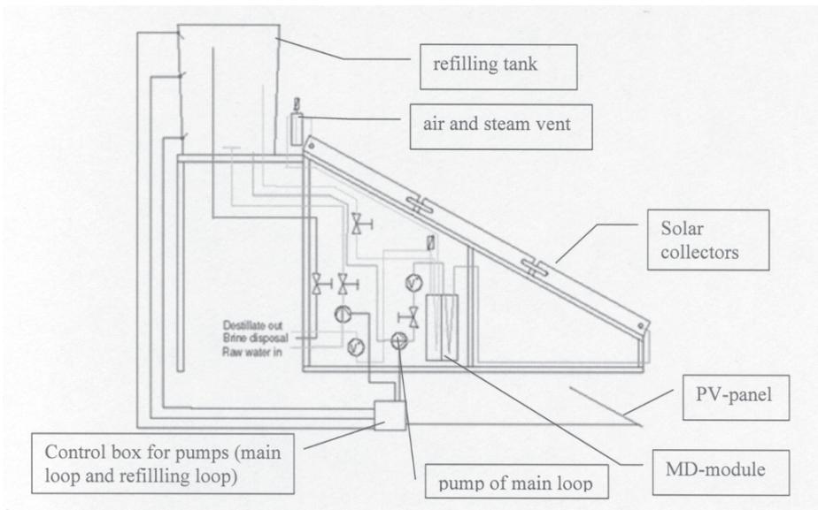
Figure 3. Schematic of the compact system.
