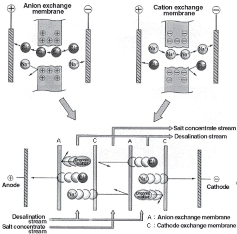
Figure 2. Principle of electrodialysis. Source: Astom Corporation.
