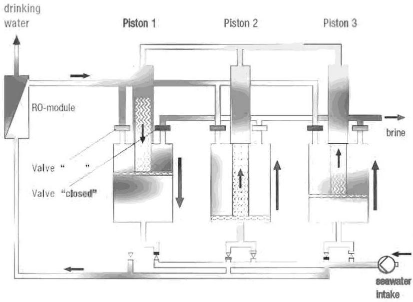
Figure 7. Enercon's energy recovery unit. Source: Enercon.
