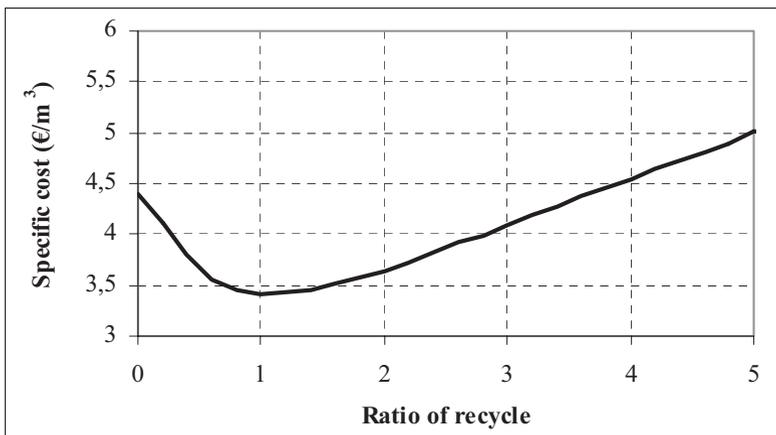
Figure 4. Specific cost of the desalted water as a function of the recycle ratio.
