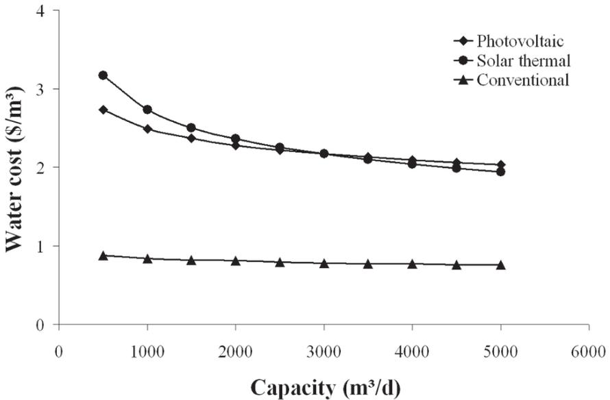
Figure 1. Water cost as a function of plant capacity by means of two solar systems (PV/RO and ST/MEE) and a conventional one.
