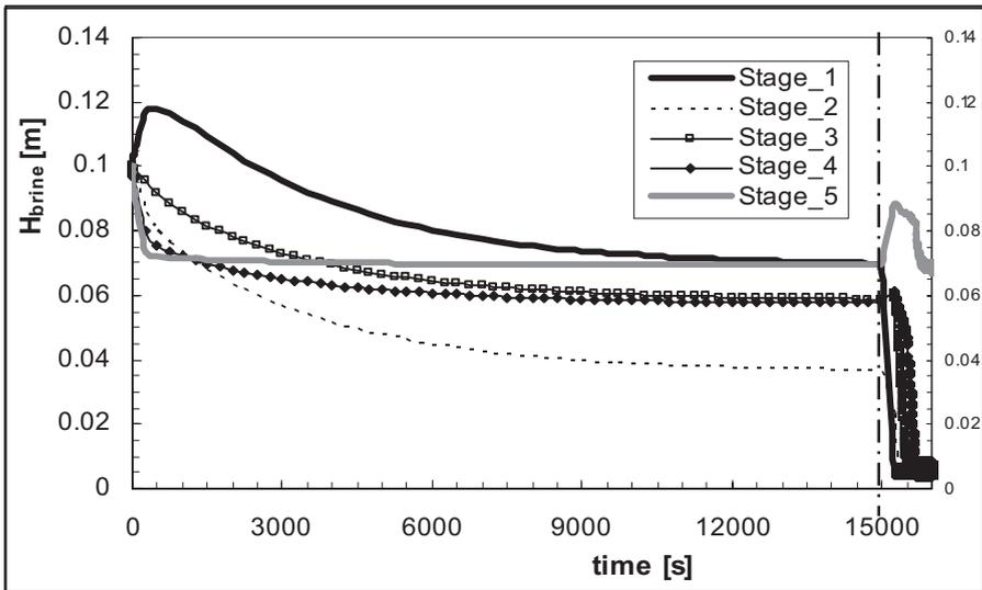
Figure 10. Trends in brine levels in the stages after a 10°K increase of inlet brine temperature.
