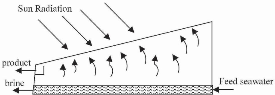
Figure 2. Schematic of simple solar still.
