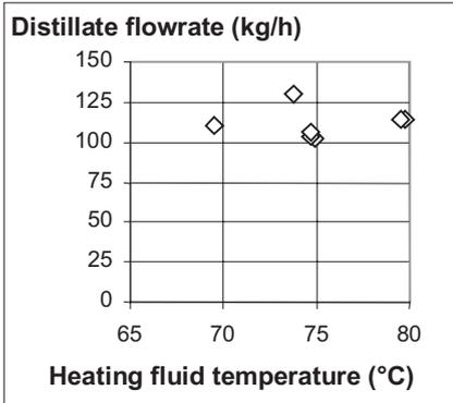
Figure 4. Variation of calculated distillate flowrate with heating fluid temperature for  $Q_h = 7 \text{ m}^3/\text{h}$ .
