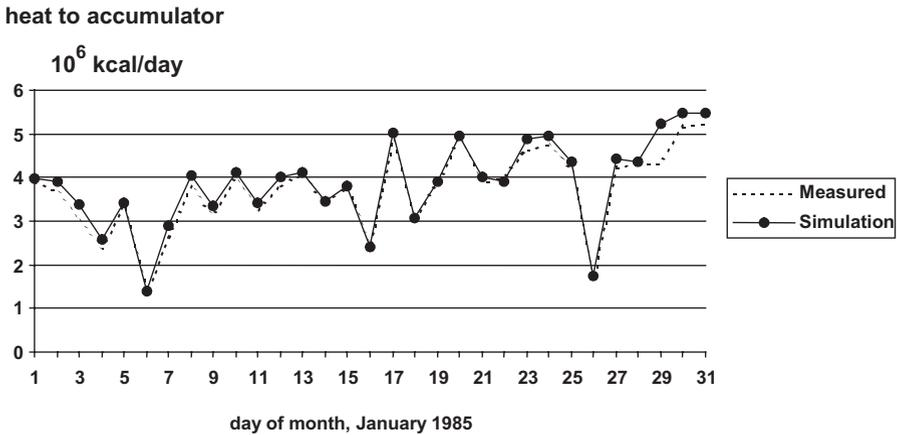
Figure 4. Daily heat supply to accumulator: comparison between measured and simulation results for January.
