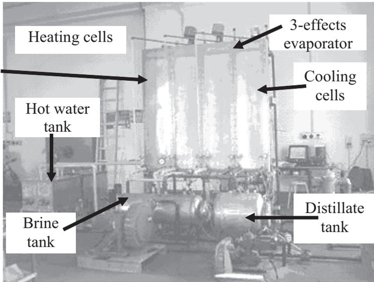
Figure 3. Photograph of the experimental three-effect seaside unit.
