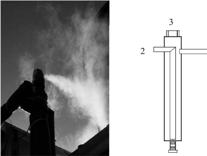
Figure 5. Sketch of the degasser (left) and photo during system stagnation. (2=inlet to degasser, 3=air and stem vent).
