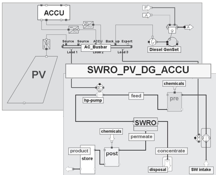
Figure 1. Integration of SWRO with Hybrid Energy Supply (PV and Diesel Generator).
