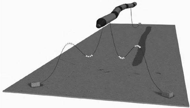
Figure 19. Pelamis device. Source: Ocean Power Delivery.
