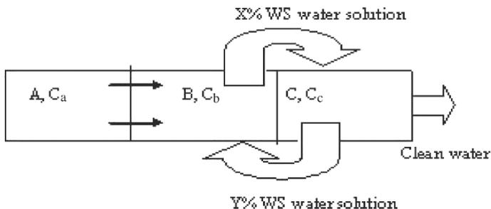
Figure 1. Principle of operation of direct osmosis desalination method (here  $Y > X$ ).
