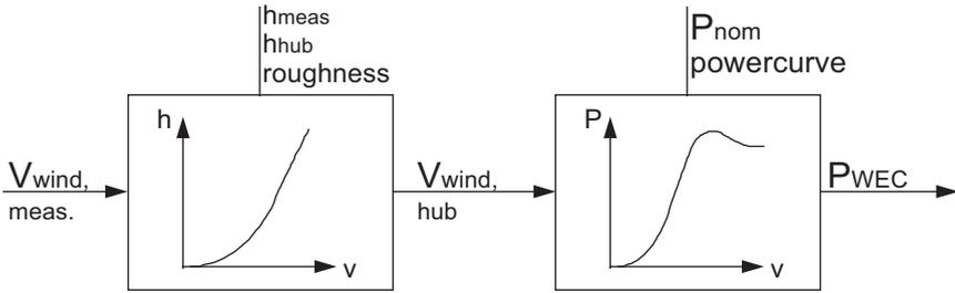
Figure 5. Modeling of Wind Energy Conversion in *RESYSproDESAL*.
