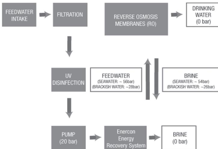
Figure 6. Basic functionality of Enercon's reverse osmosis desalination plant. Source: nercon.
