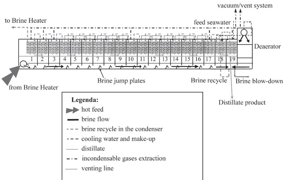
Figure 3. Sketch of a Brine Circulation MSF desalination unit.
