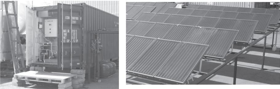
Figure 6. First commercial MEH-desalination unit produced by MAGE / TiNOX .
