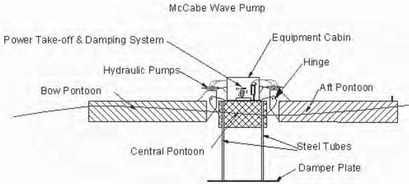
Figure 15. McCabe wave pump device. Source: Northern Ireland Assembly.
