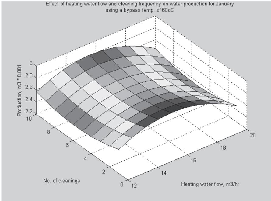
Figure 10. Effect of the number of collector cleanings and heating water flow for January using a bypass temperature of 60°C.
