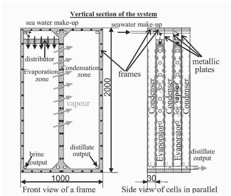
Figure 1. Front view and side view of elementary cells of EasyMED process (dimensions in mm).
