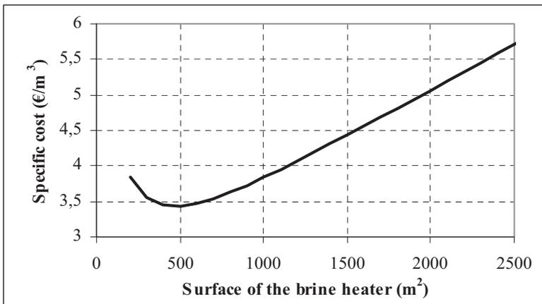
Figure 6. Specific cost as a function of the surface of the brine heater.
