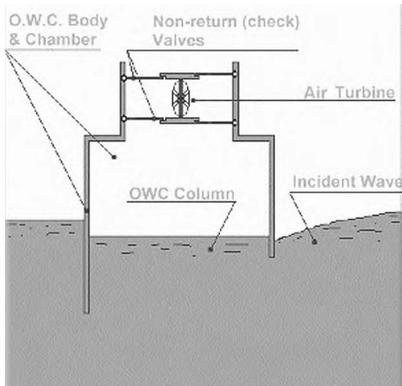
Figure 9. Oscillating water column device. Source: Daedalus Informatics Ltd.
