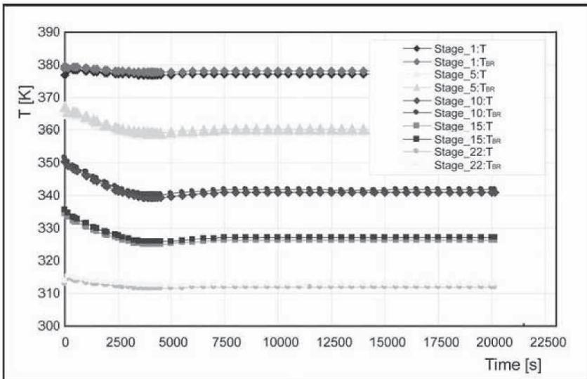
Figure 4. Brine and Vapour phase temperature trends in certain stages of the unit.
