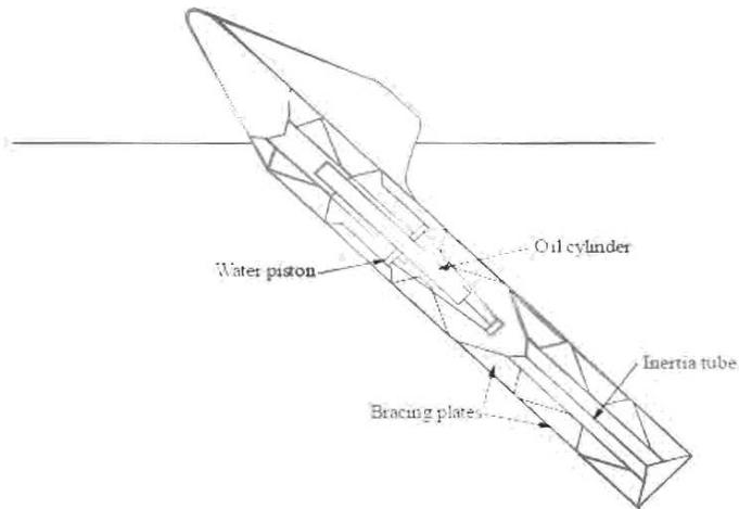
Figure 21. IPS Buoy device. Source: University of Edinburgh.
