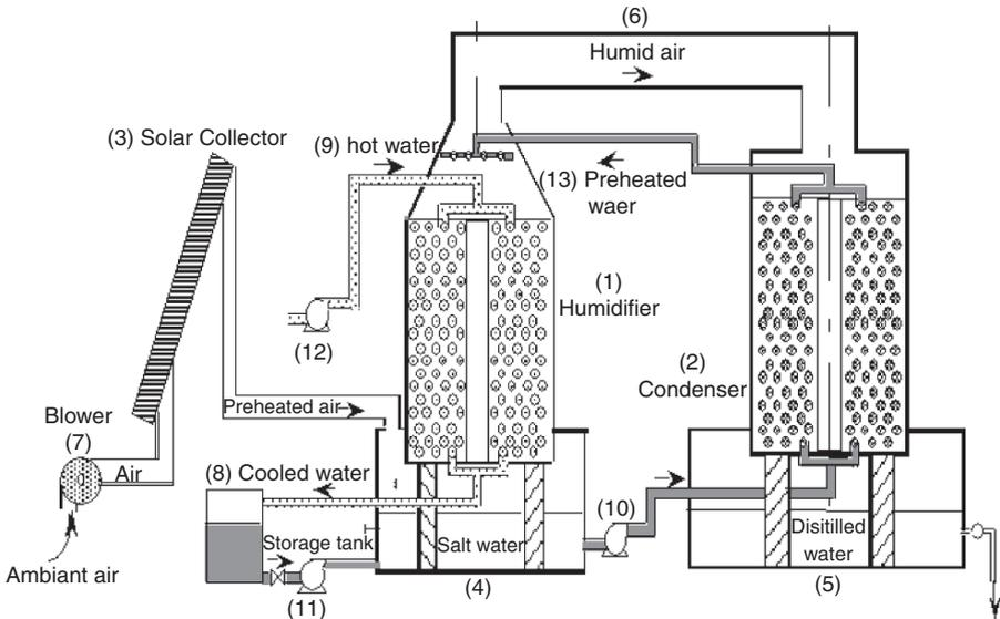
Figure 1. Presentation of the prototype functioning by the Aero-Evapo-Condensation process. (1) Humidifier; (2) Condenser; (3) Solar collector; (4) salt water tank; (5) distilled water tank; (6) pipe; (7) ventilator; (10) (11) and (12) pumps; (13) nozzle.
