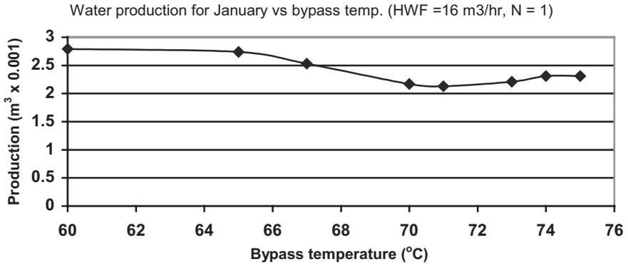
Figure 9. Effect of bypass temperature on water production for January.
