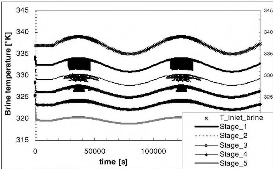
Figure 14. Trends of brine temperatures in the stages with an oscillating inlet brine temperature.
