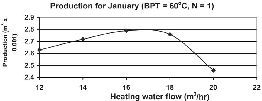
Figure 8. Effect of heating water flow (HWF) on January production. Bypass temp. (BPT) = 60°C and number of cleanings ( $N$ ) = 1.
