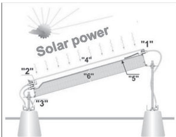
Figure 1. Detailed view of the Rosendahl collector and its working principle.
