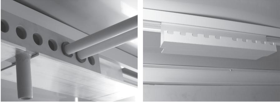
Figure 4. Interior installation components manufactured by CNC-moulding cutter.
