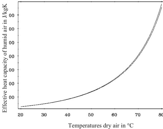
Figure 1. Effective heat capacity comprising latent and sensitive heat of a packet of saturated air at temperature T. Two lines arise due to reduced steam pressure over sea water
