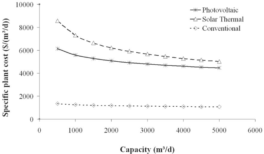
Figure 2. Specific plant cost as a function of plant capacity by means of two solar systems (PV/RO and ST/MEE) and a conventional one.
