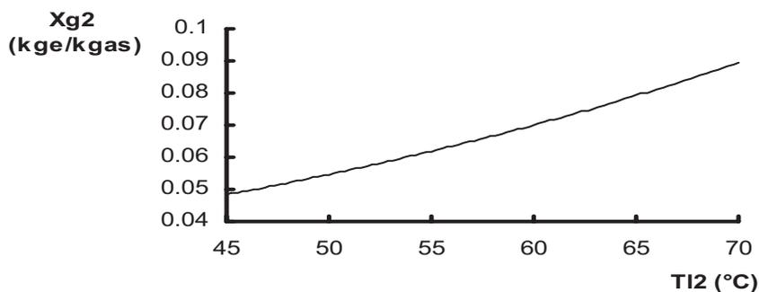
Figure 7. Impact of water temperature at the evaporation tower inlet on the air humidity (top of the evaporation tower).
