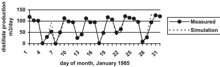
Figure 5. Comparison between measured and simulated distillate production, January.
