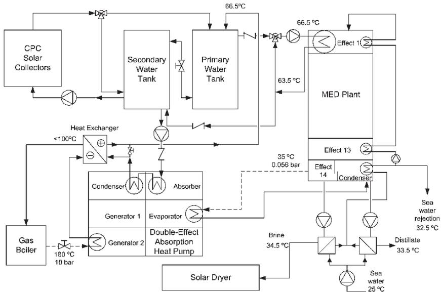
Figure 3. Final configuration proposed for AQUASOL seawater desalination system.
