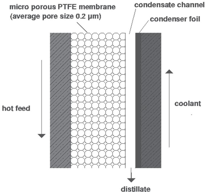
Figure 1. Principle of membrane distillation.
