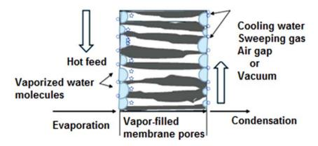
Figure 8.1 Basic working principles of MD (redrawn from [7])
