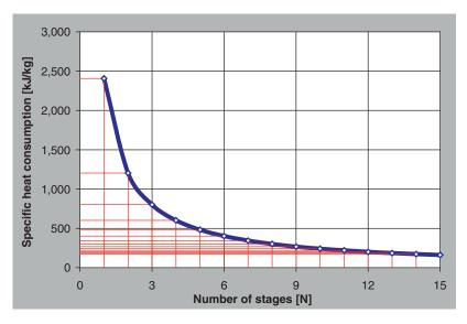
Figure 2.15 Specific heat consumption of a multiple- effect distillation plant.
