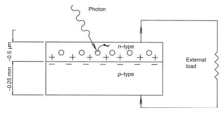
Figure 13.17 Photovoltaic cell schematics
