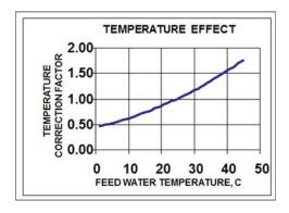
Figure 3.4 Water permeability temperature correction factor.
