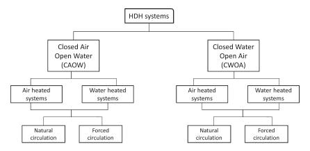
Figure 9.4 Classification of HDH systems based on cycle configurations [15].
