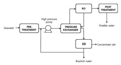
Figure 6.8 Integration of RO and ED for seawater desalination.
