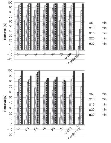
**Figure 12.4** Removal percentage of the heavy metals from electrolytes during experimental Runs #5 to #9 (top) and Runs #72 to 76 (bottom).
