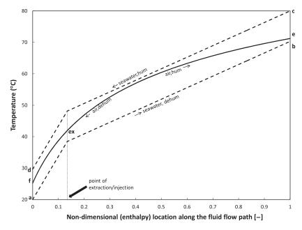
**Figure 9.18** Temperature profile representing the HDH system with a single extraction. Boundary conditions:  $T_a = 20^{\circ}$  C;  $T_c = 80^{\circ}$  C;  $T_{deh} = T_{hum} = 20^{\circ}$  KJ/kg dry air [28].
