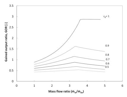
**Figure 9.9** Effect of component effectiveness of dehumidifier on performance of the WH-CAOW HDH cycle [22].
