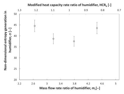
**Figure 9.20** Effect of mass flow rate ratio on non-dimensional entropy generation in the humidifier. Boundary conditions:  $T_e = 32^{\circ}\text{C}$ ;  $T_c = 60^{\circ}\text{C}$ ;  $T_{wb,e} = 20^{\circ}\text{C}$ ; P = 101.3 kPa;  $V_b = 0.27 \text{ m}^3[29]$ .
