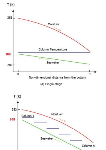
**Figure 9.25** An illustration of the temperature profile in the bubble columns for (a) single stage and (b) multi-stage [66].
