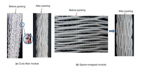
**Figure 8.8** Novel module design and fabrication: (a) curly-fiber module; (b) spacer-knitted module [52]
