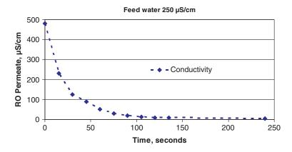
Figure 7.8 Flush up of RO system after standby
