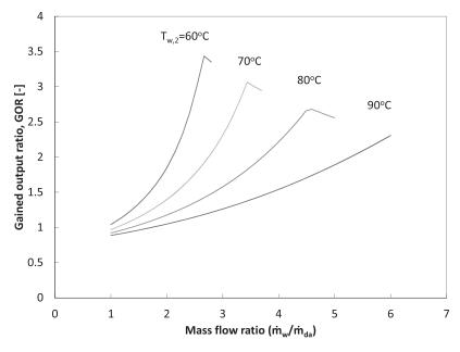
**Figure 9.10** Effect of top brine temperature on performance of the WH-CAOW HDH cycle [22].
