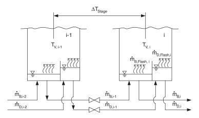
Figure 2.19 Illustration of the flashing process in a thermal desalination plant.
