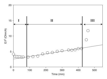
**Figure 6.6** Graph for the membrane fouling in ED process in the presence of an organic foulant (I: the period for the acclimation of foulant, II: the period for the fouling layer formation, III: the period for the concentration depletion).
