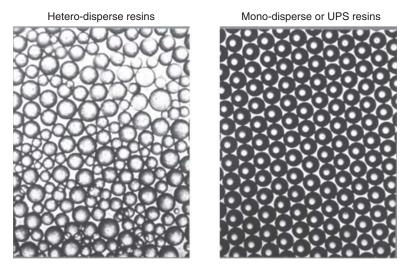
**Figure 11.8** Hetero-disperse and mono-disperse or uniform particle size (UPS) resins.
