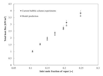
**Figure 9.23** Effect of inlet mole fraction of the vapor on the total heat flux in the bubble column measured and evaluated at Vg = 3.8 cm/s;  $D_b = 4 \text{ mm}$ ; H = 254 mm [66].
