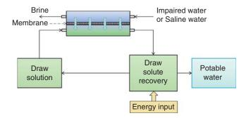
Figure 5.1 - Schematic of the generalized forward osmosis desalination process
