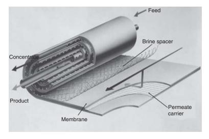
Figure 3.9 Configuration of spiral wound membrane element.
