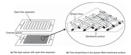
Figure 8.6 Net-type spacer design in flat-sheet membrane module [135]
