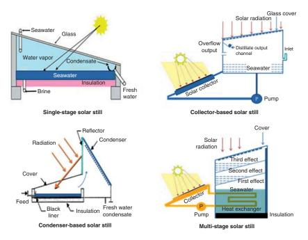
Figure 13.4 Different configurations of solar stills
