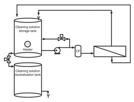
Figure 3.20 Configuration of membrane cleaning unit.
