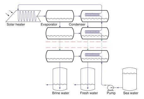
Figure 13.13 Multi-stage solar flash desalination system
