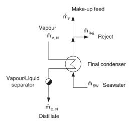
**Figure 2.22** Simplified flow sheet of the final condenser.
