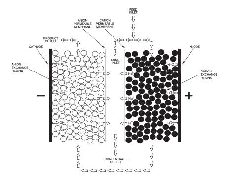
Figure 7.5 Removal mechanism in thick-cell, separate-bed CEDI cell
