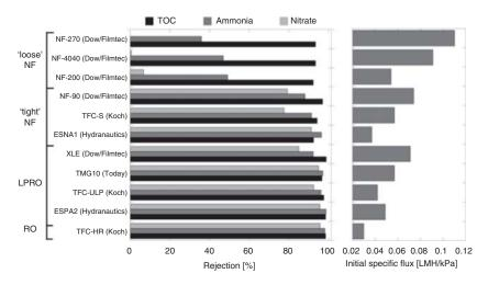
**Figure 4.5** Comparison of rejection performance (left) and pressure requirements (right, specific flux for 20 LMH permeate flux) between various RO, LPRO and NF membranes when treating microfiltered secondary effluent.
