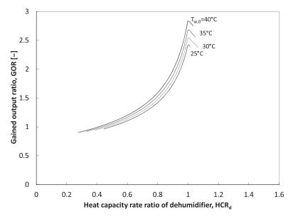
**Figure 9.14** HCR of dehumidifer versus GOR at various feedwater temperatures [22].
