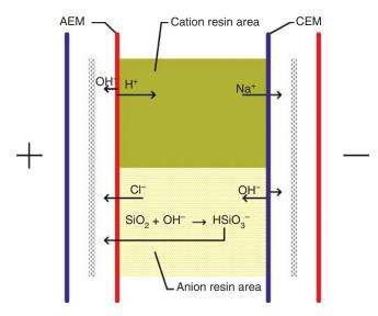
Figure 7.4 Removal mechanism in thick-cell, layered-bed CEDI cell
