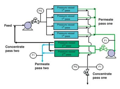
Figure 3.17 Schematic configuration of two pass RO unit.
