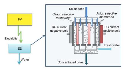
Figure 13.10 PV assisted electro-dialysis
