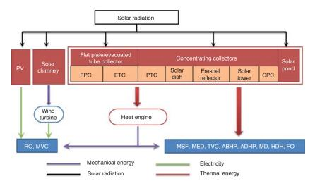
Figure 13.16 Possible solar desalination arrangements
