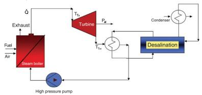
**Figure 2.43** 1. Condensation power station for electricity generation. 2. Steam generator for heat supply of a desalination plant. 3. Condensation power station with back pressure turbine for electricity generation and heat supply of a desalination plant.
