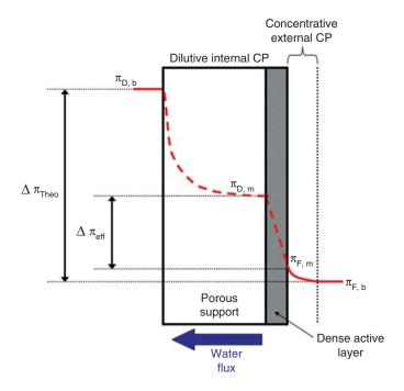
Figure 5.4 – Illustration of concentration polarization phenomenon near the active (selective) layer of the membrane.  $\pi$  refers to the osmotic pressure of the solution.  $\Delta\pi$  is indicative of the osmotic driving force across the membrane while the subscripts "Theo" and "eff" refer to the theoretical and effective driving force, respectively. Subscripts D, F, m, and b refer to the "draw", "feed", "selective layer interface", and "bulk" osmotic pressures, respectively
