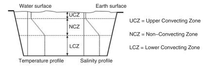
Figure 13.3 Vertical cross section of a solar pond
