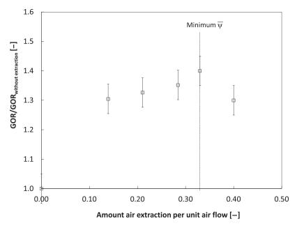
**Figure 9.21** Effect of mass flow rate of air extracted on the performance of the HDH system. Boundary conditions:  $T_a = 25^{\circ}$  C;  $T_c = 90^{\circ}$  C; N = 1;  $= 0.27 \text{ m}^3$ ;  $A_d = 8 \text{ m}^2[29]$ .
