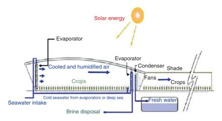
Figure 13.15 Solar assisted seawater greenhouse
