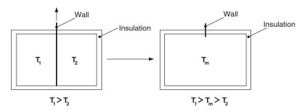
**Figure 2.5** Irreversible mixing as an example for the second rule of thermodynamics.
