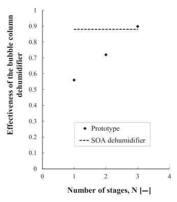
**Figure 9.26** Effect of multistaging the bubble column on energy effectiveness of the device.
