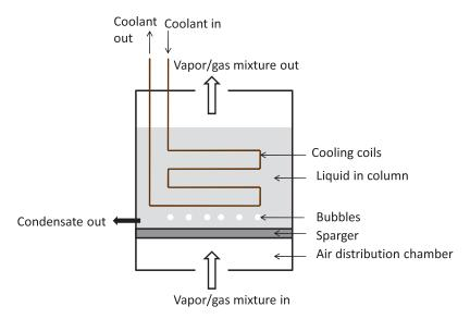
Figure 9.22 Schematic diagram of the bubble column dehumidifier [66].
