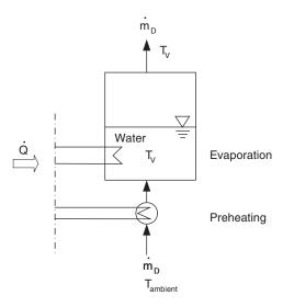
**Figure 2.4** Flow scheme of an evaporation process with preheating.
