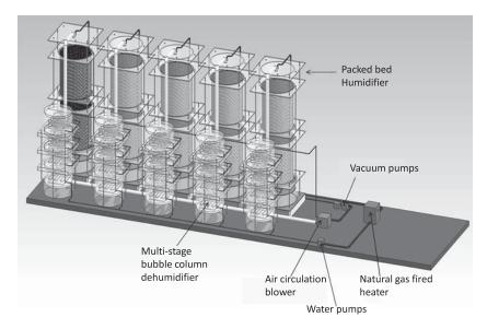
**Figure 9.28** Three-dimensional model of a trailer-mounted, sub-atmospheric-pressure, natural-gas-fired, single air extraction HDH system with a 12 foot tall packed bed humidifier and a four-stage bubble column dehumidifier [73].
