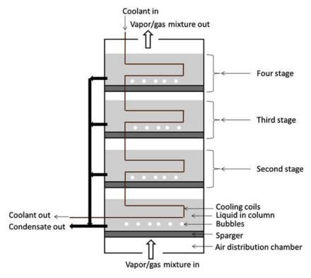
Figure 9.24 Schematic diagram of multi-stage bubble column dehumidifier [66].
