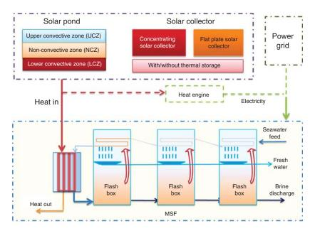
Figure 13.5 Solar assisted multi-stage flash desalination
