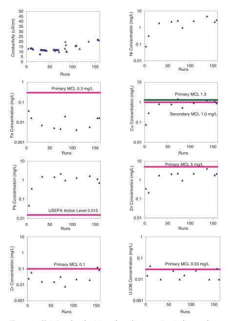
**Figure 12.5** Variation of conductivity and metal concentrations in the treated electrolyte solutions throughout the 158 runs (setpoint: 500 ohms, corresponding to 25–30 minutes contact time).
