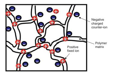
**Figure 6.2** Schematic diagram of the structure of an anion exchange membrane structure.
