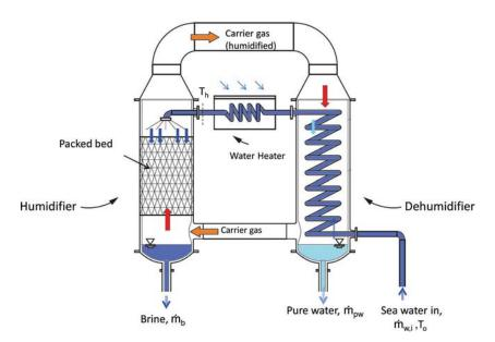
Figure 9.3 Simplest embodiment of HDH process [17].
