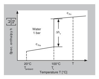
**Figure 2.3** Enthalpy – temperature diagram for water.
