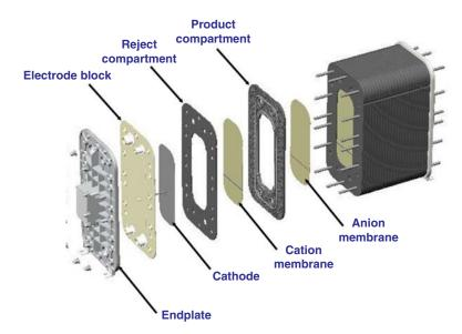
Figure 7.2 Plate-and-frame CEDI device
