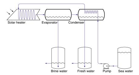
Figure 13.12 Single-stage solar flash desalination system
