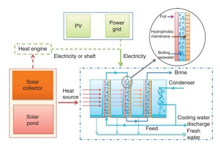
Figure 13.11 Solar driven membrane distillation
