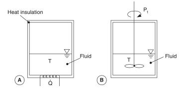
Figure 2.1 First rule of thermodynamics (Closed system).
