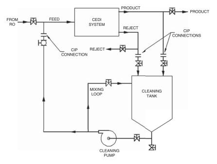
Figure 7.11 Typical CIP apparatus
