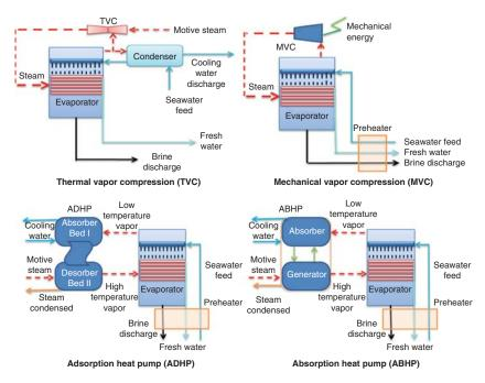
Figure 13.7 Different configurations of heat pumps
