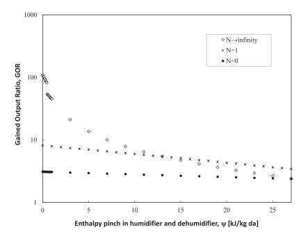
**Figure 9.19** Effect of number of extractions (for thermodynamic balancing) on the performance of the HDH system with finite and infinite size HME devices. Boundary conditions:  $T_a = 20^{\circ}$  C; sal = 35 g/kg;  $T_c = 80^{\circ}$  C;  $HCR_{deh} = 1$  [28].
