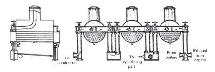
Figure 2.51 Rillieux's multiple-effect evaporator (1846)[12].
