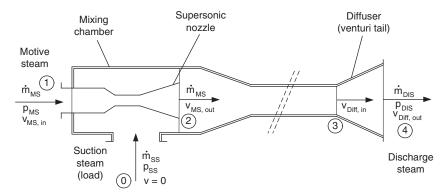
Figure 2.32 Scheme of a thermal vapour compressor.
