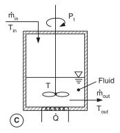
Figure 2.2 First rule of thermodynamics (Open system).
