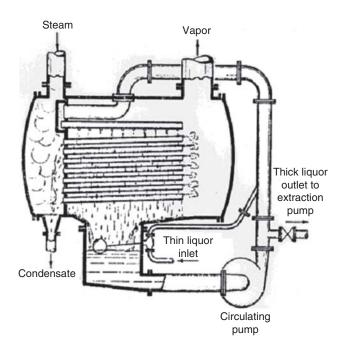
**Figure 2.53** Horizontal tube sprayed film evaporator S. Morris Lillie Sugar Manufacturing Company Philadelphia 1888 [15].
