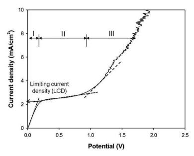
**Figure 6.4** Determination of the limiting current density in a graph between supplied potential and corresponding current. (I: Electrical resistance increased due to Ohm's law, II: Boundary layer resistance increase, III: Over-limiting current density).
