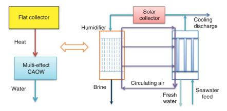
Figure 13.14 Solar assisted multi-effect CAOW system
