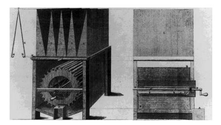
**Figure 2.50** Gautier's evaporation equipment (1720)[11].
