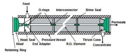
Figure 3.11 Configuration of pressure vessel with membrane elements.
