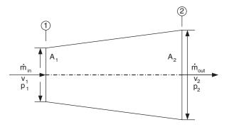
Figure 2.33 Schematic representation of a diffuser
