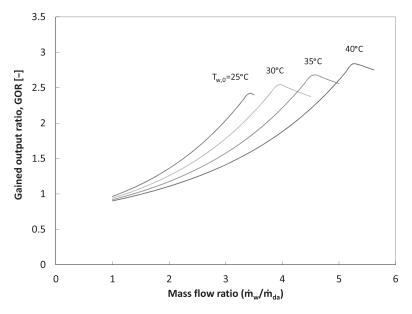
**Figure 9.13** Effect of feedwater temperature on performance of the WH-CAOW HDH cycle [22].
