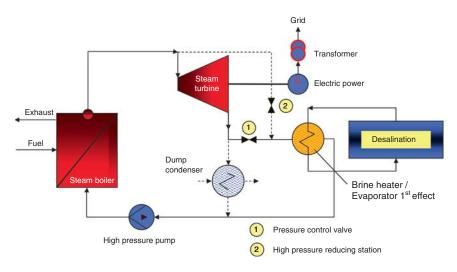
Figure 2.42 Dual purpose plant / Case 1: Back pressure turbine.
