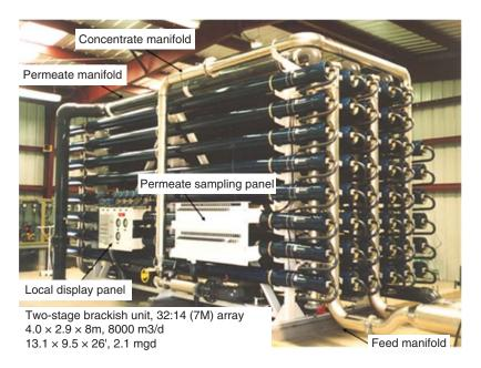
Figure 3.16 Two stage RO unit. Permeate capacity about 8,000 m3/day (2.1 mgd)
