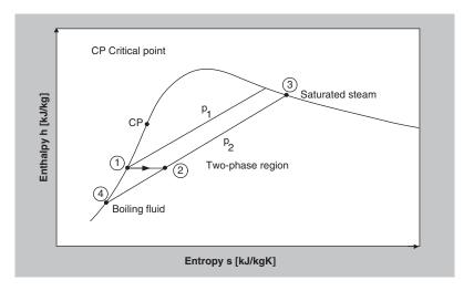
Figure 2.18 Enthalpy-entropy (h-s) diagram for flash evaporation process.
