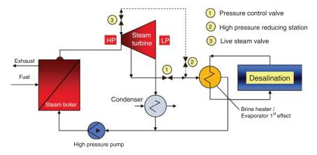
Figure 2.44 Dual purpose plant / Case 2: Controlled extraction steam turbine.
