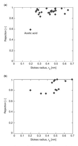
**Figure 4.4** Rejection of negatively charged (top) and positively charged (bottom) organic solutes by a NF membrane as a function of Stokes radius at a permeate flux of 20 LMH and pH of 6.5.
