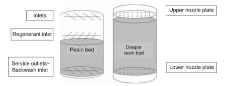
Figure 11.7 Conventional vessel and packed bed vessel.
