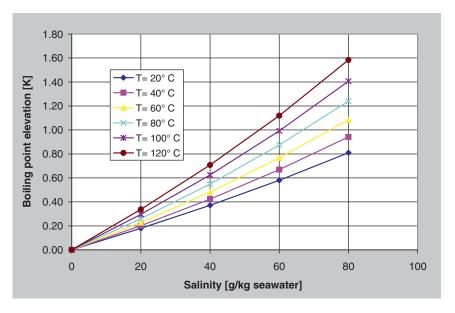
Figure 2.8 Boiling point elevation as a function of salt content and temperature[1].
