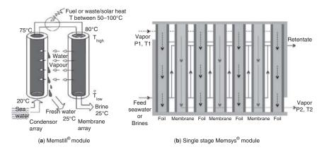
Figure 8.7 Working principles of (a) Memstill [28] and (b) Memsys [27] MD modules
