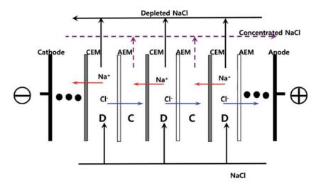
**Figure 6.1** Schematic diagram of the typical arrangement in an ED process (CEM: Cation exchange membrane, AEM: Anion exchange membrane, D: Diluate compartment, C: Concentrate compartment).
