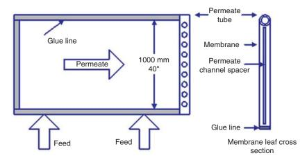
Figure 3.8 Configuration of flat sheet membrane leaf.
