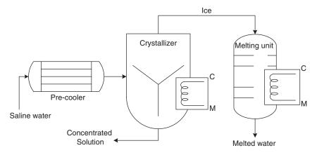
**Figure 10.1** Freezing-Melting (FM) process showing pre-cooler, crystallizer, and melting unit.
