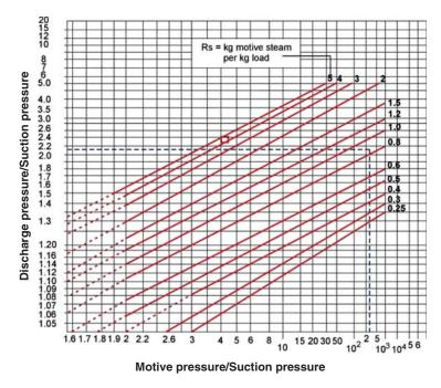
Figure 2.36 Performance diagram for a thermal vapour compressor.
