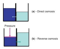
**Figure 3.1** The direct and reverse osmosis process.
