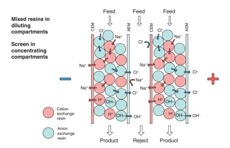
Figure 7.1 Ion transport and electrochemical regeneration in a CEDI cell
