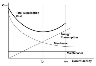
**Figure 6.5** ED desalination cost as a function of the current density ( $i_{op}$ : operating current density,  $i_{tim}$ : limiting current density).
