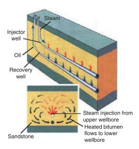
Figure 14.11 Schematic of SAGD process (source: http://pubs.usgs.gov/fs/ fs070-03/fig3.jpg).
