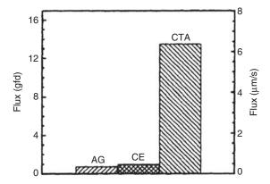
Figure 5.2 – Flux performance of 2 commercially available RO membranes from GE Water (AG, CE) and a cellulose triacetate forward osmosis membranes from Hydration Technology Innovations (CTA). The draw solution used was a 6M ammonia-carbon dioxide solution and the feed solution was a 0.5M sodium chloride solution. The temperature of the test was 50°C. Reprinted from [48]. Tests were done in a custom built crossflow benchtop FO testing system.
