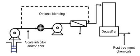
Figure 3.12 Configuration of RO system processing well water.
