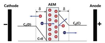
**Figure 6.3** Concentration polarization occurring on the surface of an anion exchange membrane (Co(D): Concentration in the bulk solution of diluate compartment, Co(C): Concentration in the bulk solution of concentrate compartment).
