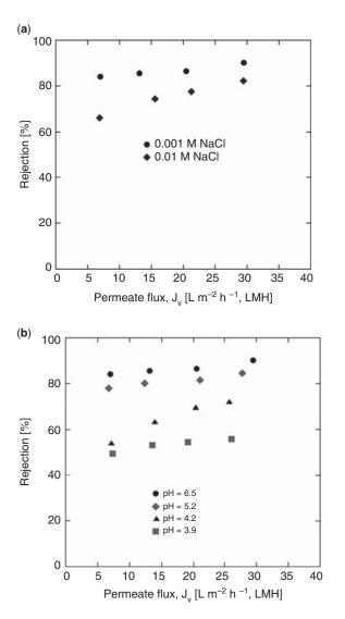
**Figure 4.2** NaCl rejection by an NF membrane for a NaCl solution as a function of permeate flux and concentration (top) and permeate flux and pH (bottom, 0.001 M NaCl).
