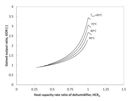
Figure 9.11 HCR of dehumidifer versus GOR at various top brine temperatures [22].
