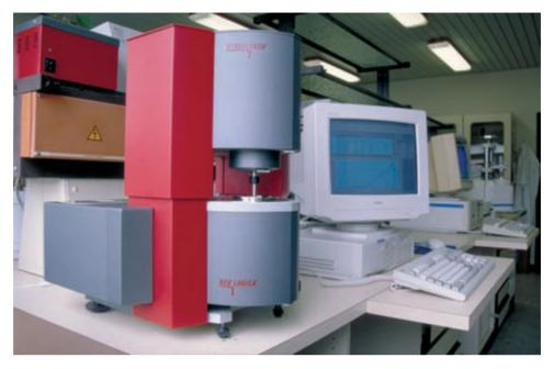
**Plate 5** Stresstech CS rheometer for controlled stress viscosity measurement. With permission of Danisco A/S, Brabrand, Denmark, and Reologica, Sweden.
