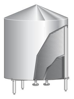
Fig. 5.9 Tubular holding unit. By permission of Tetra Pak AB, Lund, Sweden.
