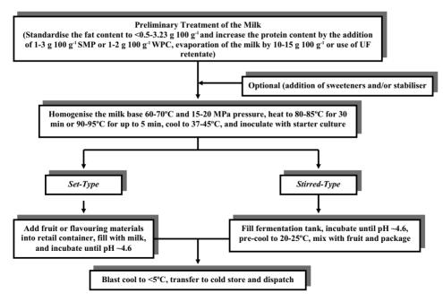
Fig. 3.1 Main processing stages during the manufacture of set and stirred yoghurt.
