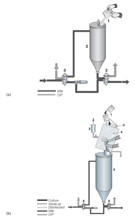
**Fig. 2.9** In-line inoculation system using concentrated freeze-dried or frozen cultures. (a) -1, Starter culture package; 2, Mixing container; 3, Mix-proof valves. (b) -1, Starter culture package; 2, Disinfectant container; 3, Sight glass; 4, Inoculation 'box'; 5, Mixing container; 6, Mix-proof valves. By permission of Tetra Pak AB, Lund, Sweden.
