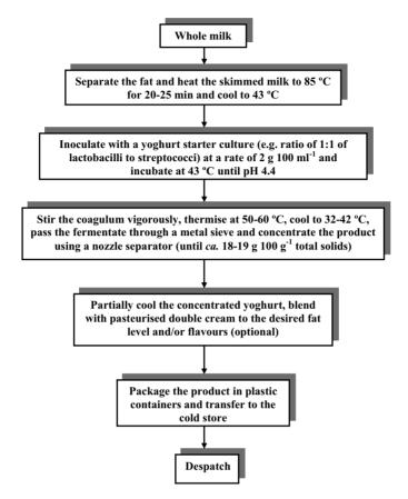
Fig. 6.3 Production of concentrated yoghurt using the nozzle separator method.
