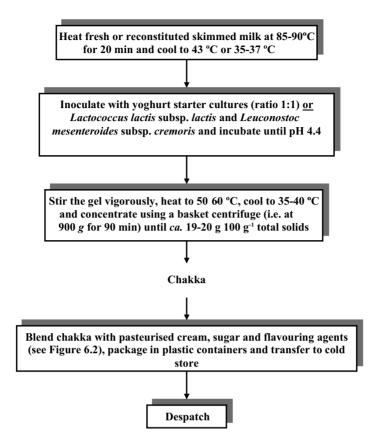
Fig. 6.7 Production line for shrikhand using basket centrifuge.
