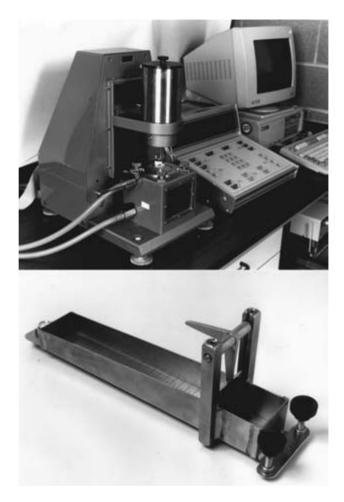
**Fig. 4.2** (a) The dynamic rheometer (Rheo Tech International, Surrey, UK) is capable of discriminating between gels of different strengths, while (b) the Bostwick Consistometer (Christison Particle Technologies, Gateshead, UK) is a typical simple device that can be employed to obtain an objective comparison of the viscosities of samples of stirred fruit yoghurt.
