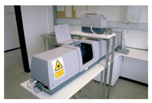
**Plate 4** The Malvern Mastersizer for measuring of particle size distribution. With permission of Danisco A/S, Brabrand, Denmark.
