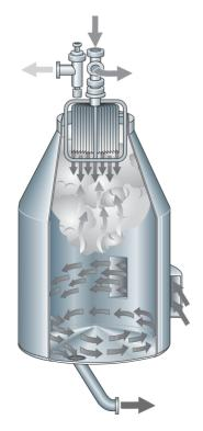
Fig. 5.8 Flow of milk and air in the vacuum deaerator with built-in condenser. By permission of Tetra Pak AB, Lund, Sweden.
