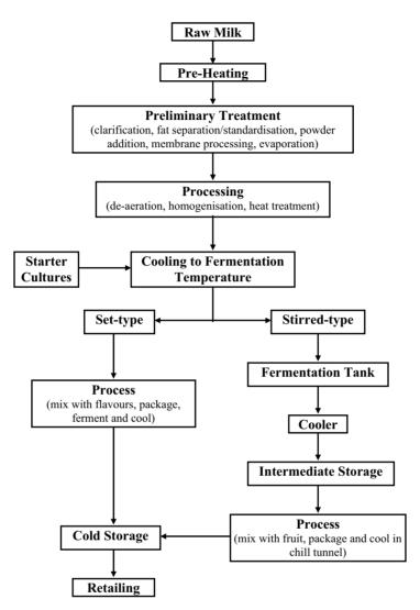
Fig. 1.1 Flow diagram showing the manufacturing stages of fermented milk products.
