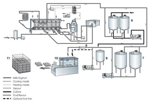
**Fig. 3.4** Production line for set yoghurt. 1, Bulk starter culture tanks; 2, buffer tanks; 3, fruit/flavour tank; 4, in-line mixer; 5, filling machine; 6, incubation. By permission of Tetra Pak AB, Lund, Sweden.
