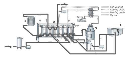
**Fig. 3.2** Flow diagram of general pre-treatment of milk for the manufacture of set and stirred yoghurt. 1, Balance tank; 2, plate heat exchanger (PHE); 3, evaporator; 4, homogeniser; 5, holding tube. By permission of Tetra Pak AB, Lund, Sweden.
