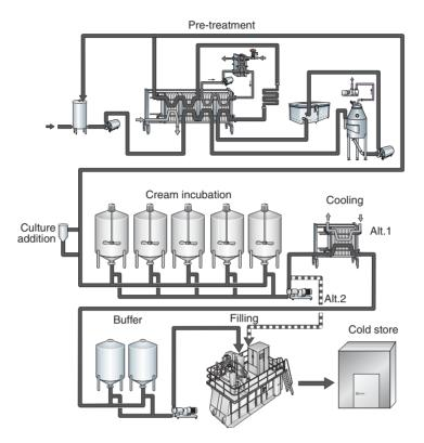
Fig. 9.1 Production lines for stirred- and set-types of cultured cream for cold distribution. By permission of Tetra Pak AB, Lund, Sweden.
