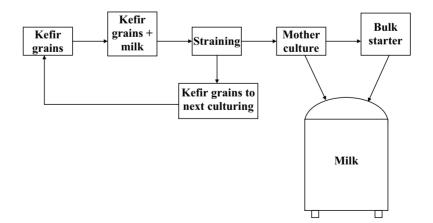
Fig. 8.7 Production stages for kefir grain preparation and the manufacture of kefir.
