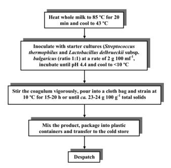
Fig. 6.1 Generalised scheme illustrating the different stages of the production of traditional labneh.
