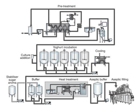
**Fig. 5.12** Production of stabilised long-life drinking yoghurt for storage at ambient temperature. By permission of Tetra Pak AB, Lund, Sweden.
