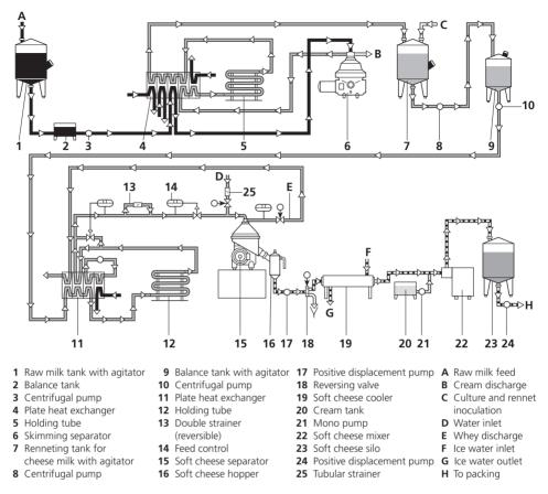
**Fig. 6.4** Illustration of a typical thermo-soft cheese plant that can be used for the production of concentrated yoghurt. By permission of GEA-Westfalia Separator AG, Oelde, Germany.
