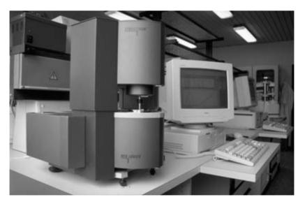
**Fig. 5.16** Stresstech CS rheometer for controlled stress viscosity measurement. With permission of Danisco A/S, Brabrand, Denmark and Reologica, Sweden. Reproduced in colour as Plate 5, after page 110.
