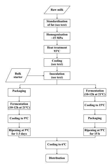
Fig. 8.9 Generalised scheme for the industrial production of kefir using kefir 'wash' or fermentate as a starter culture.
