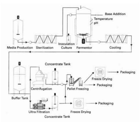
**Fig. 2.8** Production of a typical commercial starter culture. Redrawn from Høier, E., Janzen, T., Henriksen, C.M., Rattray, F., Brockmann, E. & Johansen, E. (1999) The production, application and action of lactic cheese starter cultures. *Technology of Cheesemaking* (ed. B.A. Law), pp. 99–131, Sheffield Academic Press, Sheffield. By permission of Sheffield Academic Press, Blackwell Publishing, and Chr. Hansen A/S, Hørsholm, Denmark.
