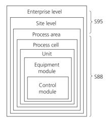
Fig. 10.2 Illustration of the structure used to model an enterprise according to specific standards (ANSI/ISA-S88 and ANSI/ISA-S95). By permission of Tetra Pak processing system AB, Lund, Sweden.
