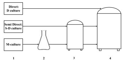
Fig. 8.8 Flow diagram for the industrial production of kefir using different types of cultures. 1, Lyophilised starter culture; 2, mother culture; 3, bulk starter culture; 4, kefir.
