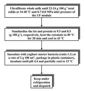
Fig. 6.8 Production of labneh from UF whole-milk retentates.
