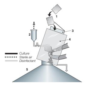
**Fig. 2.10** Hygienic inoculation system fitted on top of a fermentation or bulk starter culture tank. 1, Starter culture package; 2, disinfectant container; 3, sight glass; 4, inoculation 'box'; 5, incubation or bulk starter culture tank. By permission of Tetra Pak AB, Lund, Sweden.
