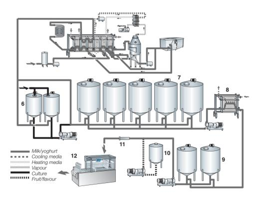
**Fig. 3.3** Production line for stirred yoghurt. 1, Bulk starter culture tanks; 2, incubation/fermentation tanks; 3, plate cooler; 4, buffer tanks; 5, fruit/flavour tank; 6, in-line mixer; 7, filling machine. By permission of Tetra Pak AB, Lund, Sweden.
