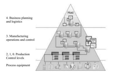
**Fig. 10.1** Overview of the different levels of automation in a yoghurt/food production line. By permission of Tetra Pak processing system AB, Lund, Sweden.
