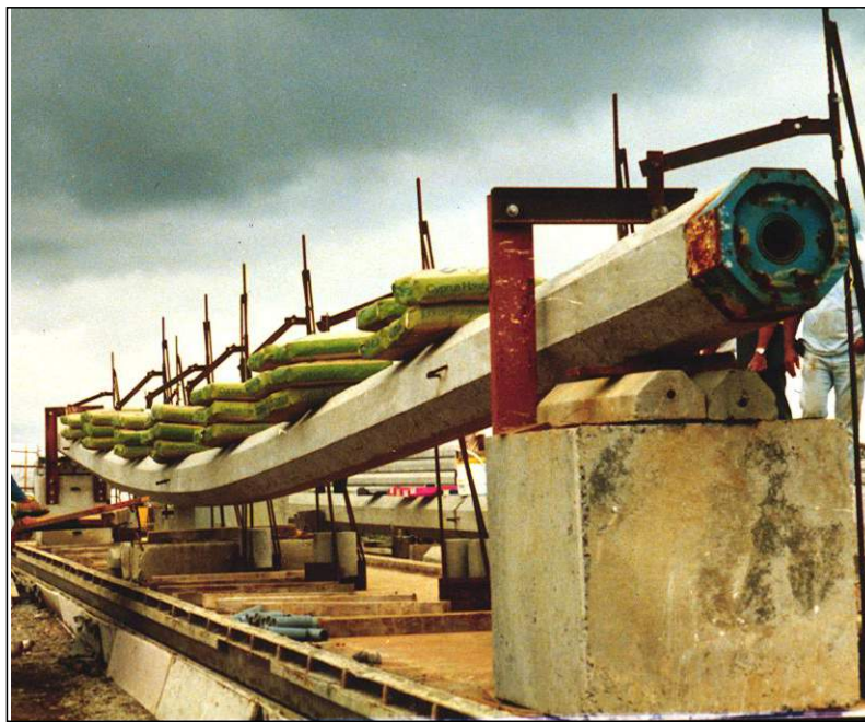
Fig. 7.40 Verifying the principle of the curvature probe
