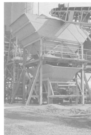
FIG. 9.A.2—Overhead aggregate bins with weighing hopper below.
