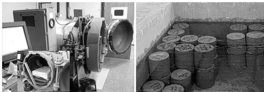
FIGURE 3.2 Steam and water curing of RPC.
