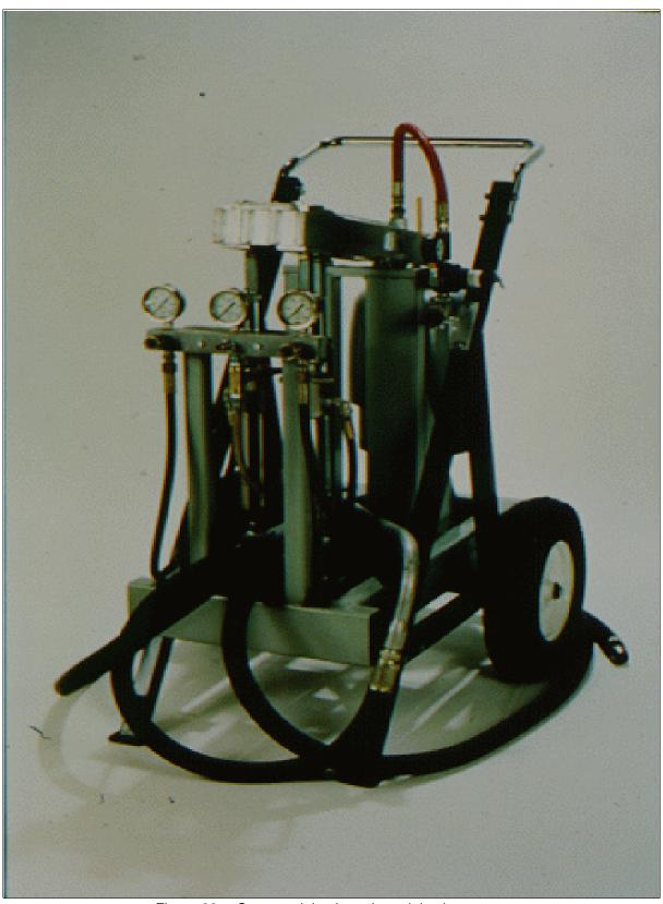
Figure 63.—Commercial polyurethane injection pump.
