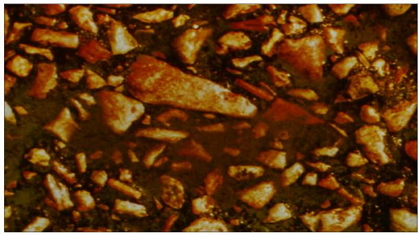
Figure 24.—Abrasion-erosion damage caused by sand or silt.
