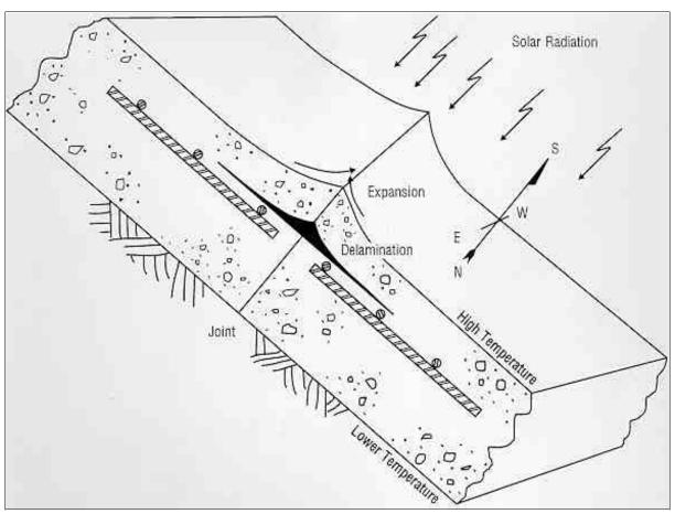
Figure 17.—Delamination caused by solar expansion.
