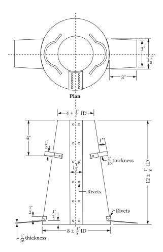
**Figure 19** Mold for slump cone. Copyright ASTM. Reprinted with permission.
