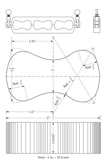
Figure 7 Briquet gang mold and specimen. Copyright ASTM. Reprinted with permission.
