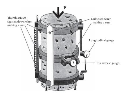
Assembly of the compressometer-extensioneter and the specimen. After the data is obtained, the device is removed and the concrete cylinder is loaded to failure.
