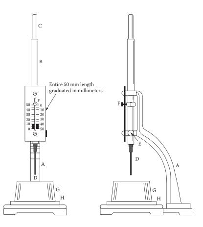
Vicat Apparatus. Copyright ASTM. Reprinted with permission.
