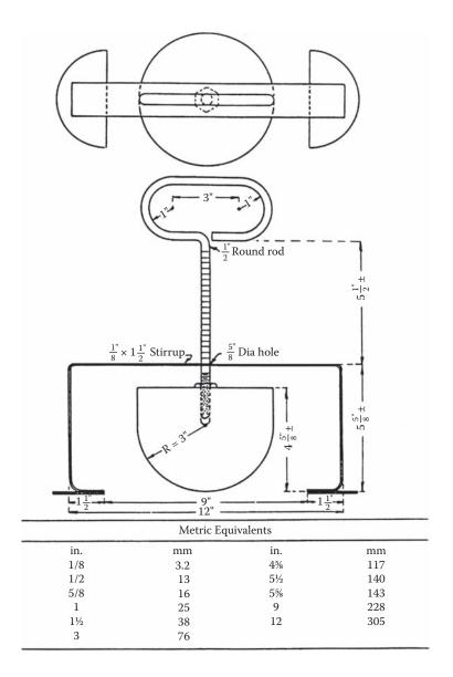
Ball penetration apparatus and metric equivalents. Copyright ASTM. Reprinted with permission.
