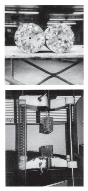
Figure 44 Photographs of a tension specimen after failure.
