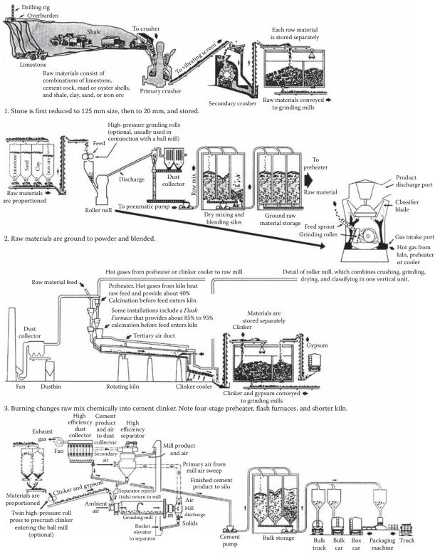
4. Clinker with gypsum is ground into portland cement and shipped.
