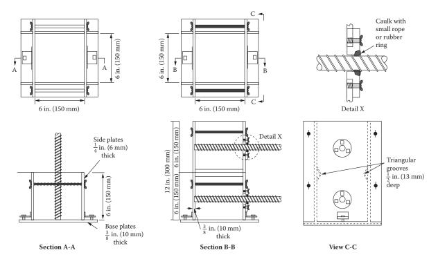
Molds for bond specimens. Copyright ASTM. Reprinted with permission.
