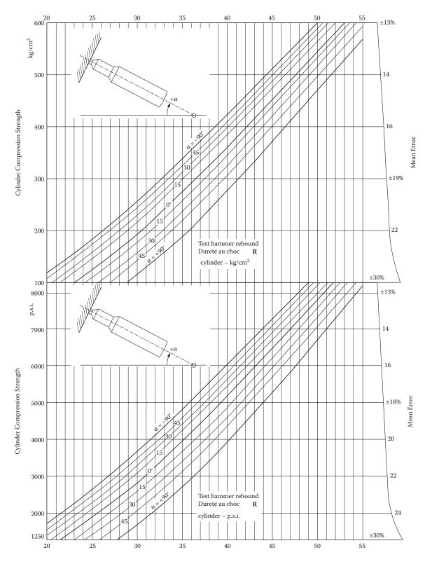
(a) Typical impact hammer calibration curves. Courtesy of ELE International, Inc., Soiltest Products Division, Lake Bluff, Illinois.(b) Hammer in portable carrying case. Courtesy of Soiltest, Inc.
