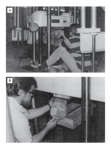
Top photograph showing the specimen being positioned in the testing machine. The bottom photograph was taken after the concrete specimen was loaded to failure and was being removed from the test apparatus with the fracture indicated.
