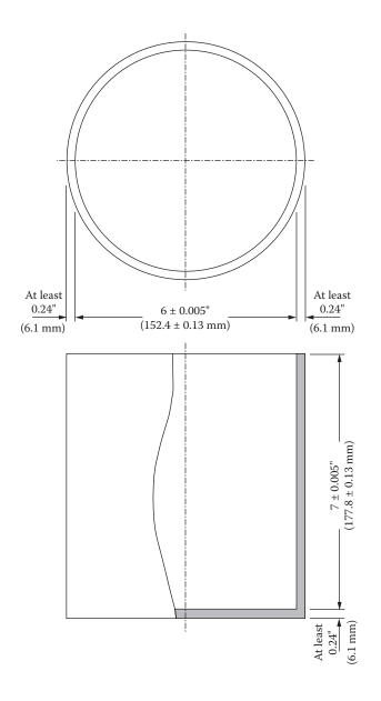
Cylindrical mold. Copyright ASTM. Reprinted with permission.
