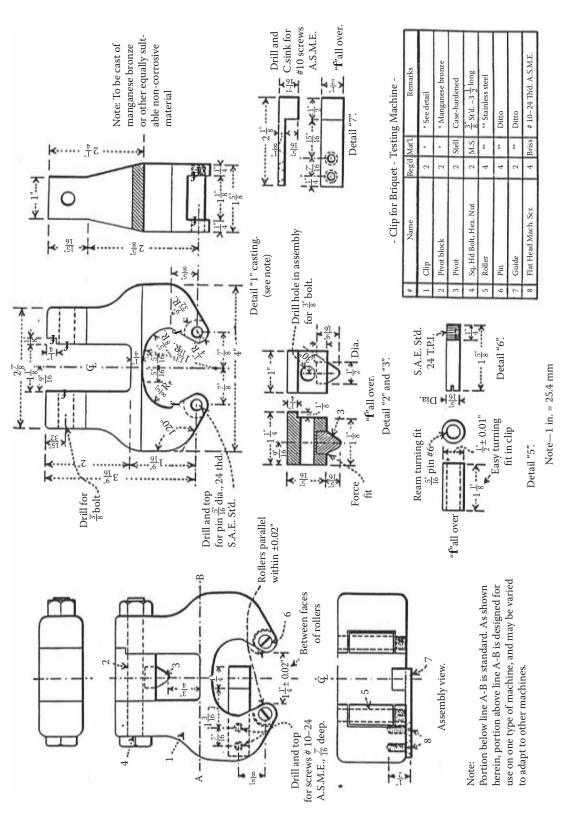
Figure 8 Clips for briquet testing machine. Copyright ASTM. Reprinted with permission.
