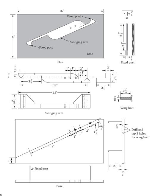
Details of the proportional caliper (drawings are not to scale).
