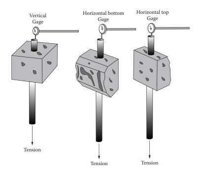
Schematic of bond Test Procedure, showing the differences in the concrete configuration for vertical, horizontal bottom, and horizontal top RE-bars due to the way the specimens are cast.
