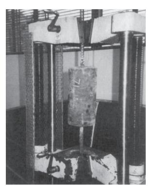
**Figure 43** Cylindrical tension specimen in the testing machine.
