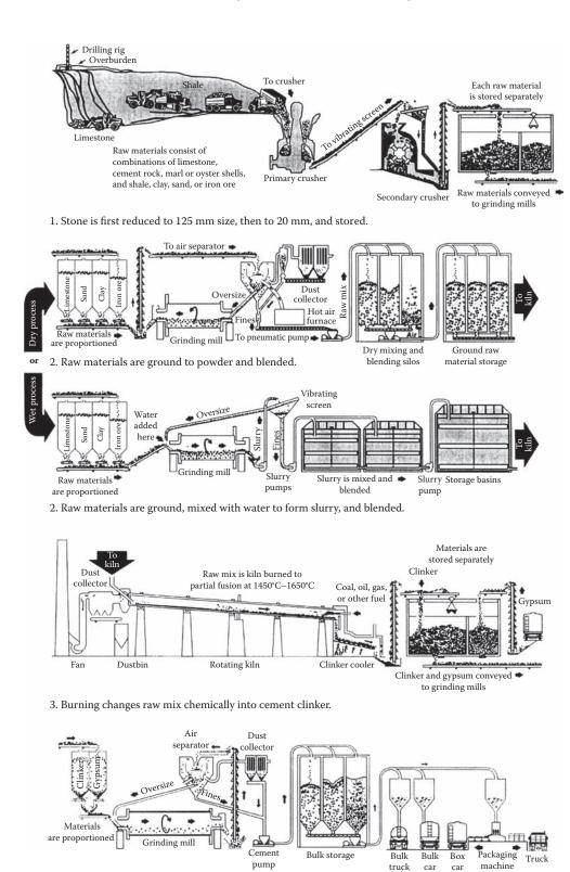
4. Clinker with gypsum is ground into cement and shipped.
