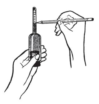
Chace air indicator shown being used to determine the approximate air content of fresh concrete. Reprinted with permission of the Canadian Portland Cement Association.
