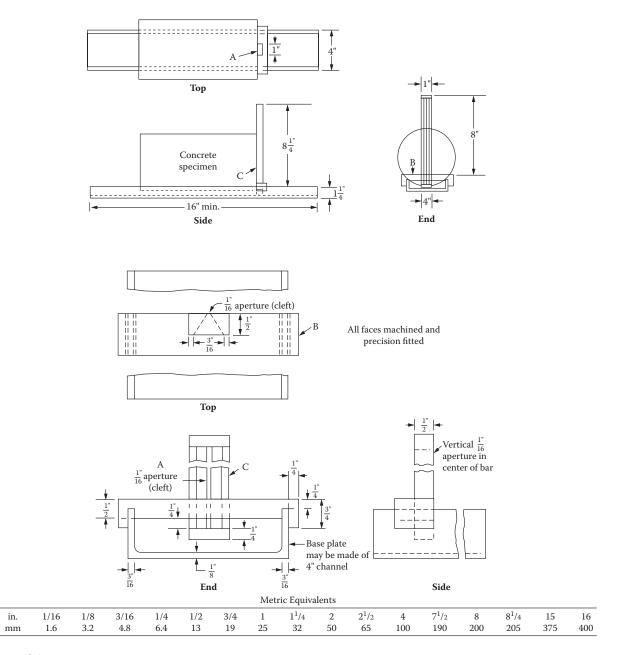
Details of an apparatus for aligning a specimen. Copyright ASTM. Reprinted with permission.
