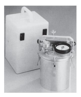
Photograph of a type B air meter, sheet 1 of 3. Courtesy of ELE International, Inc., Soiltest Products Division, Lake Bluff, Illinois.
