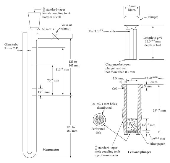
Blaine air permeability apparatus. Copyright ASTM. Reprinted with permission.
