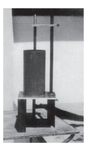
Photograph and sketch of fixture and RE-bar for concrete test specimens. Deformed RE-bar = 1 cm ( $\frac{1}{10}$  in.) diameter. Drill to obtain close to a No. 6 bar or 2-cm diameter fit about 3 cm or  $\frac{1}{10}$  in. in depth.
