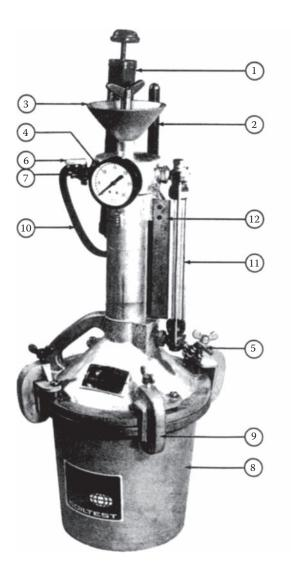
Diagram of a type A air meter: (1) hand pump, (2) tamping rod, (3) funnel and thumb valve, (4) pressure gauge, (5) petcock (drain), (6) petcock (air), (7) snifter valve, (8) container, (9) clamps and thumb screws, (10) hose attachment, (11) water glass, (12) graduated scale. Courtesy of ELE International, Inc., Soiltest Products Division, Lake Bluff, Illinois.
