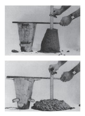
**Figure 20** Demonstration of the use of a slump cone. The top photograph illustrates a low slump and the bottom a high slump. Reprinted with permission of the Canadian Portland Cement Association.
