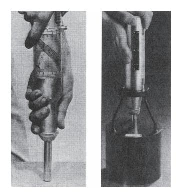
Photographs showing the impact hammer in operation in the vertical position, directed downward, and the calibration anvil for the impact hammer in the right photograph. Courtesy of ELE International, Inc., Soiltest Products Division, Lake Bluff, Illinois.
