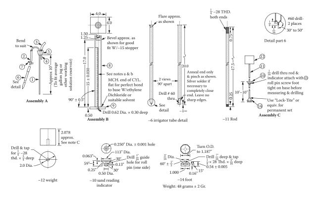
Sand equivalent test apparatus. Copyright ASTM. Reprinted with permission.
