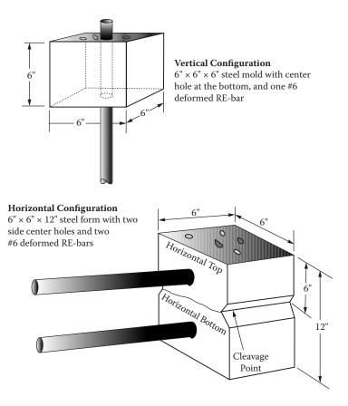
Figure 26 Schematic of bond specimens.
