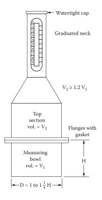
Volumetric apparatus for measuring the air content of fresh concrete.
