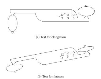
Use of the proportional calipers in testing for particle shape.
