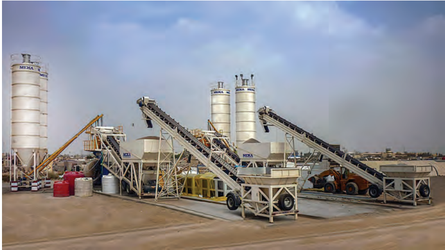
FIGURE 10.10 Aggregates transition system to the mixer by using of conveyor belt. (“MOBILE CONCRETE BATCHING PLANT mekaglobal”)
