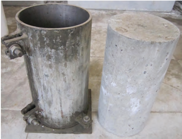
FIGURE 1.14 Standard 15 × 30 cm cylinder mold and specimen. (Photograph by the author.)
