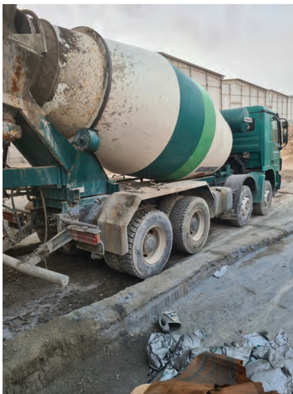
FIGURE 5.9 You may transport concrete for a long distance with truck mixers. (Photograph by the author.)
