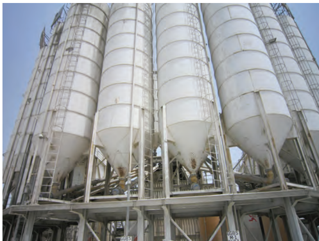
FIGURE 10.5 Cement and other binder storage. (Photograph by the author.)
