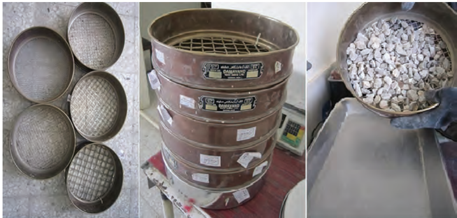
FIGURE 4.28 Sieves for the coarse aggregates and the amount remained after shaking. (Photograph by the author.)
