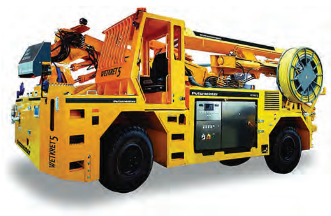
FIGURE 5.2 Tunnel shotcrete device. (“Putzmeister Wetkret 5.”)
