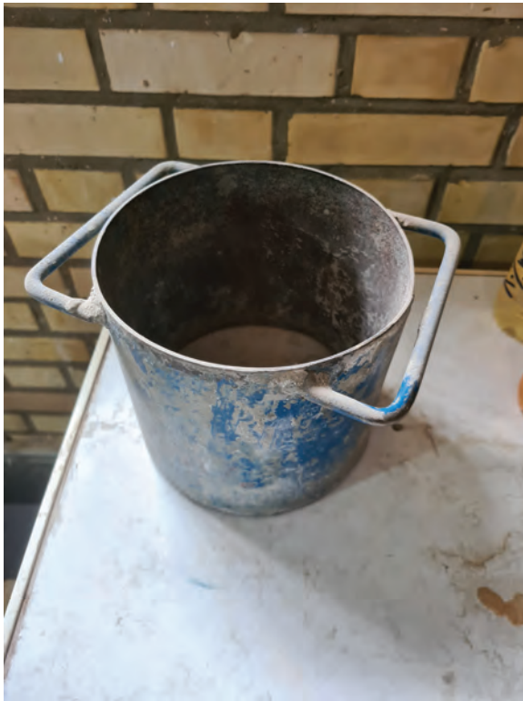
FIGURE 7.7 Container with defined volumes for the test of density. (Photograph by the author.)
