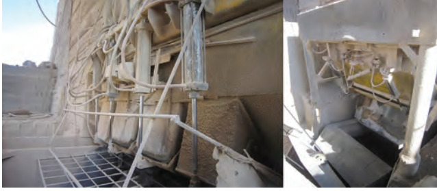
FIGURE 10.8 Aggregate weighing system with different pneumatic valves. (Photograph by the author.)
