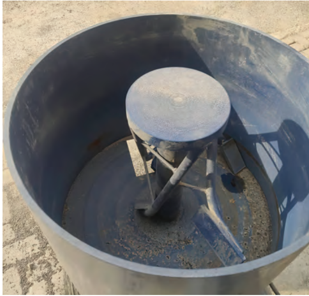
FIGURE 13.19 Pan mixer, suitable for the production of RPC. (Photograph by the author.)
