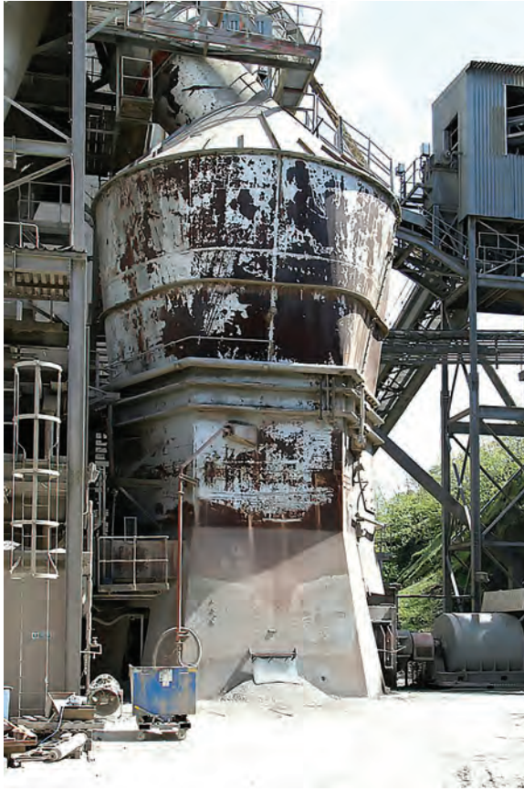
FIGURE 2.11 Picture of a roller mill. This is for the raw materials, but similar ones can be used for cement. (“Hanson Cement, Clitheroe” by Alan Murray-Rust.)
