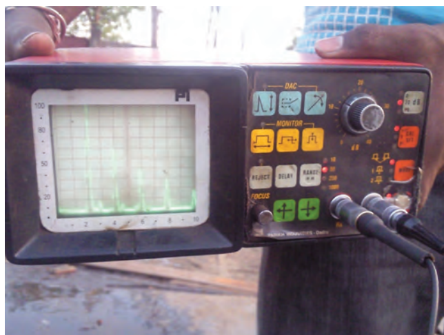
FIGURE 7.19 Multipurpose ultrasonic test instrument. (“Ultrasonic Testing Machine showing readings” by Abhijit Nandi used under a Creative Commons Attribution-Share Alike 3.0 Unported license.)
