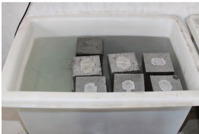
FIGURE 7.18 Concrete specimens immersed in water. (Photograph by the author.)
