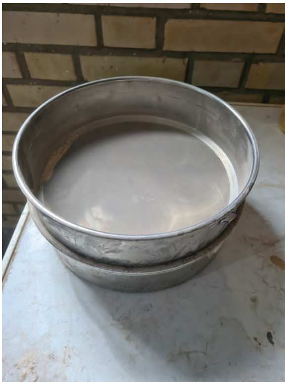
FIGURE 2.14 Sieve for cement particle size testing. (Photograph by the author.)
