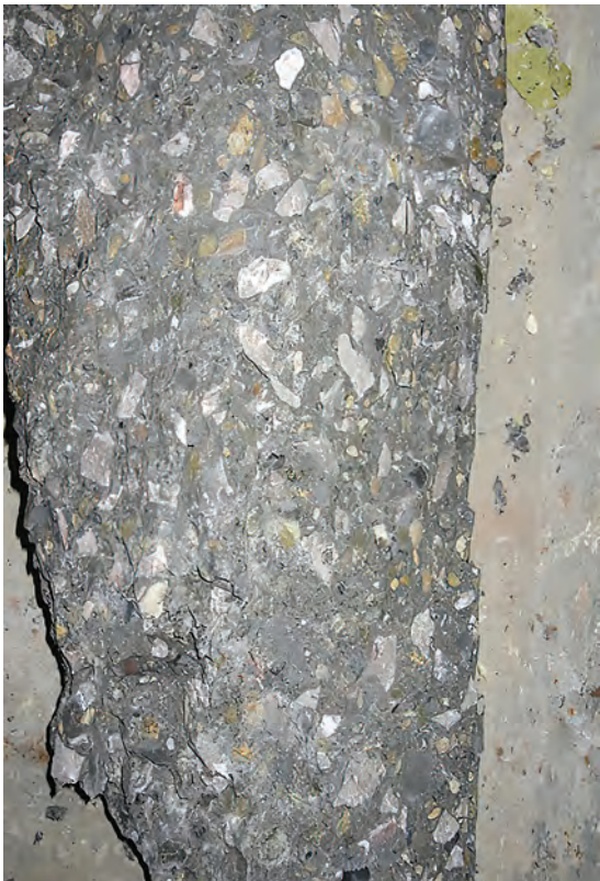
FIGURE 13.14 Aggregates crushing in high-strength concrete. (Photograph by the author.)
