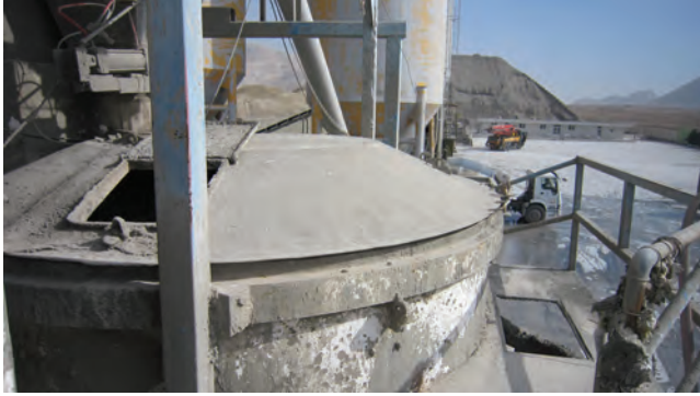
FIGURE 10.13 Pan mixer system. (Photograph by the author.)
