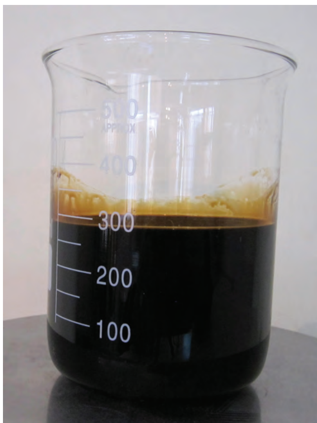
FIGURE 5.10 Lignosulfonate plasticizer. (Photograph by the author.)
