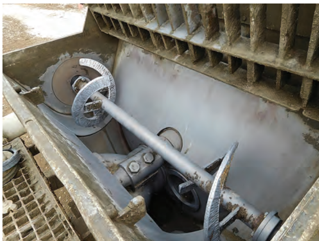
FIGURE 5.27 Concrete pump hopper and its mixer. (“Aldi, Cosne, concrete pump.”)
