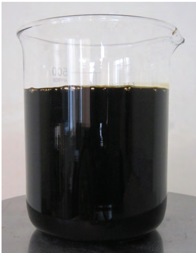
FIGURE 5.11 Poly naphthalene sulfonate super-plasticizer. (Photograph by the author.)
