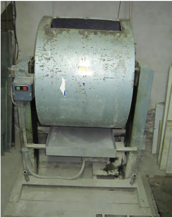
FIGURE 4.27 Los Angeles test machine. (Photograph by the author.)
