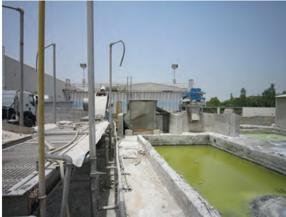
FIGURE 6.5 A concrete recycling system that it can recycle aggregates and water from the concrete sewage. (Photograph by the author.)
