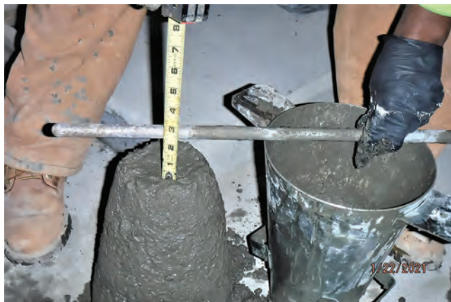
FIGURE 7.2 Measuring concrete slump. (“Conducting a slump test on the concrete” by MTA Construction & Development Mega Projects.)
