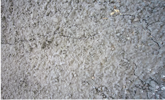
FIGURE 12.8 Chemical shrinkage and cracks. (Photograph by the author.)
