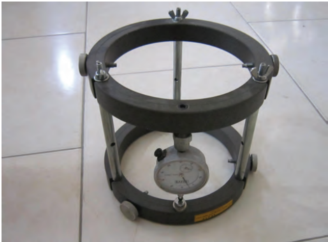
FIGURE 7.15 Instrument for testing of elastic modules and Poisson’s ratio of concrete. (Photograph by the author.)
