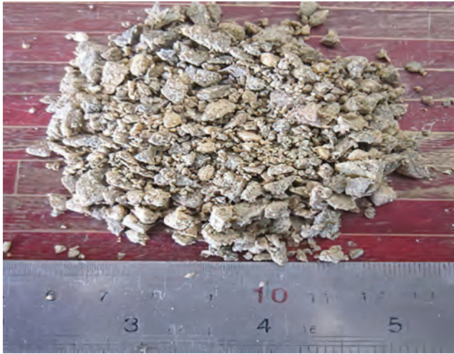
FIGURE 4.22 Picture of 0–8 sand. (Photograph by the author.)
