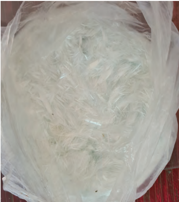
FIGURE 11.4 Glass fibers for use in the production of glass fiber reinforced concrete. (Photograph by the author.)
