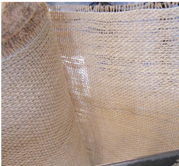
FIGURE 6.6 Special cotton textile for use in water curing for the protection of water. (Photograph by the author.)
