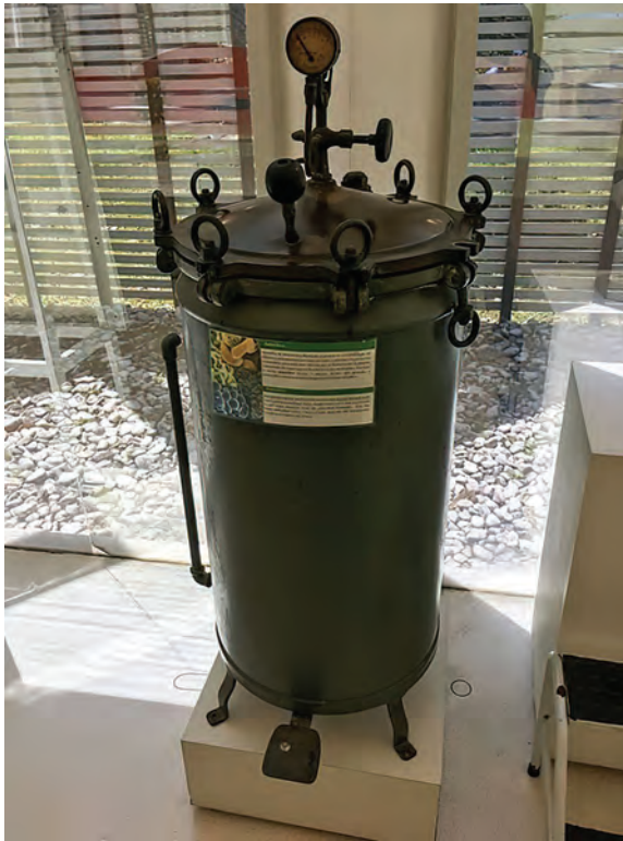
FIGURE 2.18 Picture of autoclave. (“Instituto Butantan, São Paulo, Brazil.Autoclave” by Mike Peel.)
