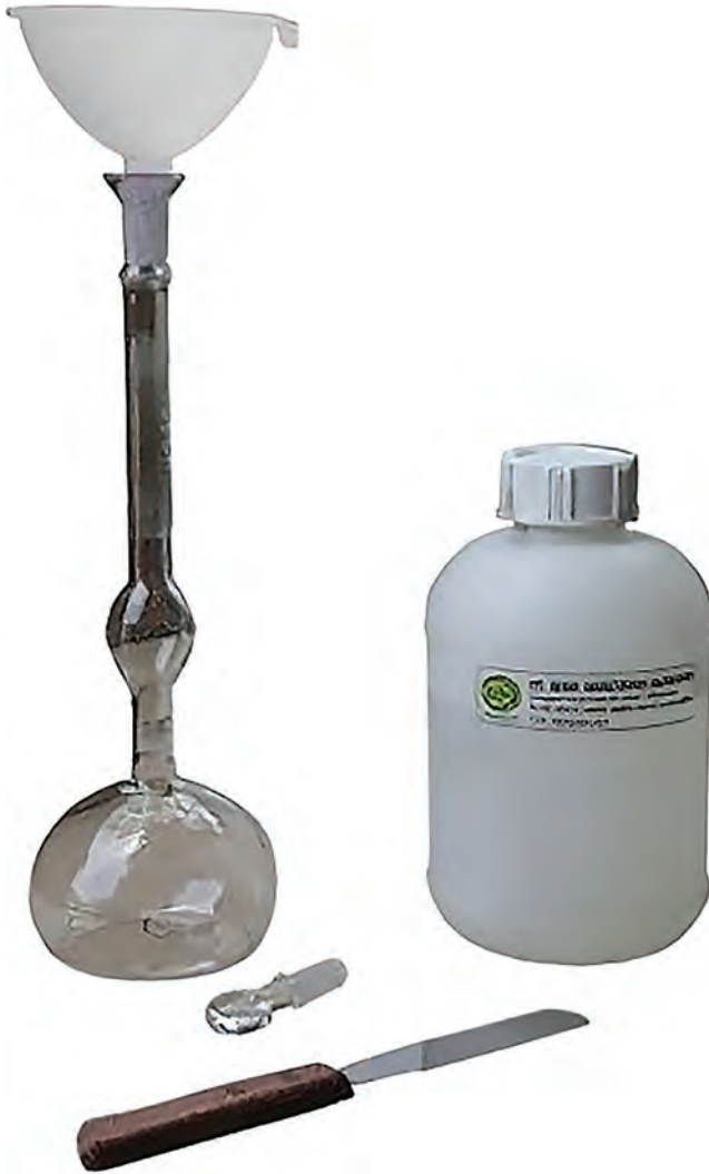
FIGURE 2.22 The Le Chatelier flask for cement-specific gravity test. (“Specific gravity test”).
