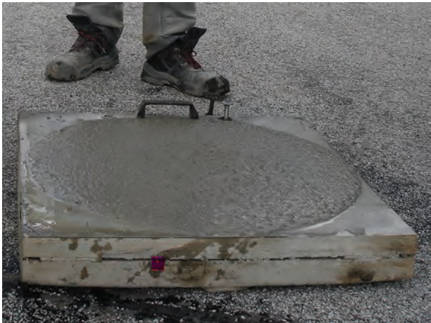
FIGURE 13.3 Slump flow test for SCC concrete. (“Flow test after”)
