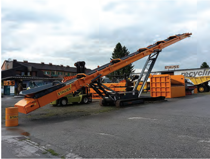
FIGURE 10.18 A conveyor belt that is suitable for concrete transportation. (“Mobile conveyor belt from TRIDIC”.)
