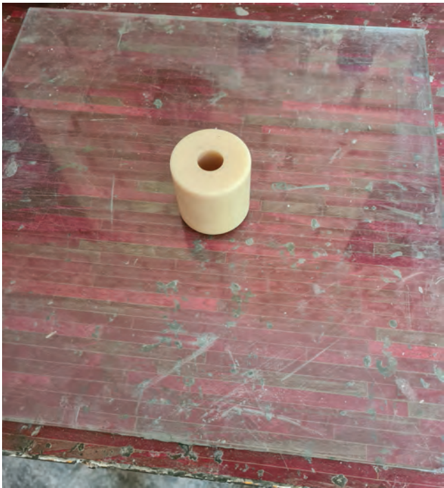
FIGURE 5.17 Mini slump test instruments. (Photograph by the author.)
