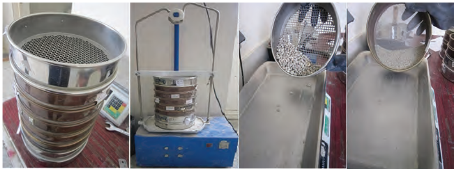
FIGURE 4.32 Sieve analysis test for fine aggregates. (Photograph by the author.)
