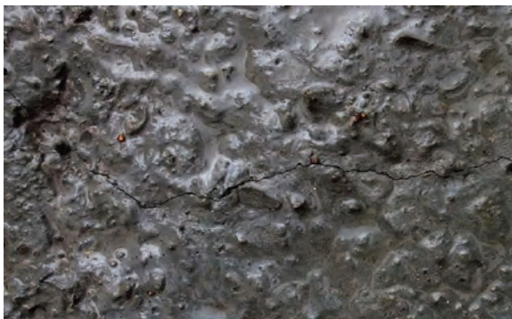
FIGURE 12.7 Plastic shrinkage and cracks. (Photograph created by the author.)
