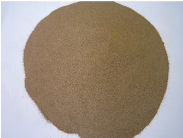
FIGURE 4.23 Picture of dune sand. (Photograph by the author.)
