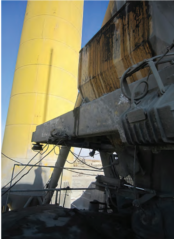
FIGURE 10.11 Cement discharging system by using the pneumatic valve. (Photograph by the author.)
