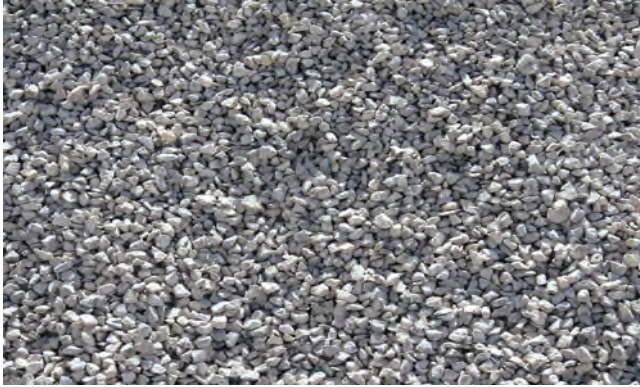
FIGURE 4.26 A deposit of crushed gravel in a ready mixed plant. (Photograph by the author.)
