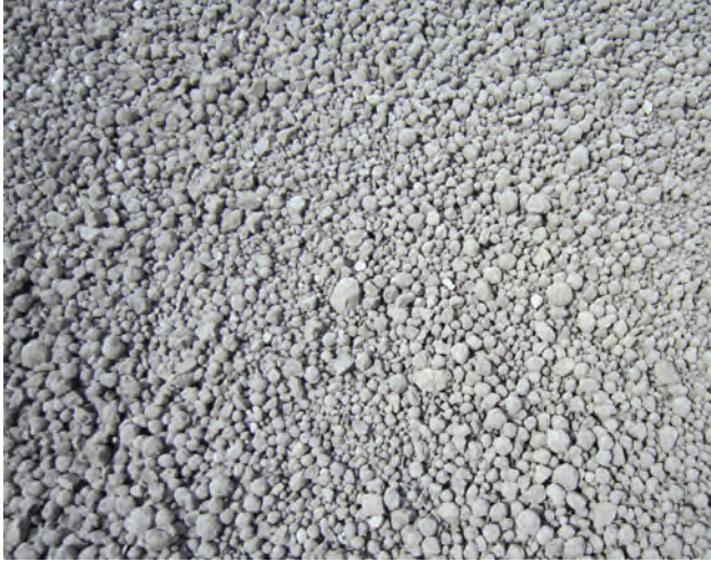
FIGURE 2.7 Portland cement clinker. (Photograph by the author.)
