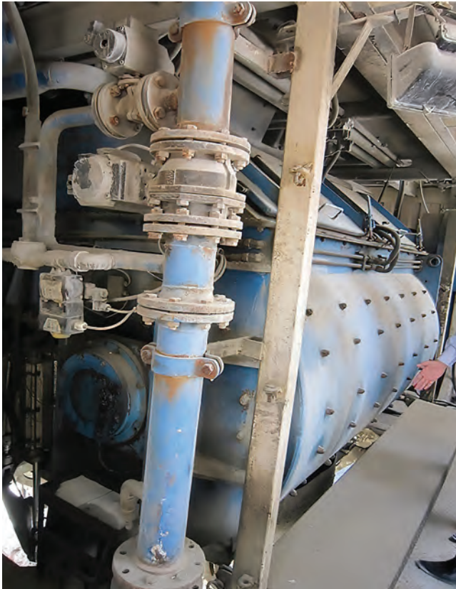
FIGURE 10.14 Twin shaft mixer system. (Photograph by the author.)
