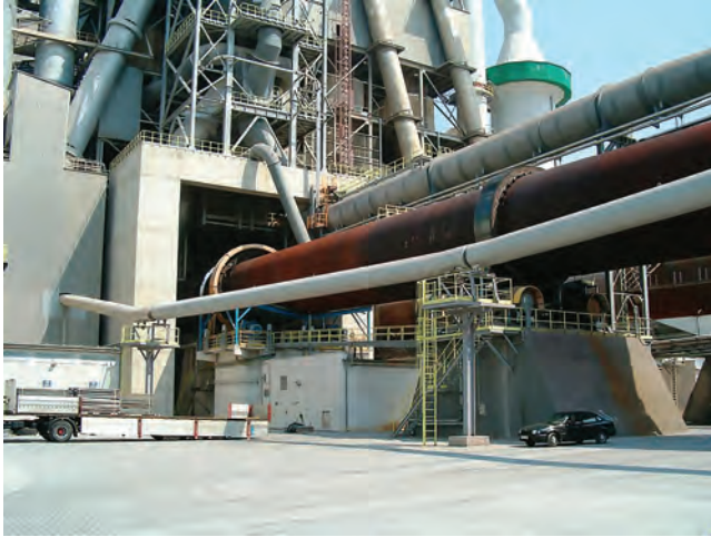
FIGURE 2.9 The roller cylinder kiln of a cement factory. (“Cement kiln. Location: Gorazdze Cement Plant near Chorula (Poland)”.)
