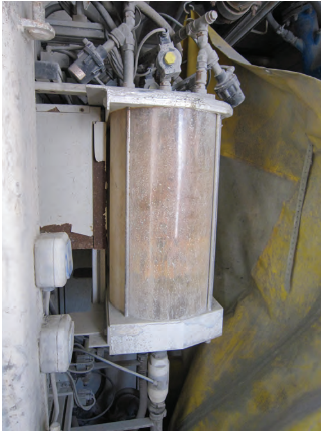
FIGURE 10.12 Volume base admixture dosing system. (Photograph by the author.)
