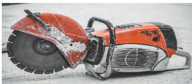
FIGURE 13.22 Cutting instrument for the surface of cylinder specimens (“Concrete cutter”)
