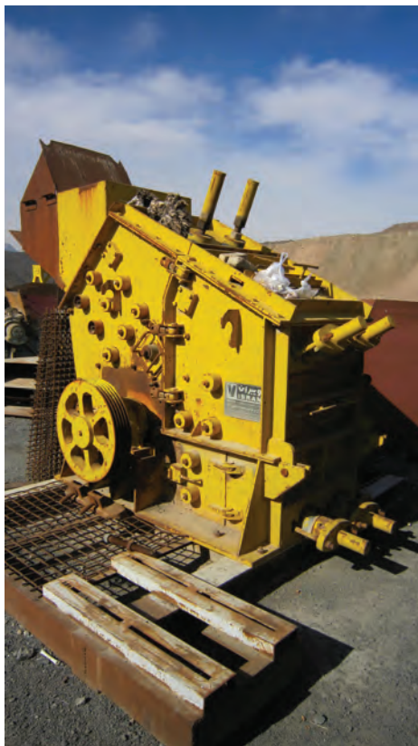
FIGURE 4.25 A sand maker machine. (Photograph by the author.)
