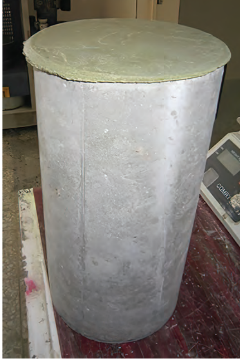
FIGURE 13.17 A capped cylinder specimens with melted sulfur and silica sand. (Photograph by the author.)
