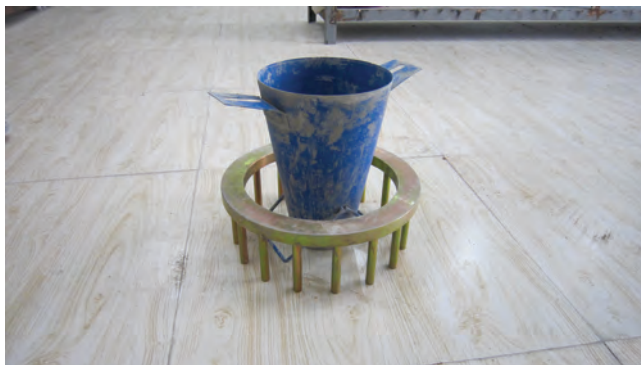
FIGURE 13.4 J-ring test for SCC concrete. (Photograph by the author.)
