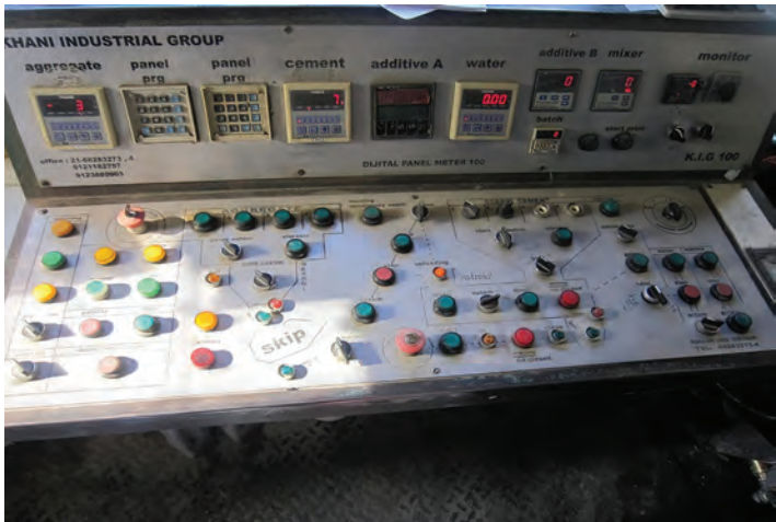
FIGURE 10.16 Half-automatic batching control system. (Photograph by the author.)
