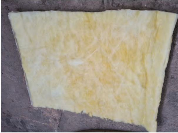
FIGURE 1.12 Suitable blankets to control the temperature of concrete in winter. (Photograph by the author.)
