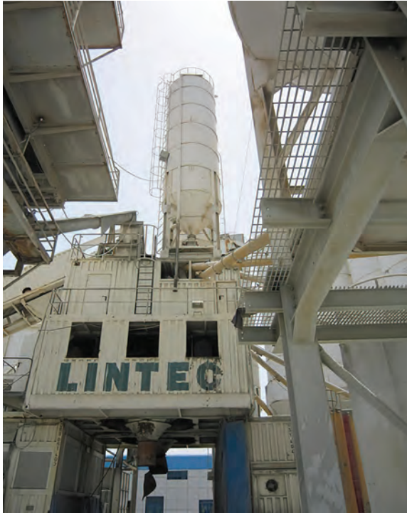
FIGURE 3.11 A special silo for silica fume direct use in concrete. (Photograph by the author.)
