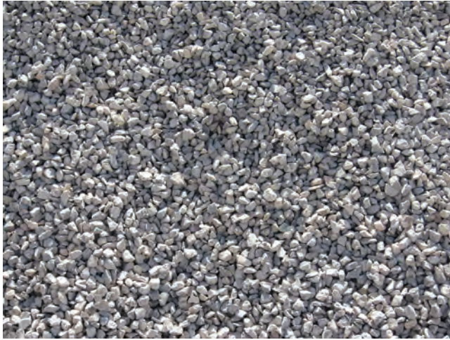
FIGURE 2.5 Limestone as raw materials for the production of Portland cement. (Photograph by the author.)
