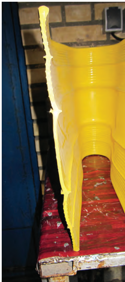
FIGURE 13.11 Section of types of PVC water stop tapes. (Photograph by the author.)
