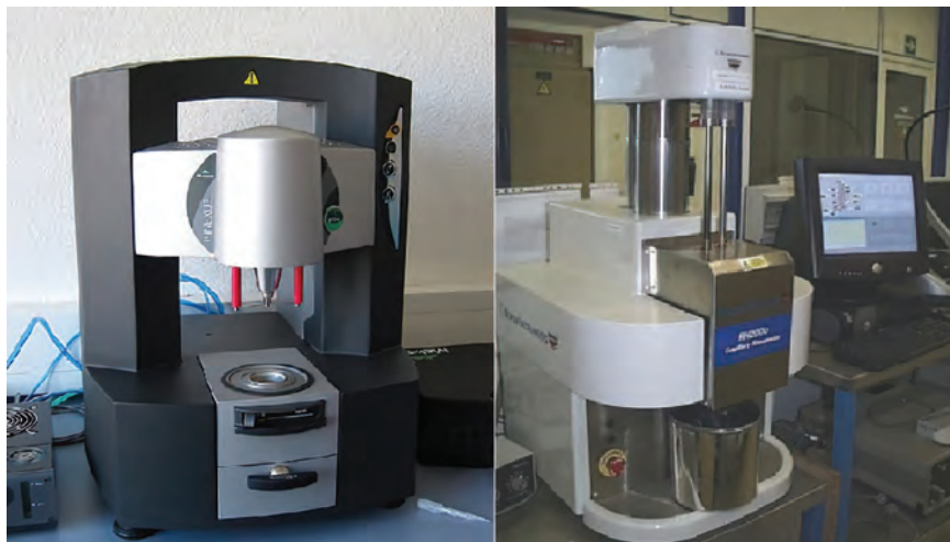
FIGURE 7.5 Two different types of rheometers. (“rheometer” by Olivier Cleynen used under a Creative Commons Attribution-Share Alike 4.0 International license), (“Capillary rheometer” by Cjp24 used under a Creative Commons Attribution-Share Alike 3.0 Unported license.)
