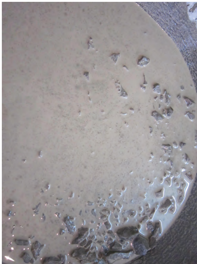
FIGURE 5.15 A segregated concrete with very low quality. (Photograph by the author.)
