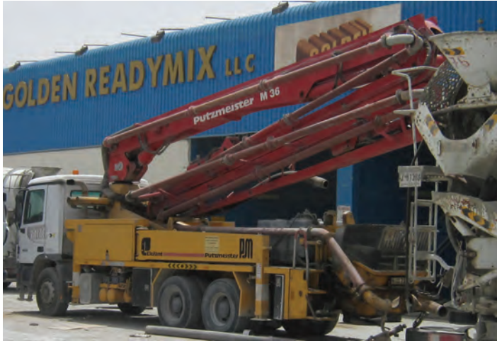
FIGURE 10.22 Boom concrete pump. (Photograph by the author.)
