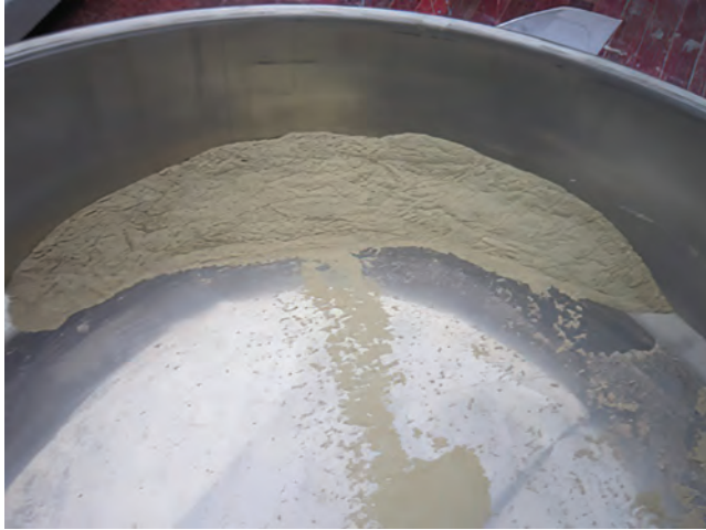
FIGURE 4.38 Passing of sieve No. 200 for a natural sand. (Photograph by the author.)
