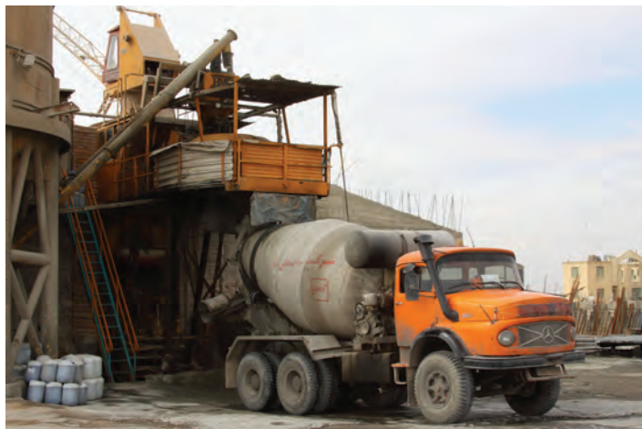
FIGURE 10.17 Truck mixer under the batching, the special vehicle for concrete transportation. (Photograph by the author.)
