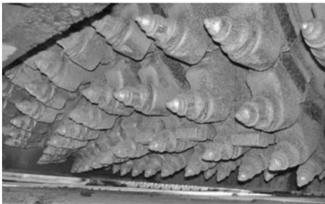
FIGURE 23.3 Fine milling heads spaced \leq 8 mm apart as shown are being used to minimize damage to the milled surface.
