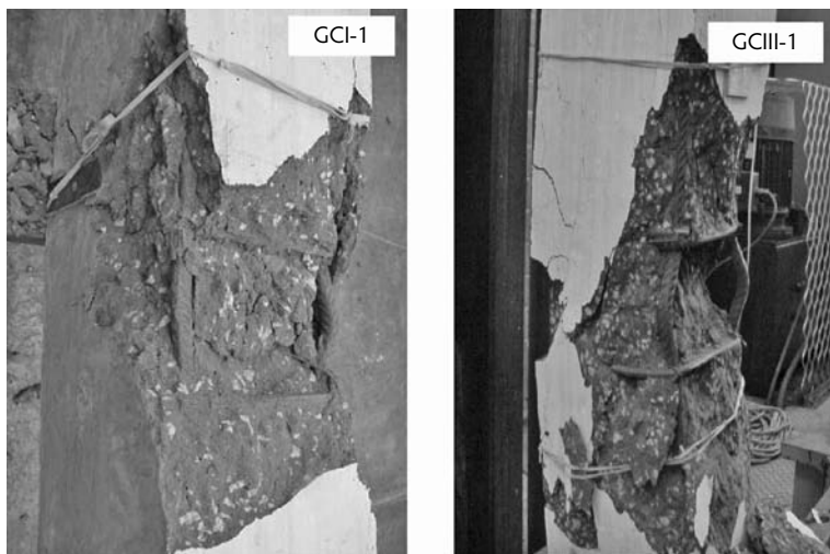
FIGURE 26.12 Failure mode of reinforced geopolymer concrete columns. (From Sumajouw, M.D.J. and Rangan, B.V., Low-Calcium Fly-Ash-Based Geopolymer Concrete: Reinforced Beams and Columns , Research Report GC3, Faculty of Engineering, Curtin University of Technology, Perth, 2006.)
