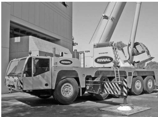
FIGURE 19.23 Tilting operator cab on an all-terrain crane superstructure.
