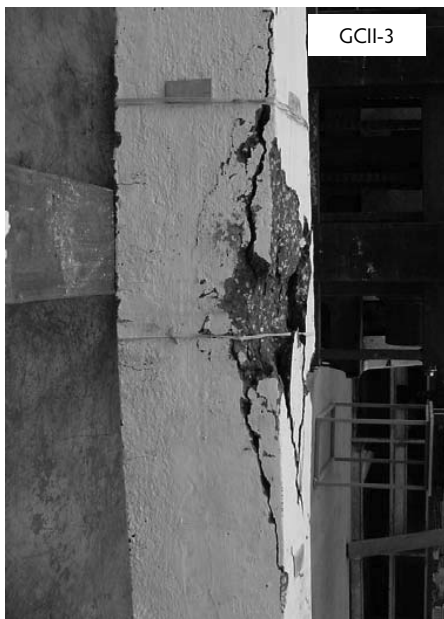
Failure mode of reinforced geopolymer concrete columns. (From Sumajouw, M.D.J. and Rangan, B.V., Low-Calcium Fly-Ash-Based Geopolymer Concrete: Reinforced Beams and Columns , Research Report GC3, Faculty of Engineering, Curtin University of Technology, Perth, 2006.)
