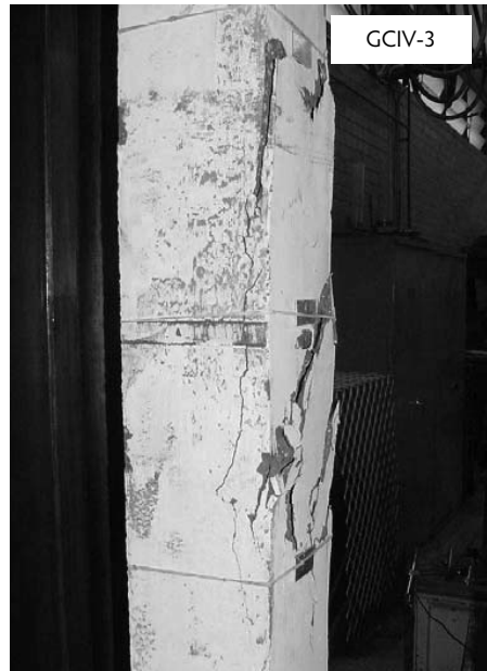
Failure mode of reinforced geopolymer concrete columns. (From Sumajouw, M.D.J. and Rangan, B.V., Low-Calcium Fly-Ash-Based Geopolymer Concrete: Reinforced Beams and Columns , Research Report GC3, Faculty of Engineering, Curtin University of Technology, Perth, 2006.)
