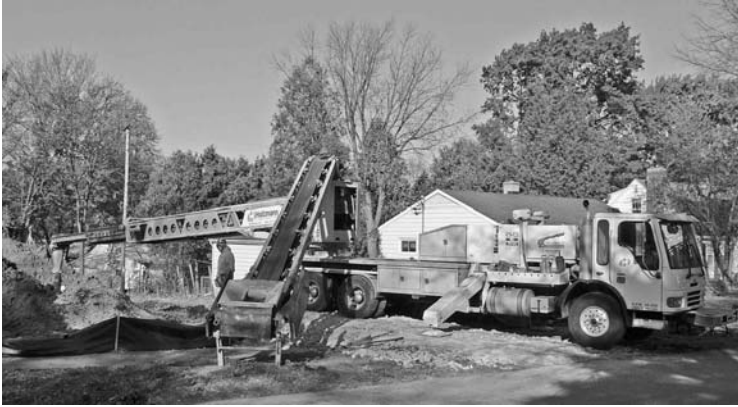
FIGURE 19.26 Truck-mounted telescopic belt conveyor.
