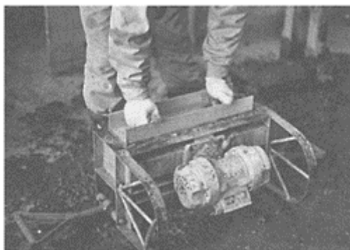
Photo 1. Instant-stripping apparatus and vibrating compaction of no-slump concrete
