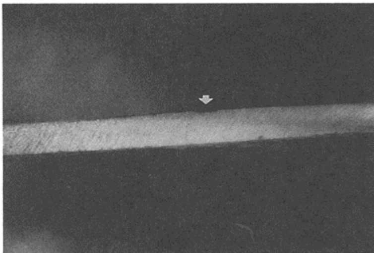
Fig. 6. Micrograph of the corrosion depth in the plate (cross section) embedded in the plain concrete after three months of immersion in sea-water.
