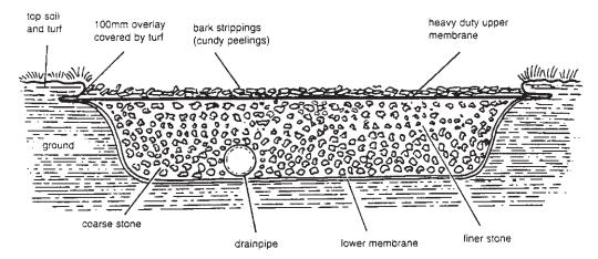
Fig. 31.11 Cross-section of a cow track.
