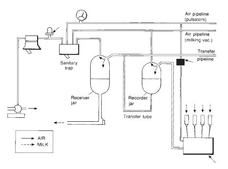
Fig. 26.3 Recorder milking machine.
