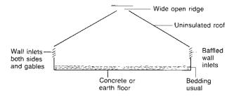
**Fig. 56.1** Cross-section of 'climatic' livestock house with open ridge and baffled wall ventilators.
