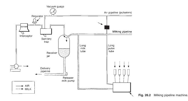
has been reached. When the vacuum level drops, the regulator closes; this stops admission of air and the vacuum level rises until the preset level of vacuum is reached, at which time the regulator opens again and admits air.
