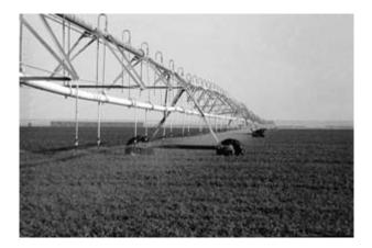
Fig. 71.1 A centre pivot irrigation system.
