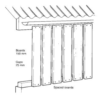
Fig. 56.10 Wall ventilation with spaced boarding.
