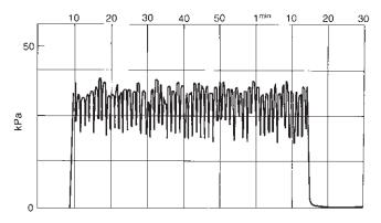
Fig. 26.5 Vacuum changes (cyclic fluctuations) at the teat end during milk flow.
