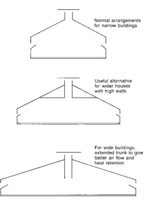
**Fig. 56.2** Alternative arrangements suitable for natural ventilation of various widths of buildings and using outlet ('chimney') trunks.
