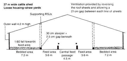
Fig. 4.24 A 27.5 m (90 ft) wide cattle shed with loose housing (reprinted from Hughes, 2000).
