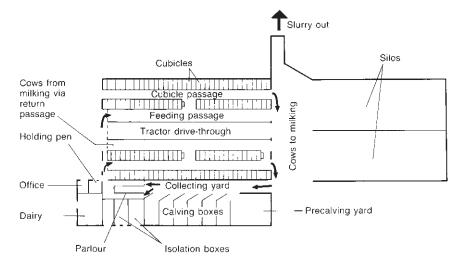
Fig. 4.17 Typical layout of a dairy unit.
