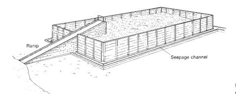
Fig. 4.27 A weeping-walled slurry compound.
