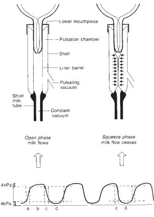
Fig. 26.4 Pulsation chamber waveform.
