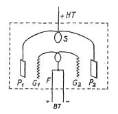
Fig. 7 – Double triode multiple lamp with symmetrical connections and a single filament, according to the original drawing of the author's patent.
