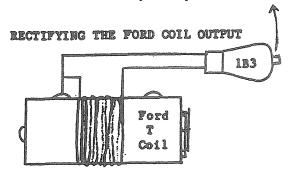
Wind 15 or more turns of fairly heavy insulated copper wire around the middle of the Model T Ford Coil. One lead from the winding goes to the Hi-voltage output of the Coil, and to pin 2 or 7 of the IB3 tube. The other lead goes to the other pin, as only two pins of the tube, 2 and 7, are used in this hookup. The souped-up or rectified voltage is drawn off the top of the tube to the spark gap and condenser.
