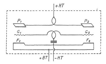
A further improvement of the device is seen in Figure 6. of which Lakhovsky says: "This illustration, also taken from my patent, shows a double and symmetrical oscillator where the filaments are mounted in series. It is also provided for, eventually, to place within a condenser so located as the electrodes and the loops of the oscillating circuit, within the same evacuated glass-vessel''.
