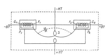
Figure 7 shows us a double-oscillator with a single filament, that is the two lamps of Figure 6 within a single vessel and with just one heat-source.
