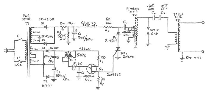
Note: Optional ground for Tesla coil secondary, if it reduces output do not use. R3 made from four 25K 10w resistors in parallel. VR1 linear taper. C1 may or may not be polarized. C6, C7 could be single .0025/15KV capacitor. SCR1, Q1 and all diodes can be standard replacement equivelants. MFR Type: T1 - TRIAD. T2 - Stancor H0 6246, Thordarson fly. Alternate values: R3 - 1K ohm, 225 watts; C5 - 1 microfarad, 600v.
