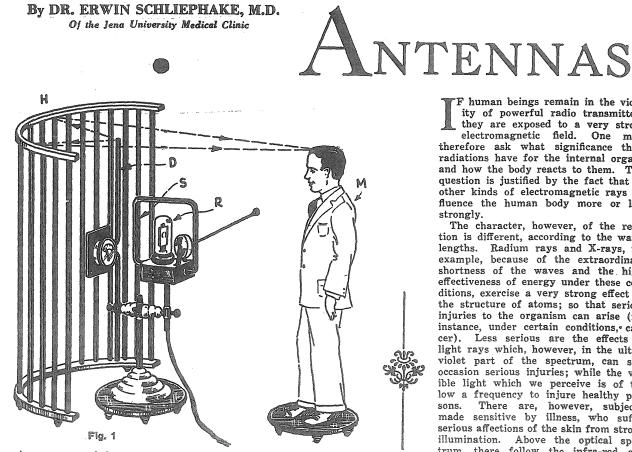
Arrangement of the apparatus used by Dr. Schliephake in measur-ing and observing the effects of short waves on the human body, absorption, et cetera. H, parabolic reflector formed of wires; D, antenna, charged inductively by the coil S; vacuum tube at R, and beside it wave changing condenser; subject at M.
