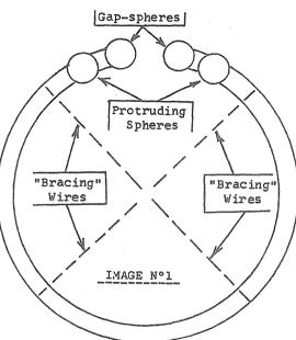
Detail of outer ring on Lakhovsky's original MWO antenna. Front view above, side view below
