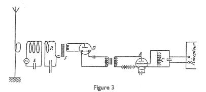
It employs iron's properties of magnetic saturation (see the magazine Onde Electrique, Volume No 5, pp 237-263, June 1926) and it uses a powerful triode "A" which generates oscillations directly into circuit "E", exciting the antenna directly. Coupled to "E" is most used arrangements are those made by one Mr Reinartz and one Mr Bourne.
