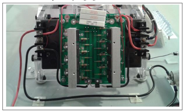
This is all of the larger **Red** and **Black** wires that connect between the batteries, meters, terminal blocks, and other sections of the circuit. When
