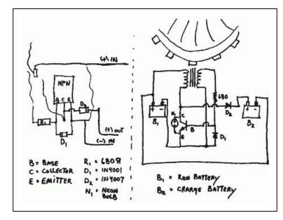
all of the supposed smart <u>guys</u> who had not looked at it before, and second, he used the two battery system where the motor ran from one battery and charged the second battery directly from the recovered energy.
