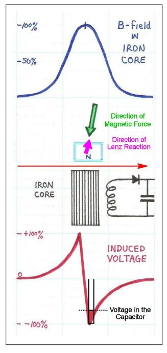
by this current is applied back toward the external magnetic field in exact opposition to the angle by which it is induced. In this case, it reduces the permanent magnet's attraction to the iron core, which is still mostly vertical in its orientation at this moment.
