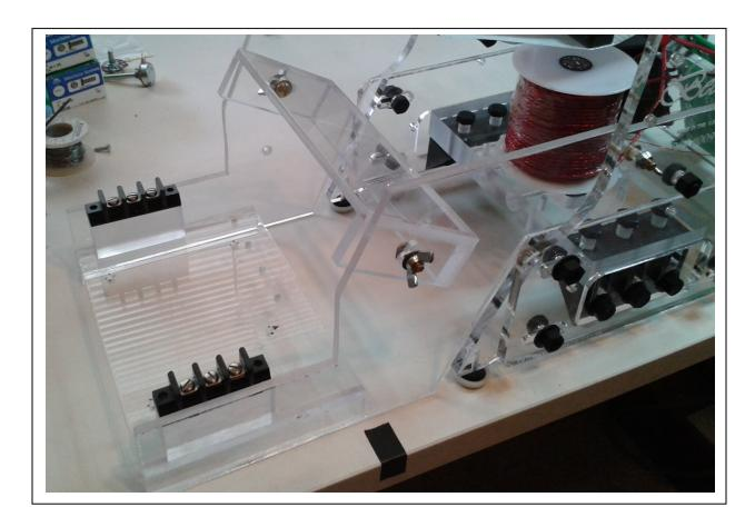
The frame extension pieces bolt to the vertical supports of the original SG
