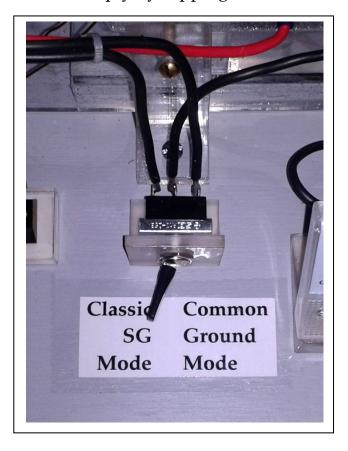
**BLACK** wires that are attached to the outer connections of the switch and feed off to the left of the photo, connect to the either the Run Battery positive terminal (+) to create the Classic SG Mode circuit, or the Run Battery negative terminal (-) through the new diode to create the Common Ground or Generator Mode circuit.
