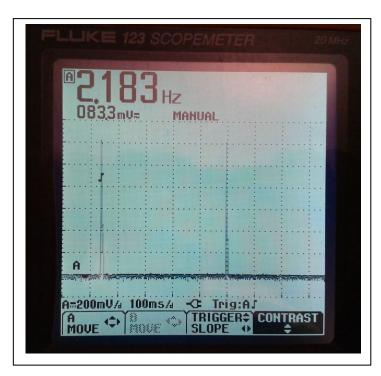
The first thing we can see is that the capacitor circuit is discharging into the charge battery B2 at a rate of 2.183 times per second. While this discharge
