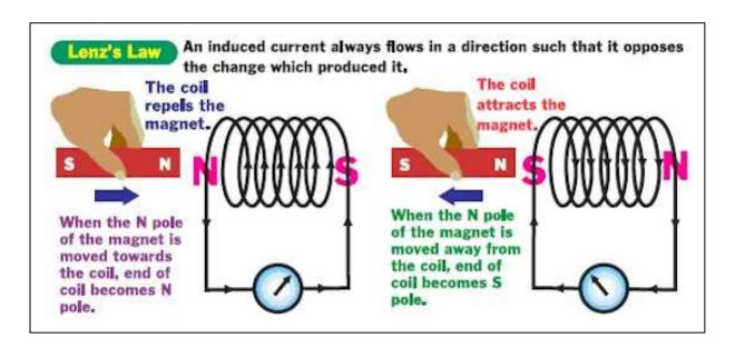
If the North Pole of the permanent magnet approaches the coil, current flows in the coil in a way that produces a second magnetic field that repels the magnet's approach. When the North Pole of the permanent magnet is then pulled away, the induced current in the coil reverses and produces a magnetic field that tries to attract it back in. In its most basic presentation, Lenz's Law can be illustrated like this:
