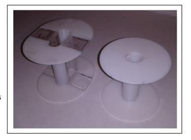
the permanent magnets. Therefore, a plastic spool like the one used for the power coil was cut in half and the center section was extended by 1 inch.
