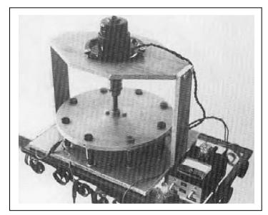
All of the circuitry, including the capacitor, is in the box to the right, with the mechanical relay visible on top. The two switches allowed the motor to run directly from the battery to get the unit up to speed, and then be put in "run mode" so that the circuit automatically switched the functions as
