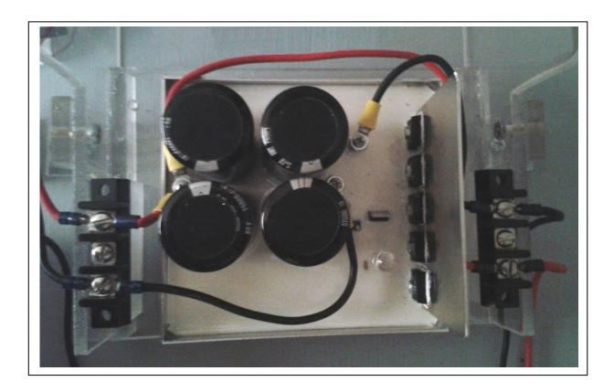
Here is an overhead photograph of the Capacitor Module wired in place. The wires coming in from the left provide the pathway to charge the capacitors with the coil discharges from the SG machine. The wires going out on the right provide the pathway to discharge the capacitors to the secondary battery (B2). The module senses the voltage in the capacitors, discharging them when that voltage rises to about 24 volts and then shuts off the discharge when the voltage drops to about 18 volts.
