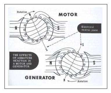
generates against itself or a generator that inherently motors against itself, depending on which force leads the other. Modern theory calls this the "armature reaction" and shows it as an angular displacement of the "electrical neutral line" in the rotor.
