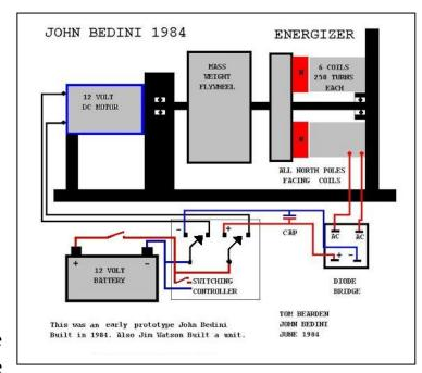
capacitor through a "full wave bridge" rectifier, whereas a single diode has been discussed before. The FWB simply clips both the forward and trailing
