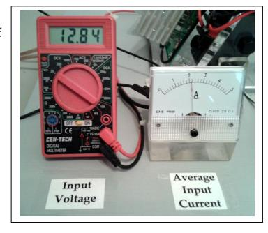
at about 335 RPM. So, according to the analog ammeter, the current input has risen from 1.4 amps in the Classic SG Mode to 2.15 amps in the Generator Mode. The ratio of increase can be calculated as follows:
