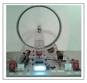
Typically, the SG circuitry is designed to draw approximately 0.25 amps per transistor, so a seven transistor circuit is expected to draw 1.75 amps from the Input Battery. The Conference Demo unit, with its balanced wheel, new bearings and fine tuned trigger circuit, was drawing 20% less
