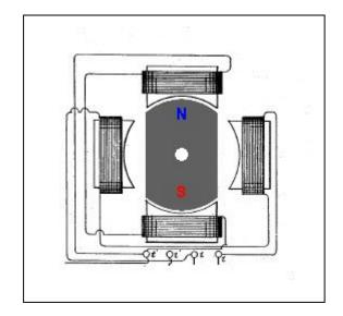
current flowing in the wire, the rotating magnet is still attracted to the iron in the pole pieces.
