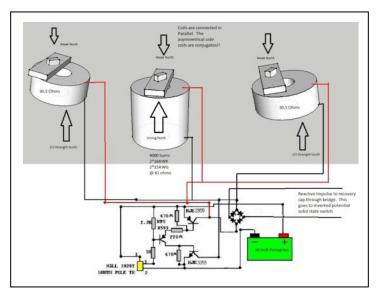
and the control circuit being basically a "Bedini-Cole Switch." The machine also had a two foot diameter "hub motor" section that operated as a motor during the "idle mode" and as a generator in "full power mode." The circuitry used here was also a modified Bedini-Cole Switch with recovery to the charge battery system.
