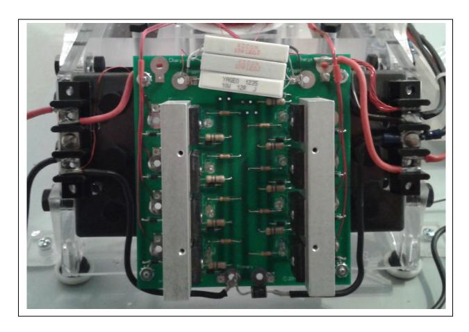
There are only two modifications made to this circuit board for this model. The first is that the single large 12 Ohm resistor (Yageo) at the top-center of the photo is joined by two more 12 Ohm resistors (Xicon) as part of the "fine tuning" of the trigger. This modification will be discussed in more detail shortly. The second modification is the large Diode at the bottom-center of the photo which is part of the "generator mode" circuitry which
