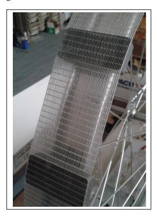
Cyanoacrylate adhesives are quite brittle after curing, and since this motor operates on an "attraction" mode, the magnetic field from the coil is trying to pull the magnets off of the wheel as they approach. With the reinforced tape in place, if the glue fails, a magnet will NOT fly across the room at 40 feet per second! Instead, you will just hear a "clicking" sound on the wheel as the magnet is pulled off of the rim slightly as it passes over the coil.
