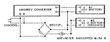
CHARGING OF BATTERY #2 VIA KROMREY CONVERTER AND BATTERY #1 VOLTAGE BATT. #2: 12.35 U, AND AFTER 4 MINUTES: 12.40 U
