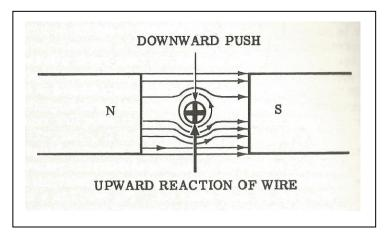
around the wire that tends to oppose the field above the wire and reinforce the field below the wire. These induced magnetic effects from the current in the wire create an upward mechanical reaction force on the wire in direct opposition to the downward motion that initiated it.
