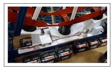
impedance circuit. The input was 36 volts (three 12 volt batteries in series) and the output was the same. The batteries boiled continuously during operation, and John never ran it for more than 30 minutes at a time in full power mode. The batteries were too small to be charged that hard.
