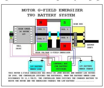
The green control box includes circuitry that monitors the battery voltages and automatically switches the batteries when the run battery drops to 11.1
