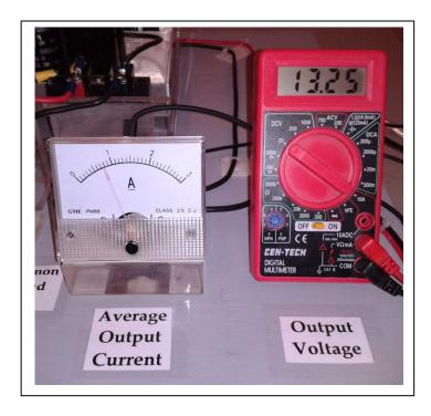
running, the indicator needle is bouncing between "0" and "1.2" on the scale. The digital Output Voltage is taken directly across battery B2.
