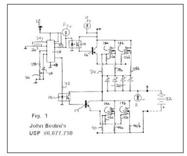
120,000uf, charged to about 25 volts. It was discharged about once a second through six parallel N-channel MosFets into a large 12 volt battery.
