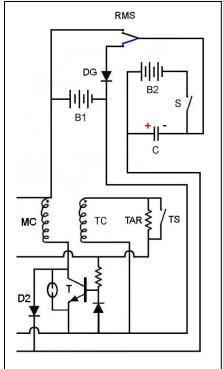
connected to the positive terminal of B1 and completes the discharge path to the negative terminal of the capacitor C through RMS. When RMS is in the upper position, (Classic SG Mode) the discharge path by-passes B1 and
