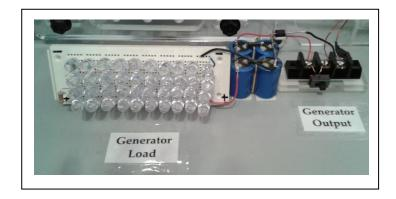
The switch was a simple toggle type. The diode was a 6A100. The four capacitors together had a capacitance of 470uf. The resistor was rated for 100 Ohms at one watt. The 40 LEDs were wired as 4 parallel strings of 10
