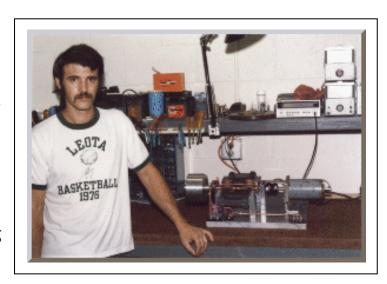
The early models proved that Kromrey was correct about the low drag characteristics of the generator. But there was something else that he hadn't mentioned. The machine was HORRIDLY LOUD when running. It made this deep, harsh growl sound like a Buzz Saw as the magnetic fields were cut. No modifications were ever found to quiet the thing down.
