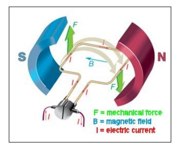
that will try to reverse the flow of current. If the mechanical force in the direction of **F** becomes the "input" to the device, the machine becomes a "generator" and produces electric current in the opposite direction shown.
