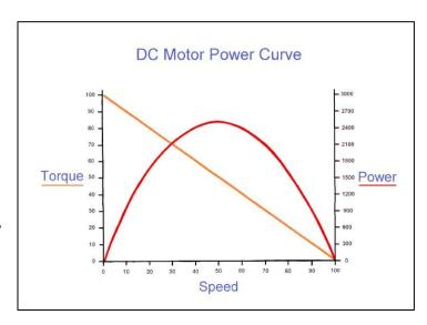
between the Speed, the Torque produced, and the consequent Power, which is a cross-product of the Speed and Torque. In this diagram, the Torque is shown by the **Orange Line** and the Power is shown by the **Red Line**. In a motor like this, the Torque is a direct consequence of how much electric current is moving through the armature windings in front of the stator magnets.
