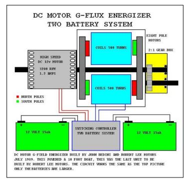
So, by 1989, we see significant improvements to the Self-running Energizer circuit disclosed in the 1984 book which only used one battery. The drawing above shows a two pole rotor but specifically stipulates an eight pole rotor. This arrangement was tested on a wide variety of systems over the years, such as in this model.
