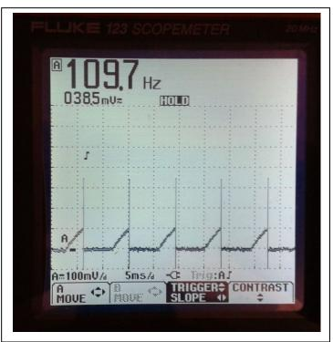
this image was produced. It shows pulses that peak at a height of about one division repeating 109.7 times per second.
