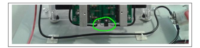
Since this was a display model designed for public demonstrations, both the SG Classic Mode connections and the Generator Mode connections were built into the machine. A switch was added to the circuitry so that the machine could be run in either mode, simply by flipping the switch.
