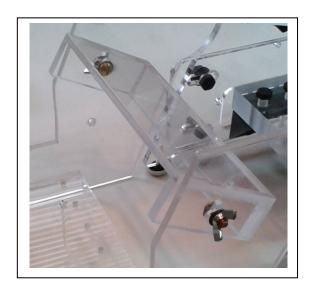
created. Since the magnets on the wheel were going to be exerting a strong attraction force toward the core in the generator coil, the coil had to be held absolutely rigidly to avoid vibrations in the frame and the possibility of an accident if the coil moved uncontrollably toward the rotating wheel.
