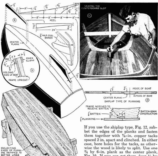
flat-head brass screws and to the sides with 1¼-in. No. 6 flat-head brass screws spaced 1½ in. apart in a staggered row. Then fair off the sides, transom and stem, a job which must be done carefully to avoid leaks. At this point, select the type of bottom construction. If it is to be the batten-seam type, battens must be mortised at the proper places and the planks are fastened to the battens with 1¼-in. copper nails spaced 2 in. apart and clinched.
