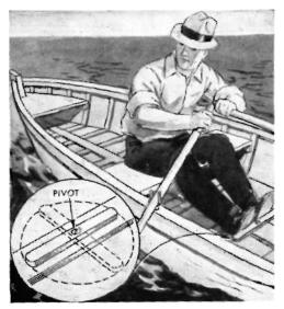
Footrests usually are attached so that they are in the way when scrubbing or bailing out a boat. If the rest is pivoted, it may be turned out of the way when not in use. The pivot bolt should be tight enough to hold the rest in closed position.
