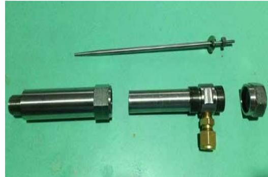
Injector expanded view without insulator with connected fuel and plasmoid inlet
