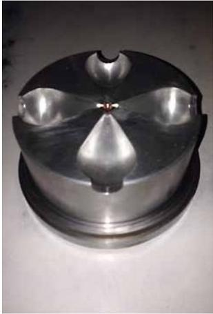
Implosive cylinder head concentrating force into a central tungsten carbide sphere.
