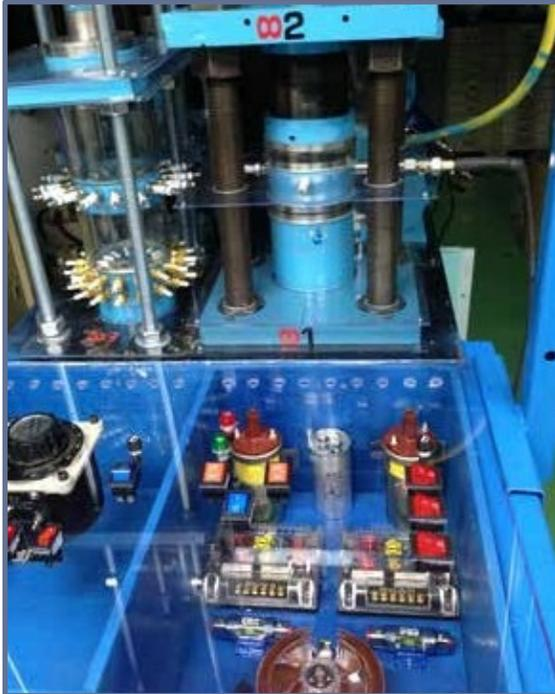
Electronic control panel with variac, modified car coils and plasma generator.
