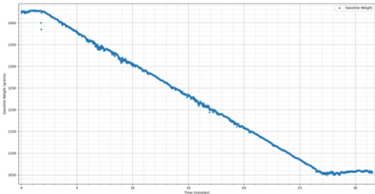
Figure XX. Weight of graduated cylinder containing gasoline during Unloaded#2 generator test. The linear decline middle portion was regressed to obtain fuel consumption rate. A rate of 0.244 grams/second (0.878 kg/hr) was obtained. Pink vertical lines are used to roughly indicate relevant times during the experiment.
