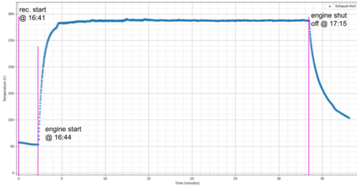
Figure XX. Exhaust port temperature during first attempted loaded generator startup/priming test. Pink vertical lines are used to roughly indicate relevant times during the experiment.
