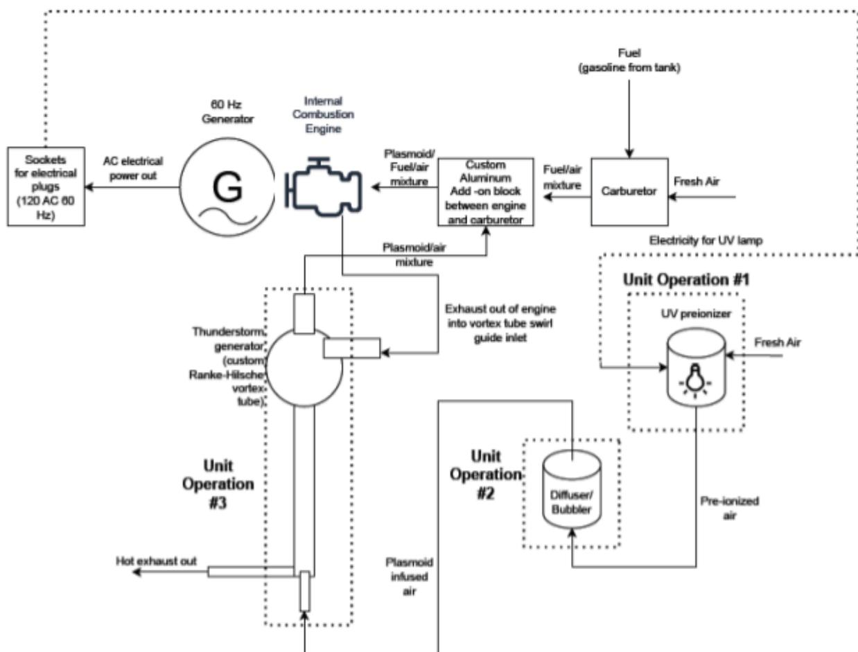
Figure 1. A process flow diagram of the VGR system attached to a portable gasoline engine electric generator. This flow diagram was created based on the system the author inspected during the live demonstrations witnessed on 8/13/2023 and 8/14/2023.
