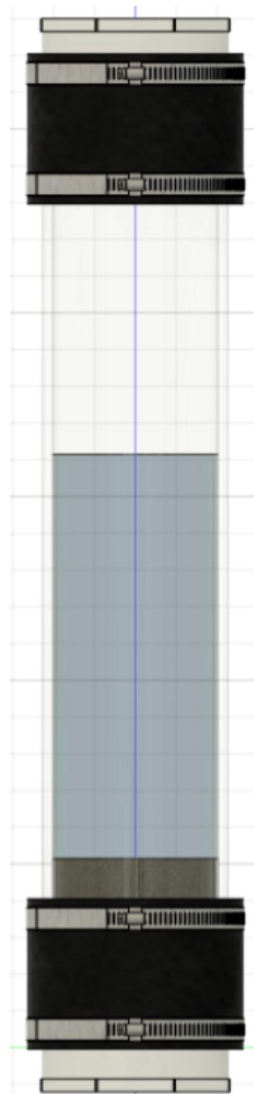
Figure 6. Model depiction of the bubbler unit. Air enters through the bottom PVC cap and diffuses through the porous stone into the water. Steel wool is located inside and above the water.
