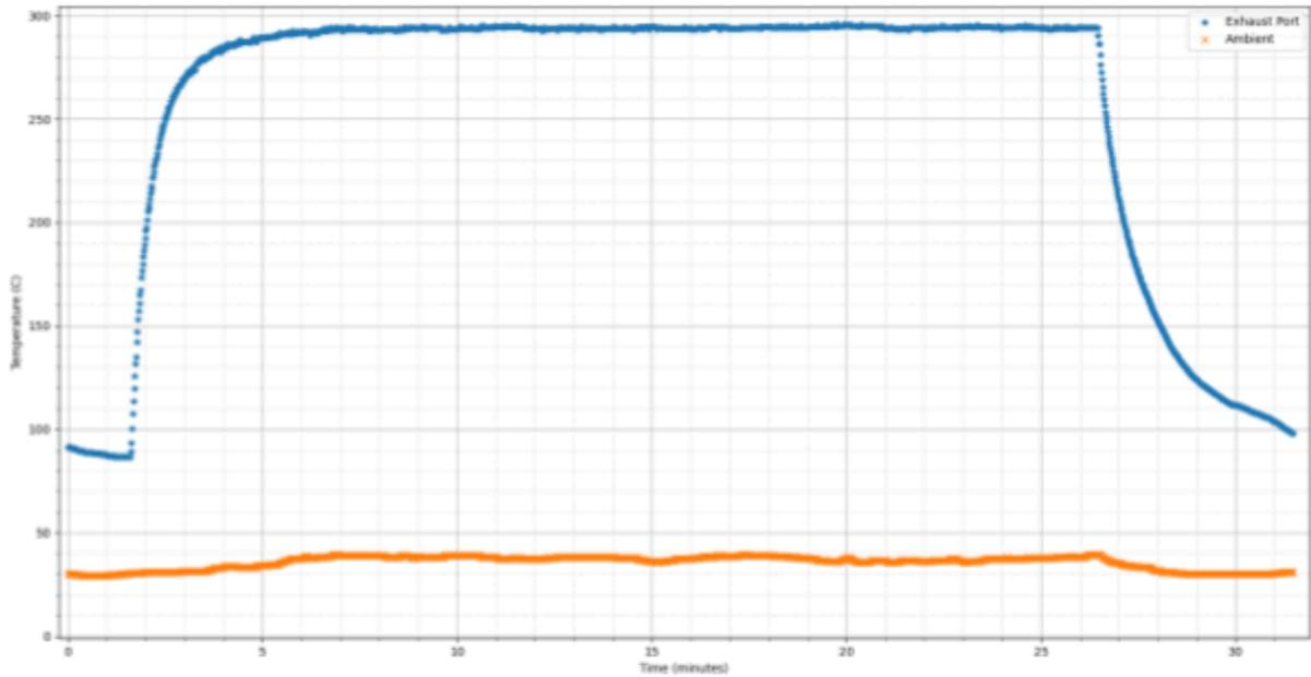
Figure XX. Exhaust port and ambient temperatures during Unloaded#2 generator test. Pink vertical lines are used to roughly indicate relevant times during the experiment.
