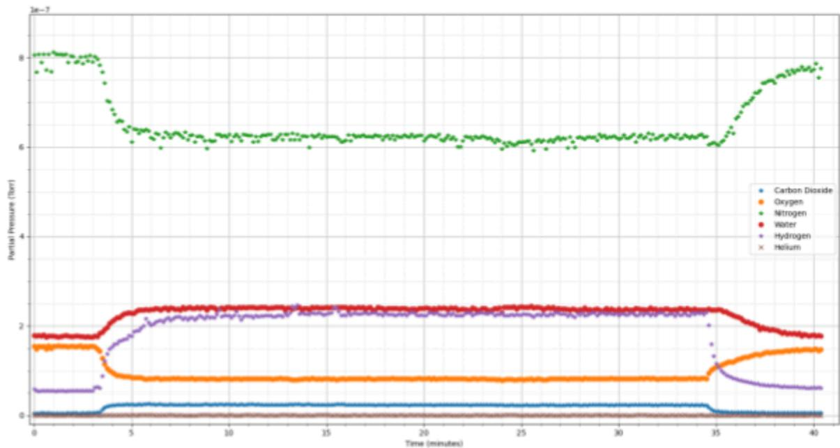
Figure XX. Mass spectrometer gas analysis of first attempted loaded generator start-up/priming run.
