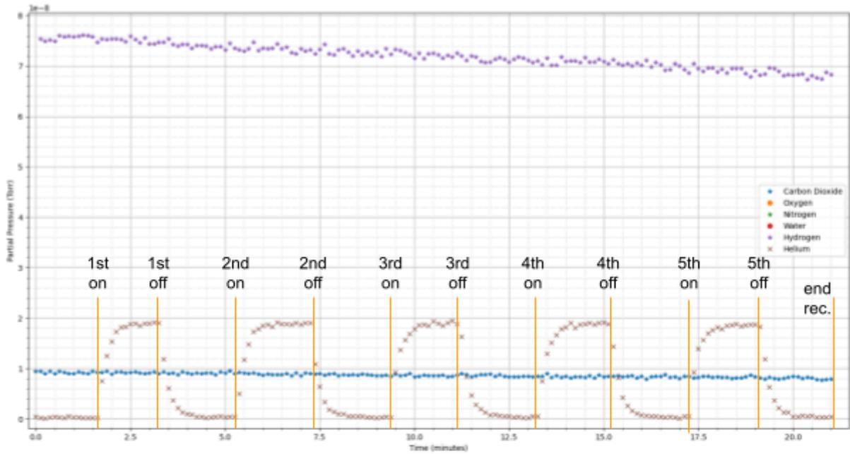
Figure XX. Gas sampling characterization test. Response to flowing 50 SCCM helium gas into the sampling inlet for 120 seconds at 120 second intervals. The graph is zoomed in to highlight the helium mass peaks. Orange vertical lines roughly indicate on and off times of helium flows, and end of record.
