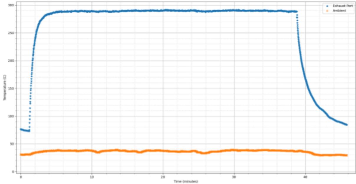
Figure XX. Exhaust port and ambient temperatures during Unloaded#3 generator test. Pink vertical lines are used to roughly indicate relevant times during the experiment.
