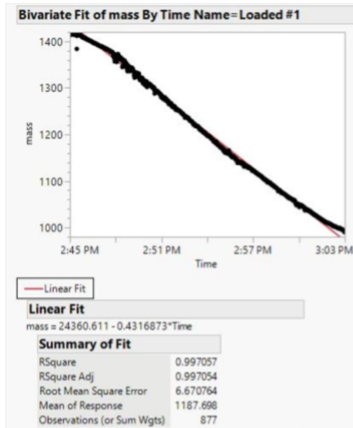
Figure XX. Linear regression of Loaded#1 test. A slope of -0.432 grams fuel/second is obtained with a coefficient of determination ( $R^2$ ) value of 0.997057.
