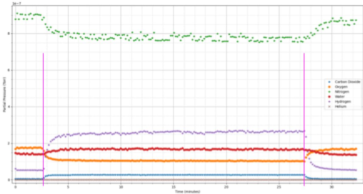
Figure XX. Mass spectrometer gas analysis of Unloaded#2 generator test.
