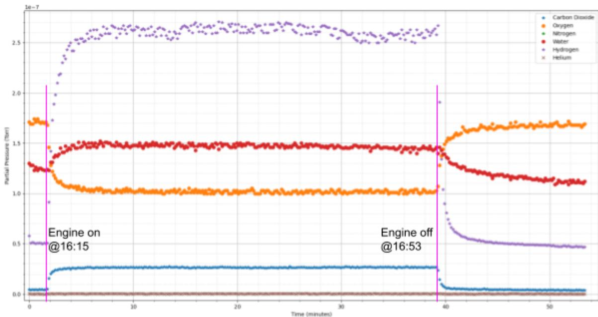
Figure XX. Zoomed in mass spectrometer gas analysis of Unloaded#3 generator test.
