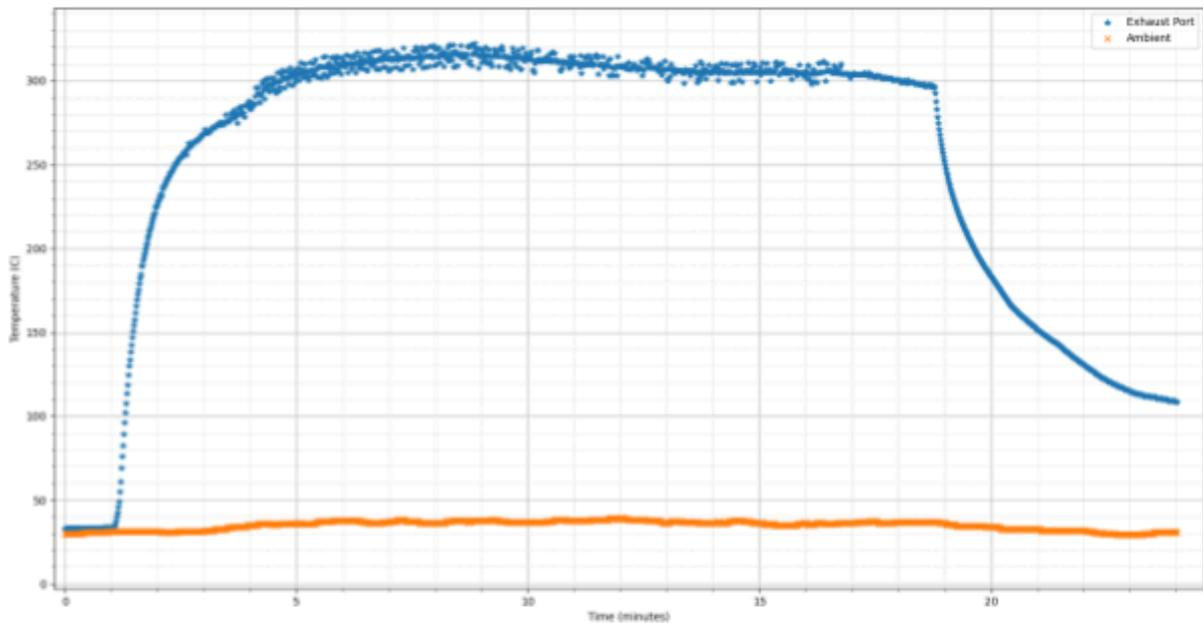
Figure XX. Exhaust port and ambient temperatures during Loaded#1 generator test. Signal noise induced by the generator can be seen on the exhaust port temperatures starting ~3.5 minute mark, and ending ~17 minute mark. Pink vertical lines are used to roughly indicate relevant times during the experiment.
