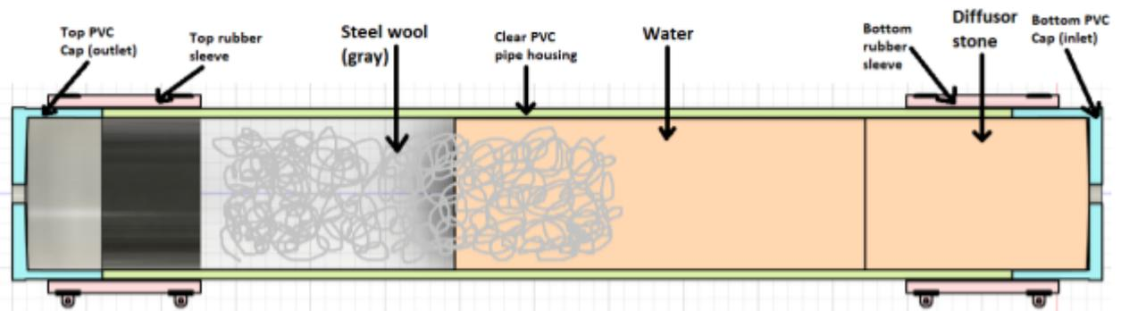
Figure 7. Cross sectional view of the bubbler unit labeled #2 in Figure 3.
