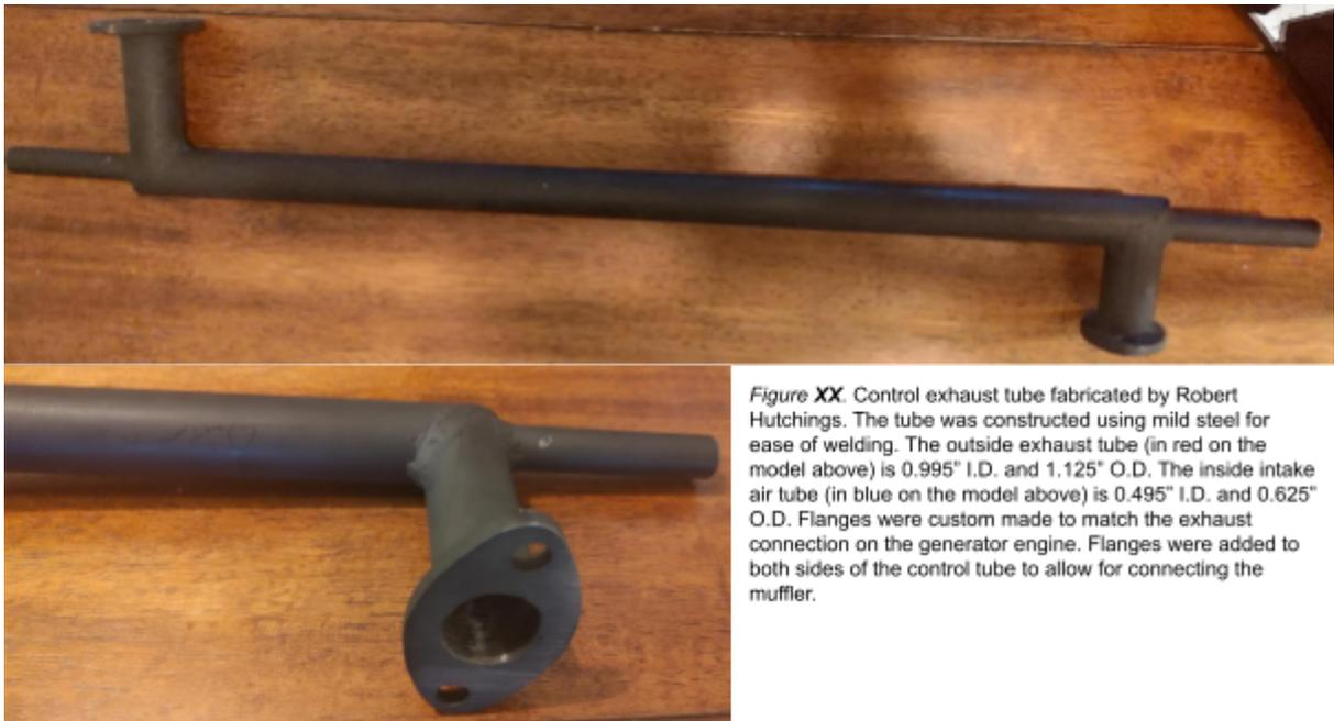
Figure XX. Control exhaust tube fabricated by Robert Hutchings. The tube was constructed using mild steel for ease of welding. The outside exhaust tube (in red on the model above) is 0.995" I.D. and 1.125" O.D. The inside intake air tube (in blue on the model above) is 0.495" I.D. and 0.625" O.D. Flanges were custom made to match the exhaust connection on the generator engine. Flanges were added to both sides of the control tube to allow for connecting the muffler.
