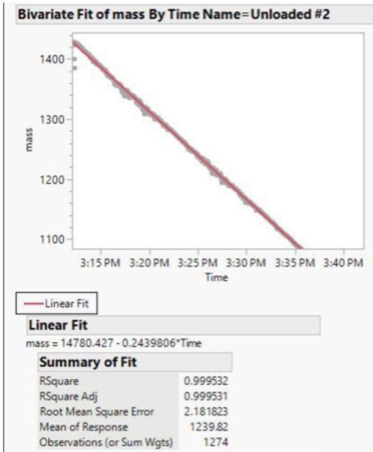
Figure XX. Linear regression of Unloaded#2 test. A slope of -0.244 grams fuel/second is obtained with a coefficient of determination ( $R^2$ ) value of 0.999532.
