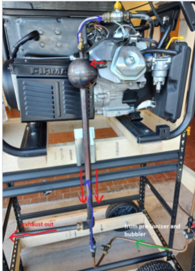
Figure 2. Frontside view of the VGR system depicting the internal combustion engine, thunderstorm generator, and carburetor. Cold intake air flow is depicted with blue arrows, hot combustion exhaust is depicted with red arrows.
