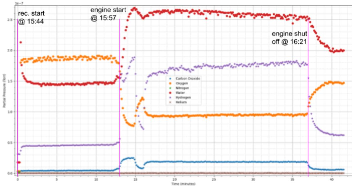
Figure XX. Mass spectrometer gas analysis of first unloaded generator start-up/priming run. Peak disruptions beginning around 15 minutes are due to the sampling inlet disconnecting from exhaust outlet. The sampling inlet was reconnected around the 16 minute mark on the graph. This is a zoomed in view excluding the nitrogen signal to show better resolution of carbon dioxide. Pink vertical lines are used to roughly indicate relevant times during the experiment.
