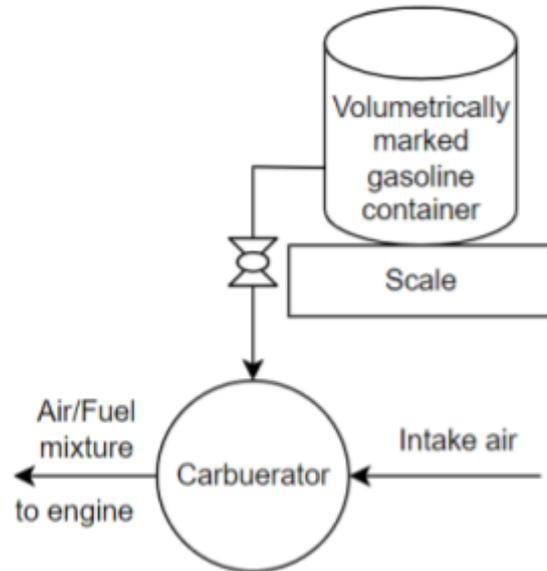
Figure XX. Schematic of custom fuel dispensing system allowing for gasoline consumption tracking.
