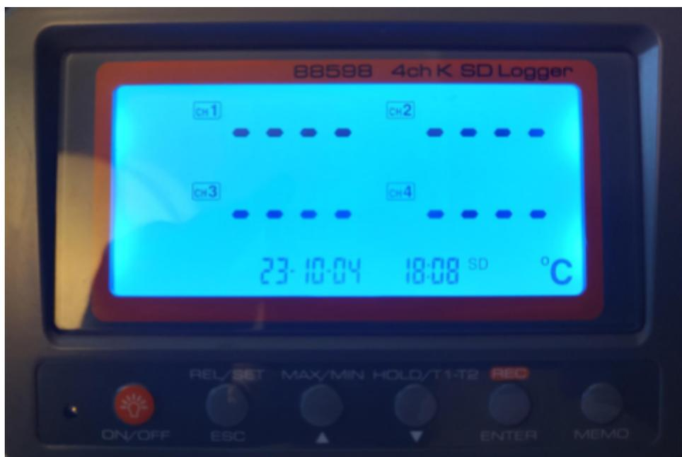
Figure XX. Four channel type K thermocouple temperature logger.
