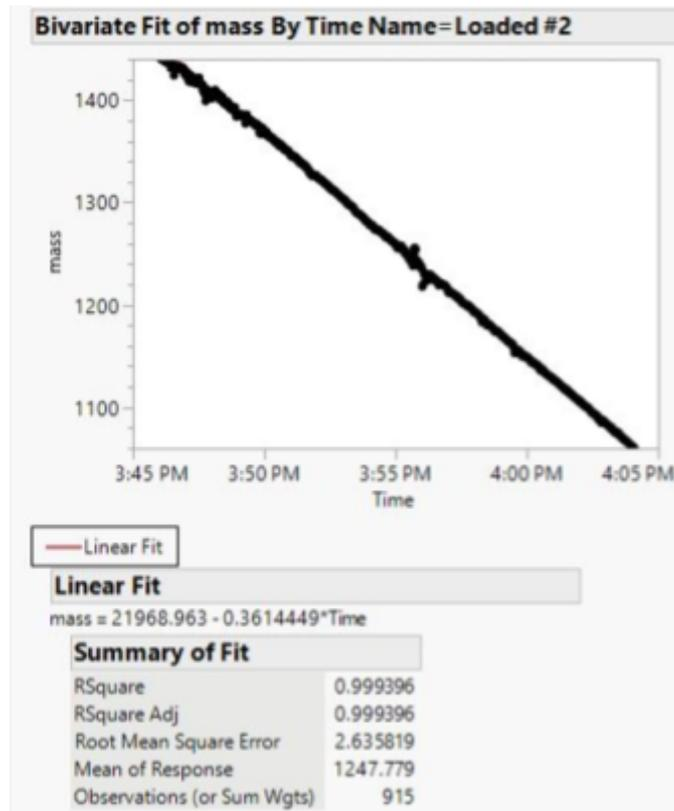
Figure XX. Linear regression of Loaded#2 test. A slope of -0.361 grams fuel/second is obtained with a coefficient of determination (R<sup>2</sup>) value of 0.999396.
