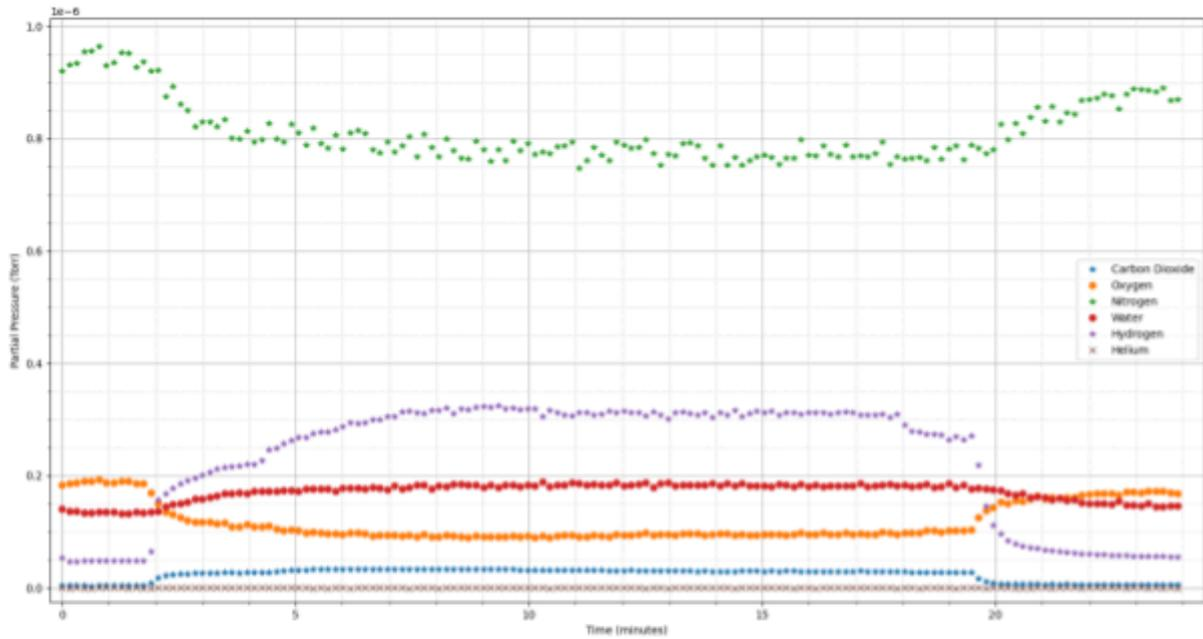
Figure XX. Mass spectrometer gas analysis of Loaded#1 generator test. The load was inconsistent during this test due to one of the hotplates continually shutting off and on. Two hot plates were used for the load, one consuming about 1,396 Watts, the second which was shutting off and on, consuming about 1,428 Watts when on.
