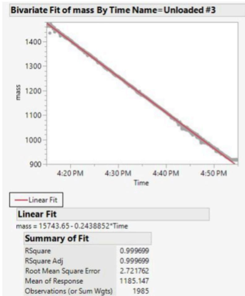
Figure XX. Linear regression of Unloaded#3 test. A slope of -0.244 grams fuel/second is obtained with a coefficient of determination ( $R^2$ ) value of 0.999699.
