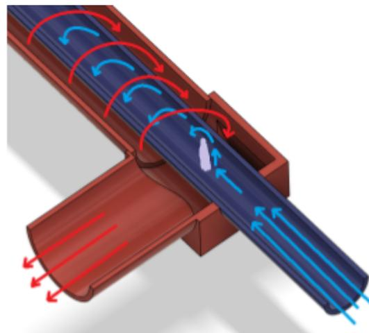
Figure 12. Exhaust (red arrows) and intake air (blue arrows) idealized fluid flows in the bottom region of the vortex tube. The blue inner tube extends all the way up to the spherical region.
