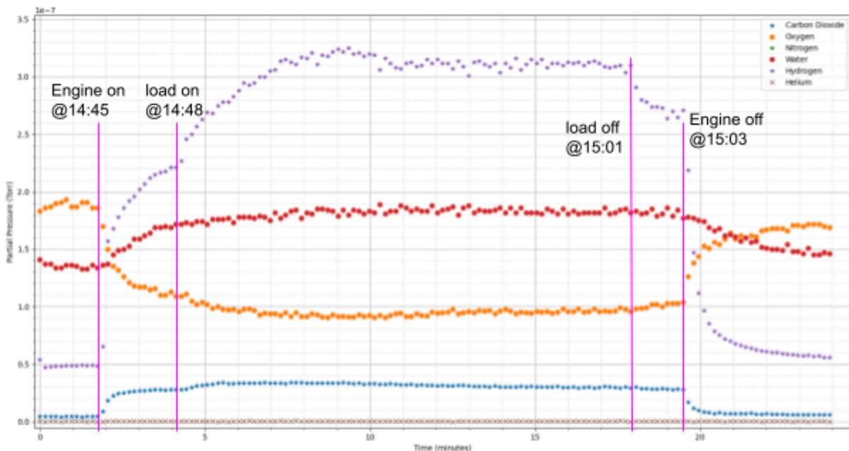
Figure XX. Zoomed in mass spectrometer gas analysis of Loaded#1 generator test. Notice the hydrogen response when load is enabled/disabled.
