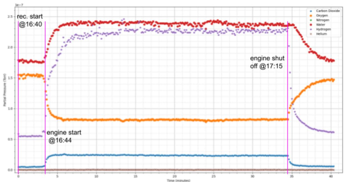
Figure XX. Mass spectrometer gas analysis of first attempted loaded generator start-up/priming run. This is a zoomed in view excluding the nitrogen signal to show better resolution of carbon dioxide. Pink vertical lines are used to roughly indicate relevant times during the experiment.
