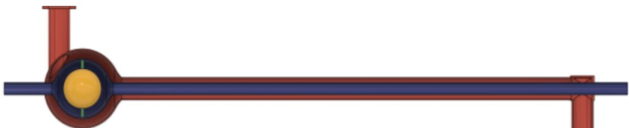
Figure 10. A CAD model representation of the Thunderstorm Generator used during the TGR system demonstration witnessed by the author. Red regions are the “hot” exhaust flow areas. Blue regions are the “cold” intake air flow areas. Exhaust gasses travel from left to right, cold intake air travels from right to left.
