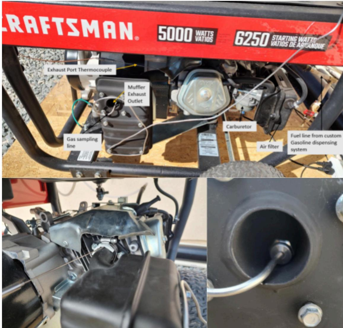
*Figure XX.* Engine side view of the Craftsman model CMXGGAS030731 generator used for the experiments in this work. The only modifications in this setup are a custom fuel dispenser, and removal of the flame arrestor screen from the muffler. Bottom left depicts where the exhaust port temperature is sampled. Bottom right depicts the insertion of the continuous gas sampling line into the muffler exhaust outlet.
