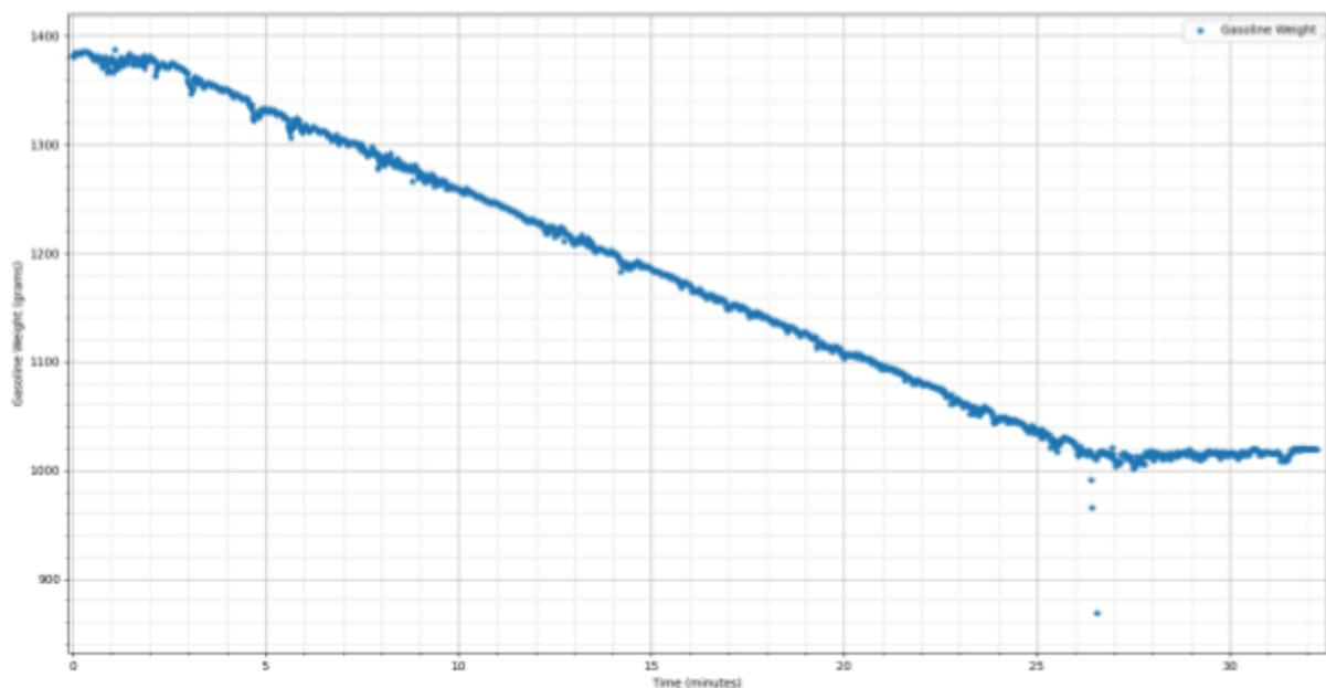
Figure XX. Weight of graduated cylinder containing gasoline during Unloaded#1 generator test. The linear decline middle portion was regressed to obtain fuel consumption rate. A rate of 0.247 grams/second (0.889 kg/hr) was obtained. Pink vertical lines are used to roughly indicate relevant times during the experiment.
