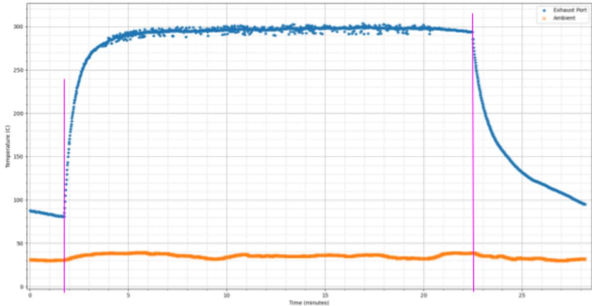
Figure XX. Exhaust port and ambient temperatures during Loaded#2 generator test. Signal noise induced by the generator can be seen on the exhaust port temperatures starting ~4.5 minute mark, and ending ~20.5 minute mark. Pink vertical lines are used to roughly indicate relevant times during the experiment.
