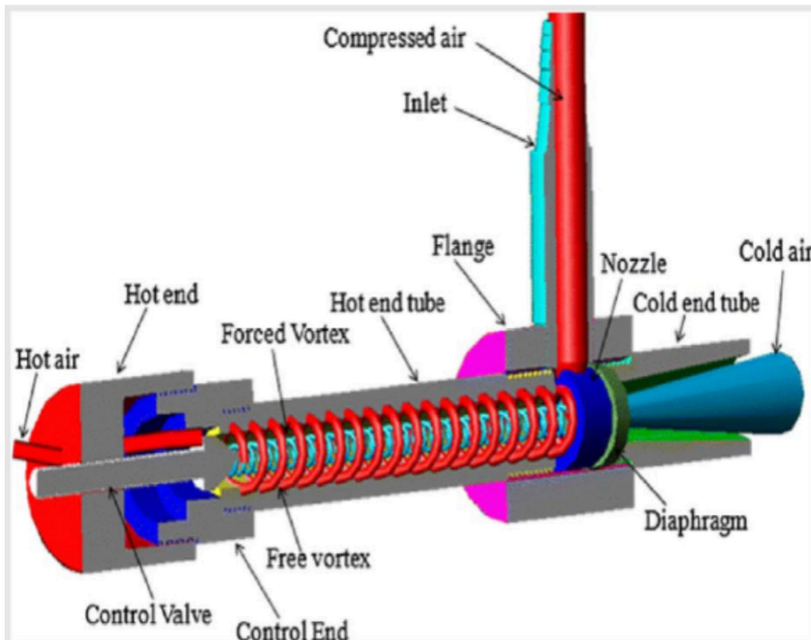
Figure 8. Sectional view of a conventional Ranque-Hilsch vortex tube. Compressed air is fed through the inlet into the swirl guide, forming a free “hot” vortex. A fraction of the free “hot” vortex is let out through the hot end of the tube via the control valve, the rest of the vortex is reflected forming the forced “cold” vortex circulating opposite of the free “hot” vortex. The forced “cold” vortex exits the tube through the cold end, opposite the hot end. (6)
