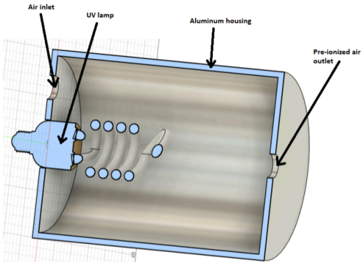
Figure 5. Cross sectional view of the pre-ionizer unit labeled #1 in Figure 3.
