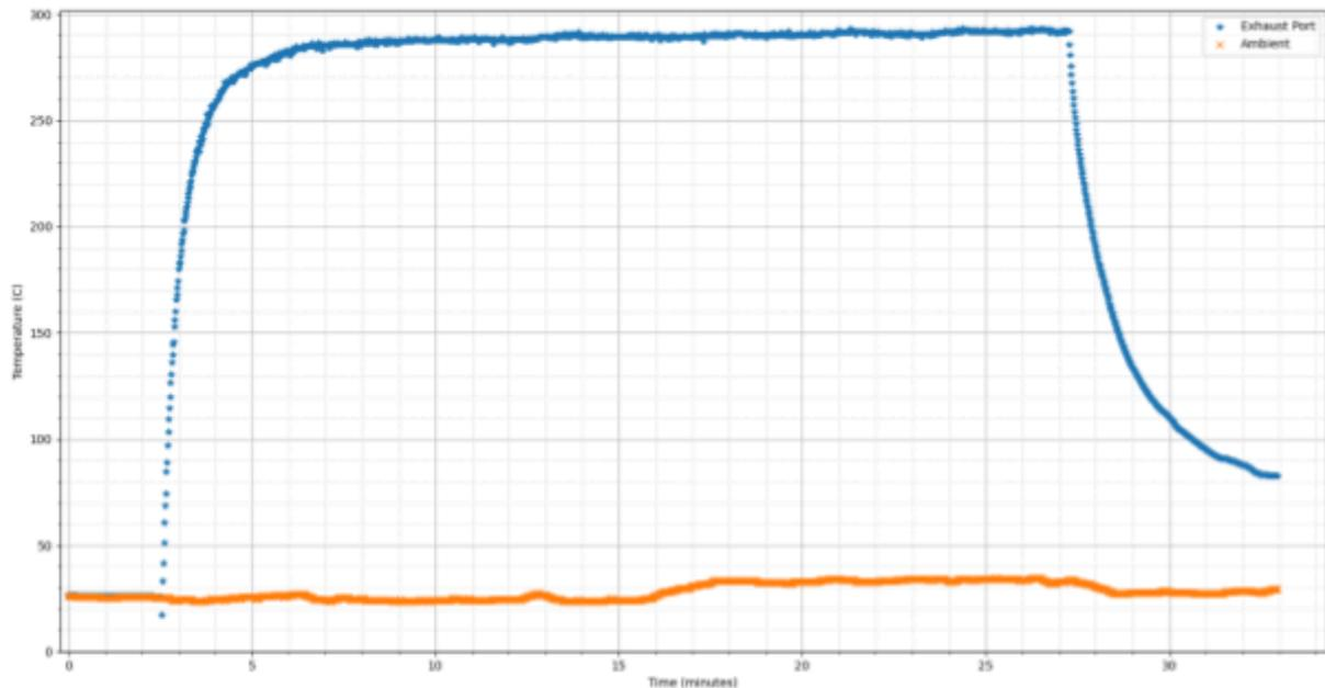
Figure XX. Exhaust port and ambient temperatures during Unloaded#1 generator test. Pink vertical lines are used to roughly indicate relevant times during the experiment.
