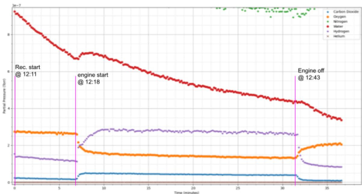
Figure XX. Zoomed in mass spectrometer gas analysis of Unloaded#1 generator test. The large decreasing water peak is due to water condensate trapped inside the sampling line, as can be seen in the following tests, the water behaviour returned to normal after the line was vacuum purged.
