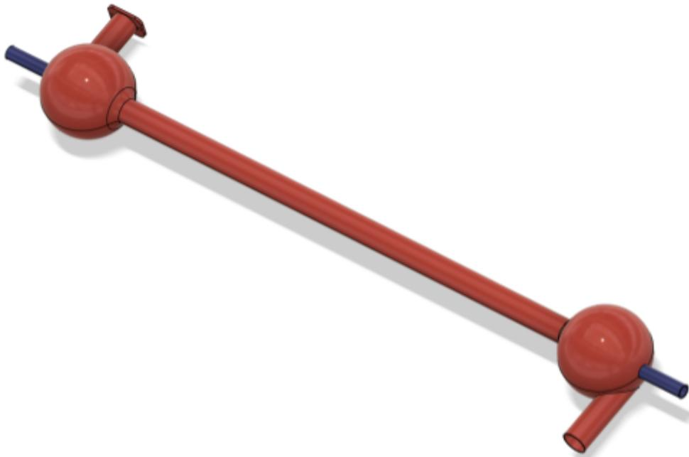
Double sphere vortex tube. Ideal design including smooth transitions from spheres to center tubes.
