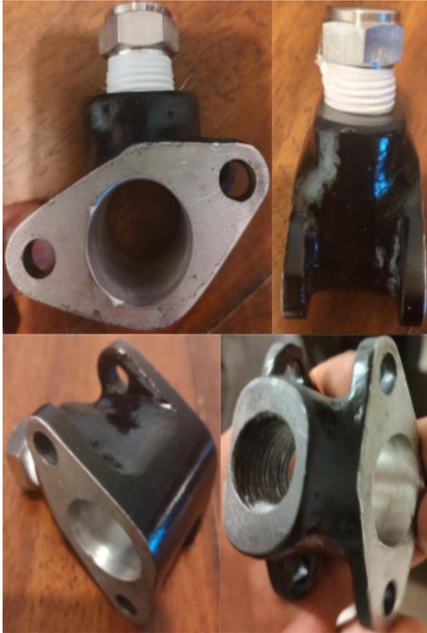
*Figure XX.* Aluminum intake air inlet to be placed between engine and carburetor. The bore is a 1" diameter. The connection is threaded 1/2" NPT. Fabricated by Robert Hutchings.
