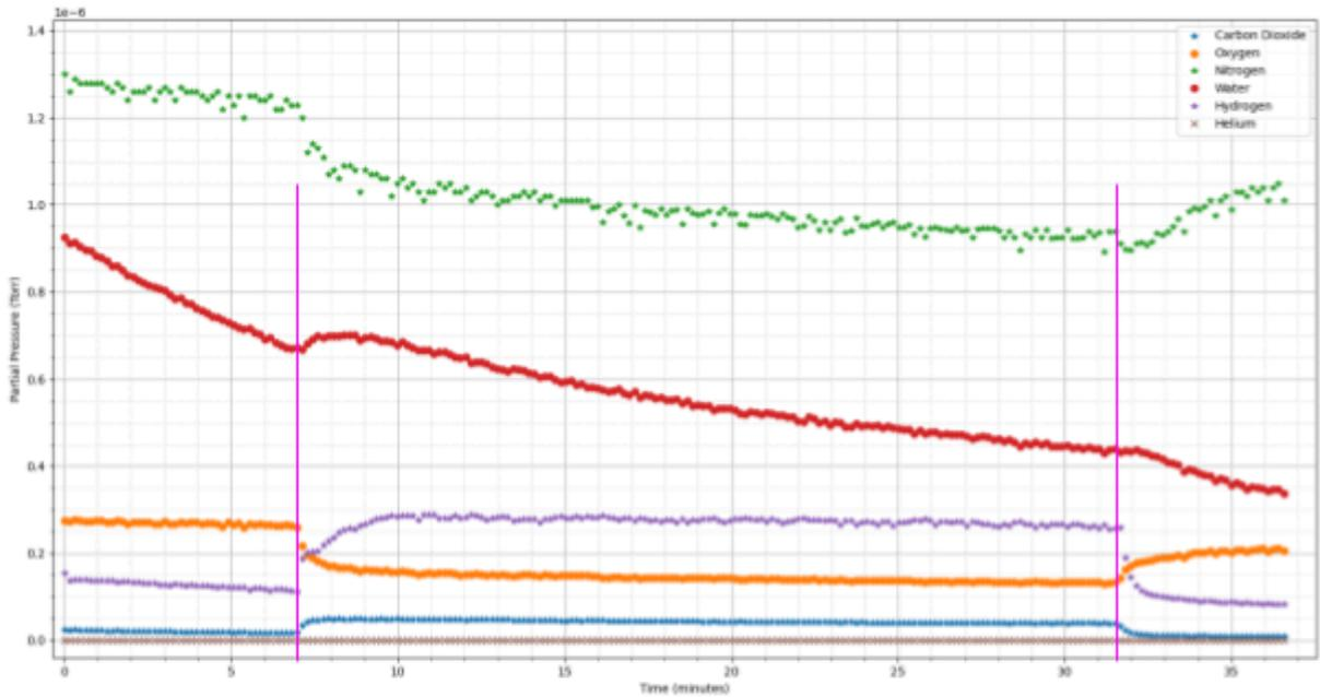
Figure XX. Mass spectrometer gas analysis of Unloaded#1 generator test. The large decreasing water peak is due to water condensate trapped inside the sampling line, as can be seen in the following tests, the water behaviour returned to normal after the line was vacuum purged.
