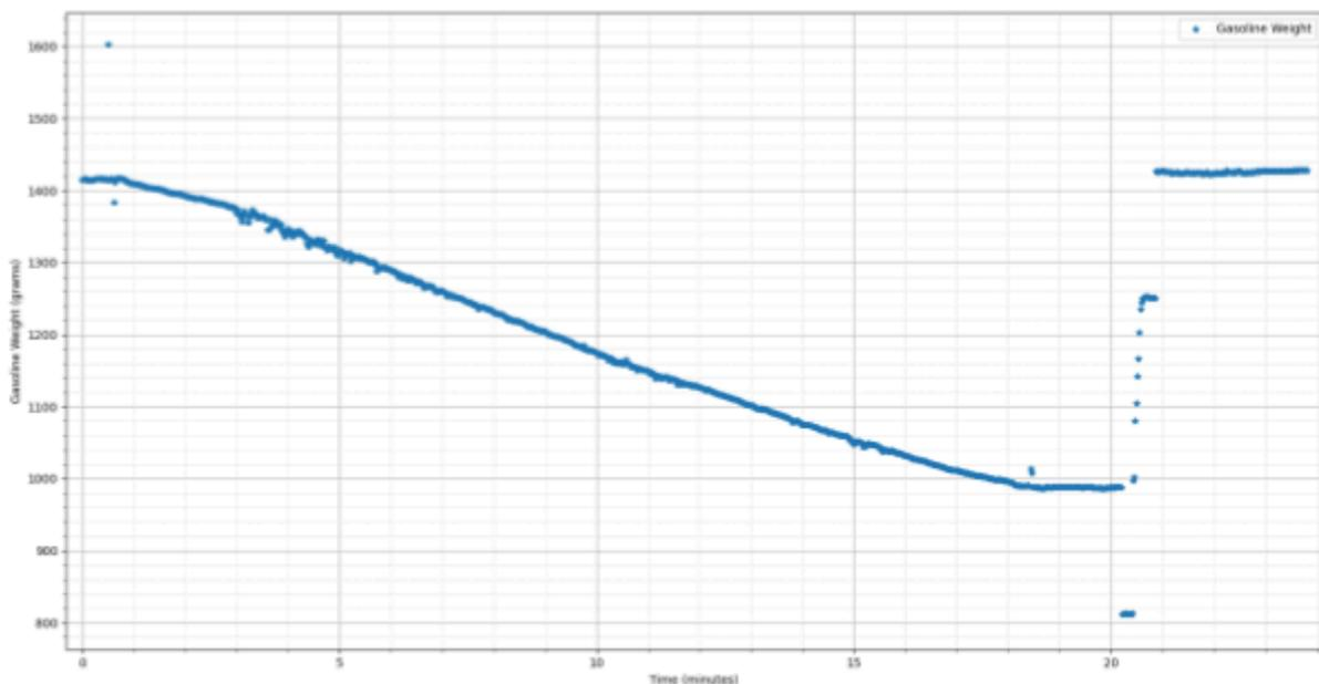
Figure XX. Weight of graduated cylinder containing gasoline during Loaded#1 generator test. The linear decline middle portion was regressed to obtain fuel consumption rate. A rate of 0.432 grams/second (1.555 kg/hr) was obtained. Pink vertical lines are used to roughly indicate relevant times during the experiment.
