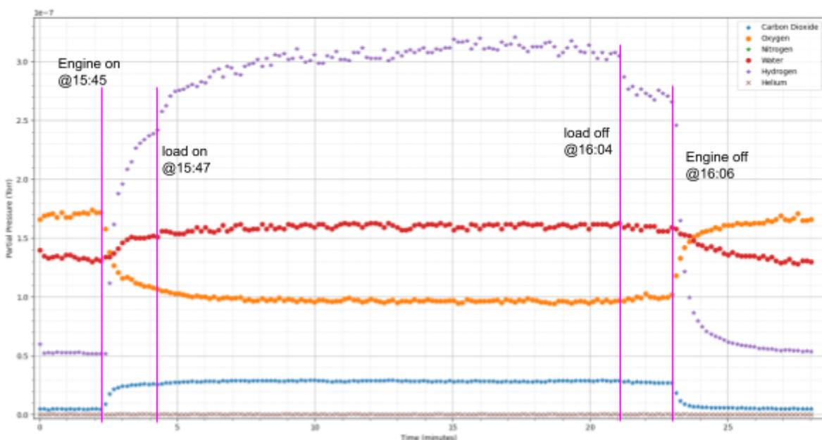
Figure XX. Zoomed in mass spectrometer gas analysis of Loaded#2 generator test.
