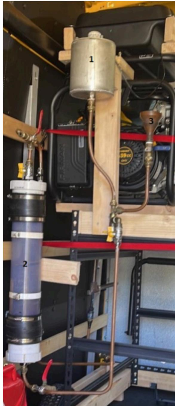
Figure 3. A side view of the TGR system depicting the air pre-ionizer (#1), bubbler/diffusor unit (#2), water feed funnel (#3). Intake air is pulled into the pre-ionizer, travels down through the pipe, and enters the bottom of the bubbler/diffusor unit.
