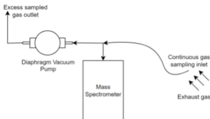
Figure XX. Diagram of continuous gas sampling and analysis system.
