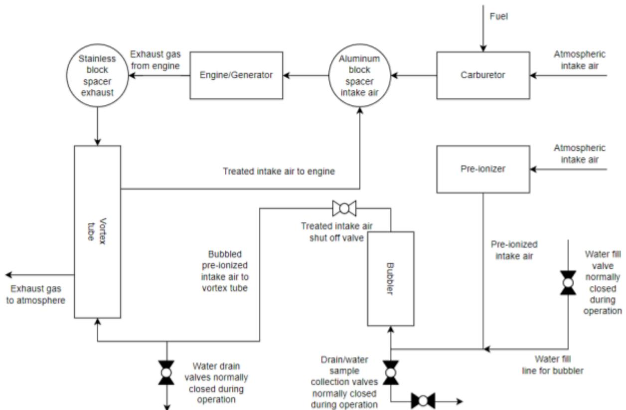
Figure 14. Process flow schematic of retrofit replication experiment.
