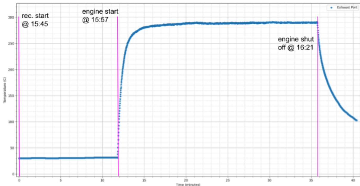
Figure XX. Exhaust port temperature during first unloaded generator startup/priming test. Pink vertical lines are used to roughly indicate relevant times during the experiment.
