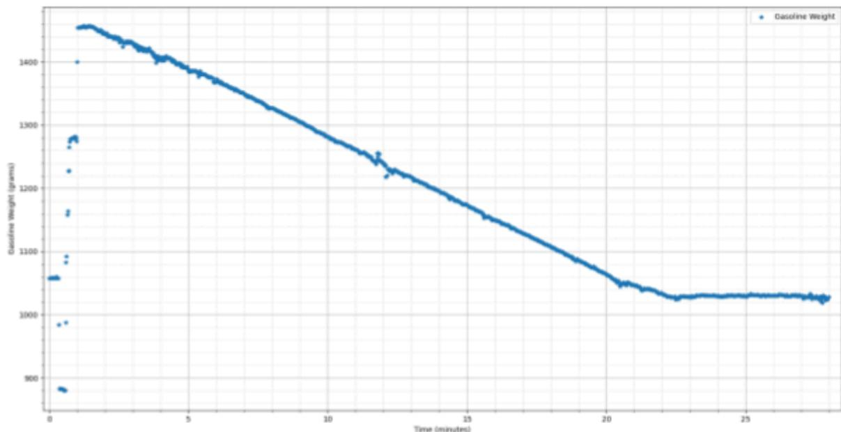
Figure XX. Weight of graduated cylinder containing gasoline during Loaded#2 generator test. The linear decline middle portion was regressed to obtain fuel consumption rate. A rate of 0.361 grams/second (1.300 kg/hr) was obtained. Pink vertical lines are used to roughly indicate relevant times during the experiment.
