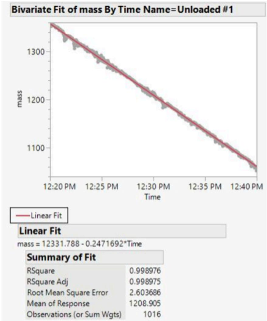
Figure XX. Linear regression of Unloaded#1 test. A slope of -0.247 grams fuel/second is obtained with a coefficient of determination ( $R^2$ ) value of 0.998976.
