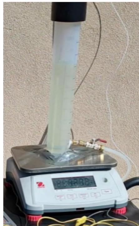
Figure XX. Metered fuel dispensing system used during experiments. Gasoline weight is recorded once per second.
