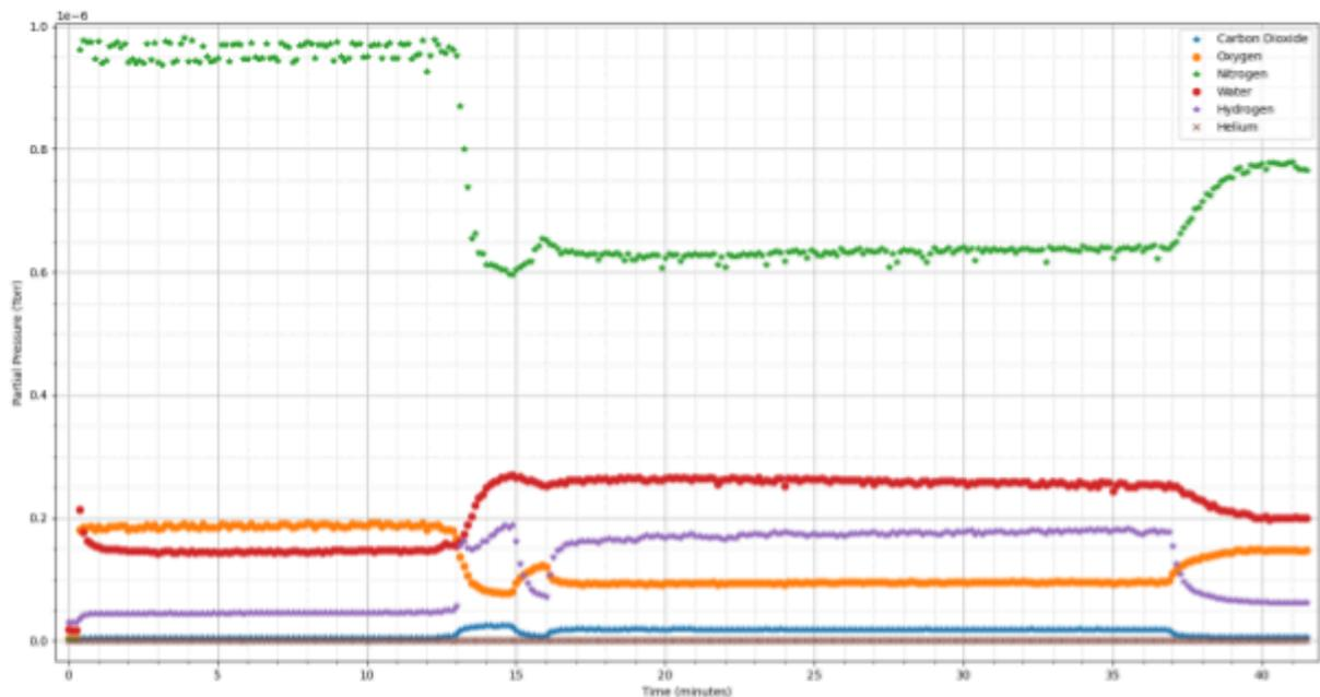
Figure XX. Mass spectrometer gas analysis of first unloaded generator start-up/priming run. Peak disruptions beginning around 15 minutes are due to the sampling inlet disconnecting from exhaust outlet. The sampling inlet was reconnected around the 16 minute mark on the graph.
