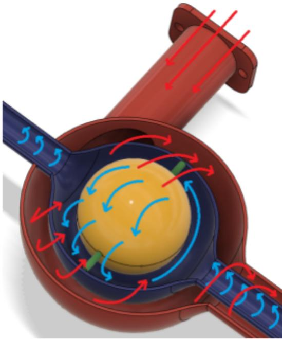
Figure 11. Exhaust (red arrows) and intake air (blue arrows) idealized fluid flows in the spherical region of the vortex tube.
