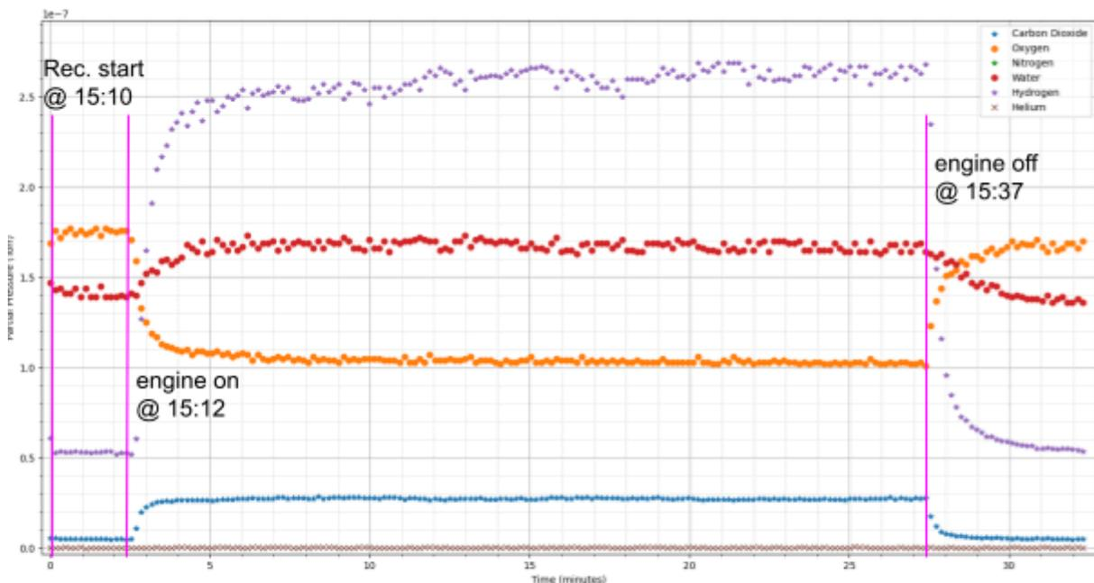
Figure XX. Zoomed in mass spectrometer gas analysis of Unloaded#2 generator test.
