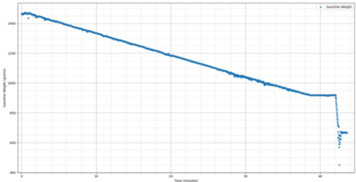
Figure XX. Weight of graduated cylinder containing gasoline during Unloaded#3 generator test. The linear decline middle portion was regressed to obtain fuel consumption rate. A rate of 0.244 grams/second (0.878 kg/hr) was obtained. Pink vertical lines are used to roughly indicate relevant times during the experiment.
