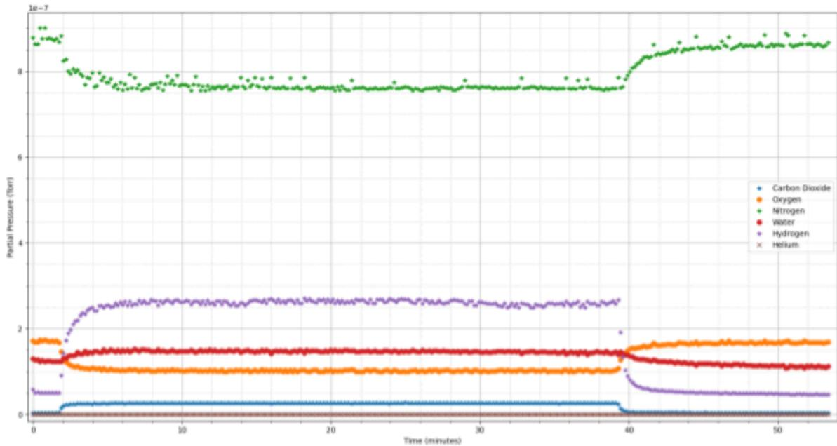
Figure XX. Mass spectrometer gas analysis of Unloaded#3 generator test.
