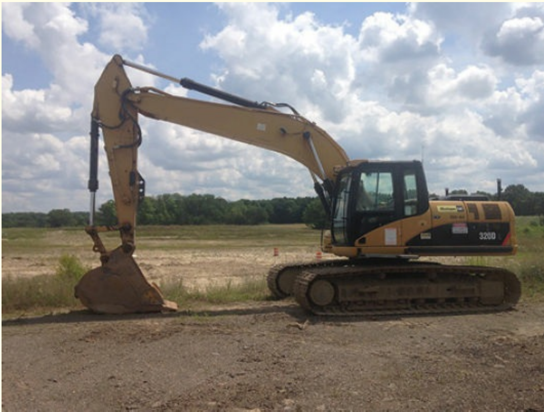
FIGURE 10-22 An excavator consists of an articulated arm, bucket, and cab mounted on a pivot.
