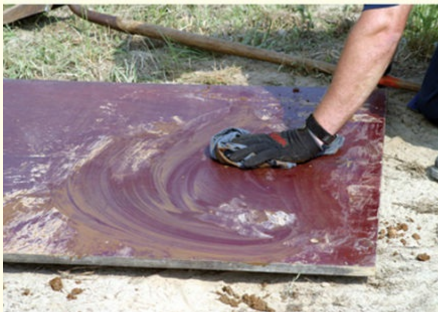
FIGURE 6-10 A. The ShorForm panel is a concrete form used as sheeting material for trench rescue operations. Although very strong, its primary purpose is to hold back running material. B. The resin-impregnated exterior of the ShorForm panel makes cleaning and upkeep easier.
