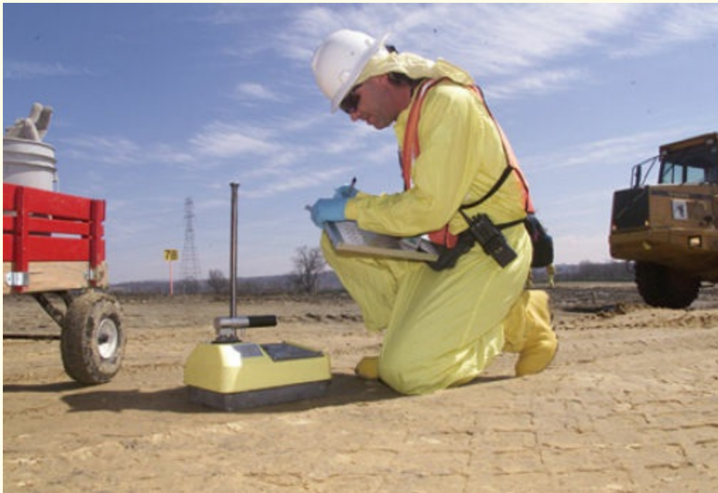
FIGURE 3-18 A nuclear moisture density gauge is a field instrument used to determine soil density and moisture. Courtesy of DOE and Fluor Fernald
