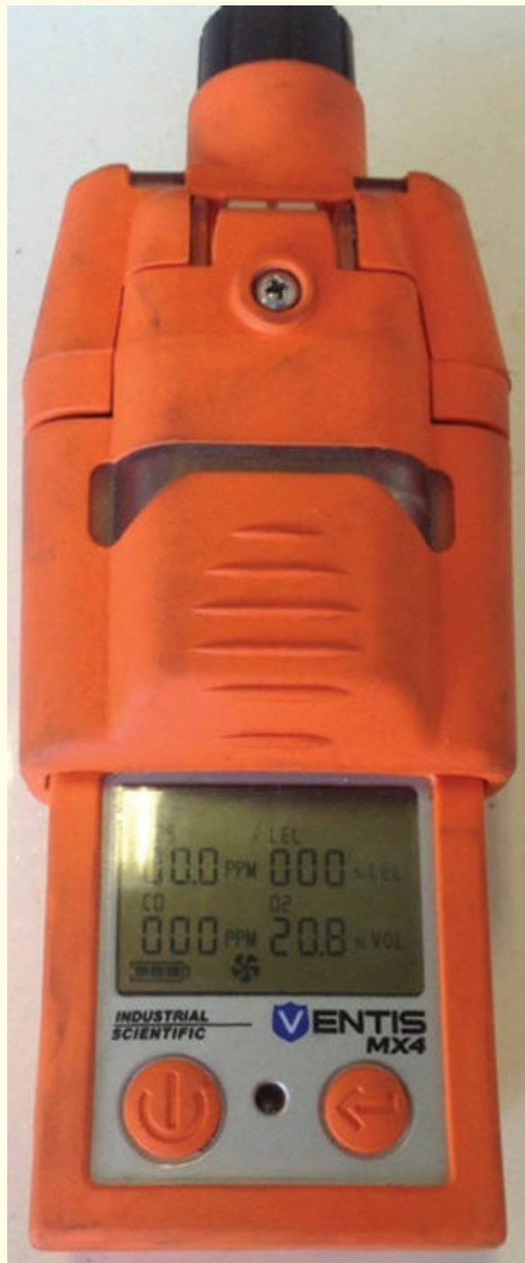
FIGURE 8-9 Rescue personnel should monitor for oxygen, flammability, and toxicity. Courtesy of Cecil V. “Buddy” Martinette, Jr. and Industrial Scientific
