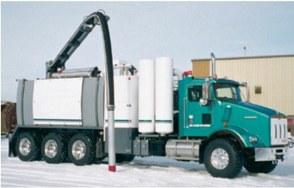
FIGURE 12-10 Hydro vac trucks reduce the soil to a product that can be picked up easily by the vacuum. Courtesy of Badger Daylighting
