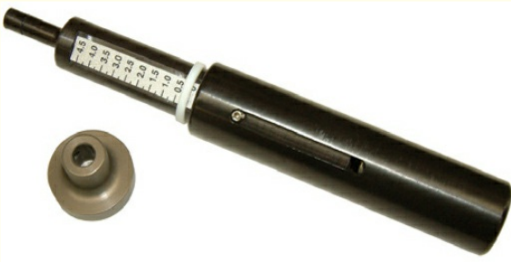
FIGURE 3-14 The penetrometer is a field instrument that is used to determine soil strength. Courtesy of Cecil V. "Buddy" Martinette, Jr.
