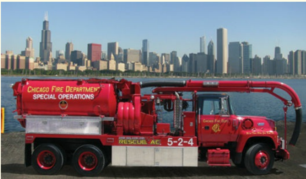
FIGURE 12-9 Centrifugal vacuum truck. Courtesy of Rescue Vac
