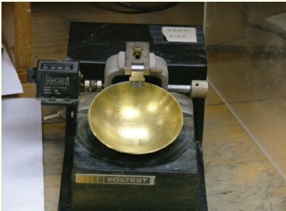
FIGURE 3-17 The Atterberg testing instrument is primarily used to determine a soil's liquid limit and plasticity. Courtesy of Cecil V. "Buddy" Martinette, Jr.
