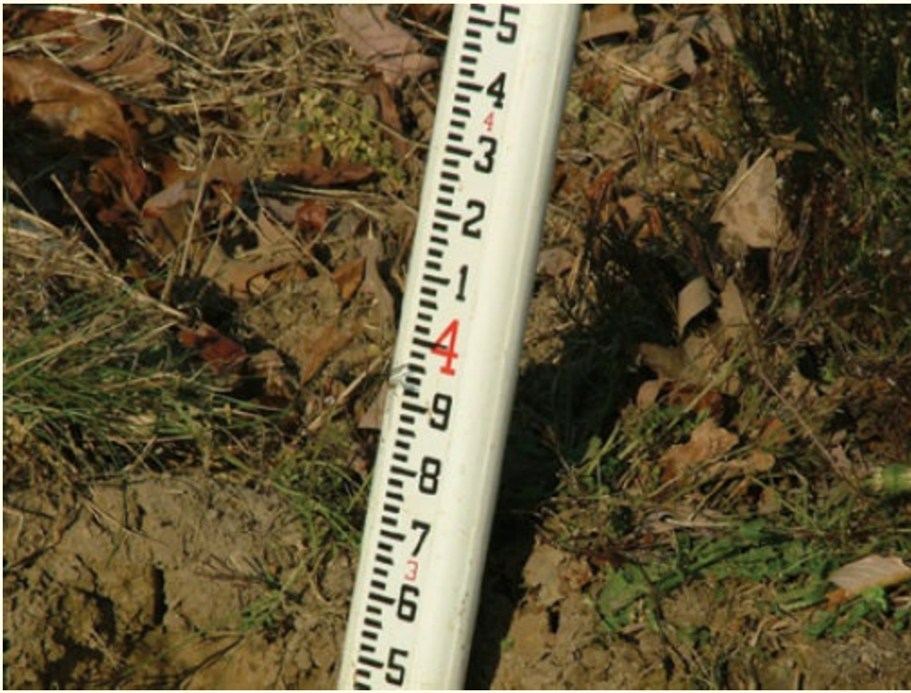
FIGURE 7-6 Grade poles can yield information about trench depth before collapse. Courtesy of Cecil V. “Buddy” Martinette, Jr.
