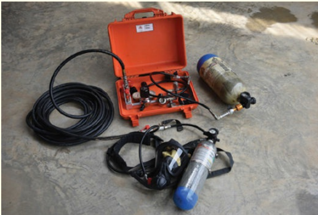
FIGURE 6-5 SABA is compact and can be used as a constant supply of air for trapped victims if SCBA cannot be used.
