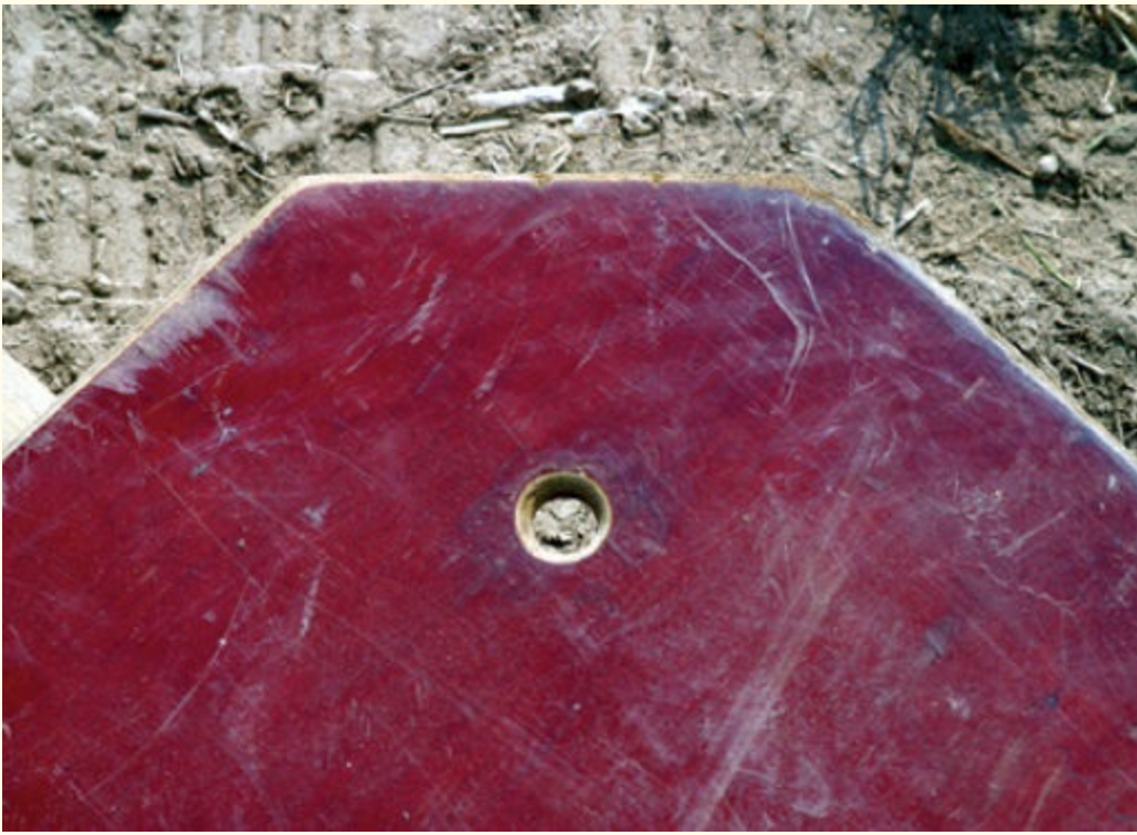
FIGURE 6-11 Cutting panel corners is a method to reduce hazards to rescue personnel; it also helps reduce panel damage.
