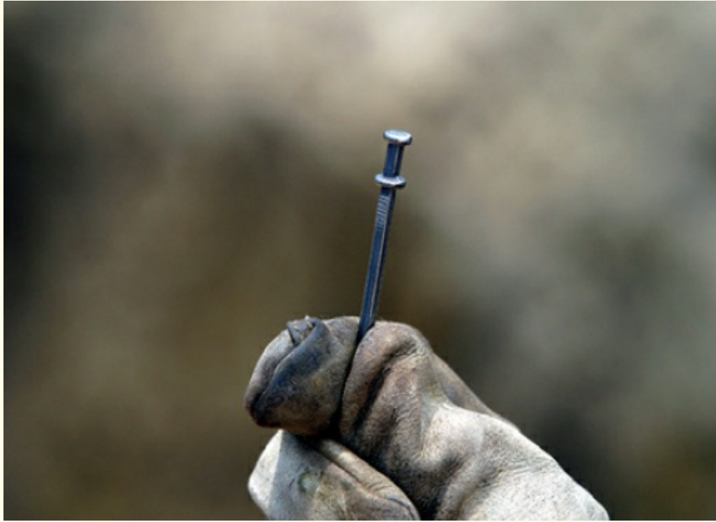
FIGURE 6-20 Duplex nails are two-shoulder nails designed for easy removal after use.
