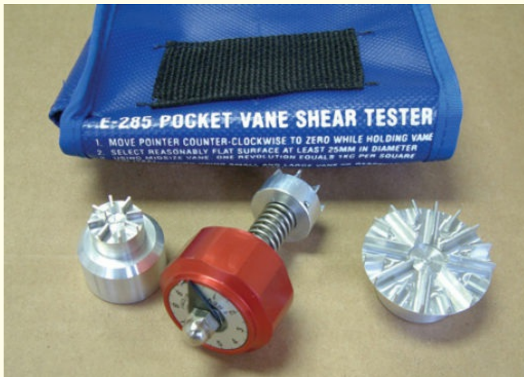
FIGURE 3-15 The shear vane is a type of field testing instrument used to determine soil strength. Courtesy of Geotest Instrument Corp.
