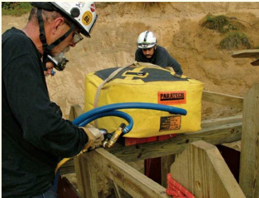
FIGURE 9-17 Low-pressure bags lift limited weight but to a much greater height than high-pressure bags.
