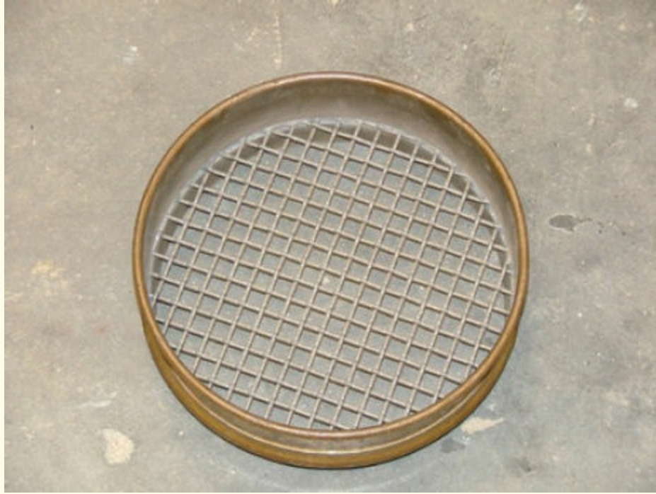
FIGURE 3-16 A soil sieve is used to determine the total makeup of a soil sample.
