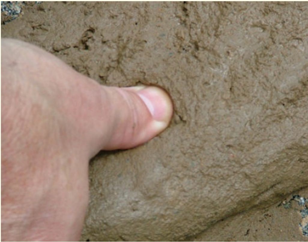
FIGURE 3-13 The degree to which your thumb penetrates a soil sample can indicate the soil's overall strength and its susceptibility to failure. Courtesy of Cecil V. "Buddy" Martinette, Jr.
