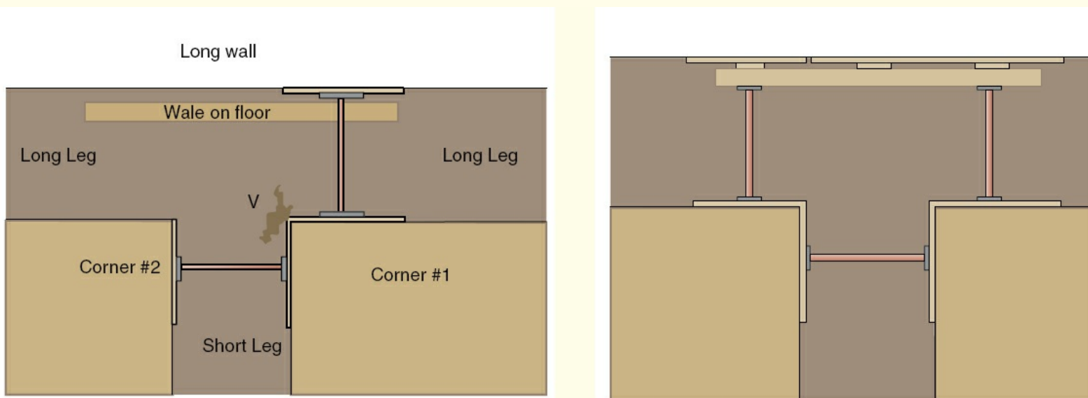
FIGURE 11-12 A. Example of area designations and a primary shoring plan. B. Example of a secondary shoring plan.
