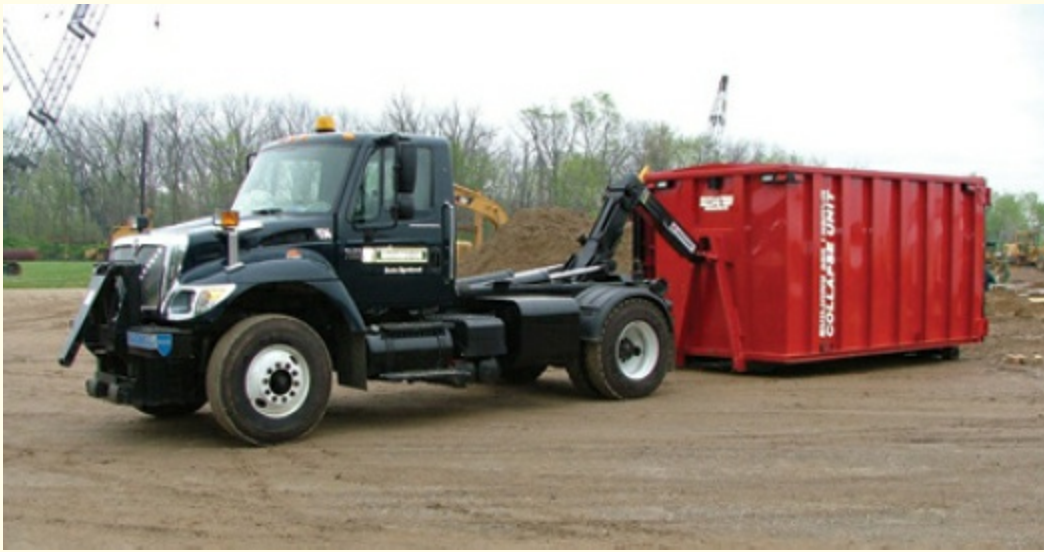
FIGURE 2-14 Pod systems are great for storing equipment by specialized discipline and for enabling quick transport of that equipment to the scene.
