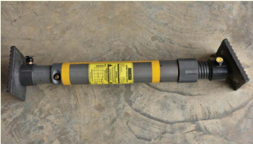
FIGURE 6-16 Pneumatic shores use air from a remote source to expand and then are locked manually.
