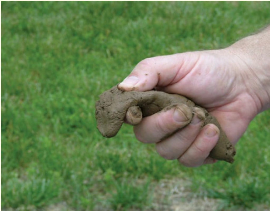
FIGURE 3-12 The ribbon test is used to determine the clay and silt content of soil.
