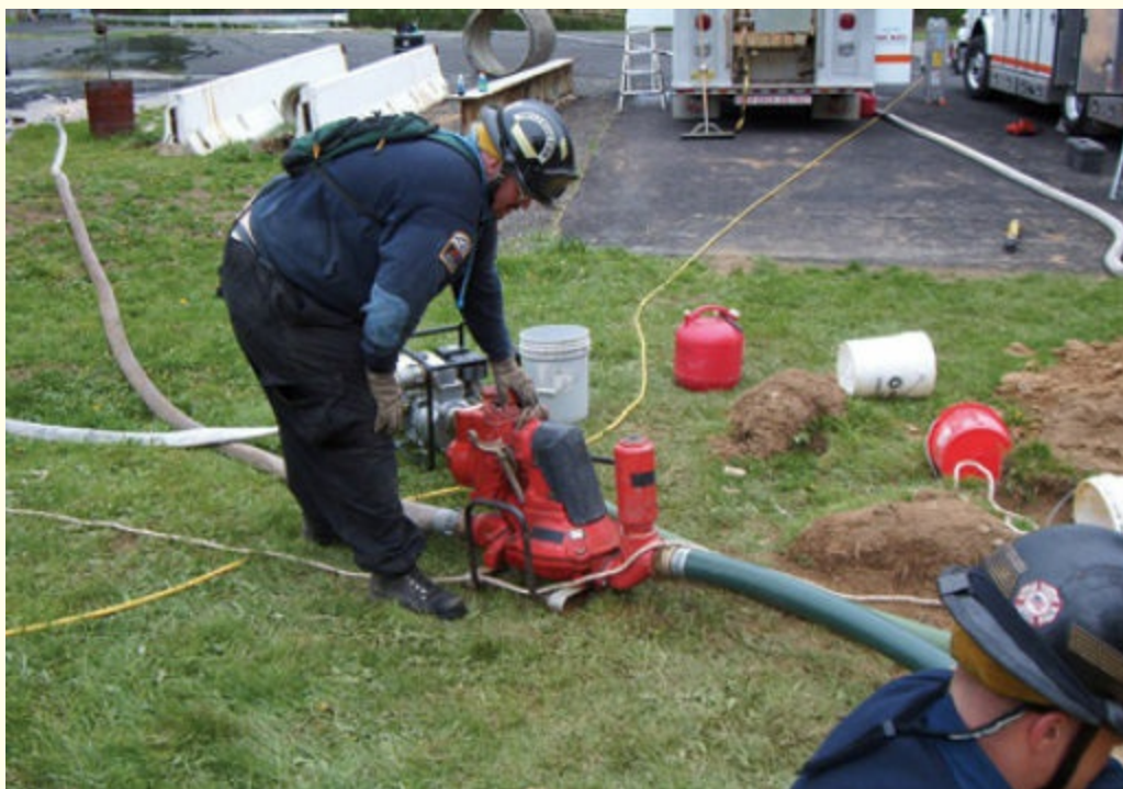
FIGURE 6-24 Mud pumps are very versatile, although they sometimes require extensive priming to pull the vacuum. Courtesy of Bob Schilp
