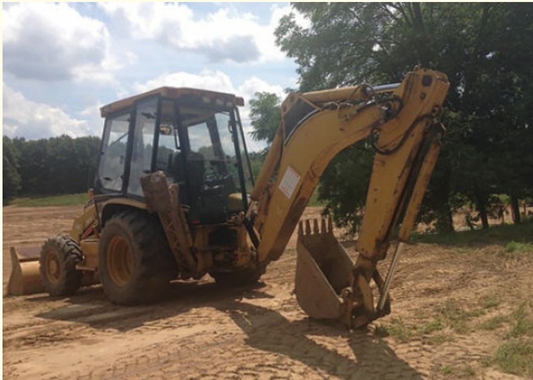
FIGURE 10-21 A backhoe consists of a digging bucket on the end of a two-part articulated arm.
