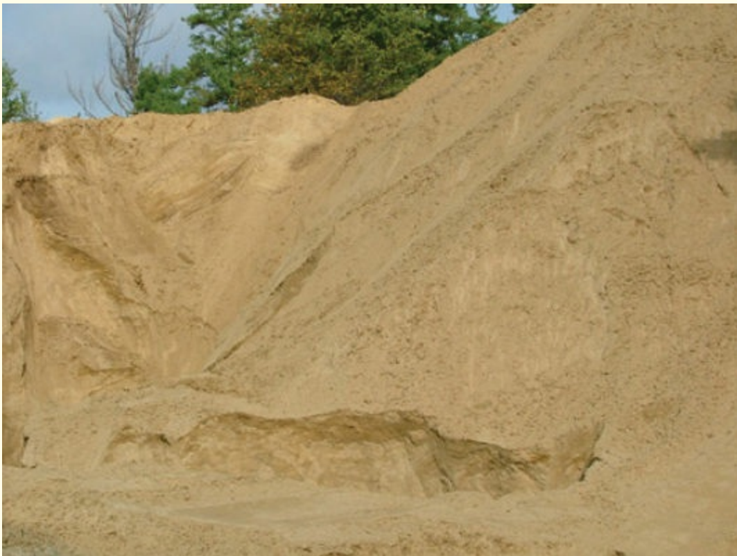
FIGURE 3-20 In some situations, moisture content will allow a running soil to have a steeper than normal angle of repose. Courtesy of Scott Shahan
