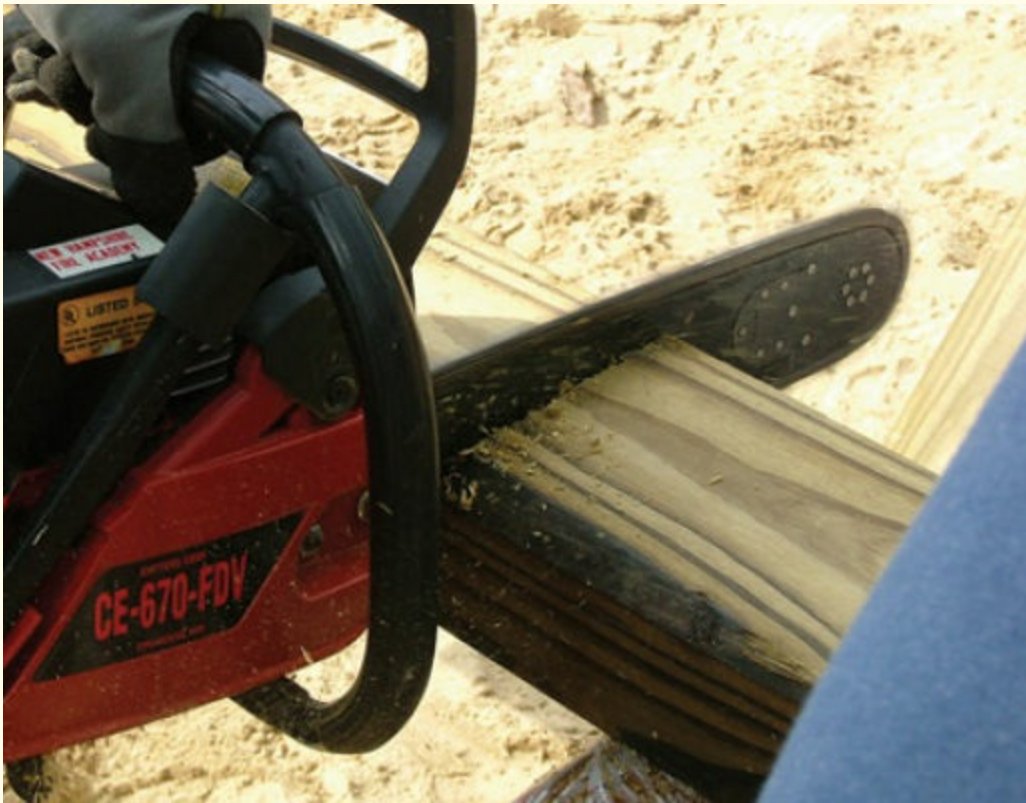
FIGURE 6-21 Extreme caution should be used when cutting shores or other material with a chainsaw. Courtesy of Cecil V. "Buddy" Martinette, Jr.
