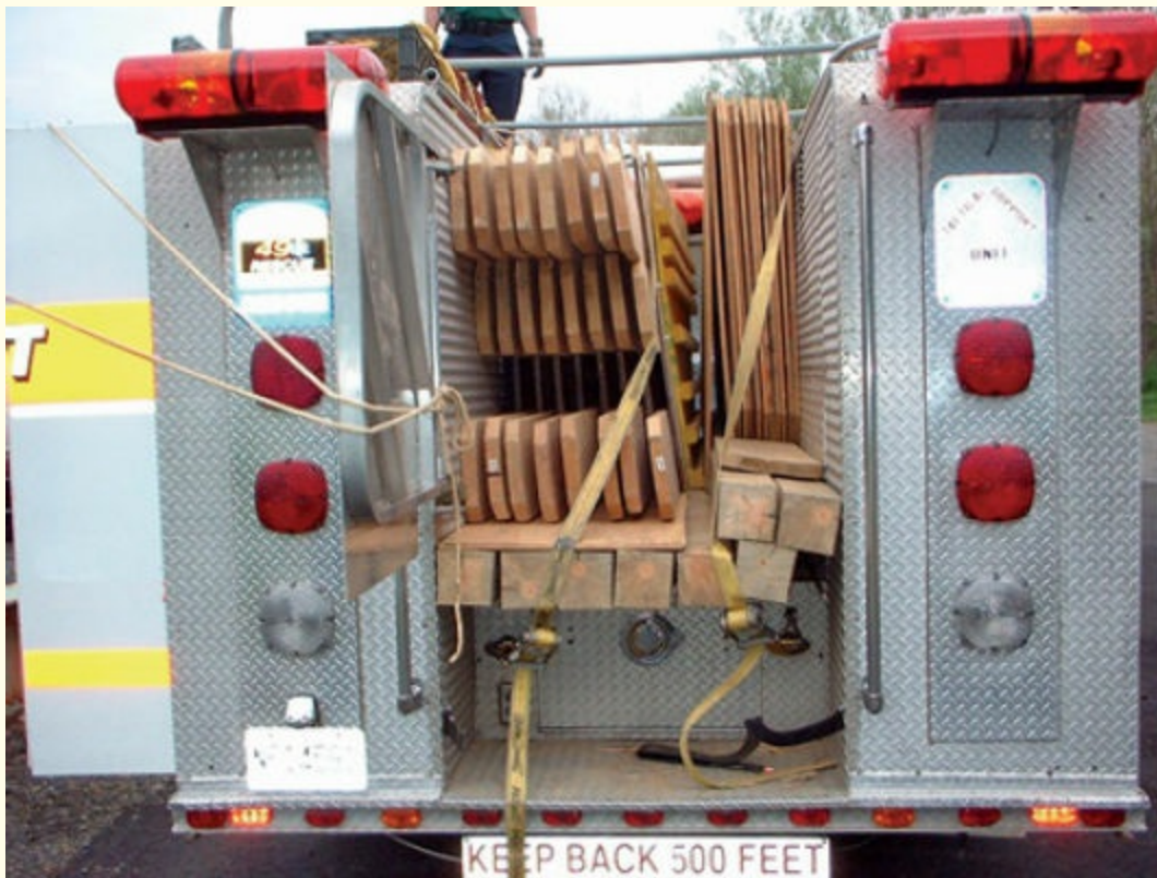
FIGURE 2-5 Medium-duty apparatus are very versatile and allow transport and storage of a wide variety of equipment, but are not very appropriate for trench rescue. Courtesy of Cecil V. "Buddy" Martinette, Jr.
