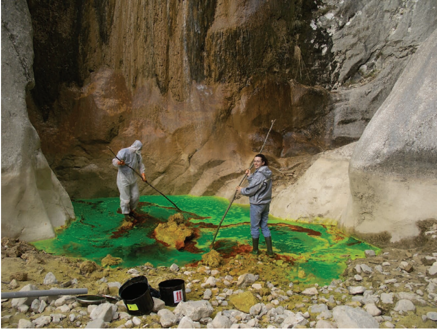
Figure 169. Fluorescein tracer injection in the Cambario Valley (Alpes-Maritimes, France) (photo G. Tennevin ). The tracer is poured into a body of water in the limestone, and flows into the deeper parts of the karstic reservoir before emerging at the submarine Cabbé Spring (Roquebrune-Cap-Martin, France).
