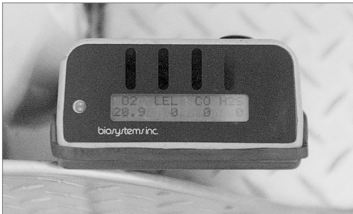
When using a four-function monitor, measure pH, oxygen, flammability, and toxicity, in that order.
