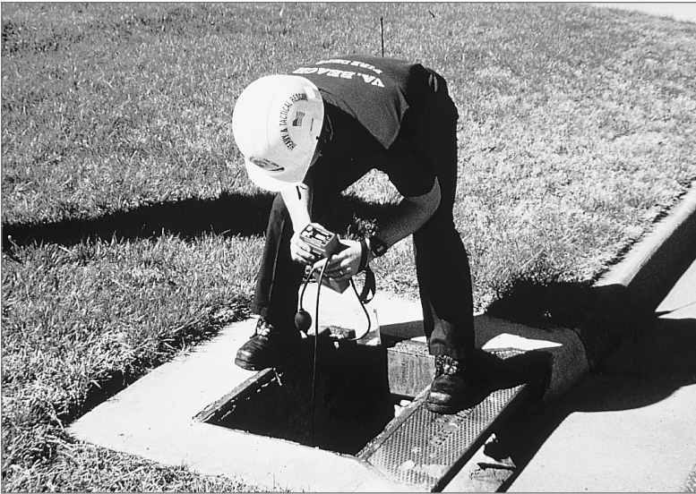
Monitoring a space using a calibrated, bump-checked, and properly maintained detector is the only way to evaluate the atmospheric hazards present.
