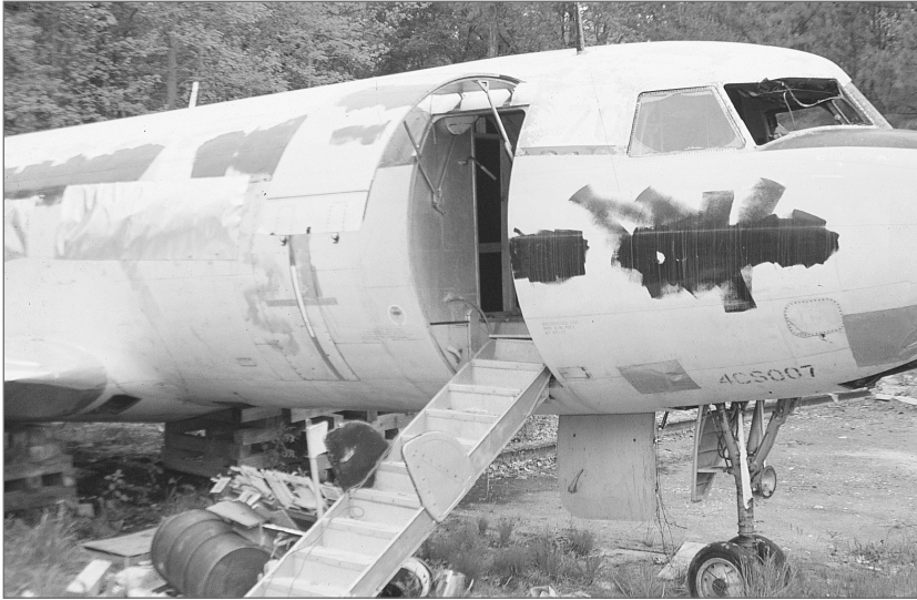
An old airplane fuselage reconfigured inside to create a confined-space training simulator.
