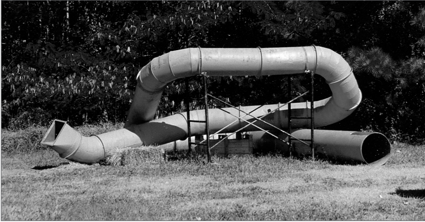
A portable training simulator made from steel pipe.
