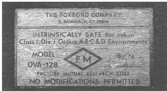
Figure 4.8 Instruments that have been tested and marked as intrinsically safe will not ignite flammable atmospheres.
