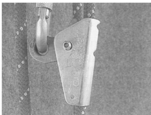
Figure 13.44 When using mechanical rope grabs such as the Gibbs ascender as a ratchet, the arrow should point toward the load when installed on the line opposite the haul line.
