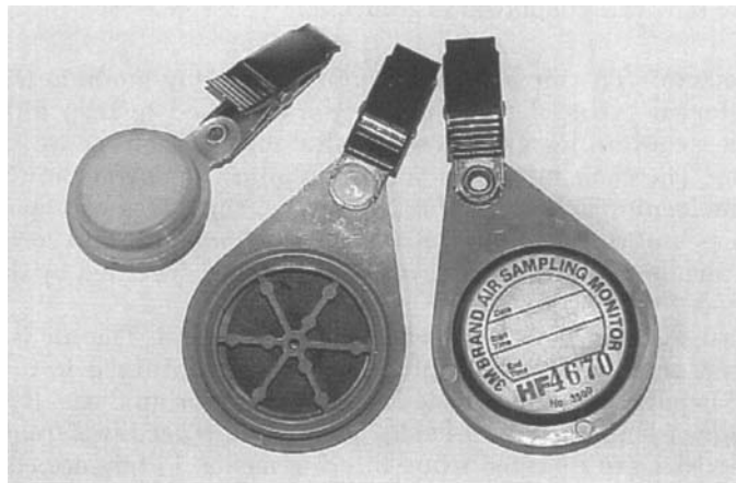
Figure 4.6 Passive sampling is an easy and effective way to measure many toxic gases and vapors.
