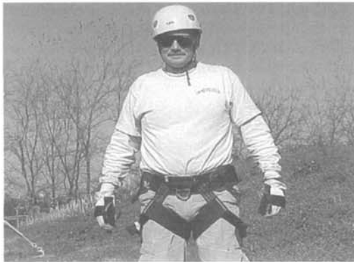
Figure 11.19 The CMC®/Roco™ seat harness is classified as a NFPA class II harness.
