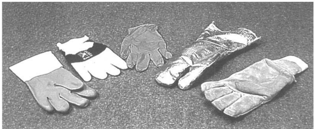
Figure 9.6 Gloves can protect the hand from cuts, burns, abrasion, chemicals, and other hazards.
