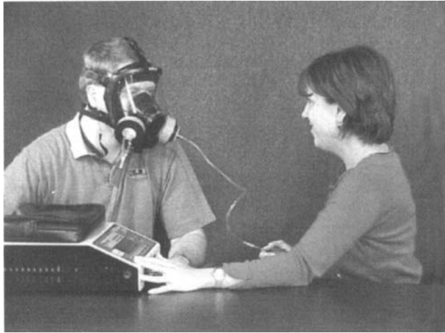
Figure 7.16 Quantitative fit tests provide a numerical fit factor that describes the quality of the fit of a respirator facepiece.
