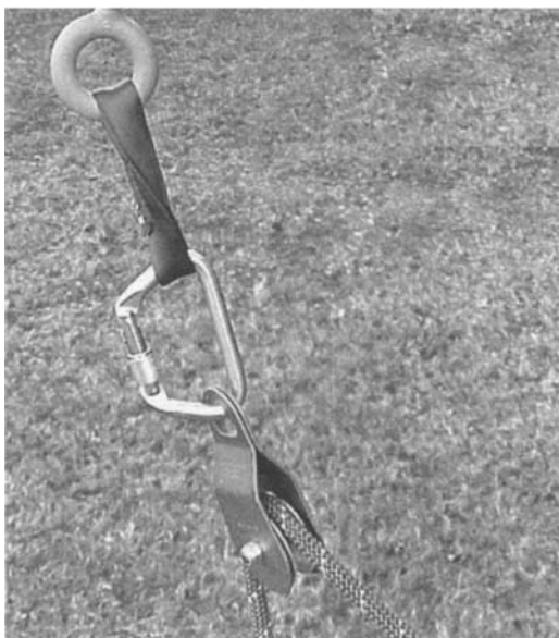
Figure 13.58 Adding a flexible connection between the directional pulley and the anchor attachment will prevent “hard linking.”
