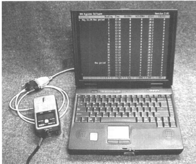
Figure 4.9 The datalogging feature on air monitoring instruments allows readings to be stored and later downloaded to a computer.
