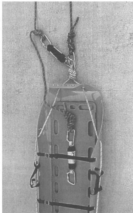
Figure 18.16 This vertical SKED is equipped with a safety belay line rigged to attach to both the rope bridle and the trainee/patient's harness.
