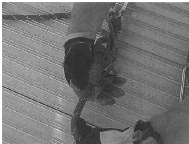
Figure 13.66 To belay a lowering operation with a TPB, hold the Prusik hitch farthest from the anchor in one hand while pulling the belay line through the hitches with the other.
