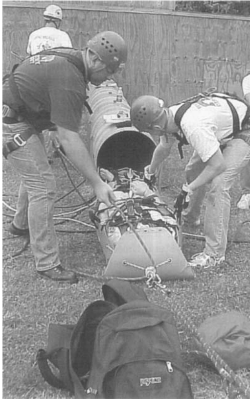
Figure 13.47 MA systems can be used for hauling packaged patients from horizontal spaces.
