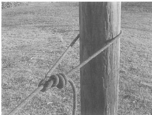
Figure 13.13 The bowline knot can be used to make the attachment to the anchor point. Remember that anytime the bowline is used, there is an approximately 33% loss of strength in the rope.
