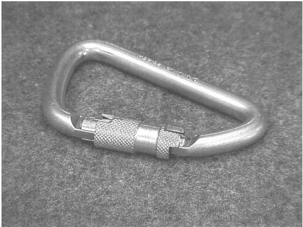
Figure 11.38 The locking nut of the autolocking carabiner requires two motions to open the gate and, once the gate is released, closes and locks itself under spring pressure.
