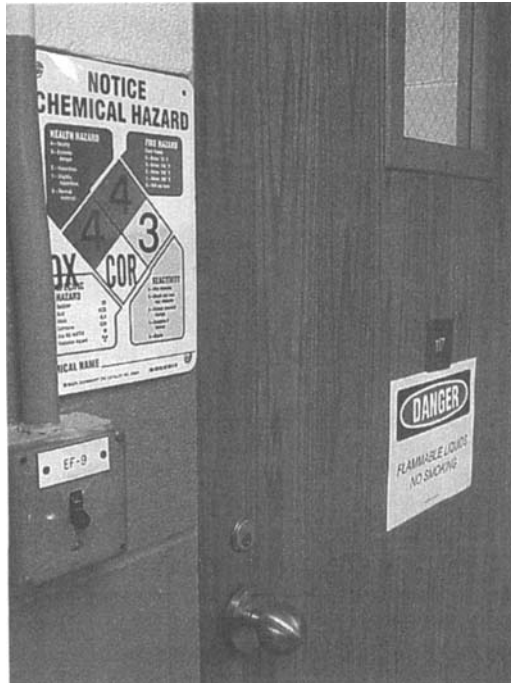
Figure 1.9 Enclosed areas are not considered confined spaces by OSHA if entry and exit are unrestricted, even though hazards to an entrant may be present.
