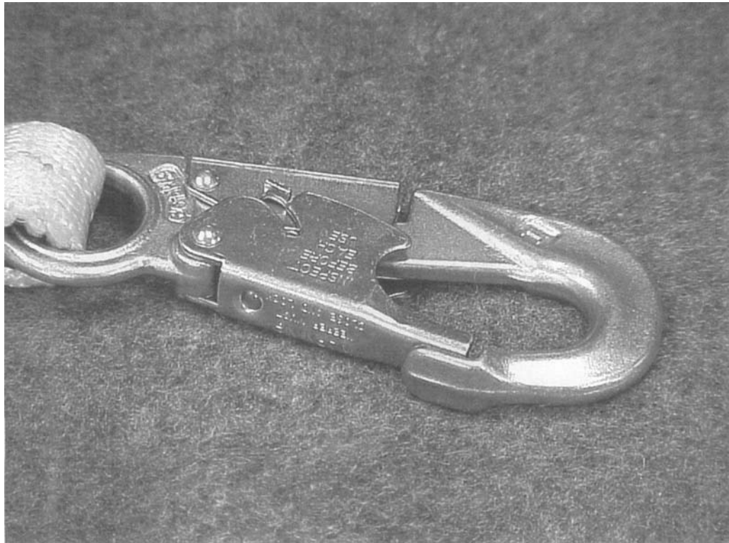
Figure 11.29 The snap hook or “lemon squeezer” has a self-closing, self-locking keeper.
