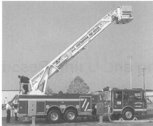
Figure 17.1 Some aerial apparatus can provide a convenient high anchor point for rescue operations.
