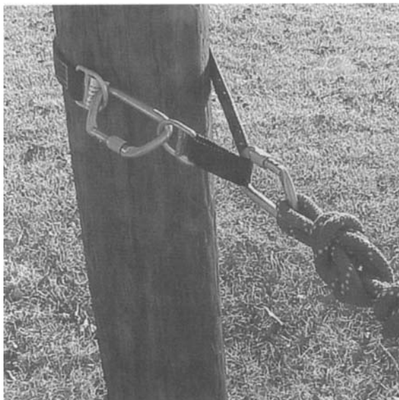
Figure 13.9 This is one method that can be used to avoid triloading carabiners when making anchor attachments.
