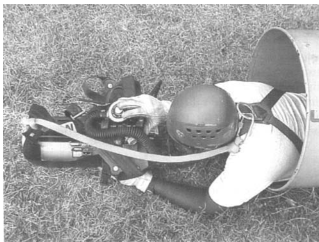
Figure 7.12 A short length of webbing or rope attached between the harness and SCBA can prevent the facepiece from being pulled off the face if the unit is dropped after being doffed for reduced profile entry.
