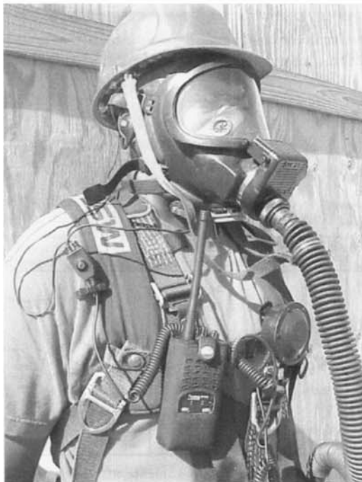
Figure 14.12 Communication equipment may include respirator facepiece voice amplifiers, two-way radios, and intercom systems.
