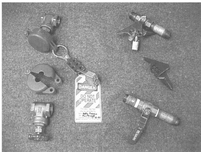
Figure 6.21 Lockout/tagout devices for valves include hoods for gate valve wheels and ball valve lockout devices.
