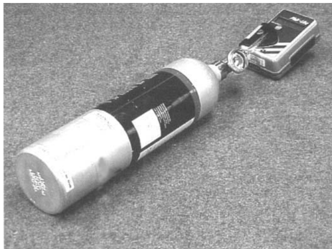
Figure 4.7 Air monitoring instruments must be calibrated against a known concentration of gas, such as from a calibration cylinder.
