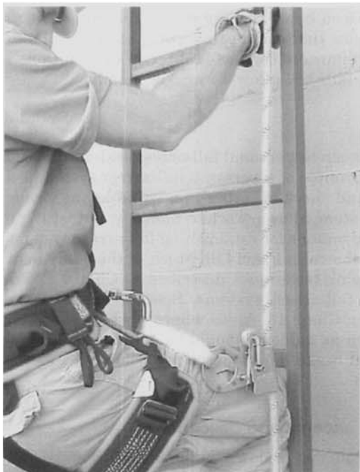
Figure 14.8 In this fall-arrest system the rope grab moves up and down the rope beside the ladder, but locks to the rope if the climber falls.
