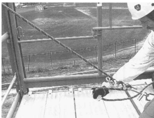
Figure 17.15 When a brake bar rack is used in a lowering system, the lowering line operator can stop the descent of the load quickly by moving the control hand ahead of the rack. The load can be held fast by holding both the control line and the loaded line in the control hand.
