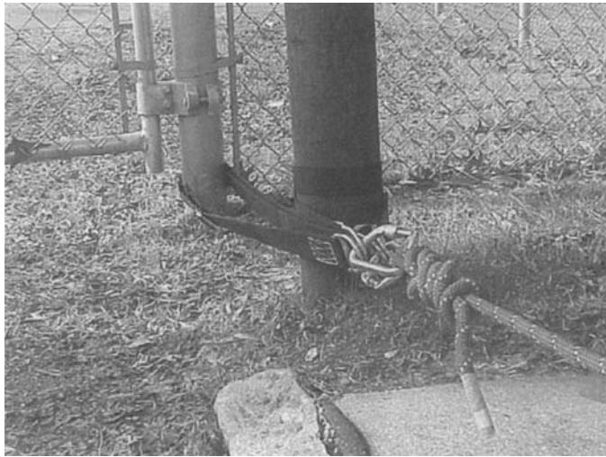
Figure 13.16 The position of the secondary or backup anchor is important. Having the backup anchor directly behind and in line with the primary anchor prevents severe pendulum swings if the primary anchor fails.
