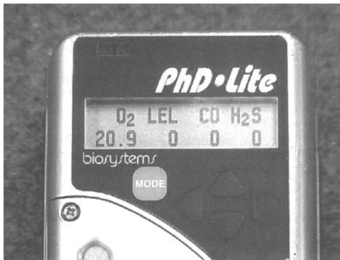
Figure 4.3 Today’s multigas monitors simultaneously measure the hazards listed in OSHA’s order of testing requirements.
