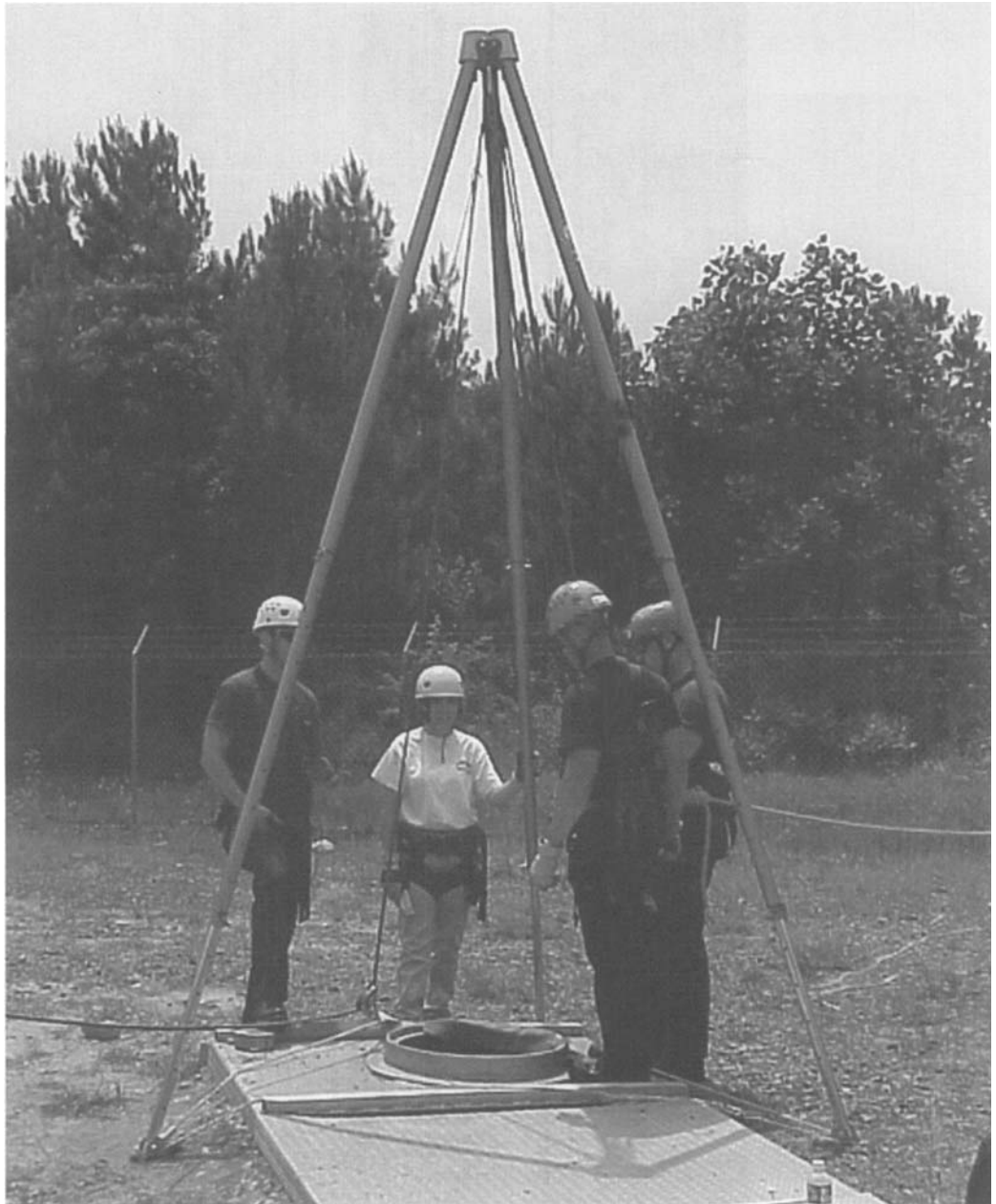
Figure 11.61 A tripod-type portable anchor system with telescoping legs can be adjusted to various lengths to accommodate different entry positions.
