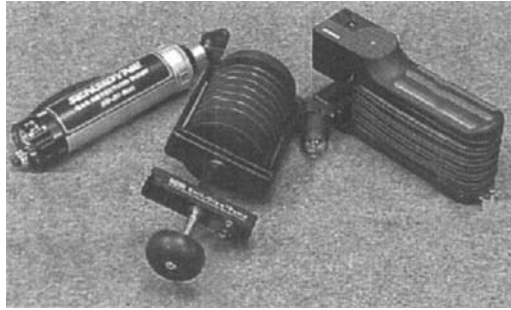
Figure 4.11 Air is drawn through short-term detector tubes with either bellows or piston pumps.
