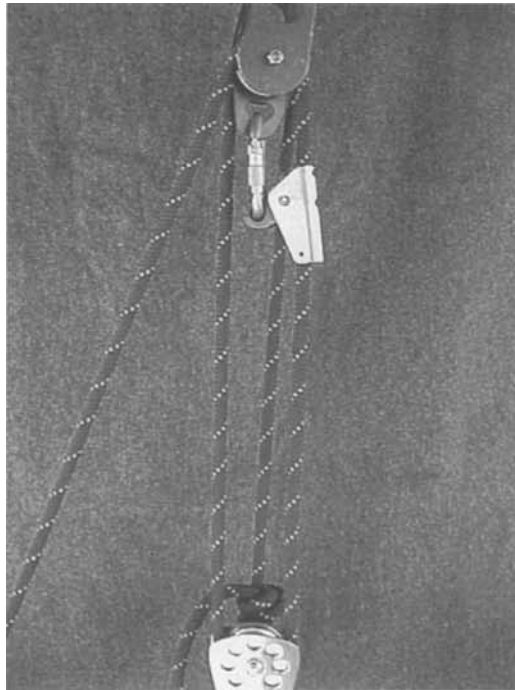
Figure 13.42 A Gibbs ascender is used as a ratchet on this MA system. It is attached to the line opposite the haul line.
