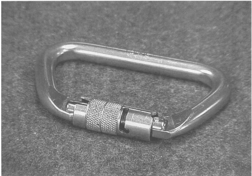
Figure 11.39 The locking nut of the safety-lock carabiner requires three motions to open the gate. Once the gate is released, it closes and locks itself under spring pressure.
