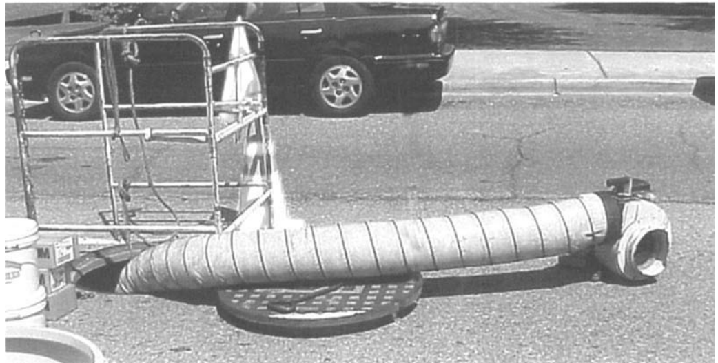
Figure 6.18 Gasoline-powered engines used to drive fans, as well as automobile exhaust emissions, may be a source of carbon monoxide introduced into spaces during ventilation operations.
