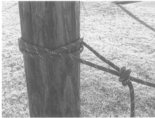
Figure 13.14 The clove hitch is used to attach to the anchor point in this example. The use of a safety knot with the clove hitch is critical.
