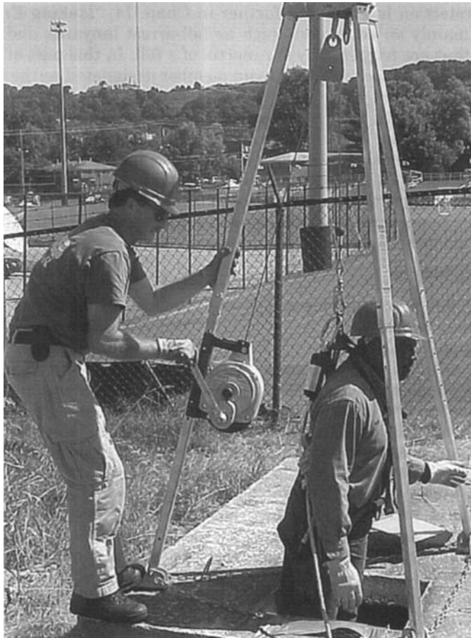
Figure 13.60 A tripod with a cable-type winch is commonly used to raise and lower personnel during vertical confined space operations.
