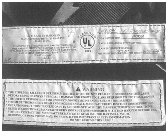
Figure 2.8 Manufacturers place certification labels on equipment meeting NFPA standard requirements.
