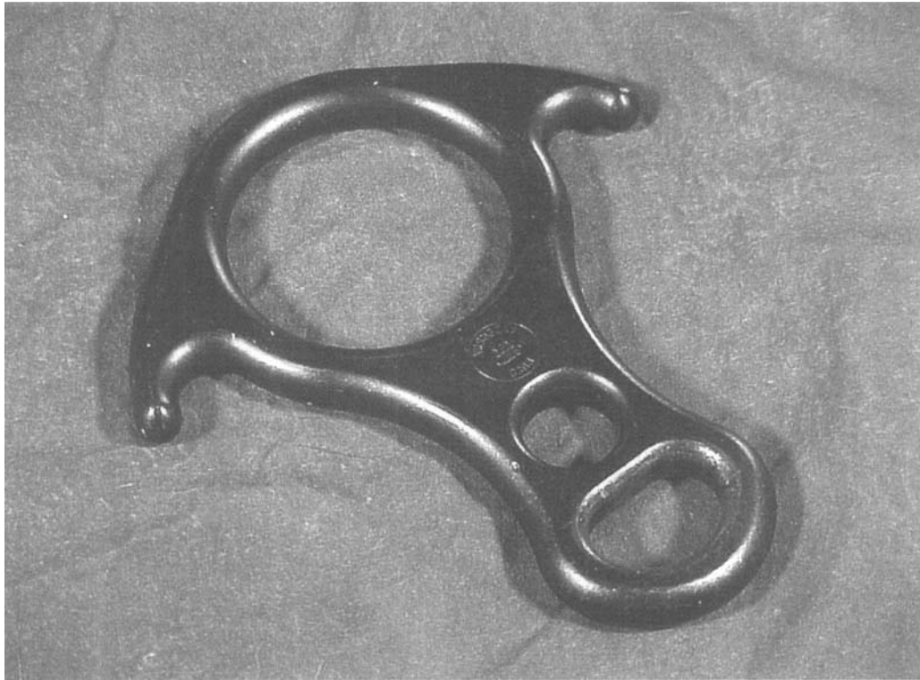
Figure 11.47 The figure 8 with ears is a descent control device used in belays, as well as short one-person rappels and lowering operations.
