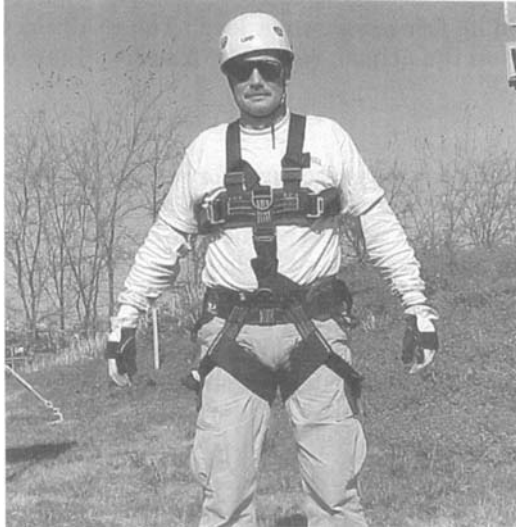
Figure 11.21 The CMC®/Roco™ seat harness used with the chest harness is an example of a harness with two-part construction that can be used together as a NFPA class III harness.
