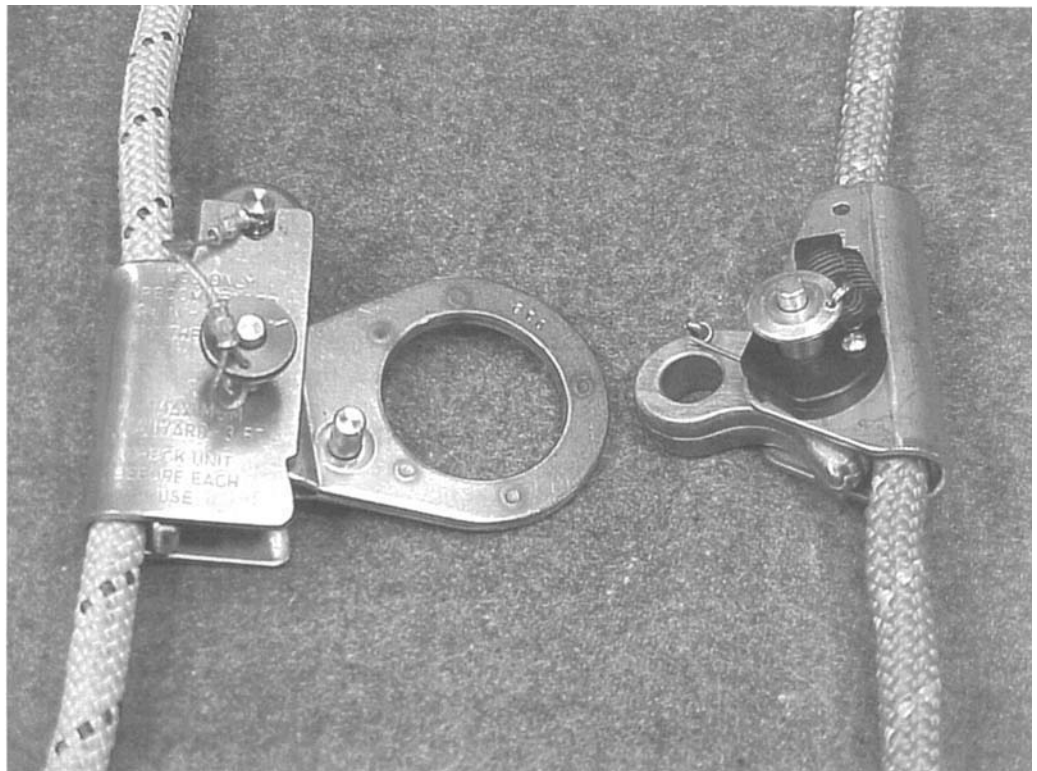
Figure 11.53 Both the MIO industrial rope grab and the Gibbs ascender can be used as a ratchet cam or a haul cam.
