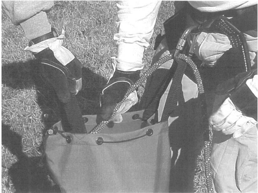
Figure 11.11 Rope can be stuffed quickly hand over hand into a rope bag for storage and easily deployed from the bag without tangling.
