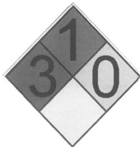
Figure 3.10 The NFPA label does not aid identification of a chemical by name, but shows its hazardous properties in color-coded diamonds using a numerical ranking system of 1 to 4.
