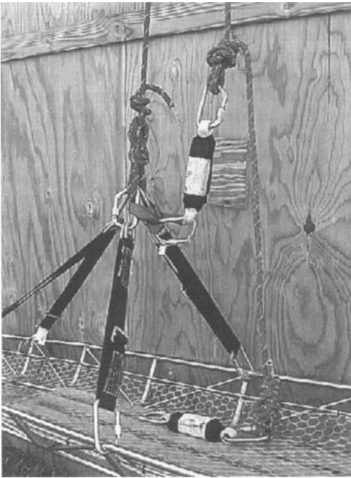
Figure 18.23 In this example, a doubled sling of webbing is passed through all the bridle hardware to create a point of attachment for the belay line at the litter bridle.
