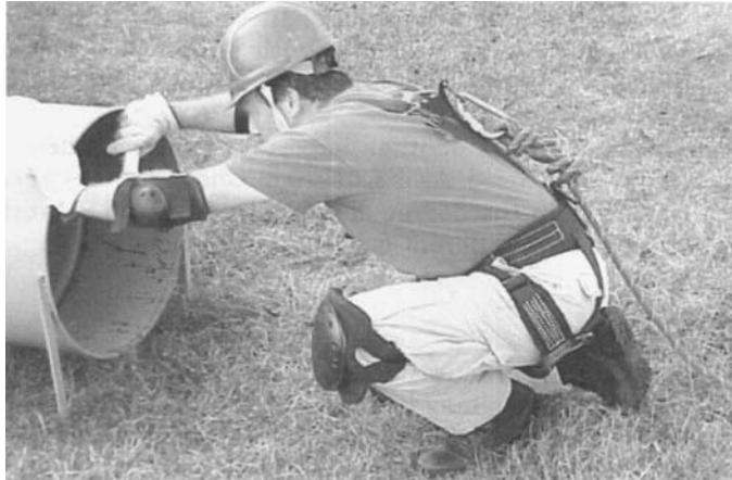
Figure 14.3 Harnesses and tag lines are standard confined space equipment, and kneepads and elbow pads can provide abrasion protection in tight spaces.
