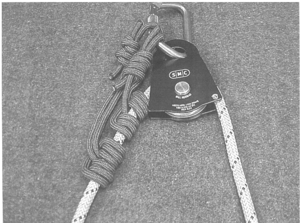
Figure 11.45 A Prusik minding pulley can be used with tandem triple-wrapped Prusik hitches.
