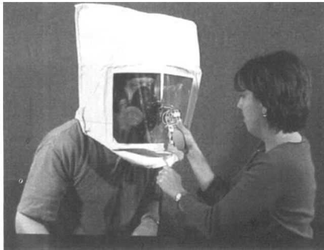
Figure 7.15 Qualitative fit tests use a challenge agent to check the fit of the facepiece to the face.
