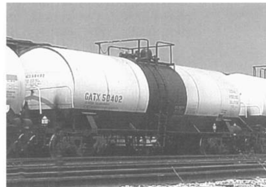
Figure 1.6 Transportation vehicles such as railcars and tank trucks are considered confined spaces.
