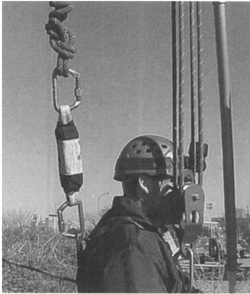
Figure 13.61 A shock absorber should be placed between the end of the safety belay line and the person who is being raised or lowered. The shock absorber will prevent shock loading of the system that could cause severe personal injury and damage or failure of anchors, ropes, and other system components.
