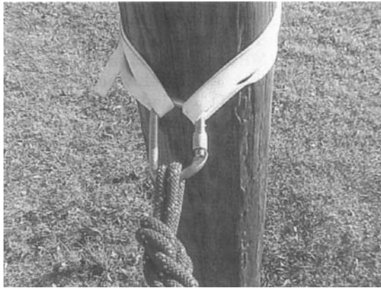
Figure 13.7 Avoid triloading carabiners when basket hitching around wider anchors.
