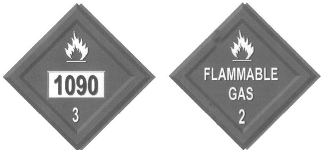
Figure 3.9 The DOT label gives information in four ways: color, symbol at the top, words stating the hazard class, and class number at the bottom.
