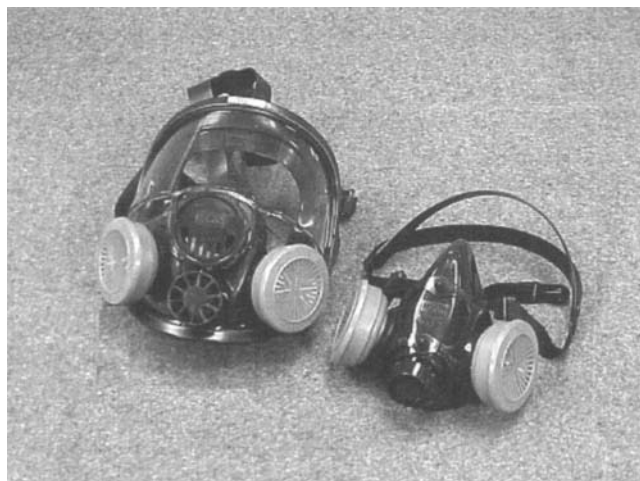
Figure 7.3 Employers can choose either full-facepiece or half-mask respirators for the protection of their employees.
