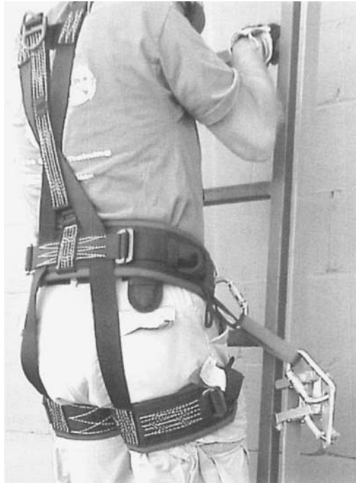
Figure 14.9 This inertial brake moves up or down a rail mounted to a ladder, but locks against the rail for fall-arrest if the climber falls.
