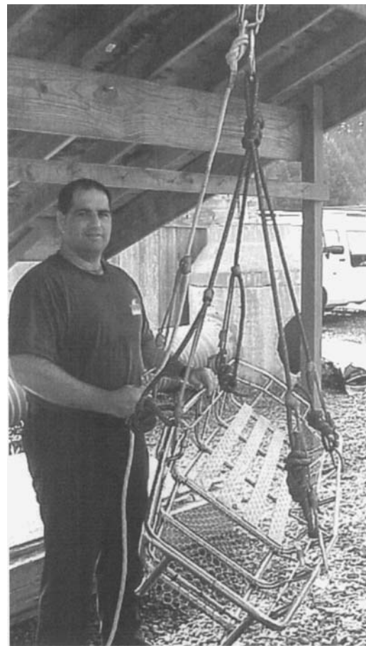
Figure 18.25 This rope bridle has legs that are universally adjustable using Prusik hitched loops of accessory cord. It also has a tender line that provides convenient positioning of a litter tender.
