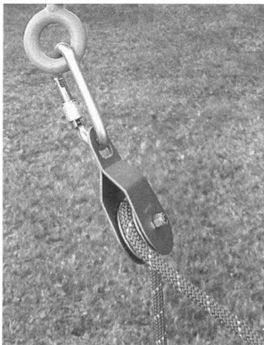
Figure 13.57 Beware of “hard linking” directional pulleys. The lack of flexibility can prevent the pulley from aligning properly with the rope.
