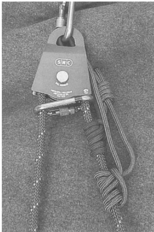
Figure 13.67 To enhance the effectiveness of the Prusik minding pulley for hauling operations, position a personal carabiner just below the pulley and above the Prusik hitches.
