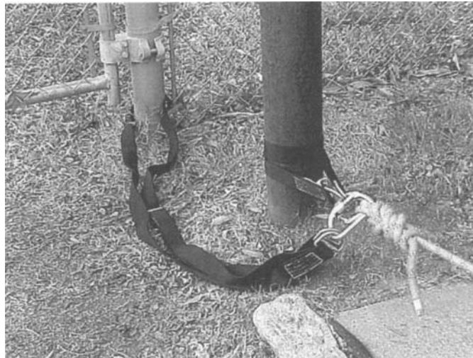
Figure 13.18 Excessive slack between the primary and secondary anchors, as seen here, will severely shock-load the system if the primary anchor fails.
