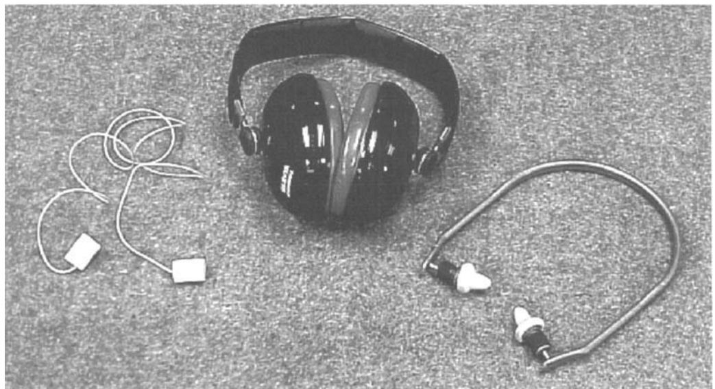
Figure 9.4 Hearing protective devices such as these earplugs, semi-inserts, and earmuffs block noise from entering the ear.
