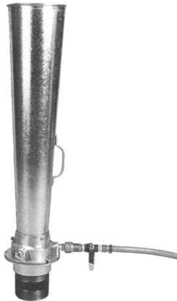
Figure 6.4 The Petro-Vent® by Air Systems International is a venturi eductor fitted with an adapter that allows it to thread directly to the 4-in vent pipe found on many storage tanks. (Photograph courtesy of Air Systems International.)
