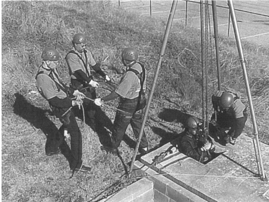
Figure 13.48 Team members perform an offset belay to lower a load with a MA system.
