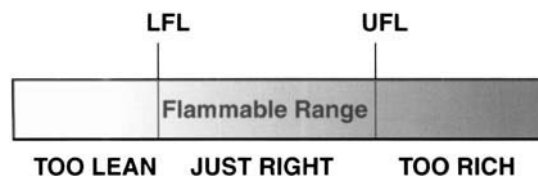
Figure 3.7 Below the lower flammable limit (LFL) the air-fuel mix is “too lean” to burn; above the upper flammable limit (UFL) it is “too rich” to burn. In the range between the limits, the mixture is just right and will ignite if an ignition source reaches it.
