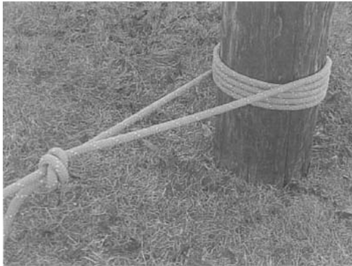
Figure 13.12 The tensionless tie-off is one method that can be used for attaching ropes to anchor points. This tensionless tie-off is wrapped 4 times around the anchor, and the end of the rope is tied back to the standing part of the rope with a barrel knot.
