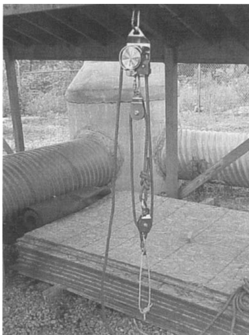
Figure 13.53 The Griptech SP1 is a manufactured MA system.
