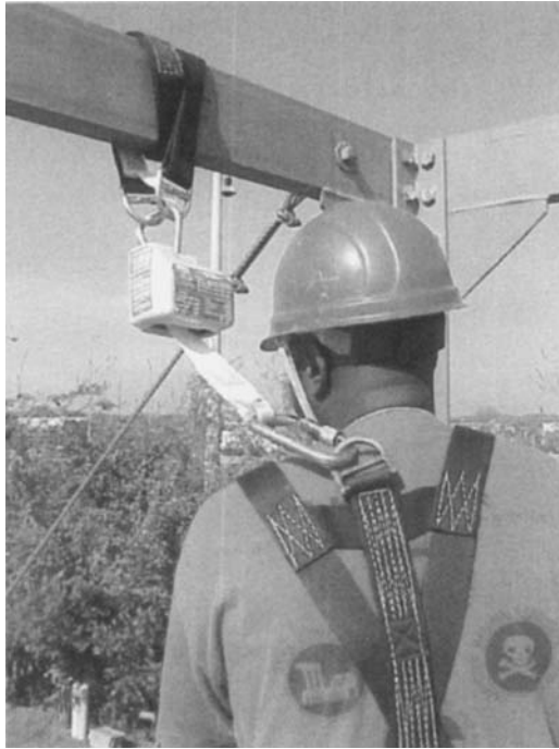
Figure 14.10 This retractable lanyard has an inertial lock for fall-arrest.
