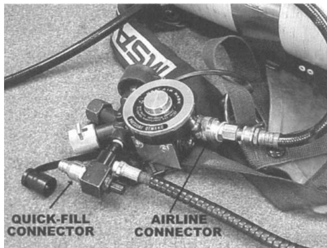
Figure 7.9 This regulator is equipped with both an airline connection and a Quick-fill® connector.
