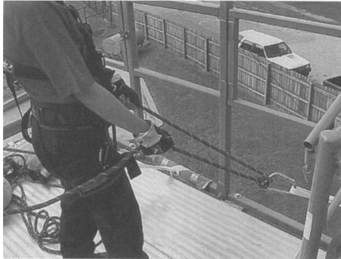
Figure 13.62 The Munter hitch is a belay technique that can be used on the safety belay line during lowering and hauling operations.
