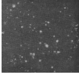
Figure 4. A foil of Pd-Ag alloy (top) was heated in vacuum to 600°C, exposed to D 2 gas for 88 hrs, and placed on photographic film.(26) The tritium (light areas) is spread over the surface but distribution is not uniform. A total of 1.5x10 12 tritium atoms are estimated to be in the sample based on calibration using a sample made to contain a known amount of tritium. The longest dimension is about 4 cm. Titanium (bottom) shows the same ability to make tritium but the sites were very local and fewer in number.
