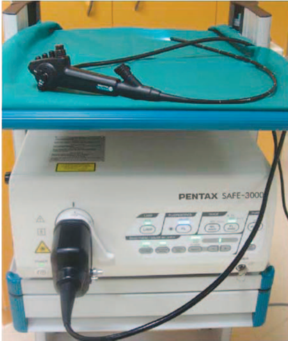
Figure 30.3 Pentax SAFE-3000 autofluorescence bronchoscopy system with flexible video-chip bronchoscope (Pentax Corporation, Tokyo, Japan).
