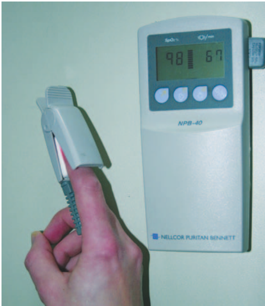
Figure 6.28 Pulse oximeter (Covidien-Nellcor™); transmission mode, display with blood oxygen saturation (left) and heart rate (right).
