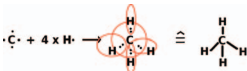
Figure 2.17 Formation of chemical bonds in methane, CH 4 . Each hydrogen atom contributes one electron and the carbon atom four electrons, all indicated by the dots (left-hand
