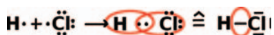
Figure 2.16 Formation of a chemical bond in hydrochloric acid, H–Cl. The hydrogen atom contributes one electron and the chlorine atom seven electrons, all indicated by the dots
