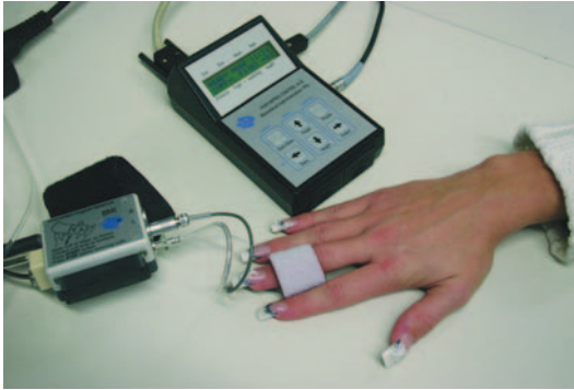
Figure 6.29 Portapres™ (Finapres Medical Systems BV) blood pressure monitor; inflatable finger cuff and control unit.
