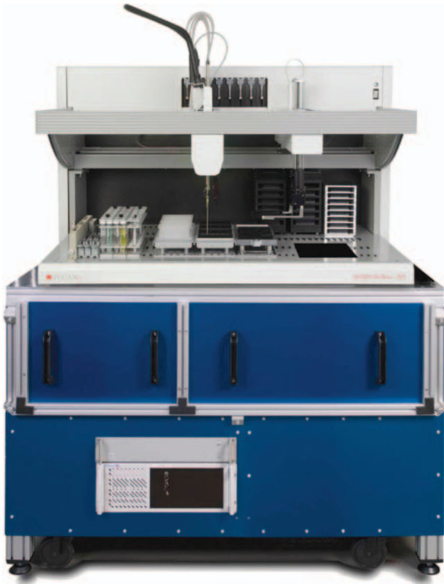
Figure 10.17 Demonstrator for the new crystallization system. A liquid-handling system for sample preparation is positioned above the optical modules inside the housing.
