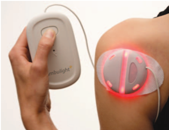
Figure 22.2 Ambulight PDT – a wearable light source for skin cancer treatment consisting of a self-adhesive light source and a separate battery-powered control unit.
