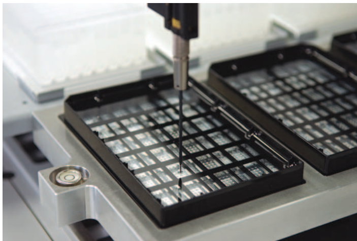
Figure 10.5 A novel microplate was developed for the new crystallization system. This figure shows how the protein solution is applied under paraffin oil. A series of six droplets of various
