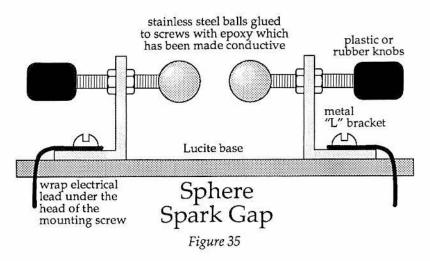
been made conductive by some additive or has been coated with a little silver paint in order to make electrical contact between the sphere and the rod. The rod is threaded through a metal stand, and plastic handles are added to allow the spheres to be turned while the device is operating. The spheres must be at least 3 sphere diameters above the base to prevent distortion of the electrical field which can give inaccurate results.
