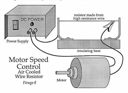
between two copper posts. One side of the wire is tied to a 12v (or similar) power supply. A wire coming from your motor is attached to an alligator clip which can be moved along the wire to increase or decrease the motor speed. This method works extremely well. However, be aware that the wire can become red hot when supplying current to the motor! Make sure to house it safely.
