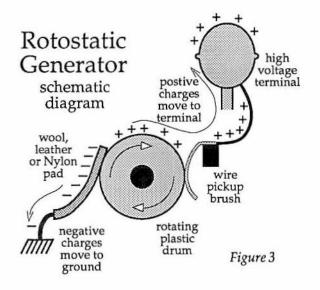
If your generator is well made it will generate enough power to light a neon bulb (Ne2 type), levitate styrofoam, and arc a spark perhaps as long as 1/16 to 1/8 inch – all of this while still being perfectly safe to touch. When touched, your generator will give your finger only a very light "pop" much like a very small static discharge from a doorknob. As an interesting side note, if you can feel a static charge at all, it will be at least 3,500 volts!
