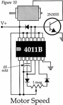
Control Solid State Figure 10 shows a very accurate and stable means of controlling a DC motor. An integrated circuit and power transistor are used to send a stream of pulses to the motor. As the pulse rate increases, the motor speed also increases. By simply turning the potentiometer, you can adjust motor speed at any time. For mid-sized DC motors a very large heat sink or water cooling is required for the transistor.
