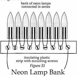
Letting a spark periodically jump the gap will trigger the lamp bank. Attaching the bank directly to generator can draw enough current from the generator (load it down) such that it never reaches peak voltage. With a small Van de Graaff a steady stream of bright flashes will occur every two or three seconds.
