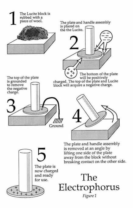
Slowly remove the metal plate by the handle, drawing it away from the Lucite at an angle. The metal plate now holds the charge you seek. Having charged your electrophorus, you can perform the experiments with Von Guericke's globe mentioned above including attracting hair, styrofoam and other small objects.
