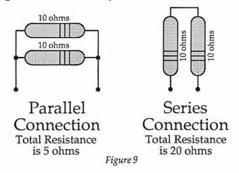
Power resistors are inexpensive, and if you buy a handful of different values you can connect them in parallel or series to get a wide variety of different values. Keep in mind that resistors have two ratings, the power handling capacity measured in Watts, and the resistance measured in Ohms.
