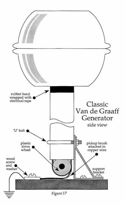
sphere of the proper dimensions. Besides, two bowls allow easy access to the top roller and brushes, and I wanted to test my hunch that almost as much power could be obtained from the bowls if the edges were heavily doped and insulated as could be obtained from a traditional spherical terminal.
