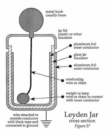
Electricity often seems to find some way to get into the jar without telling you. I was once shocked by a Leyden jar that was standing a few feet from a generator. It was not until I observed the generator and Leyden jar in a completely darkened room that I noticed a blue glow around a length of wire which had been acting as an aerial above the Leyden jar and had partially charged it although it was not even directly connected to the generator!
