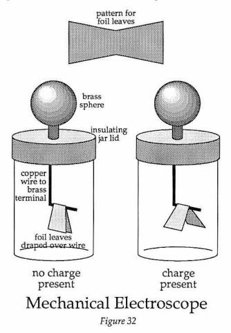
mechanical electroscope of this type can also be used to measure voltage. Heavier leaves require greater voltages to separate them. Therefore, the distance the leaves move away from one another indicates a relative voltage.
