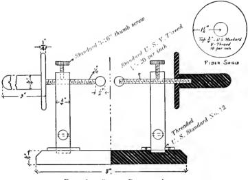
FIG. 16. - SIMPLE PRIMARY AIR-GAP.
