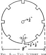
FIG. 8. — END SUPPORT FOR Secondary of Oscillation Transformer.
