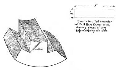
FIG. 29 - SELF-STARTING DEVICE.
