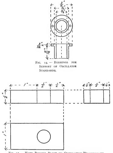
FIG. 15. - HARD RUBBER BLOCK ON OSCILLATION TRANSFORMER.
