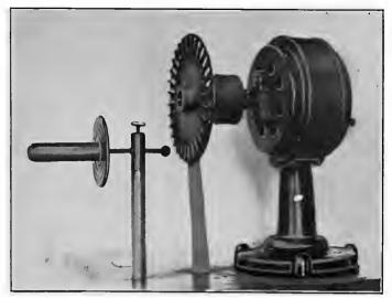
PLATE IV. - Motor-driven Interrupter.
