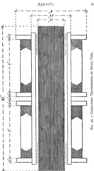
The secondary winding of this transformer consists of two sections of No. 32 B. & S. gauge double cotton covered copper wire. First saw out of  $\frac{1}{4}''$  stock four circular pieces of wood, 4" in diameter and having a  $2\frac{1}{4}''$  hole in the centre. Slip these on the primary to the positions shown in the figure. The two end ones are  $\frac{1}{2}''$  from the ends of the core and the middle ones are  $\frac{1}{4}''$  apart.
