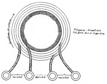
FIG. 33. - CONNECTIONS FOR PRIMARY OF TRANSFORMER.
