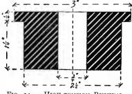
FIG. 34 - HIGH-TENSION BUSHING.
