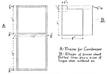
FIG. 7. - CONDENSER FRAME AND BRASS CONDENSER SHEET.
