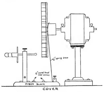
FIG. 21. - SECTION OF THE MOTOR INTERRUPTER.
