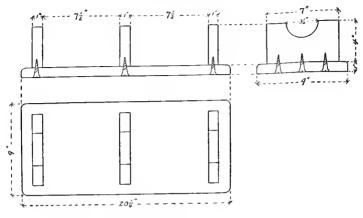
FIG. 5. — FRAME FOR SECONDARY OF TRANSFORMER.
