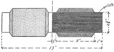
FIG 38. - PRIMARY AND CORE OF TRANSFORMER OF 7" COIL.
