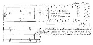
Frame on which stator coils are wound.
