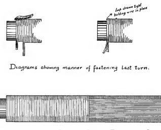
FIG 1. — METHOD OF FASTENING PRIMARY TERMINALS — COMPLETED PRIMARY.
