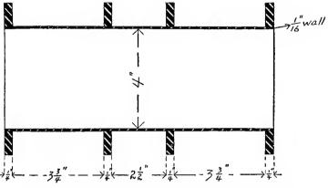
FIG. 39. - SECONDARY BOBBIN OF TRANSFORMER OF 7" COIL,
