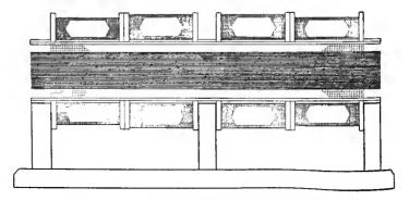
FIG. 6. - SECTION OF COMPLETED TRANSFORMER.
