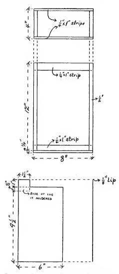
FIG. 40. - PLATE AND FRAME OF CONDENSER.
